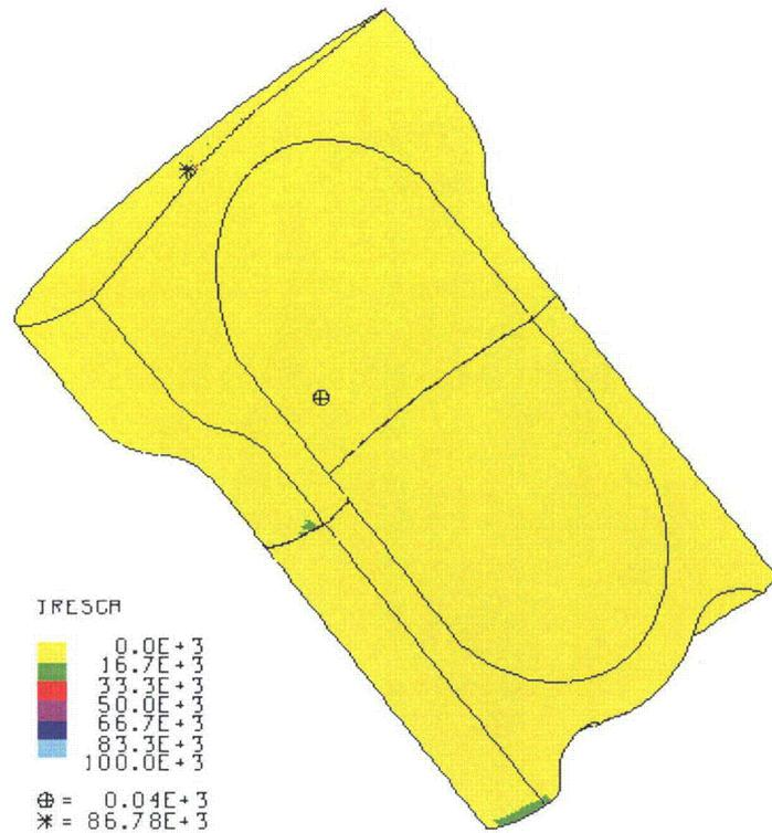
Figure 2-489. Plot of Tresca Stress in the TB-1 for HAC Run 20, 731 g Angled Plutonium Metal Hollow Cylinder, CGOC Impact when Plate Velocity Reaches Zero
