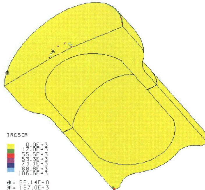
**Figure 2-393. Plot of Tresca Stress in the TB-1 for HAC Run 5, SC-2, CGOC Impact, Support Structure 45° when Stress is a Maximum**
