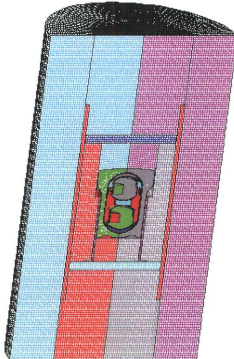
Figure 2-346. Finite Element Mesh for the SC-2, Side Impact, 45° Support Structure, Friction 0.2
