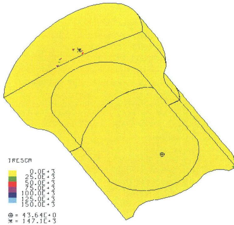
**Figure 2-450. Plot of Tresca Stress in the TB-1 for HAC Run 15, 831 g Angled Plutonium Metal Hollow Cylinder, CGOC Impact**
