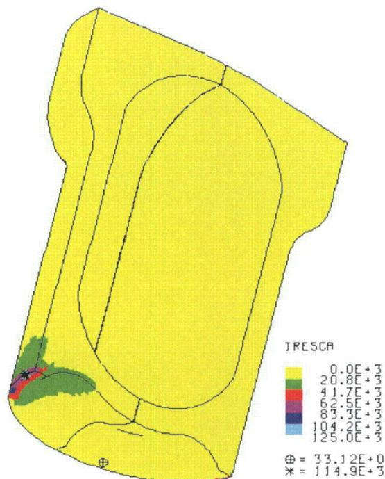
**Figure 2-465. Plot of Tresca Stress in the TB-1 for HAC Run 17, 731 g Plutonium Metal Hollow Cylinder, Side Impact when Plate Velocity Reaches Zero**
