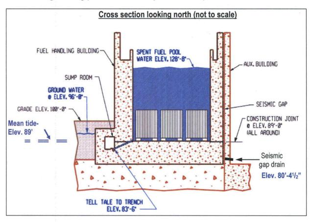
Fuel Handling Building (Cross-Section at Spent Fuel Pool):
