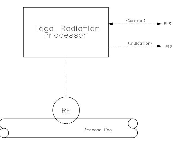
**Process In-Line Radiation Monitor**
