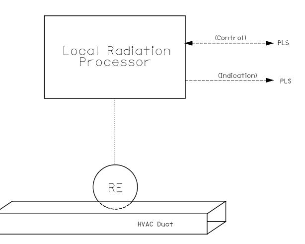
**In-Line HVAC Duct Radiation Monitor**
