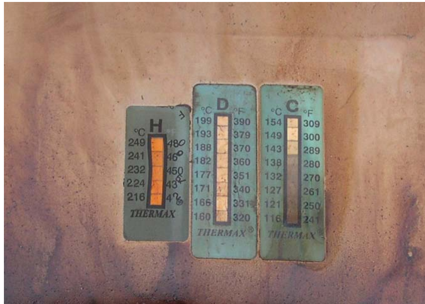
Figure 3-8 Temperature Strip Condition After CTU Burn Test
