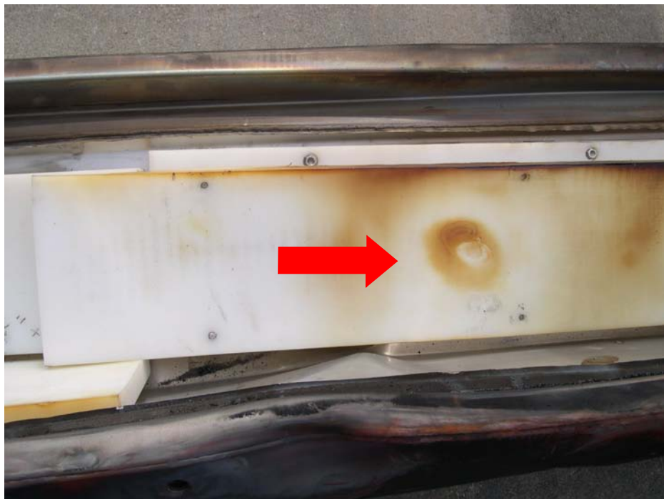
Figure 3-44 Localized Melt Spot in Lid Moderator Block
