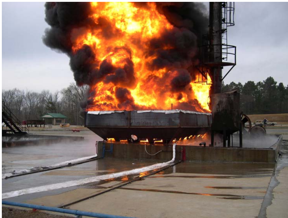
Figure 3-4 December 15, Impact Limiter Burn Test
