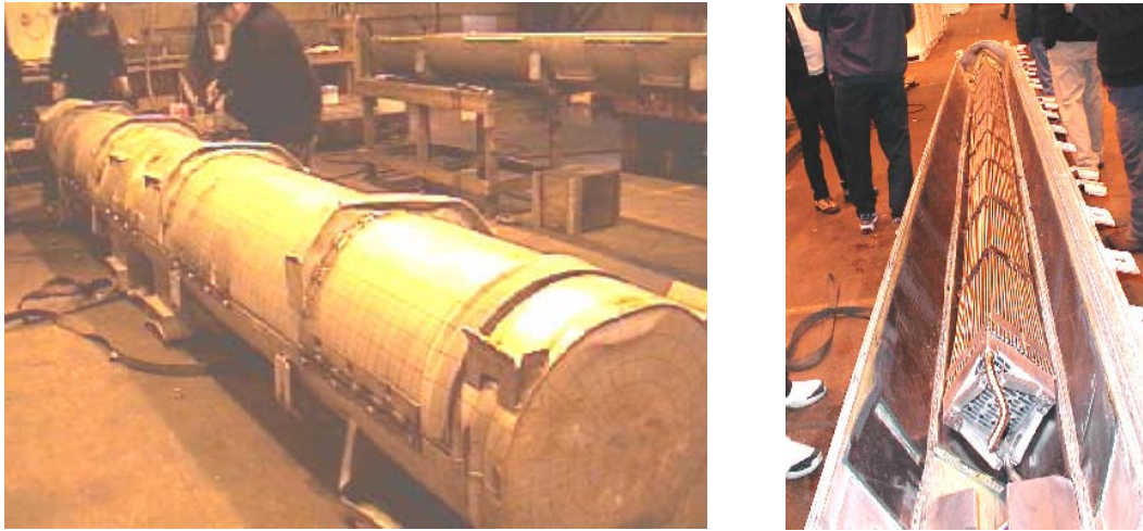
Figure 2-127 Traveller Prototype Clamshell and Bottom Impact Limiter After Test Series 3
