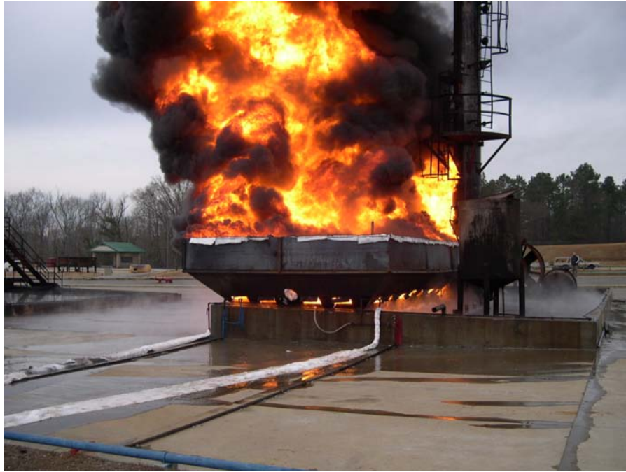
Figure 3-6 Traveller CTU During Pool Fire Test
