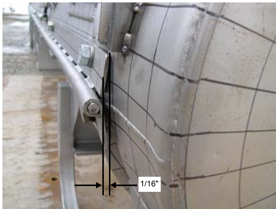
Figure 2-147 Hinge Separation at Bottom Nozzle End From Test 2
