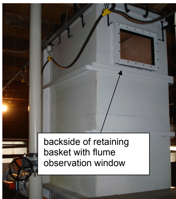
Figure E.3-9 Flume Observation Window
