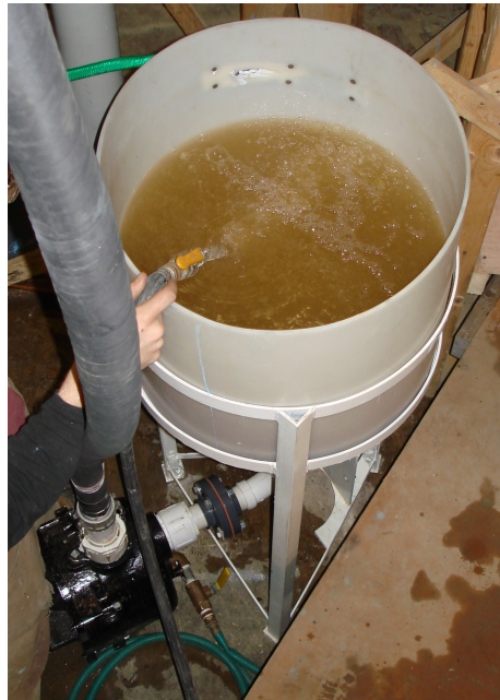
Figure E.3-8 Debris Introduction Tank and Pump
