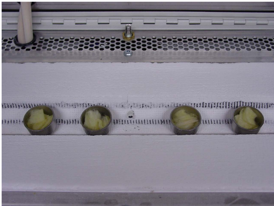
Figure D.2-2 NUKON Insulation before Heat Treatment
