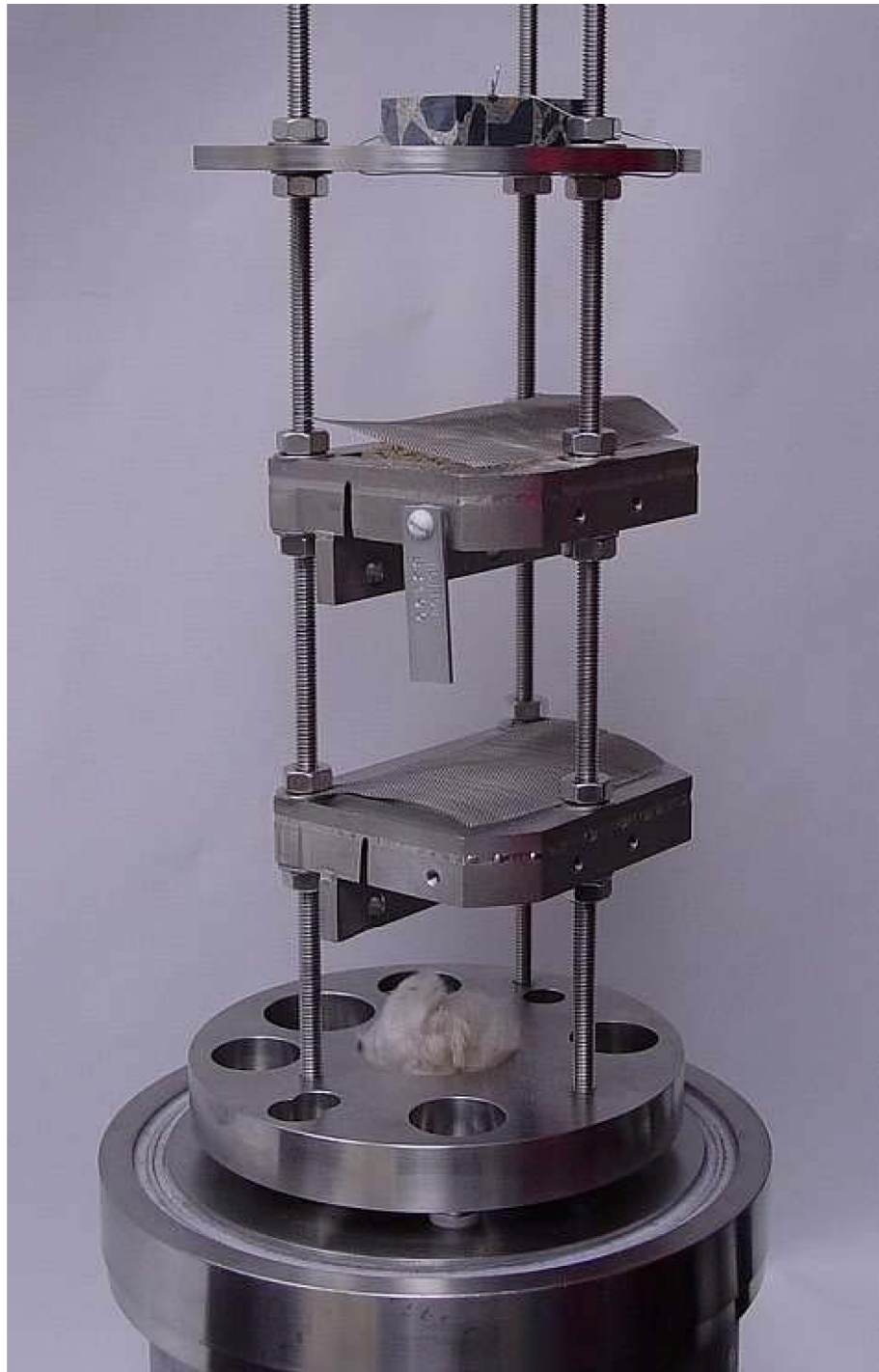
Figure D.2-8 Assembled Autoclave Internals
