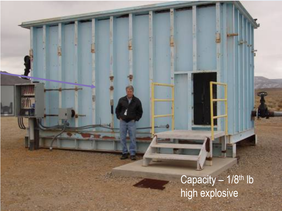
50 m 3 full sample recovery explosive aerosolization chamber
