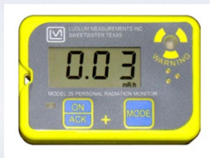
Area Radiation Detector: Release of radiation triggers alarm and data transmission
