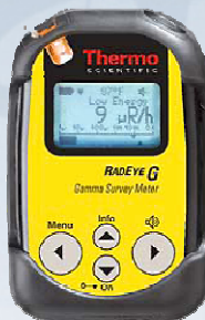
Personal Radiation Detector (PRD): Used by response force
