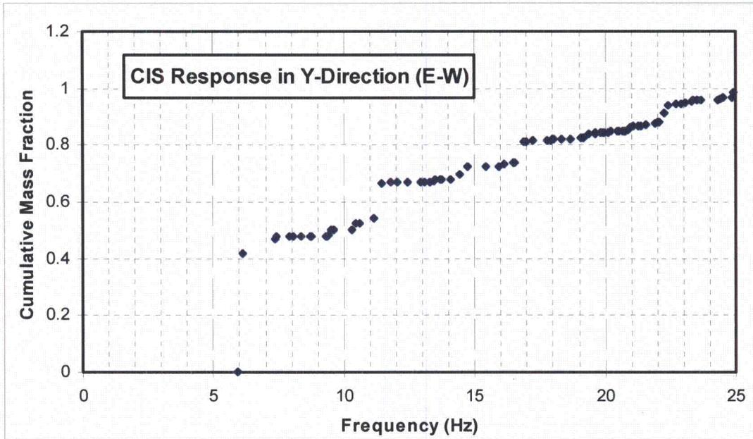
MHI US-APWR CIS ANSYS Model Transfer Functions Y-Direction
