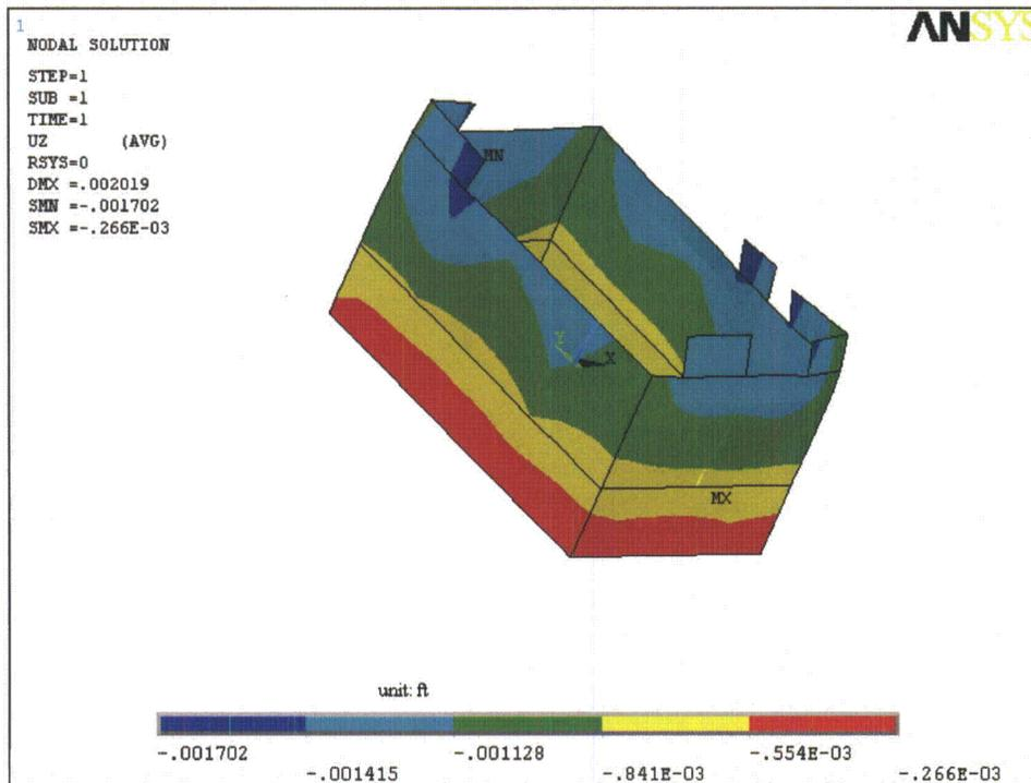
Vertical Displacement Contour: 1-g Vertical Load on ANSYS Dynamic Model
