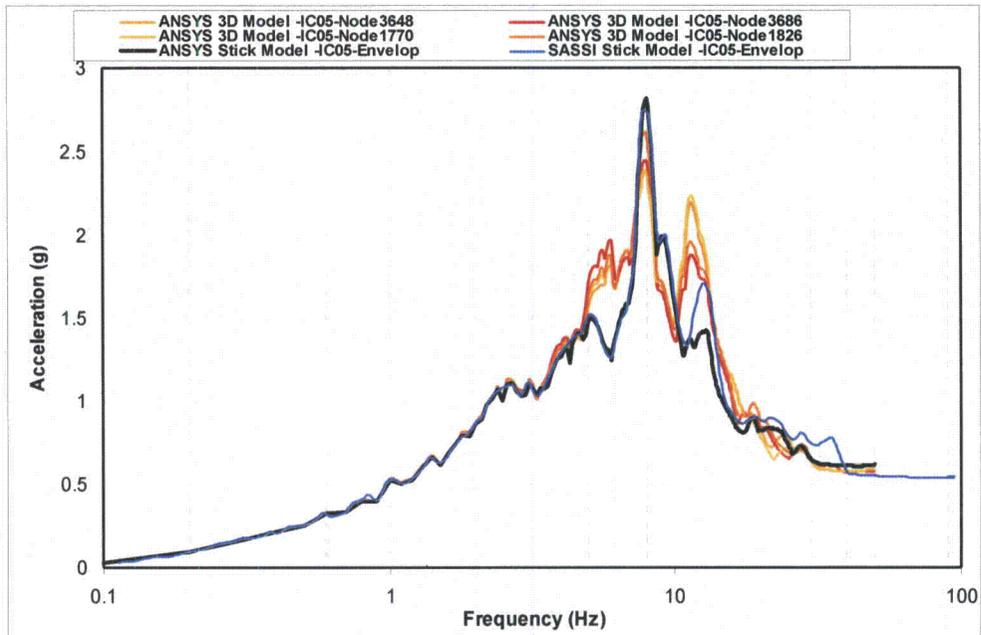
Revised Figure 5.3.5.3-4 Acceleration Response Spectrum Node IC05, NS Direction
