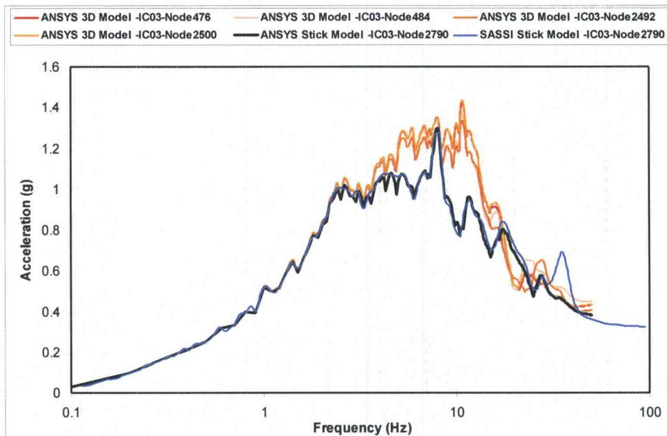
Revised Figure 5.3.5.3-1 Acceleration Response Spectrum Node IC03, NS Direction
