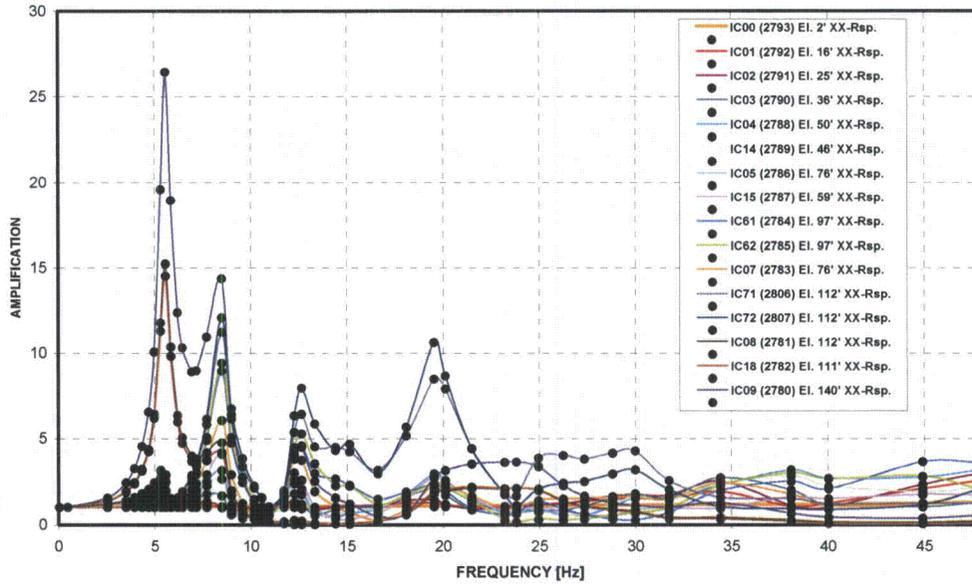
Preliminary Revised Figure 5.3.5.2-1 ANSYS Dynamic Model Transfer Functions, X-Direction
