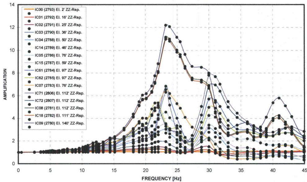
**Preliminary Revised Figure 5.3.5.2-3 ANSYS Dynamic Model Transfer Functions, Z-Direction**
