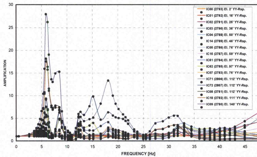
**Preliminary Revised Figure 5.3.5.2-2 ANSYS Dynamic Model Transfer Functions, Y-Direction**
