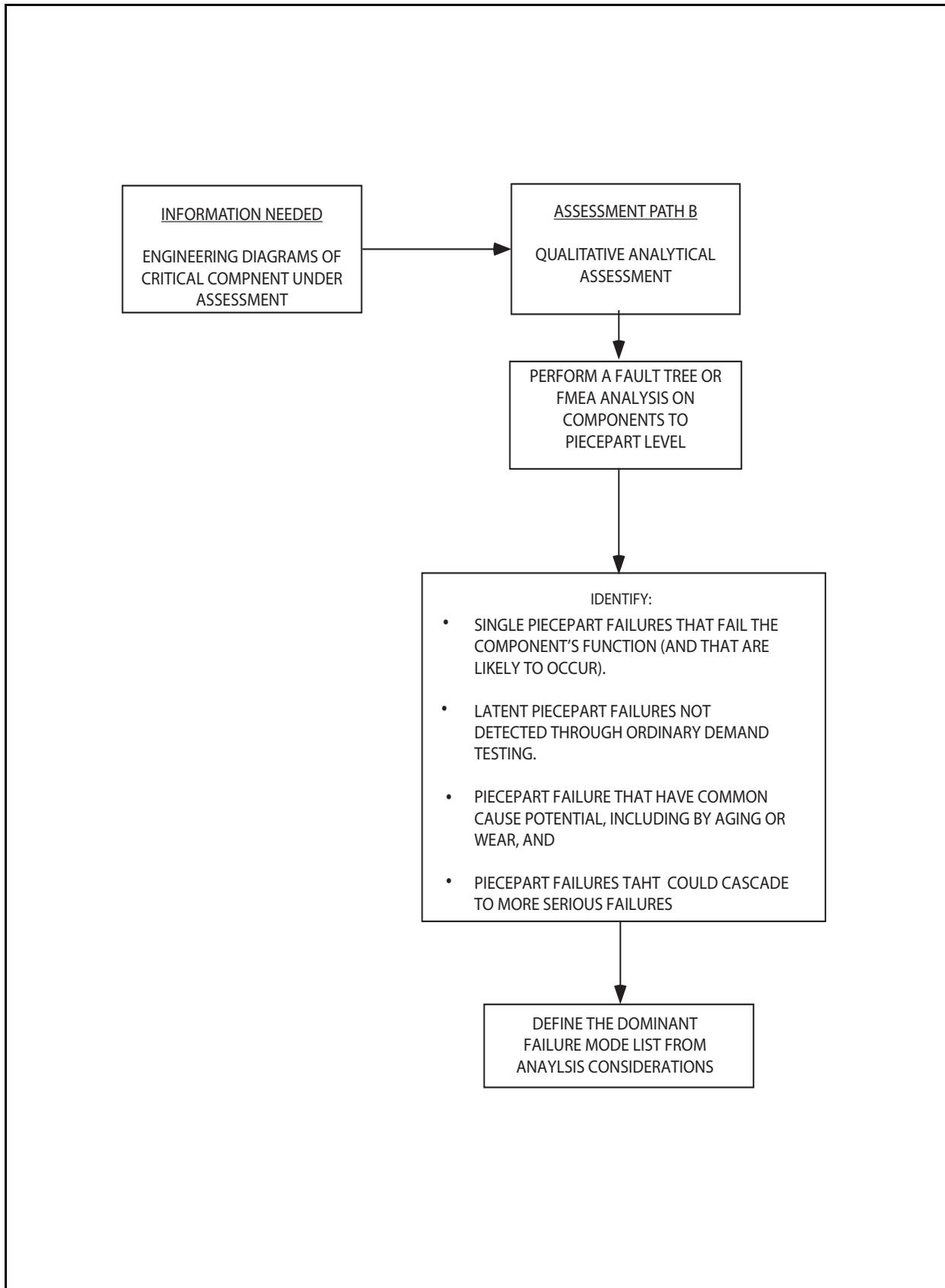
**Figure 17.3-4 Analytical Assessment to Define Failure Modes**
