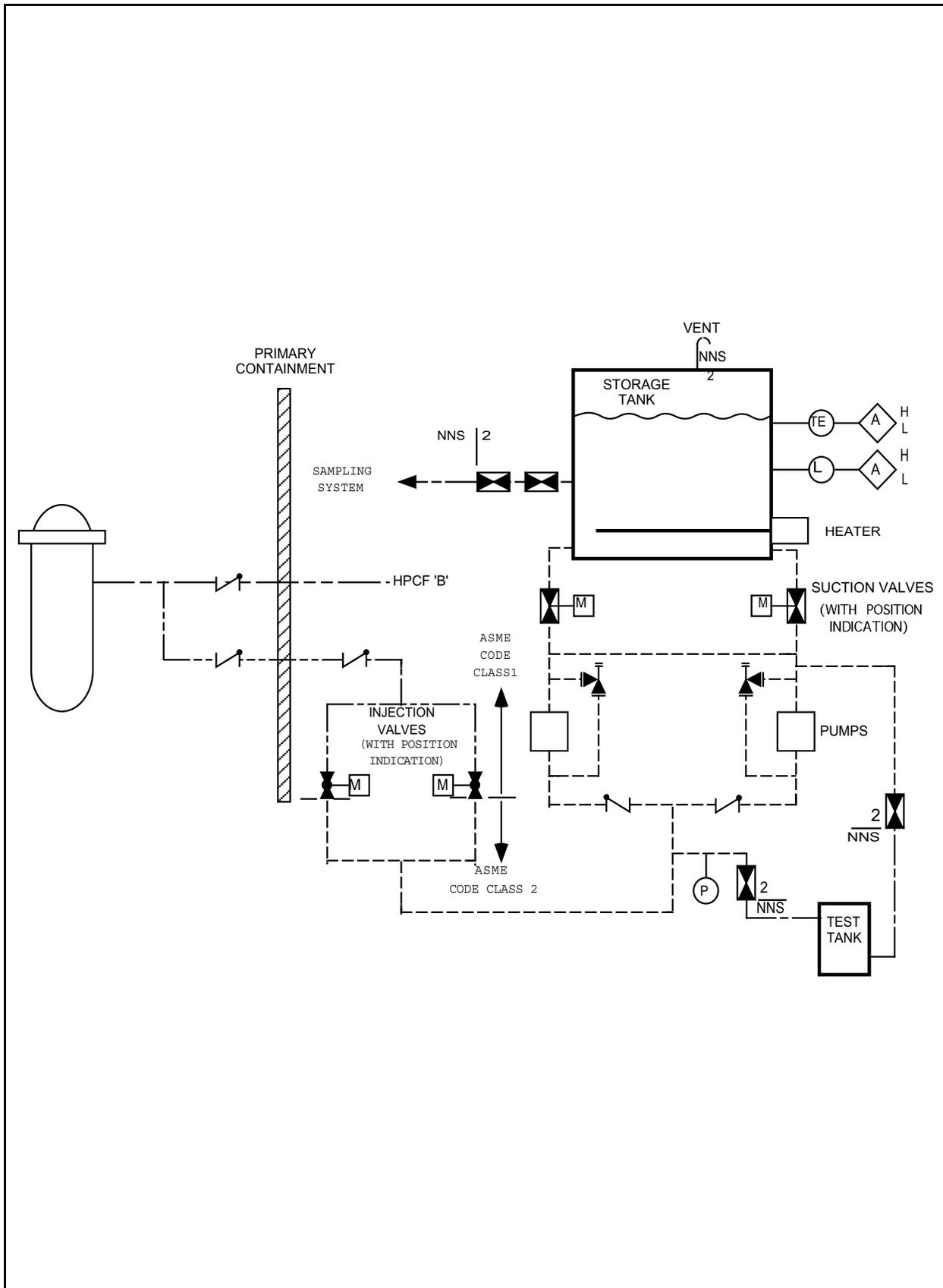
Figure 17.3-7 Standby Liquid Control System (Standby Mode)
