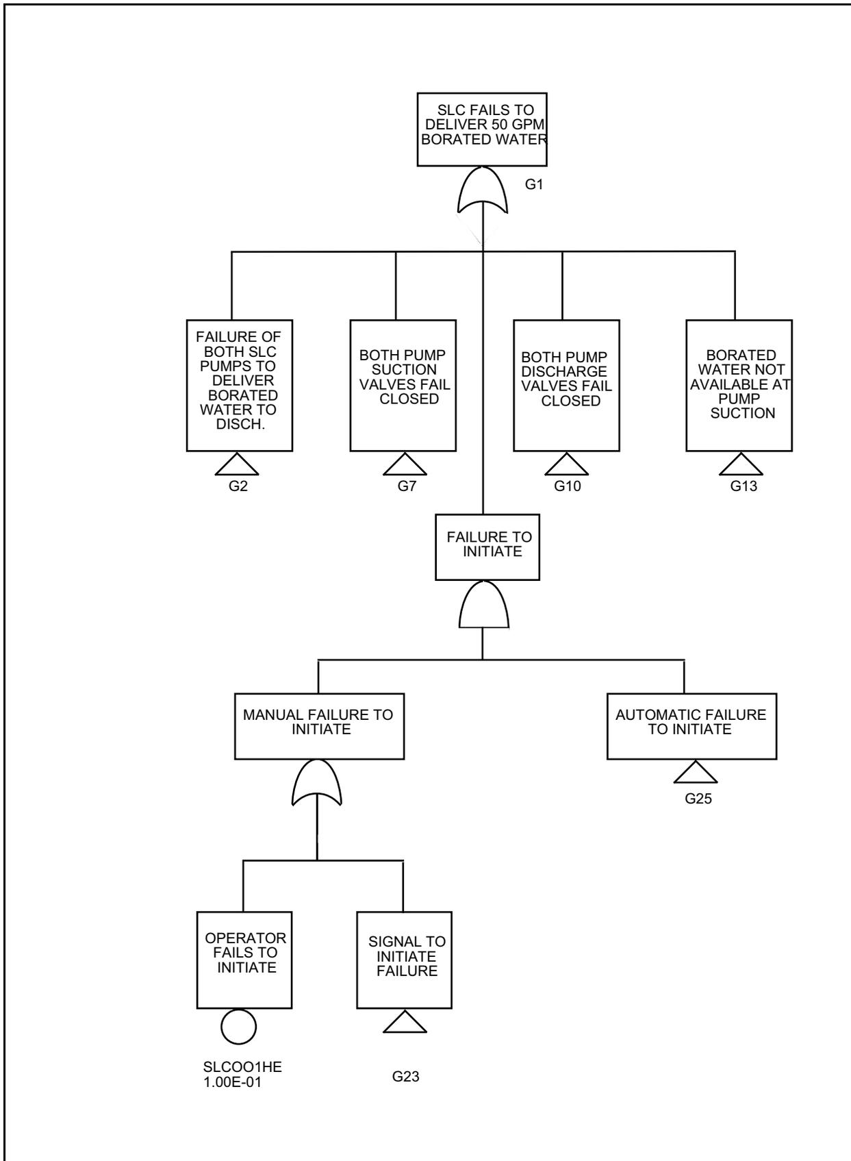
Figure 17.3-8 Standby Liquid Control System Top Level Fault Tree
