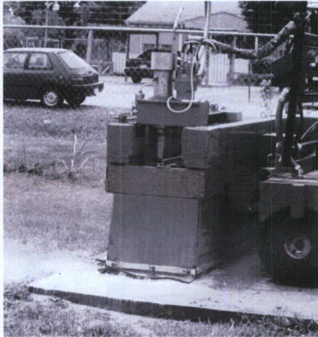
Figure 5.48 Equipment for removing concrete from surfaces.
