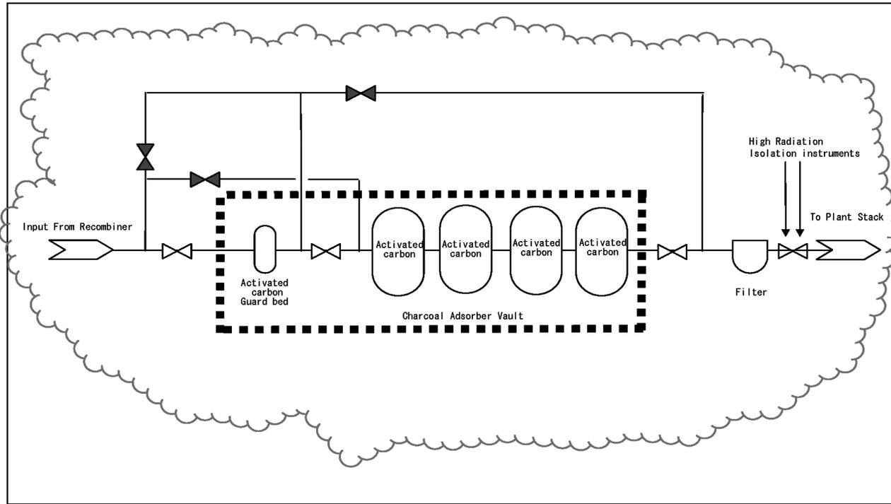
Figure 15.7-2 Offgas System (See Subsection 11.3)
