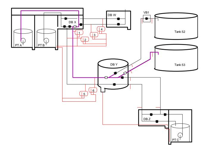
In this diagram, Diversion Box X has a large credited drain from the box into Pump Pit B. Therefore Diversion Box X is not a credited LEAK DETECTION LOCATION (waste cannot accumulate there). Diversion Boxes Y and Z also have drains, but these drains are too small to ensure that waste will not accumulate. Diversion Boxes Y and Z also have no weirs or similar devices to ensure that leakage into these boxes will be detected before the liquid exits the box.
