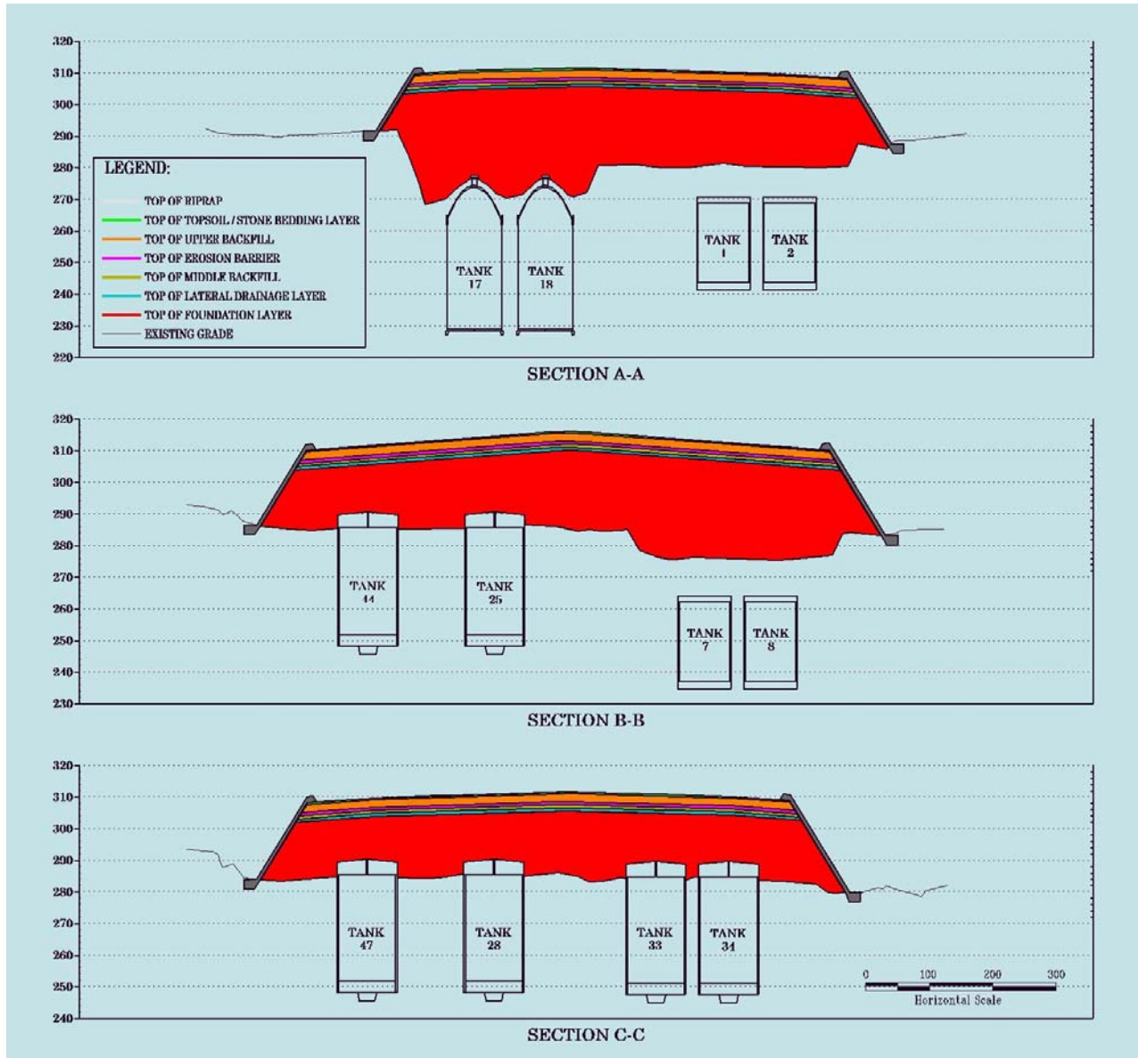
Figure 3.2-72: FTF Closure Cap Conceptual Design, Sections A-A, B-B, and C-C
