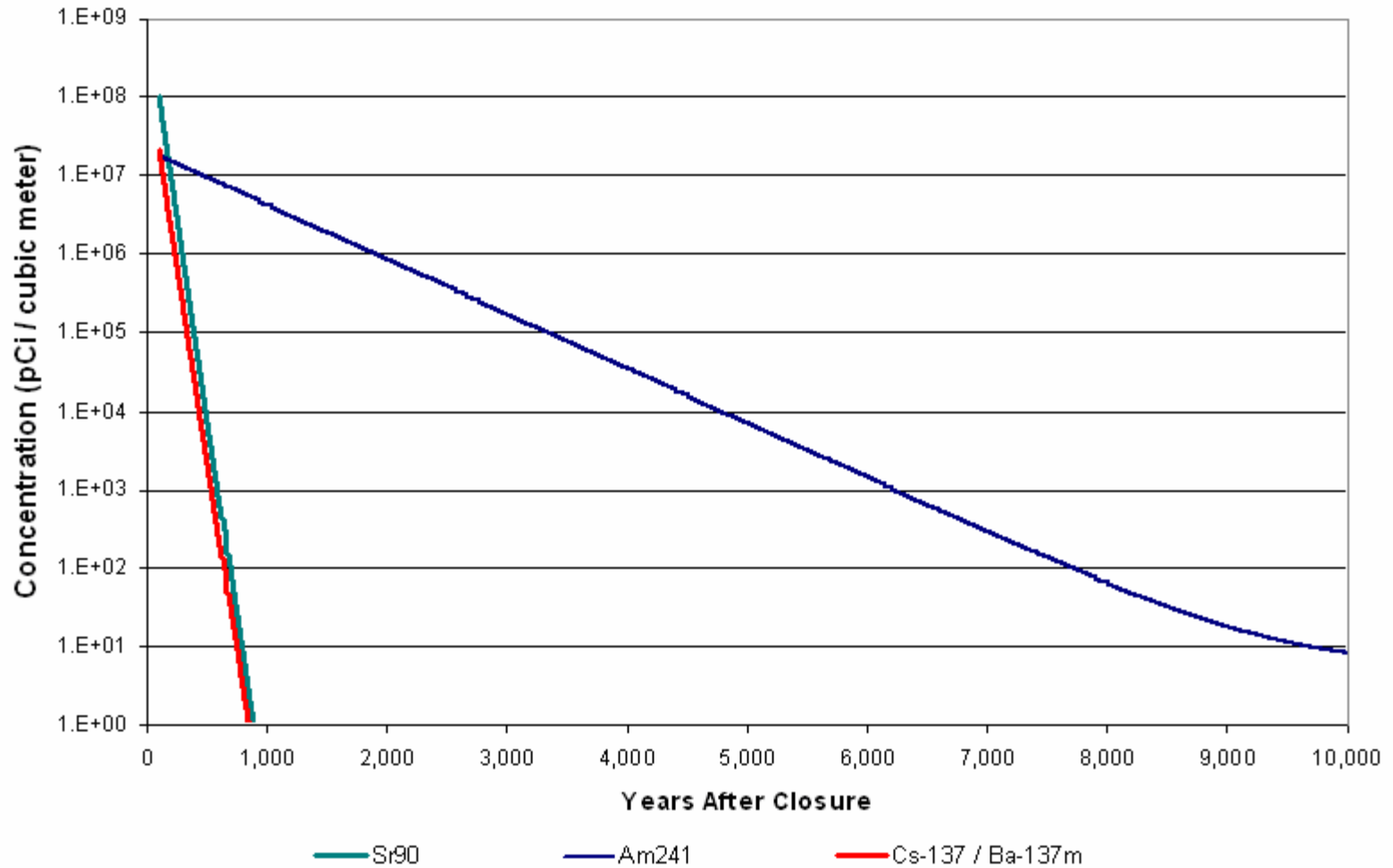
Figure 6.4-2: Concentration of Contributing Radionuclides in the Soil from Drill Cuttings
