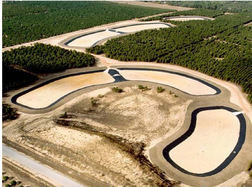
Highly-treated reclaimed water produced in the Orlando area is piped to large rapid infiltration basins (RIBs) as part of the CONSERVE project. This type of water resource development project could be constructed in the Northern Planning Region to offset the potential impacts of groundwater withdrawals.
