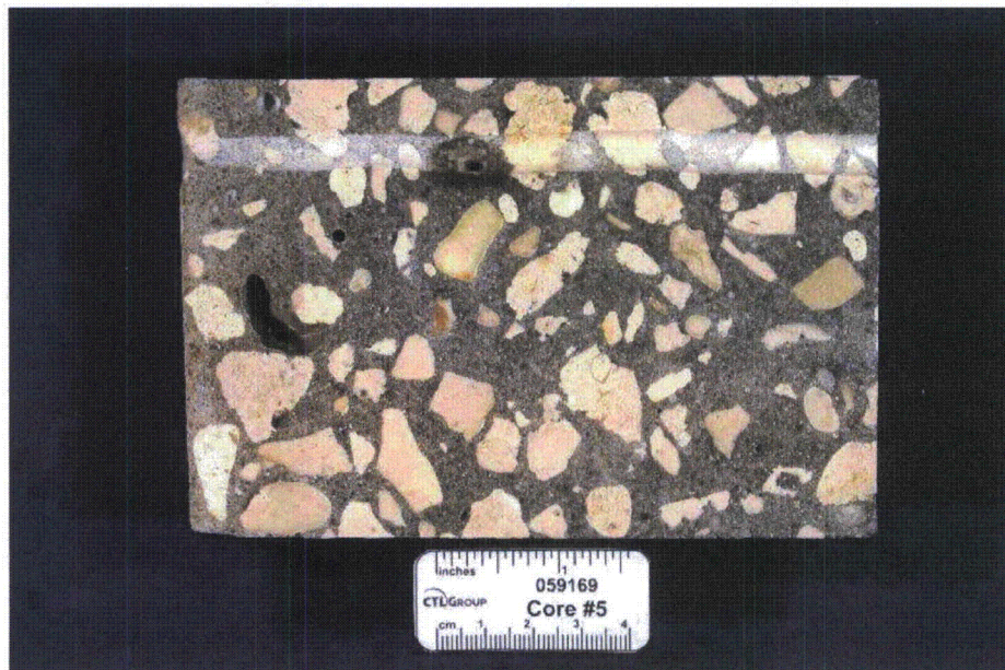
Fig. 4 View of the lapped surface of a portion of Core #5 showing the general appearance of the concrete.
