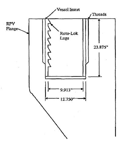
Reference Westinghouse (vendor) drawings 11073-179-003, rev. 03 and 11073-171-006, rev. 1. There are three sets of Roto-Lok lugs equally spaced around the inner circumference of the vessel insert.
