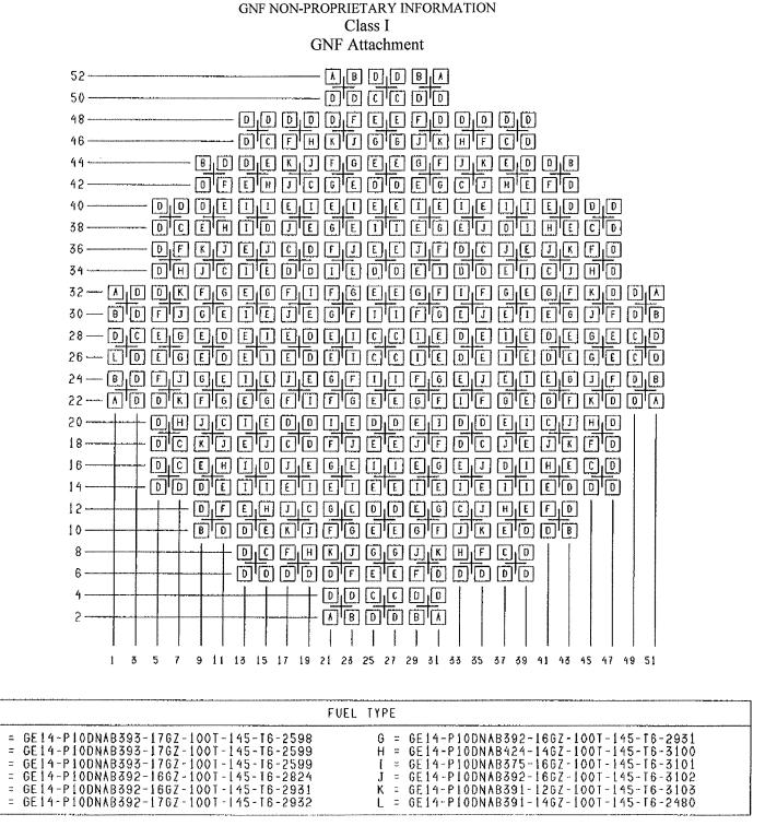
Figure 2. Previous Cycle Core Loading Diagram
