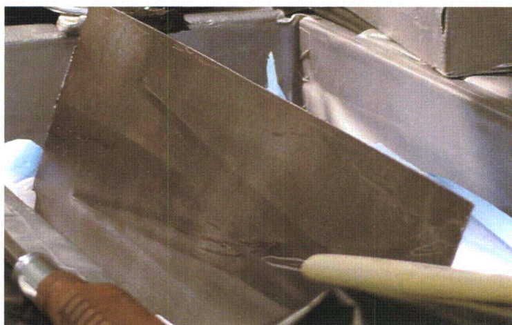
Figure 2-6 Photograph of CNS Capsule A Wrapper Showing Indentations which Indicate that the Capsule was Irradiated with the Dosimetry Wires out of the Charpy Notches
