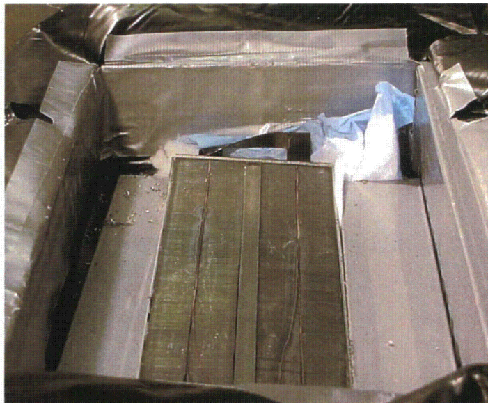
Figure 2-8 Photograph of CNS Capsule B Showing Fe and Cu Wires Out of the Charpy Notches (Capsule U-Hook is at Top of Photograph)
