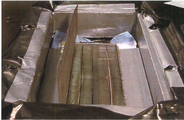
Figure 2-9 Photograph of CNS Capsule C Showing Fe and Cu Wires Out of the Charpy Notches (Capsule U-Hook is at Top of Photograph)
