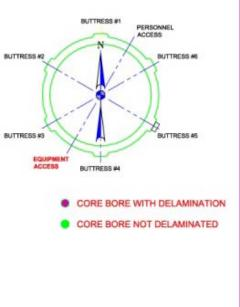
**Conclusion** – Physical observation of core boring has validated the delamination boundary, as accurately predicted by Impulse Response (IR).
