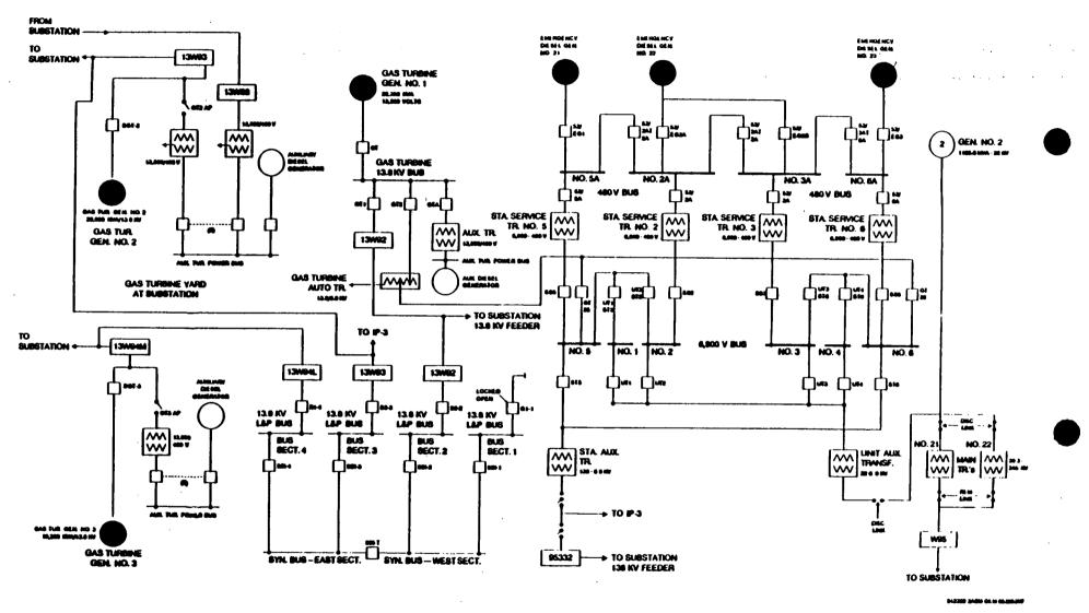
FIGURE 1. INDIAN POINT 2 ALTERNATE AC POWER SYSTEM
