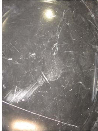
Post Test Damage - Marring
