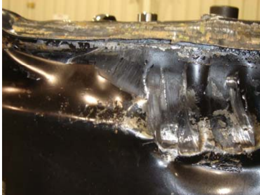
Side View - Damage from Impact of Bolt Lug onto Side Wall
