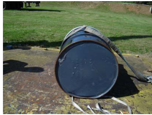
End View – Bottom End Damage
