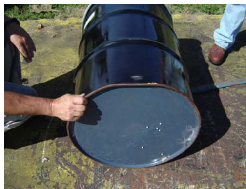
View of Bottom End Post Impact
