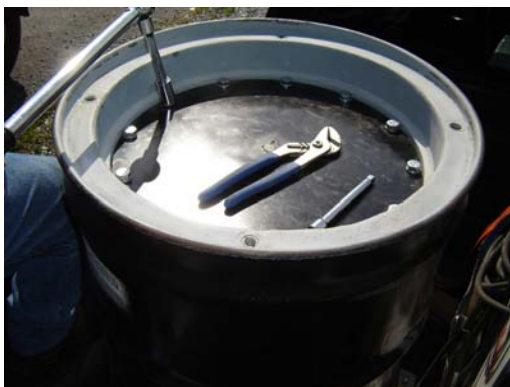
Bolted Inner Blind Flange and Top Gasket
