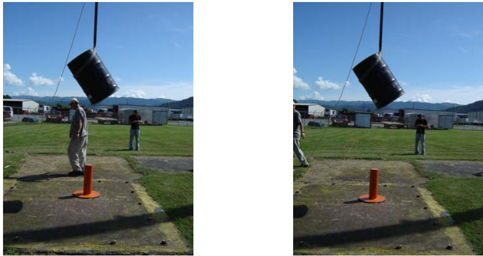
Center of Gravity – Puncture Drop Positioned over the Puncture Ram
