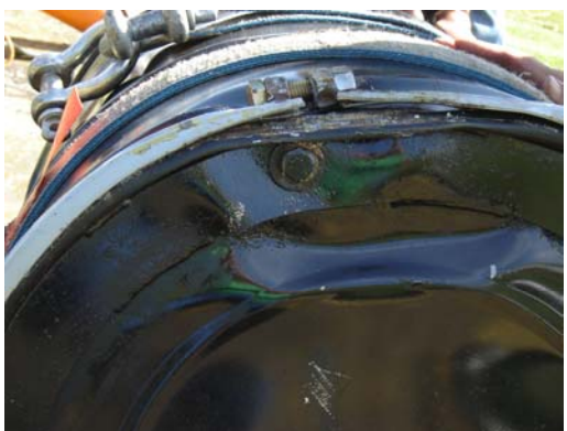
Close-up of Closure End Damage
