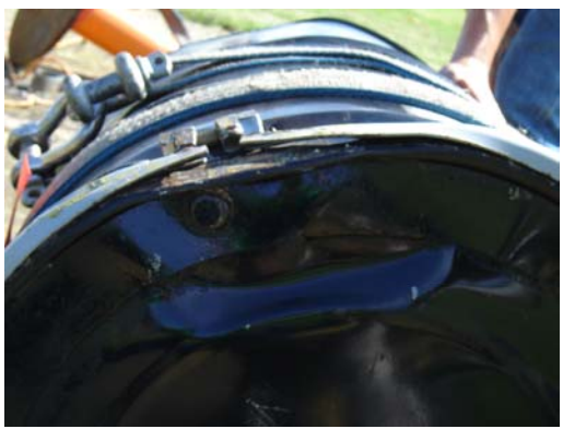
Impact Damage to Closure End
