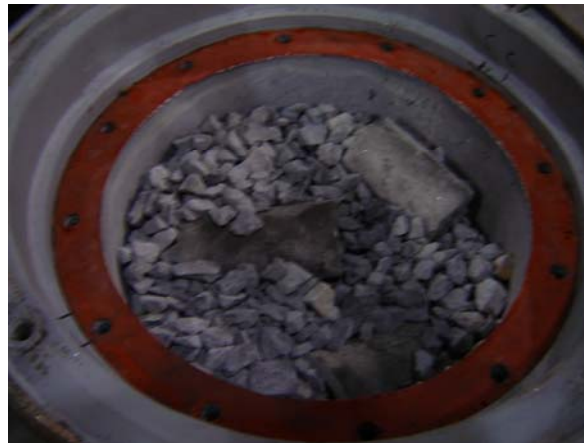
Containment Loaded With 254-1/2 Pounds of Loose Gravel
