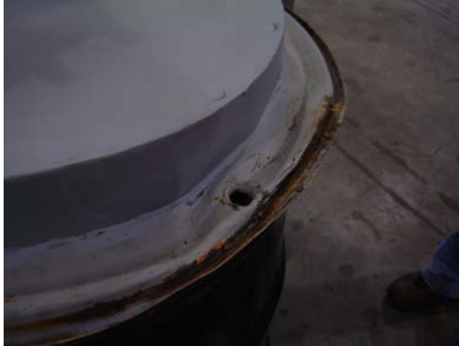
View of Damage to Top Closure
