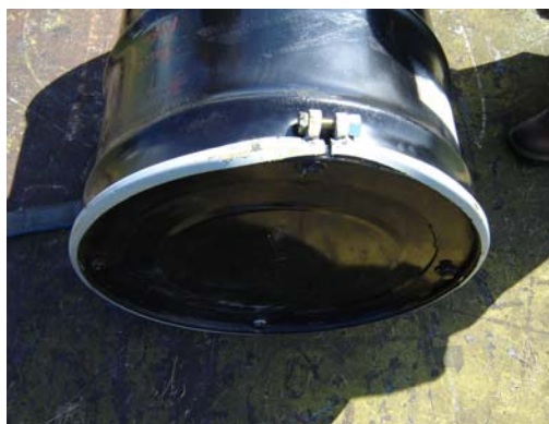
Post Drop Damage to Bolt End Impact Area
