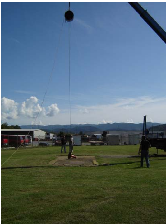
Shallow Angle Accelerated 30' HAC Drop Position
