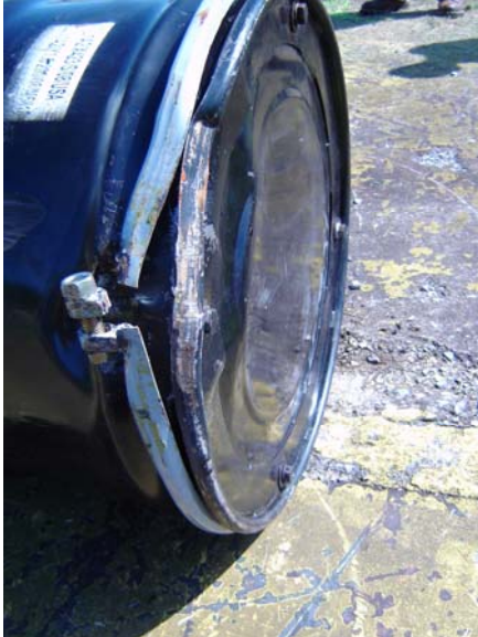
Puncture Impact Damage – No Opening
