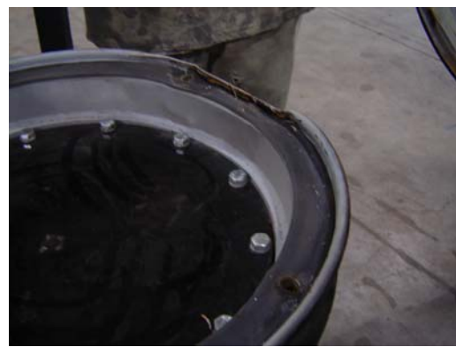
Top End Impact Area Damage
