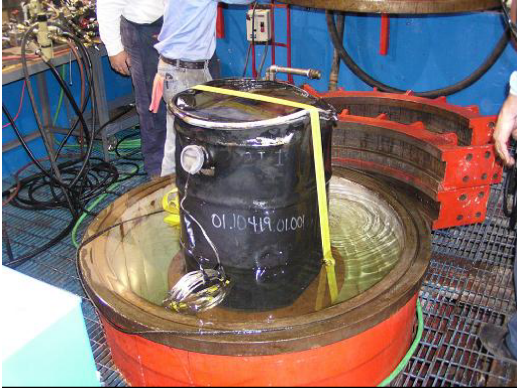
Figure 2.5.3-1 Champion Package on Test Stand – View from Thermocouple Shielding Tube
