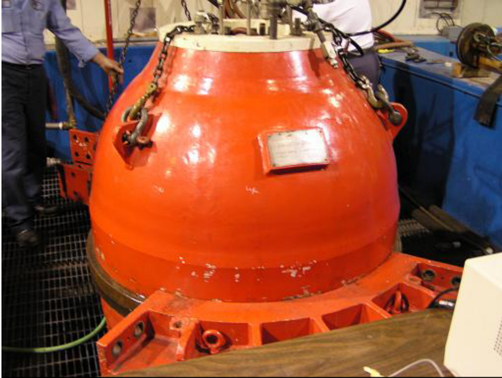
Figure 2.5.3-3 Champion Package during Immersion Test
