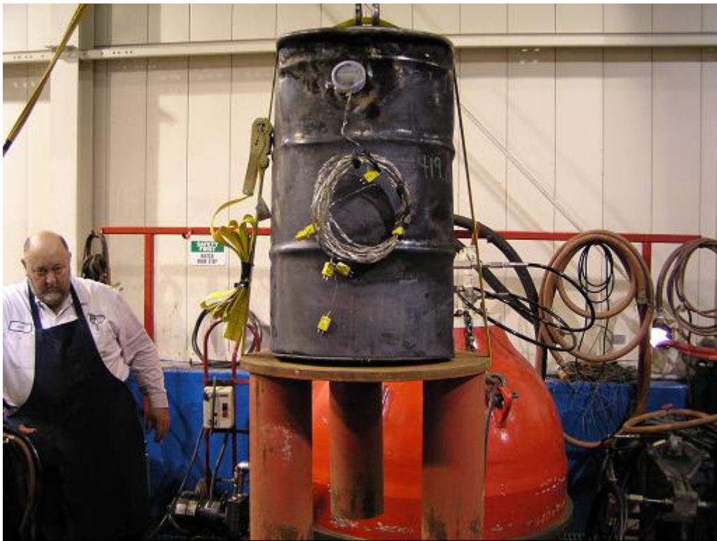
Figure 2.5.3-2 Champion Package during Immersion Testing Phase
