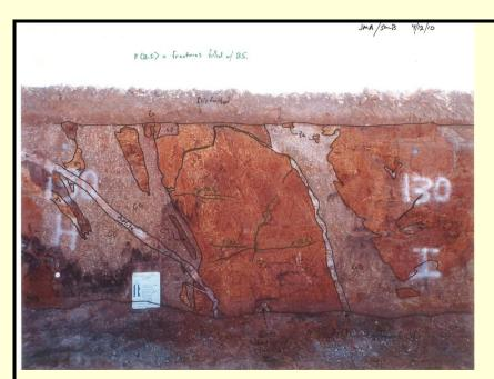
Away from NW top of excavation is deeper into the weathering and structures are preserved in the saprolite
