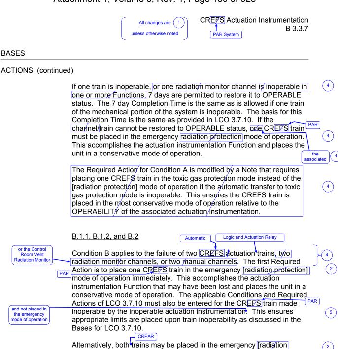
Alternatively, both trains may be placed in the emergency [radiation] protection] mode. This ensures the CREFS function is performed even in the presence of a single failure.
