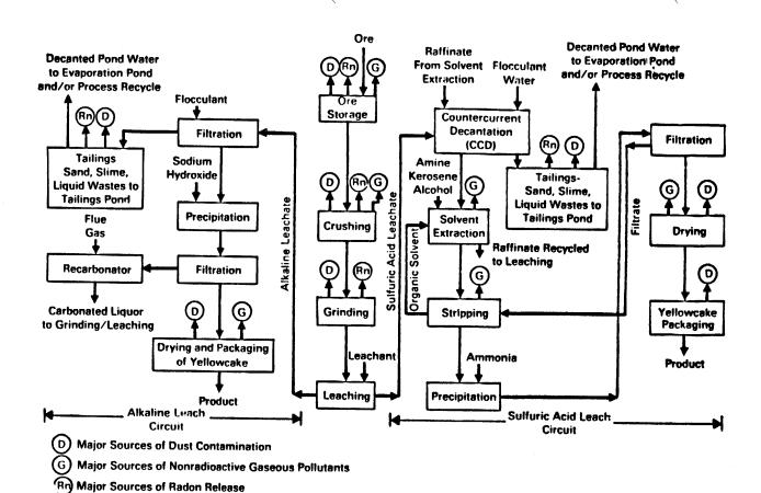
Figure 2. Block Flow Diagram for Uranium Milling Processes
