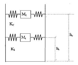
Figure 2: Mechanical models for flexible circular tanks (Malhotra et. al., 2000)
