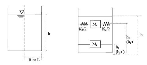
Figure 1: Description of tank dimensions and mechanical model
