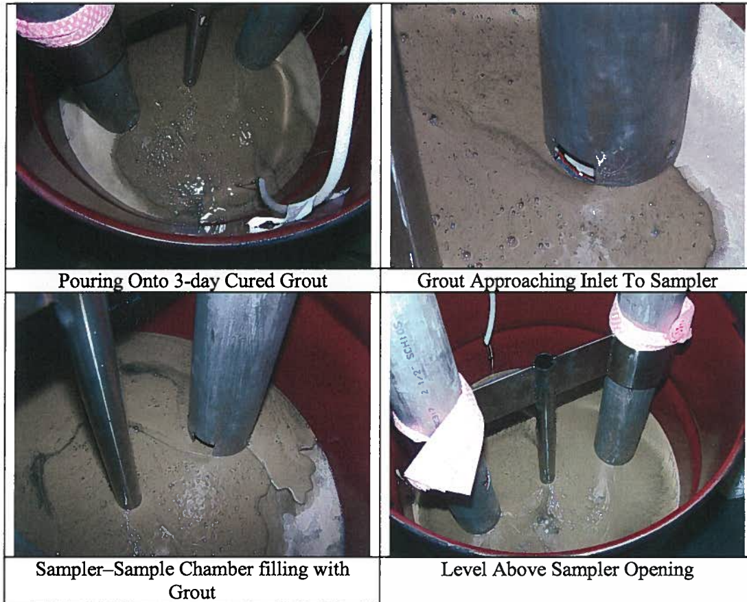
Figure 2, Grout Flow During 1 st Test – 1.5 Inches Per Hour Fill Rate.
