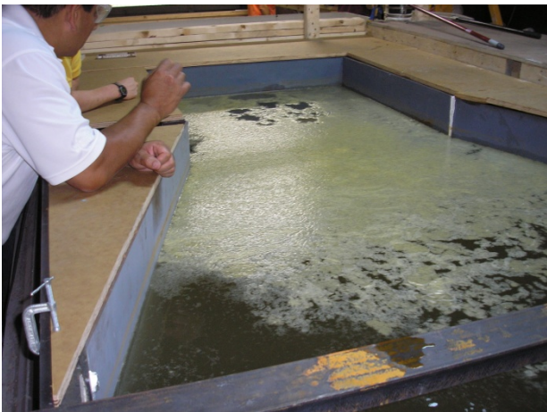
Photo 5-Fiber on Surface of Tank
