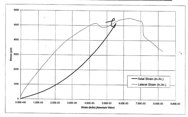
Strain values shown are in terms of absolute value: Axial Strain is negative, Comments: Lateral Strain is positive.
