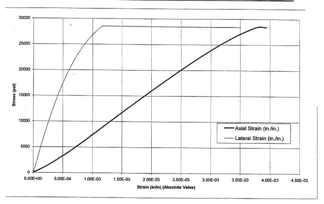
Comments: Young's Modulus and Poisson's Ratio determined using linear fit of curve from approximately 40% to 60% of unconfined compressive strength. Strain values shown are in terms of absolute value: Axial Strain is negative, Lateral Strain is positive.
