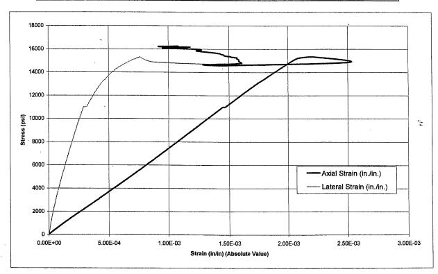
Young's Modulus and Poisson's Ratio determined using linear fit of curve from approximately 40% to 60% of unconfined compressive strength.
