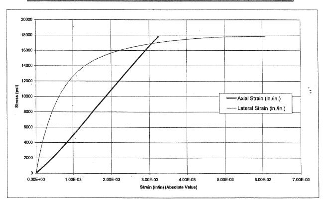
Comments: Young's Modulus and Poisson's Ratio determined using linear fit of curve from approximately 40% to 60% of unconfined compressive strength.
