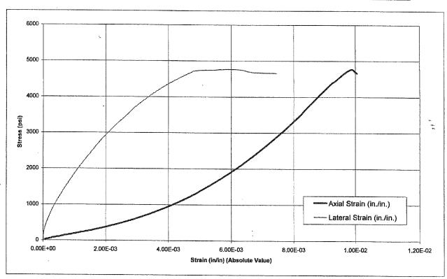
Comments: Strain values shown are in terms of absolute value: Axial Strain is negative, Lateral Strain is positive. \* = Value of Poisson's ratio is greater than 0.5 which indicates inelastic behavior probably due to presence of fractures or discontinuities affecting lateral strain.
