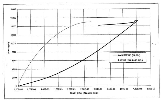
Strain values shown are in terms of absolute value: Axial Strain is negative, Lateral Strain is positive. \* = Value of Poisson's ratio is greater than 0.5 which indicates inelastic behavior probably due to presence of fractures or discontinuities affecting lateral strain.
