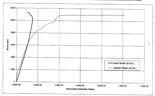
Comments: Young's Modulus and Poisson's Ratio determined using linear fit of curve from approximately 40% to 60% of unconfined compressive strength.
