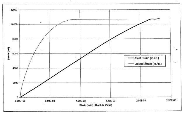
Young's Modulus and Poisson's Ratio determined using linear fit of curve from approximately 40% to 60% of unconfined compressive strength. Strain values shown are in terms of absolute value: Axial Strain is negative, Lateral Strain is positive.
