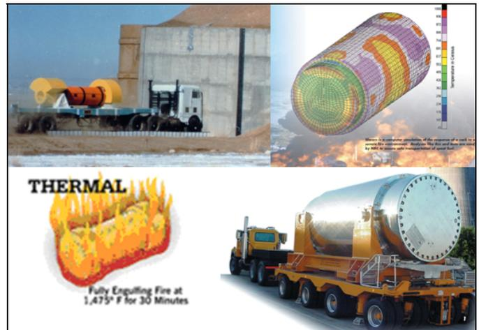
**Figure 1. Pictures of Shipping Casks [Pictures from NUREG/BR-0292 and [www.ne.doe.gov](http://www.ne.doe.gov)]:** Pictures of Truck Shipping Casks (top left and bottom right), picture of a computer simulation response of a cask to a fire environment (top right), and diagram of a cask in a fully engulfing fire (bottom left)
