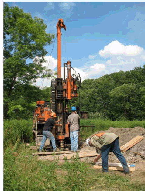
Photograph 10. Deep Testing in Area 6, Section 1, Showing Drill Rig Excavating a Soil Coring in Base of Trench, Facing North
