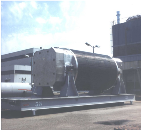
Used fuel TN12/2, TN13/2, TN112, TN17/2
