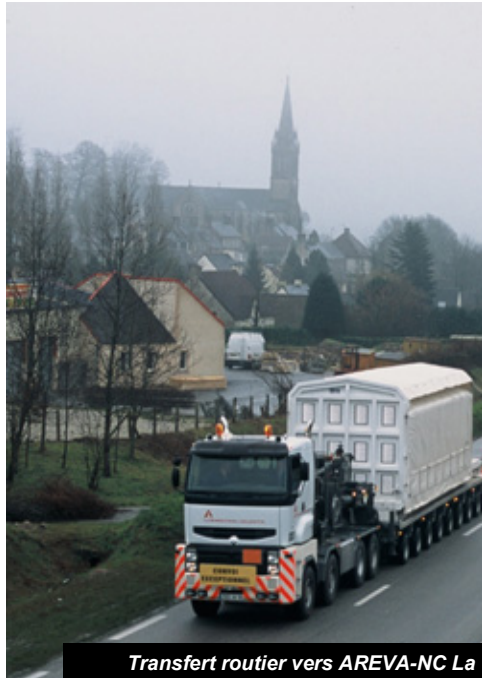
Tractor & trailer for used fuel and HLW packages
