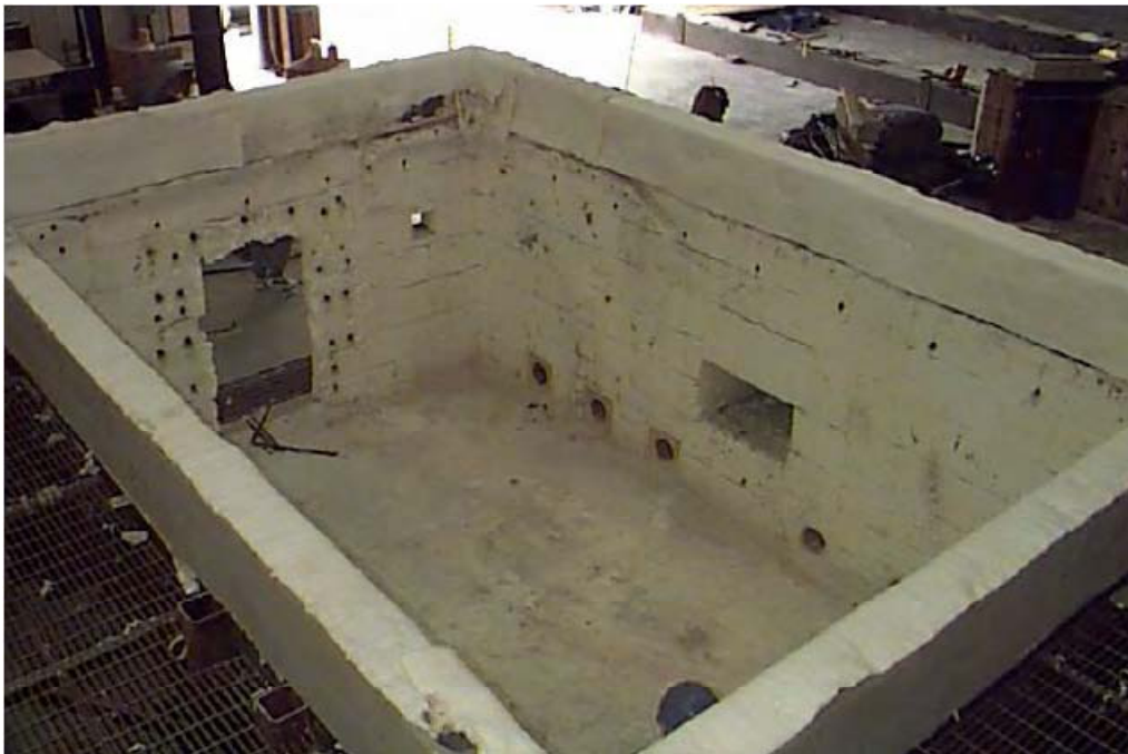
Figure G-9. 12' x 18' Horizontal Furnace (Top View) (NRC Hemyc Tests)
