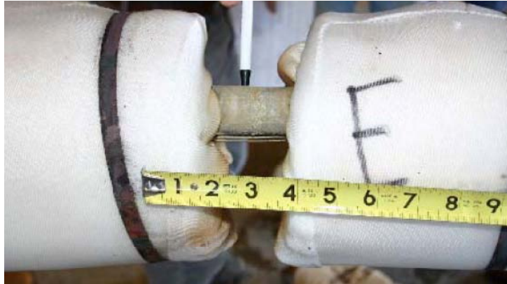
Figure 5-12. Post-test Photo of Hemyc ERFBS Showing Shrinkage at Junction (NRC Hemyc testing, 2005)
