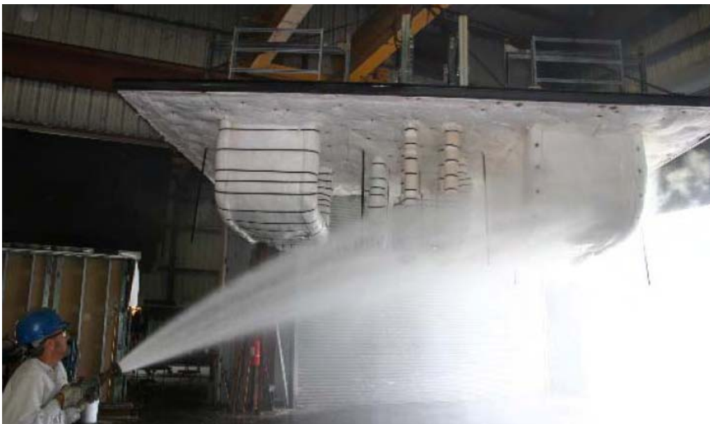
Figure G-6. Post-Fire Exposure – Hose Stream Test (NRC Hemyc Tests 2005)
