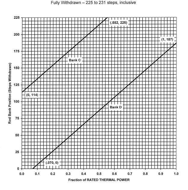
Fully Withdrawn shall be the condition where control rods are at a position within the interval  $\geq$  225 and  $\leq$  231 steps withdrawn.
