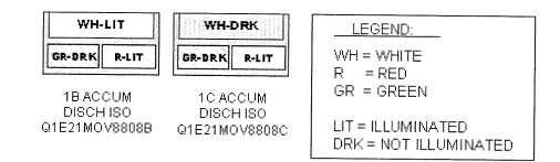
Neither of the valves are responding to MCB switch manipulation.
