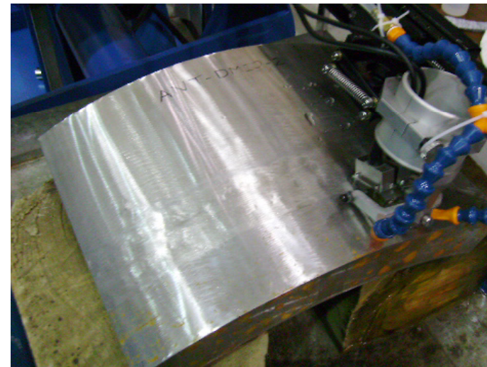
Automated UT scanning
