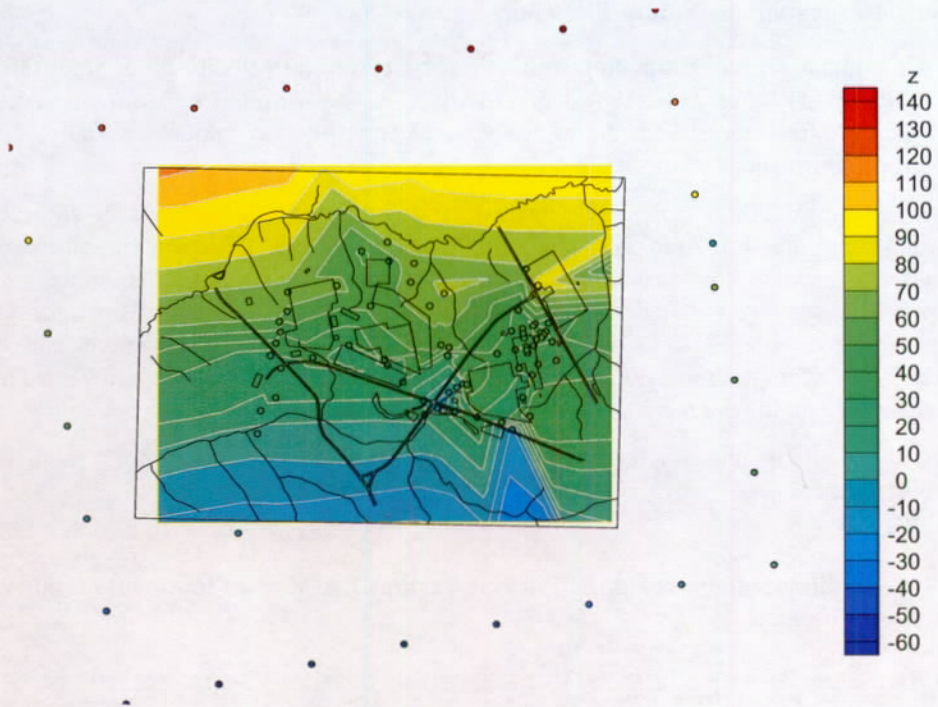
Figure 4-1. GSA/PORFLOW representation of the top of the Meyers Branch confining system (Crouch Branch confining unit).
