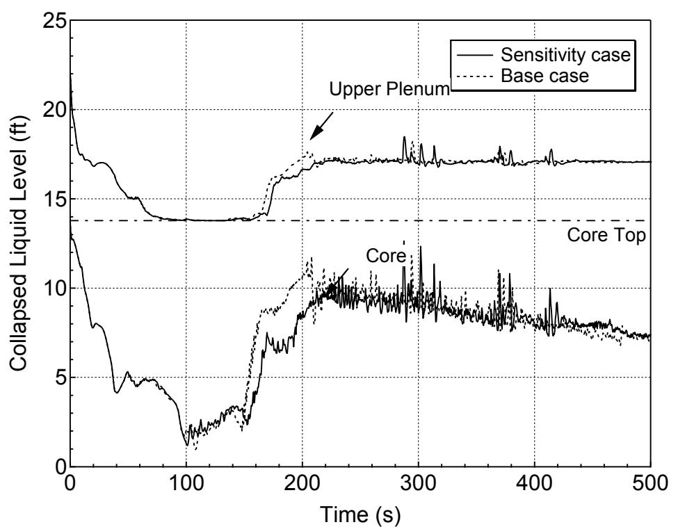
**Figure 5.4.3-22 Average Core and Upper Plenum Collapsed Levels for 1-ft<sup>2</sup> Break (Top)
