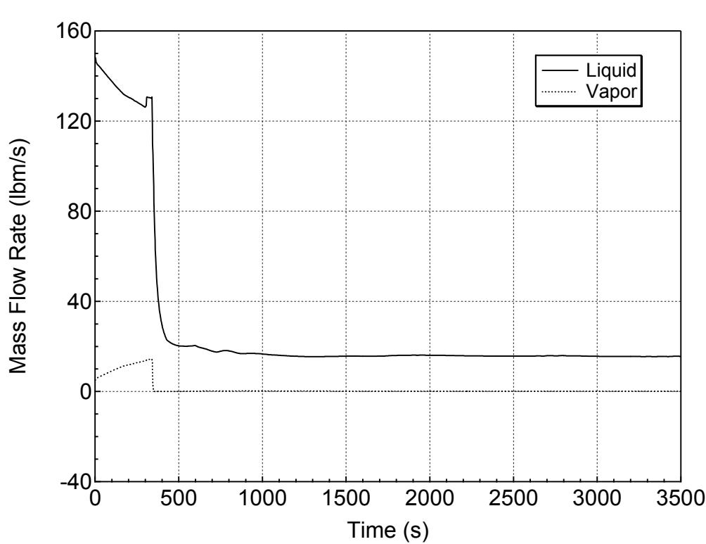
**Figure 5.2.a-9 Hot Assembly Exit Vapor and Liquid Mass Flowrates
