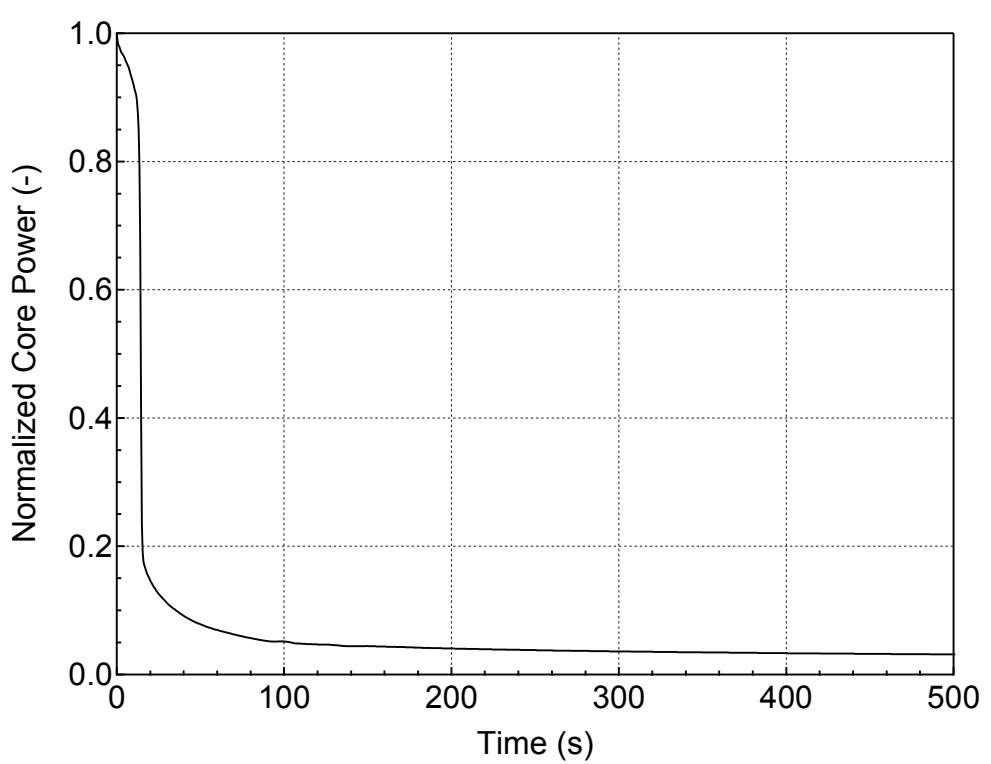
**Figure 5.3.1.c-20 Normalized Core Power for 7-inch Break (Homogeneous)
