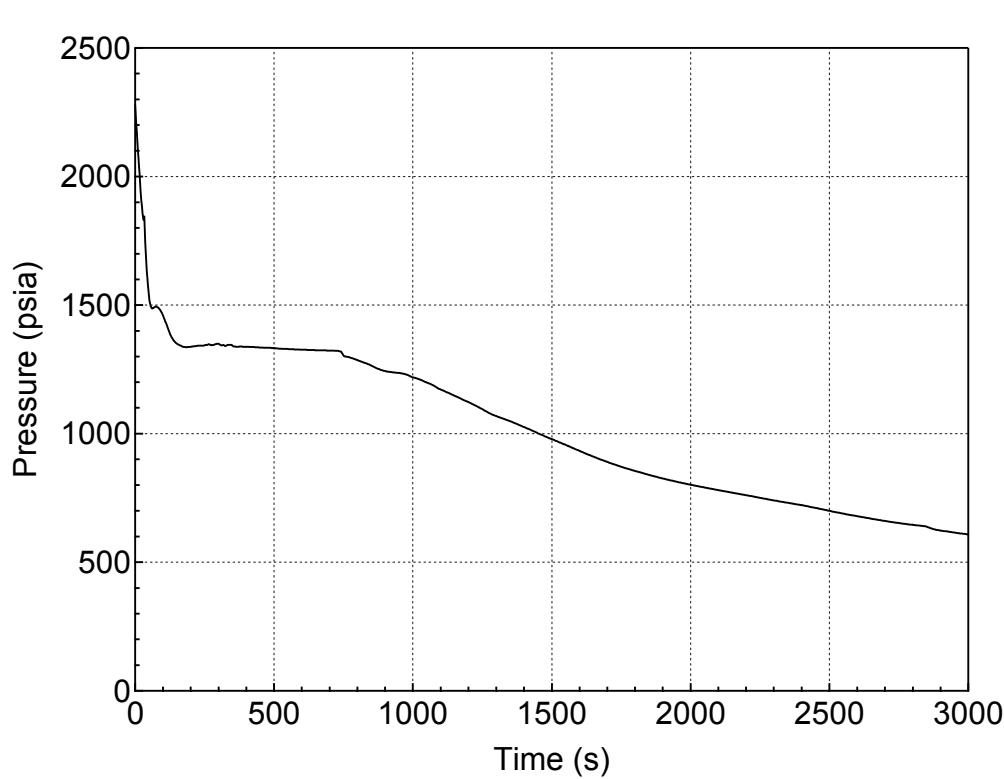
**Figure 5.1.2-1 RCS (Pressurizer) Pressure Transient for DVI-line Break
