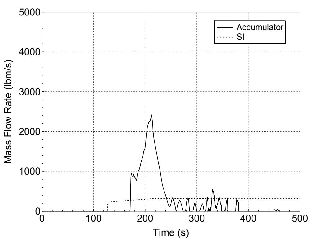
**Figure 5.2.j-4 Accumulator and Safety Injection Mass Flowrates
