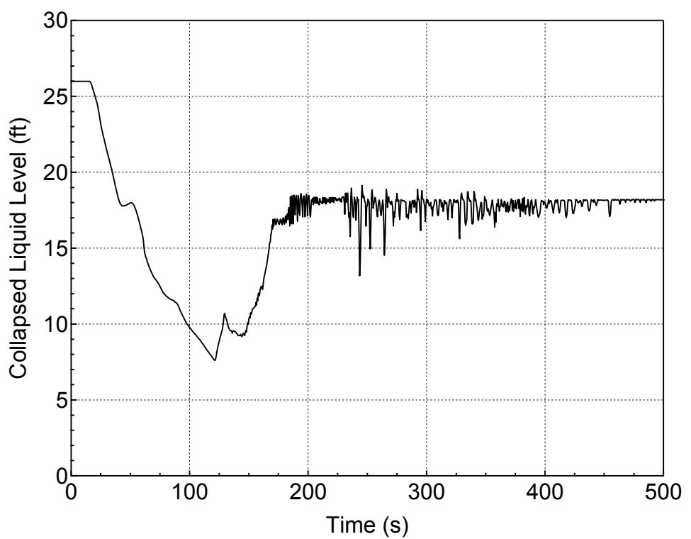
**Figure 5.3.2.a-24 Downcomer Collapsed Level for 12-inch Break (Homogeneous)
