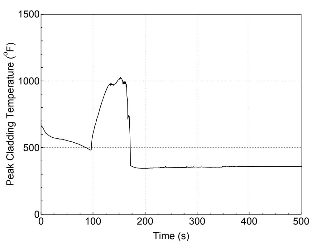
**Figure 5.1.1.a-17 PCT at All Elevations for Hot Rod in Hot Assembly
