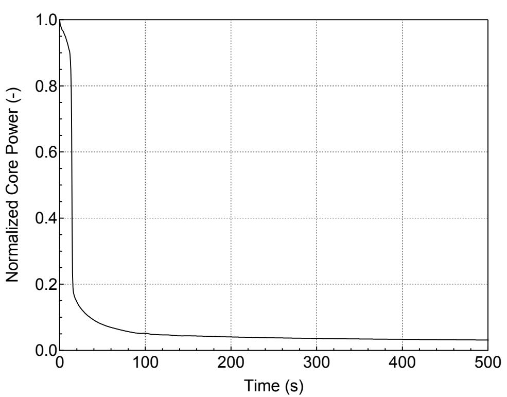
**Figure 5.3.1.c-2 Normalized Core Power for 7-inch Break (Top)
