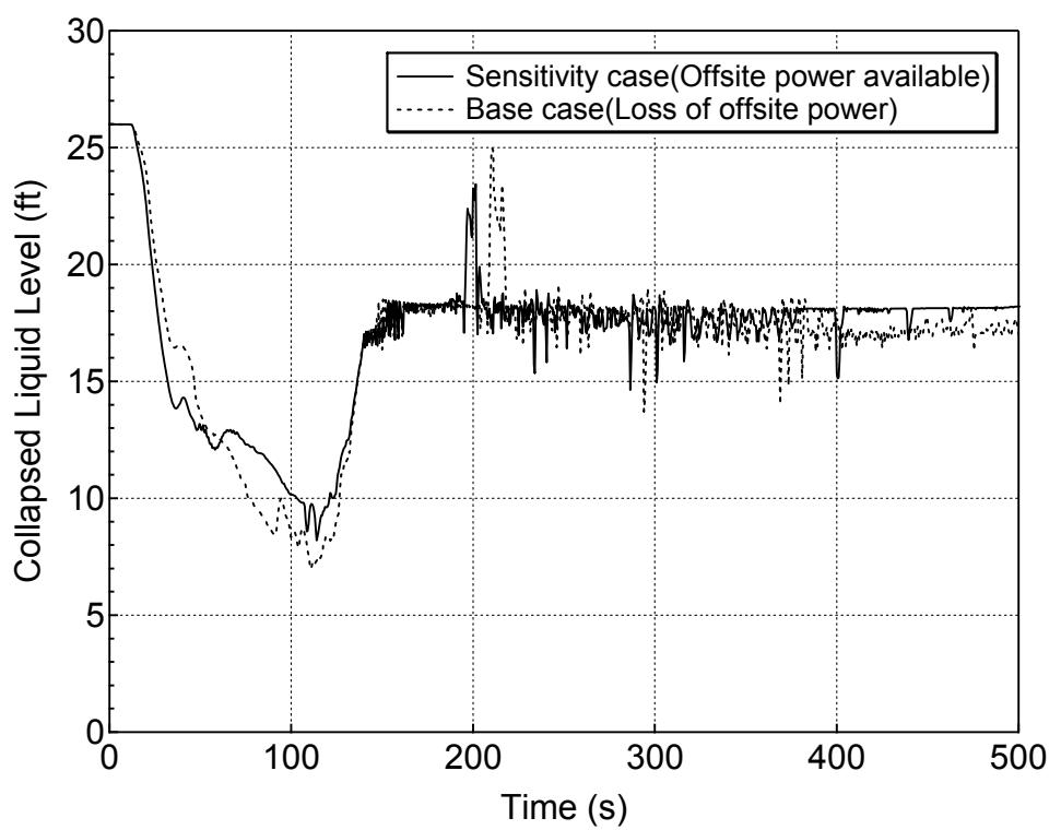
**Figure 5.6.2-21 Downcomer Collapsed Level for 1-ft<sup>2</sup> Break (Top)
