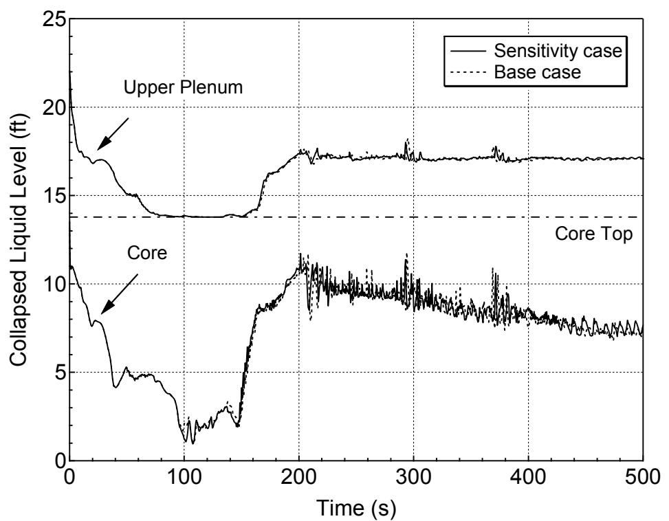
**Figure 5.5.b-10 Hot Assembly Core and Upper Plenum Collapsed Levels
