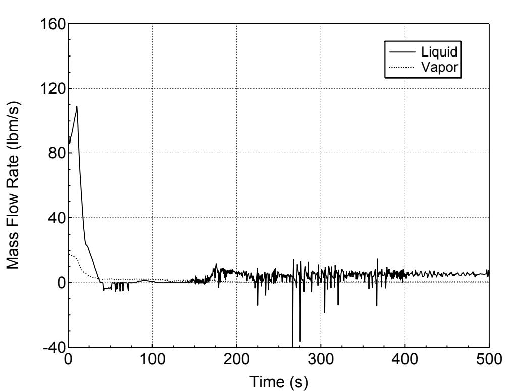
**Figure 5.3.2.b-18 Hot Assembly Exit Vapor and Liquid Mass Flowrates for 13-inch Break (Side) (Break Orientation Sensitivity Study)**
