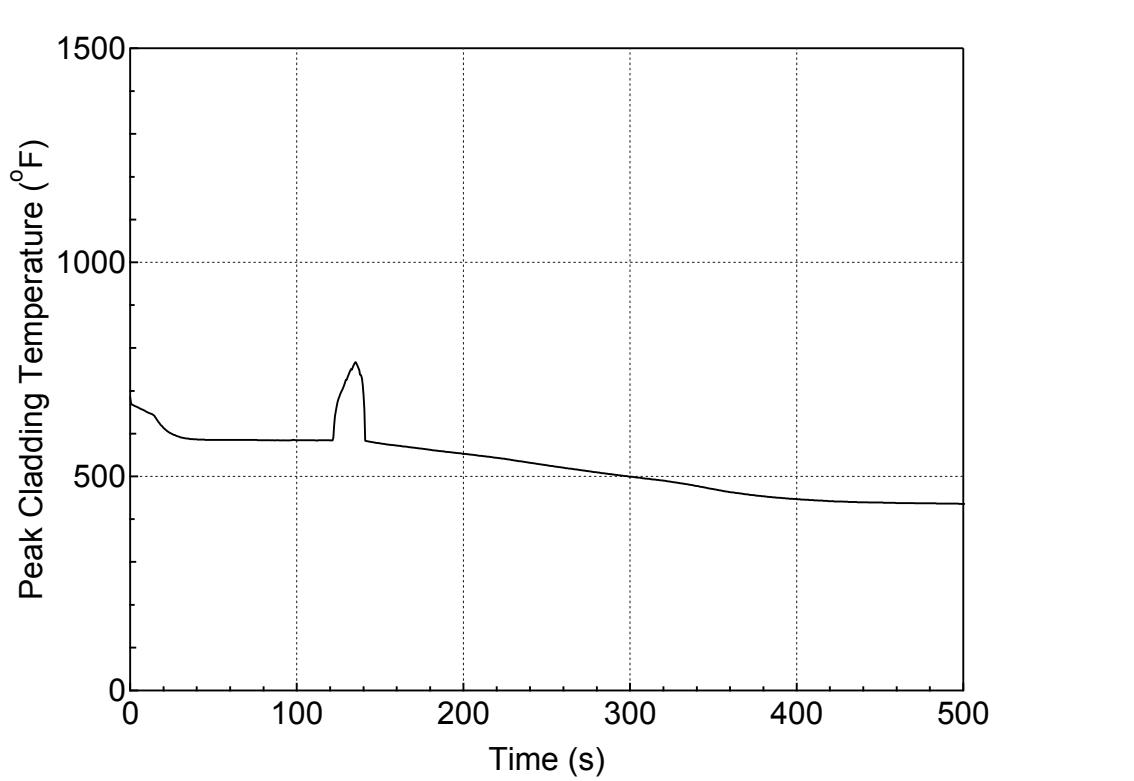
**Figure 5.3.1.d-26 PCT at All Elevations for Hot Rod in Hot Assembly
