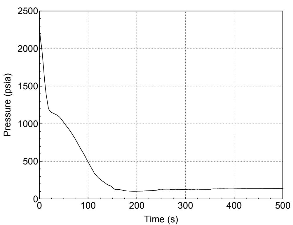
**Figure 5.3.2.c-19 RCS (Pressurizer) Pressure Transient for 1-ft<sup>2</sup> Break (Homogeneous)
