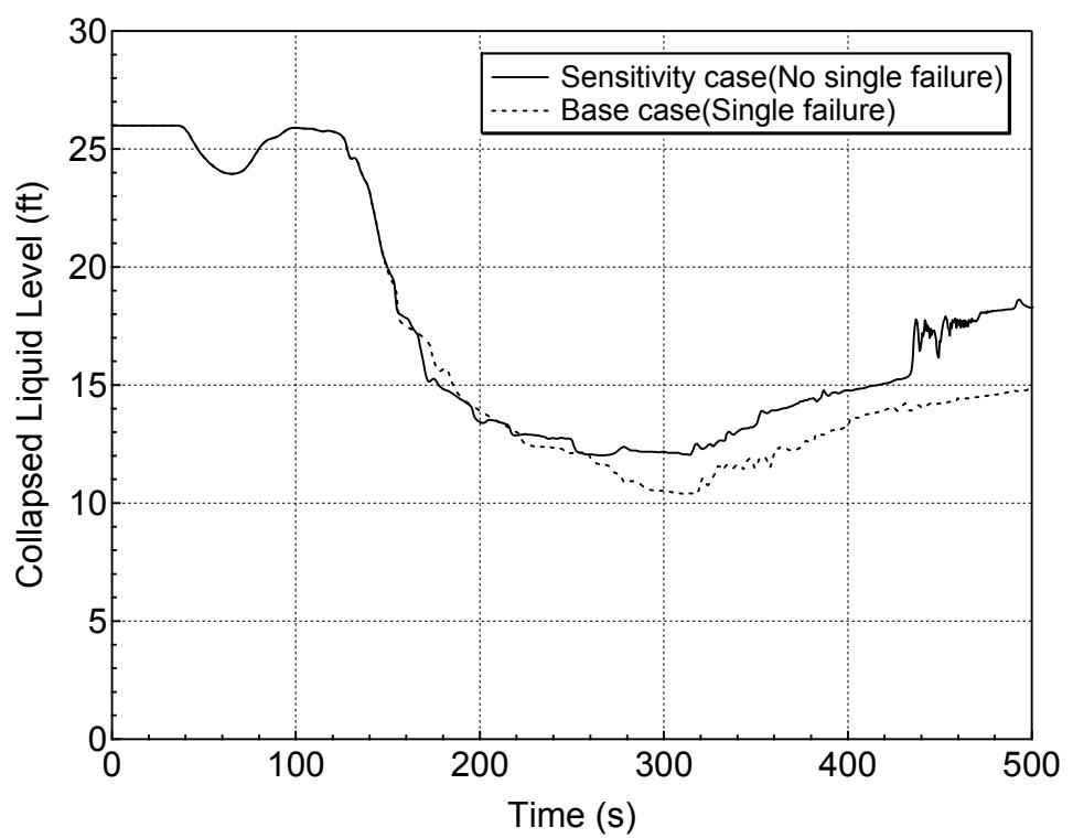
**Figure 5.6.1-8 Downcomer Collapsed Level for 7.5-inch Break (Top)
