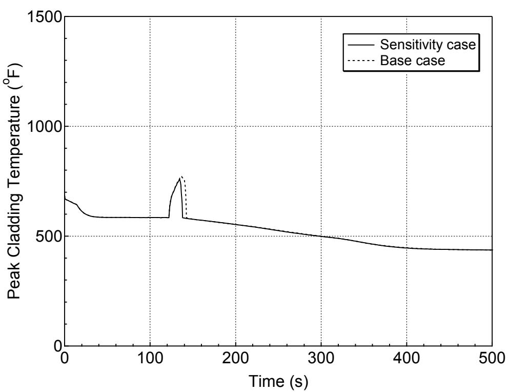
**Figure 5.4.3-11 PCT at All Elevations for Hot Rod in Hot Assembly
