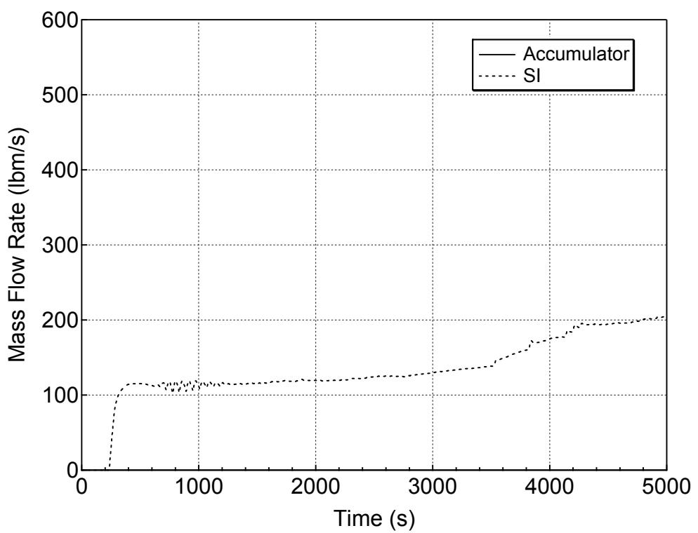
**Figure 5.2.b-4 Accumulator and Safety Injection Mass Flowrates
