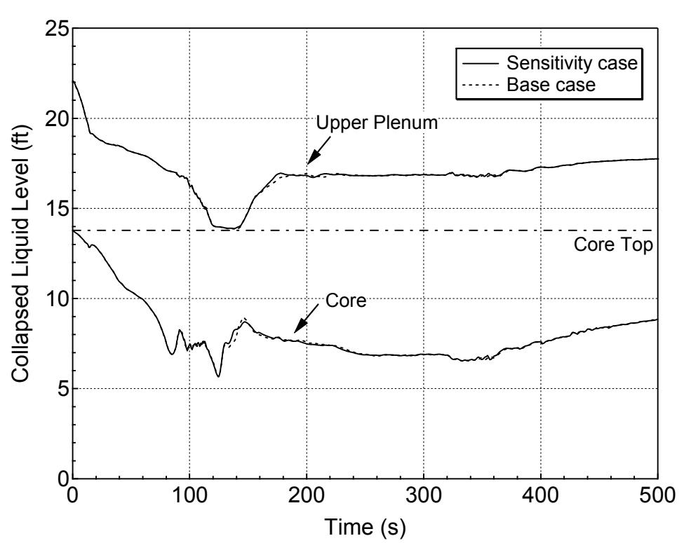
**Figure 5.4.1-9 Average Core and Upper Plenum Collapsed Levels for 7.5-inch Break (Top)
