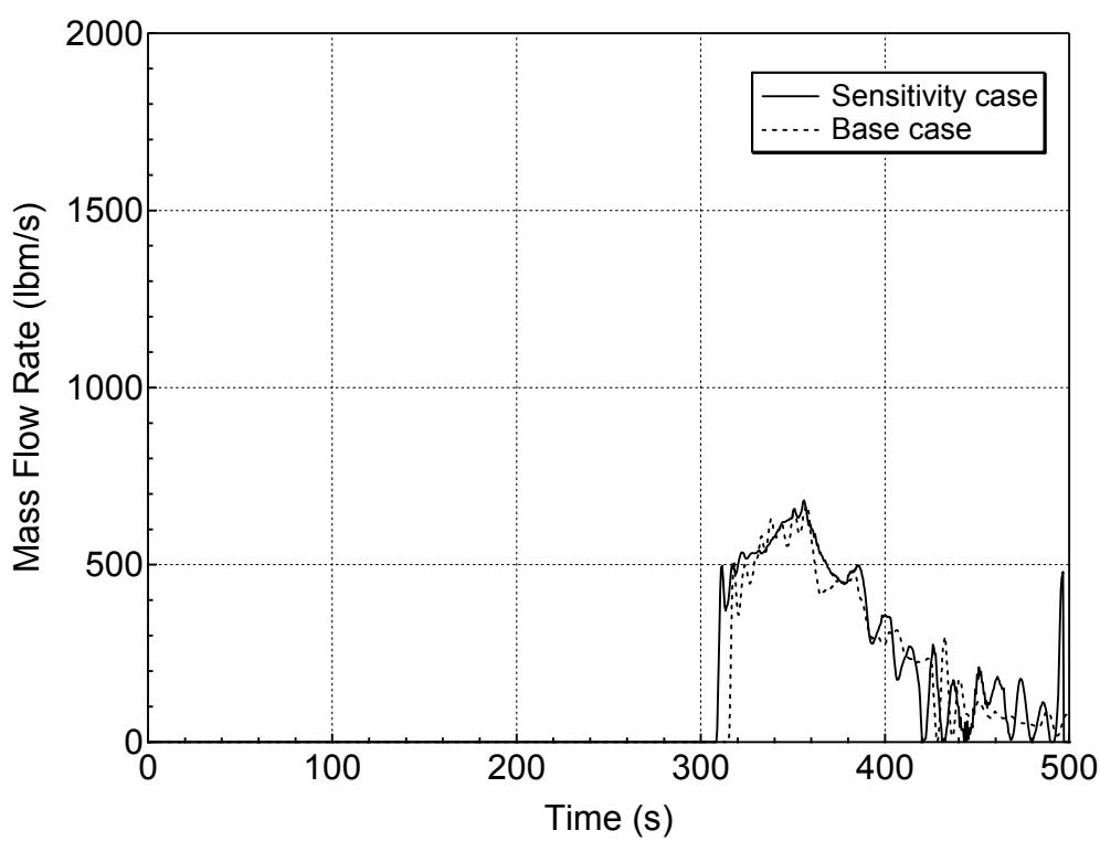
**Figure 5.4.2-5 Accumulator Injection Mass Flowrate for 7.5-inch Break (Top)
