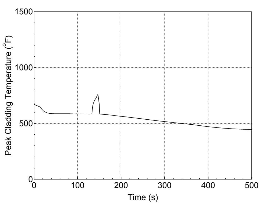
**Figure 5.2.g-8 PCT at All Elevations for Hot Rod in Hot Assembly
