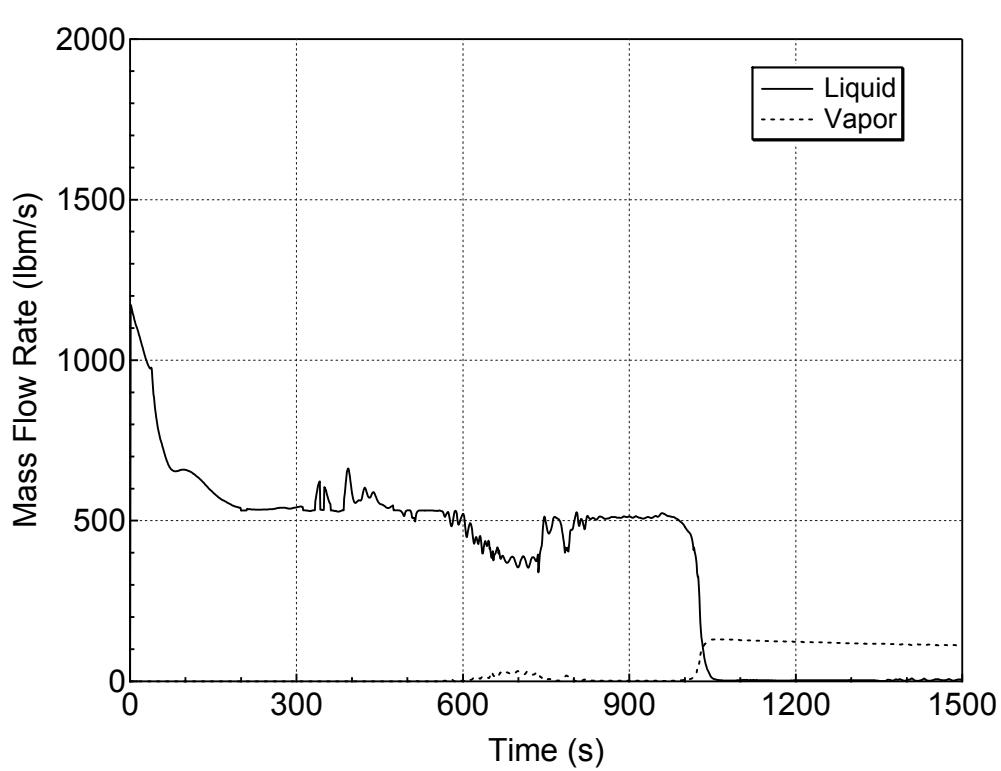
**Figure 5.2.c-3 Liquid and Vapor Discharges through the Break
