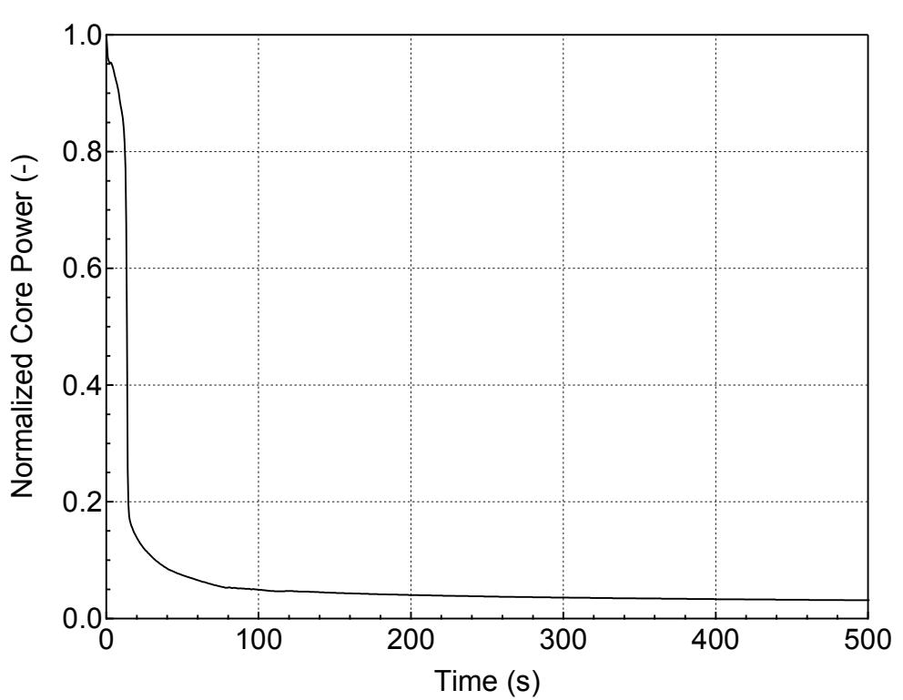
**Figure 5.3.1.e-20 Normalized Core Power for 8-inch Break (Homogeneous)
