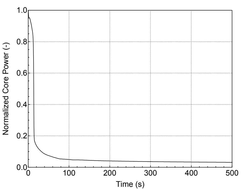
**Figure 5.2.h-2 Normalized Core Power for 8-inch Break (Bottom)
