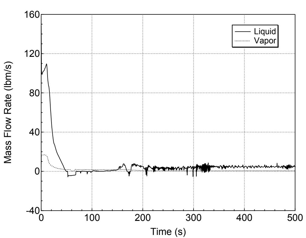
**Figure 5.2.k-9 Hot Assembly Exit Vapor and Liquid Mass Flowrates
