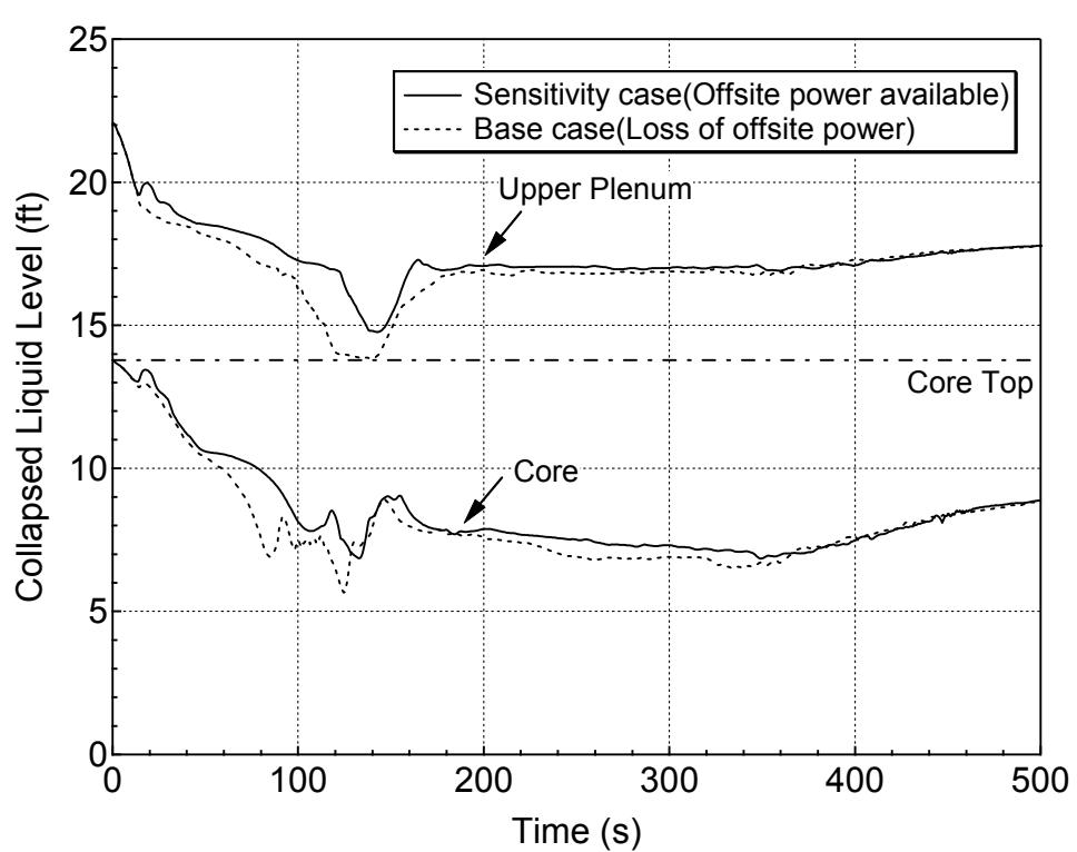
**Figure 5.6.2-9 Average Core and Upper Plenum Collapsed Levels
