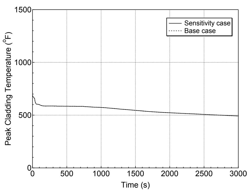
**Figure 5.5.c-11 PCT at All Elevations for Hot Rod in Hot Assembly for DVI-line Break
