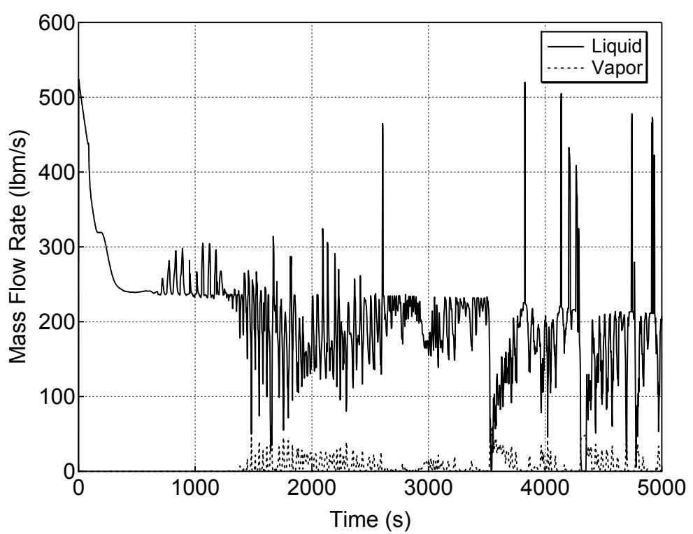
**Figure 5.1.1.a-3 Liquid and Vapor Discharges through the Break
