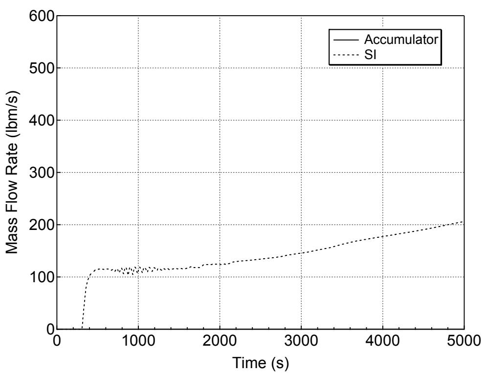
**Figure 5.1.1.b-4 Accumulator and Safety Injection Mass Flowrates
