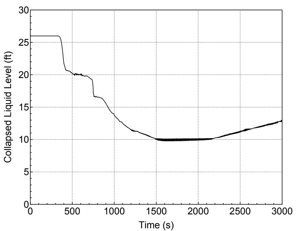
**Figure 5.1.2-6 Downcomer Collapsed Level for DVI-line Break
