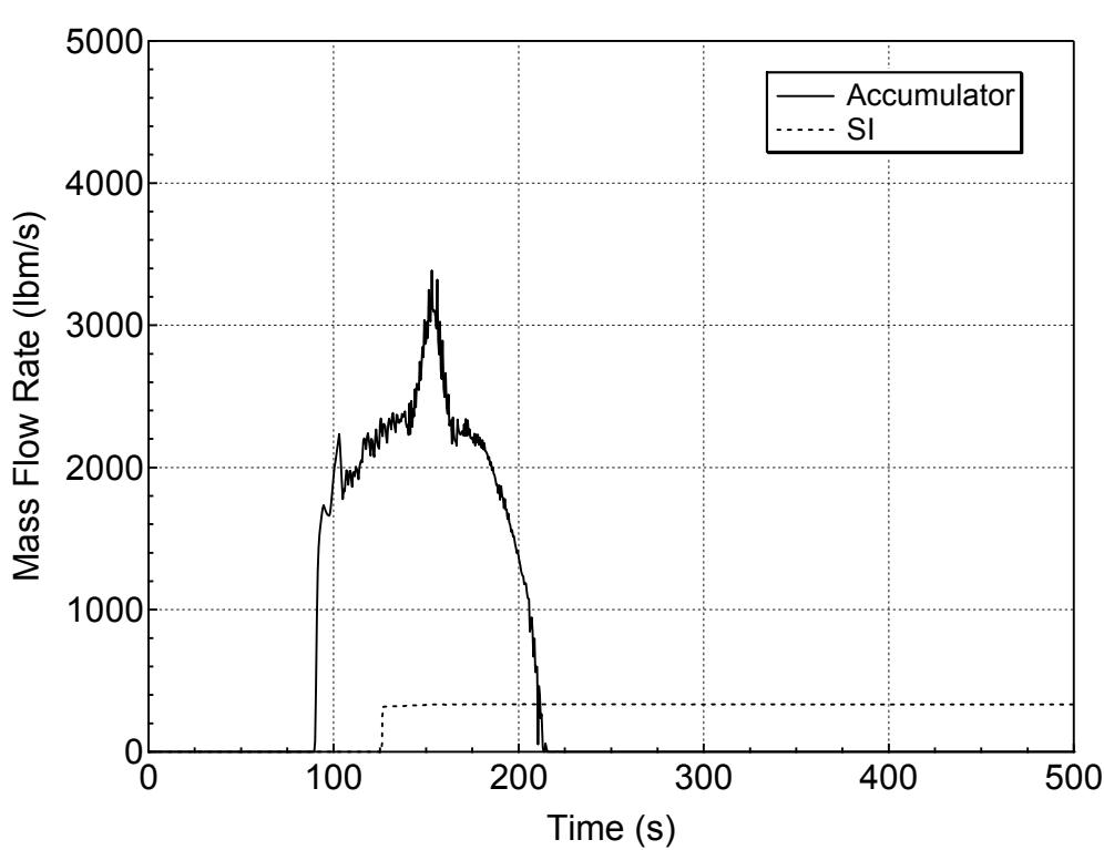
**Figure 5.1.1.a-13 Accumulator and Safety Injection Mass Flowrates
