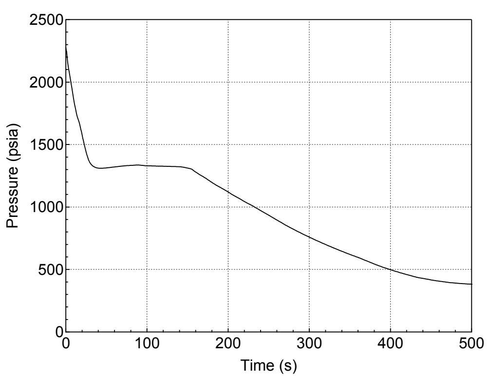
**Figure 5.3.1.c-10 RCS (Pressurizer) Pressure Transient for 7-inch Break (Side)
