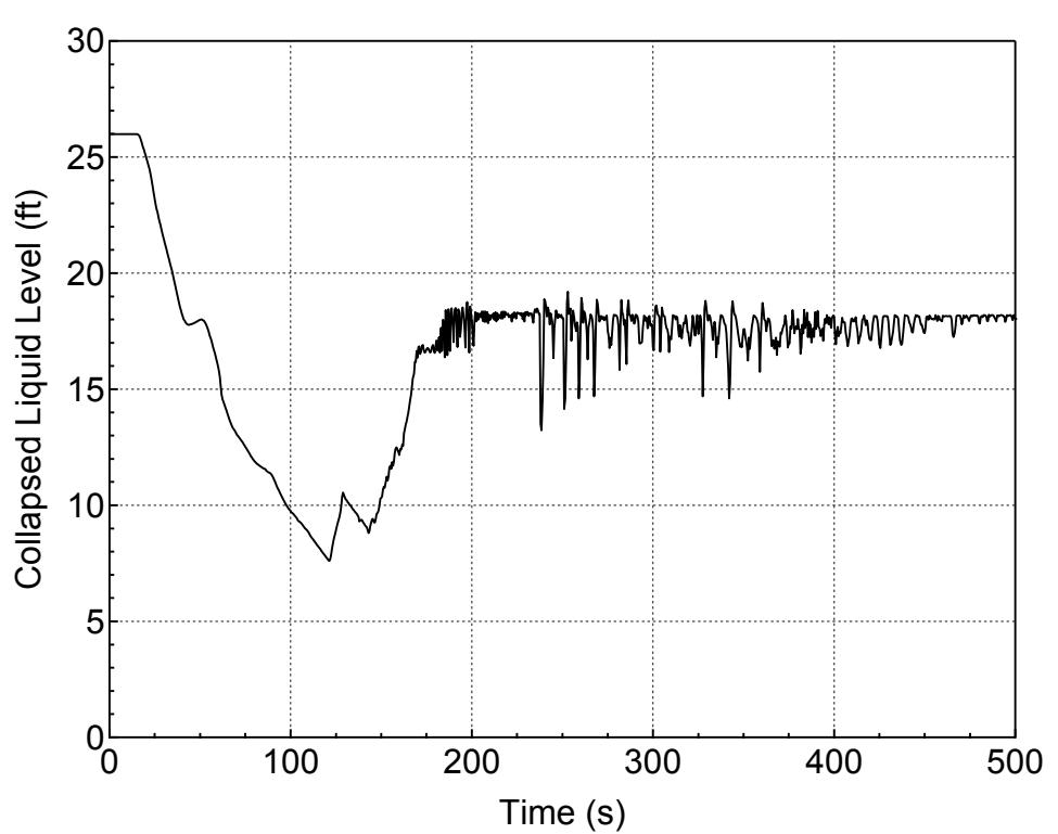
**Figure 5.3.2.a-15 Downcomer Collapsed Level for 12-inch Break (Side)
