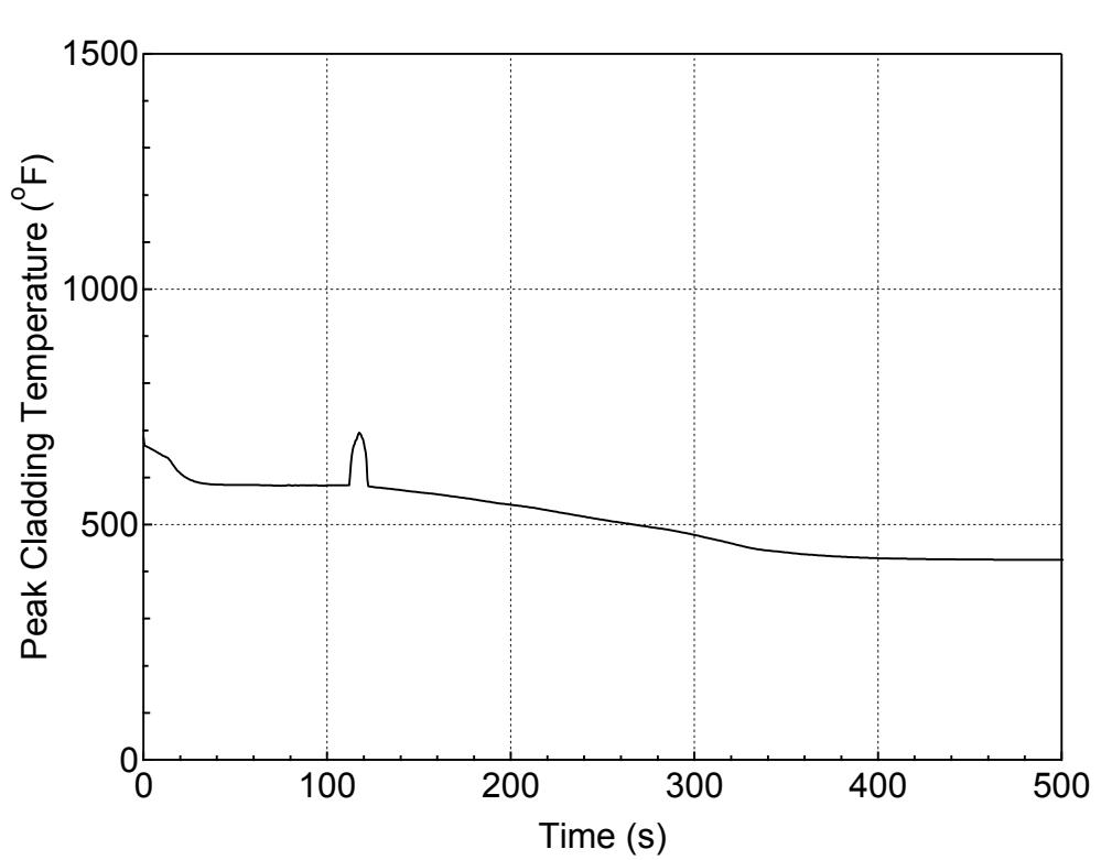
**Figure 5.2.h-8 PCT at All Elevations for Hot Rod in Hot Assembly
