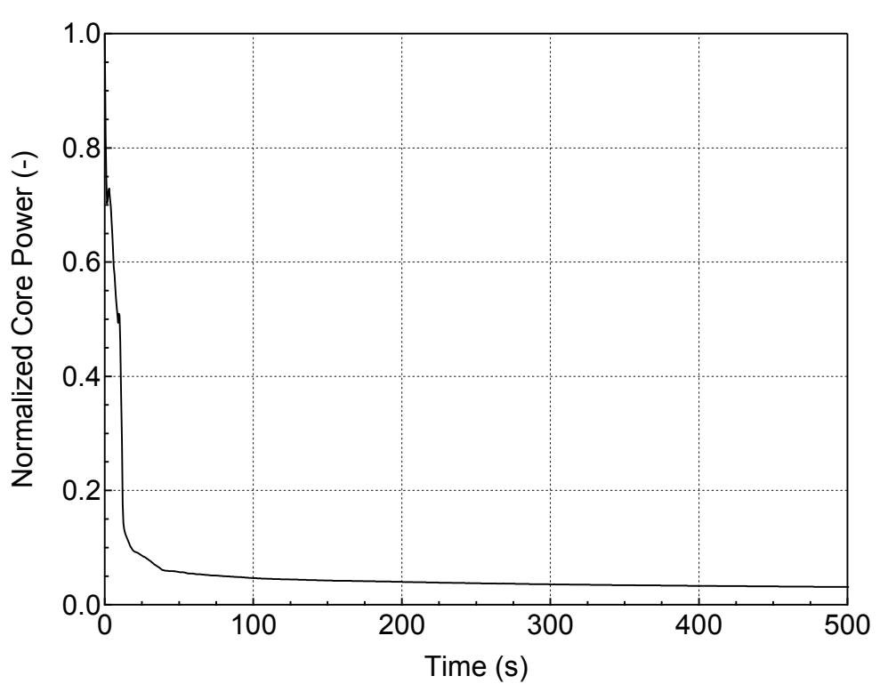
**Figure 5.3.2.c-20 Normalized Core Power for 1-ft<sup>2</sup> Break (Homogeneous)
