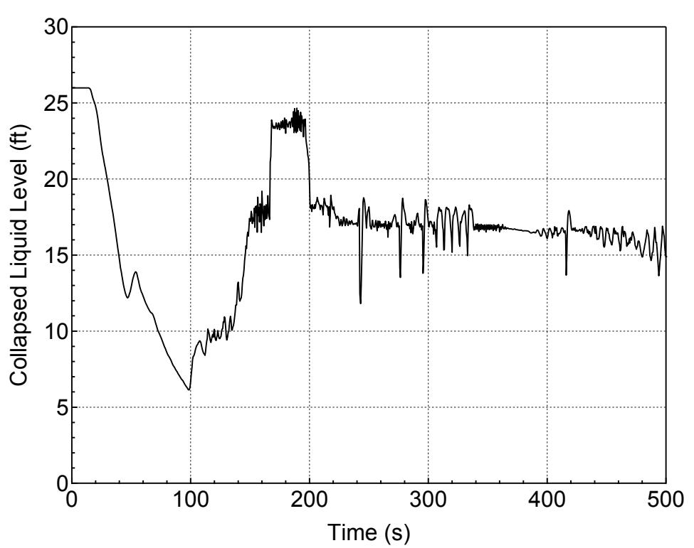
**Figure 5.1.1.c-15 Downcomer Collapsed Level for 1-ft<sup>2</sup> Break (Bottom)
