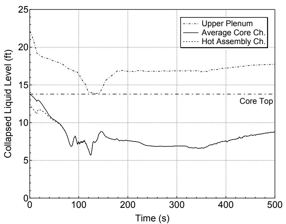
**Figure 5.3.1.d-25 Core and Upper Plenum Collapsed Levels for 7.5-inch Break (Side)
