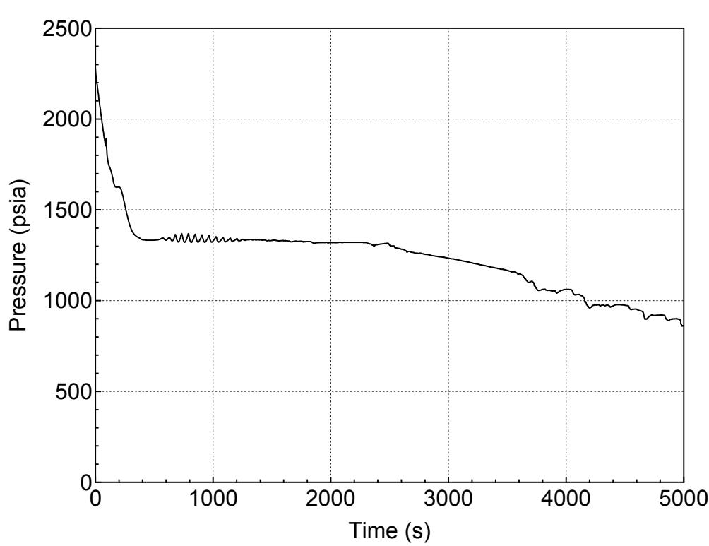
**Figure 5.1.1.c-1 RCS (Pressurizer) Pressure Transient for 2-inch Break (Bottom)
