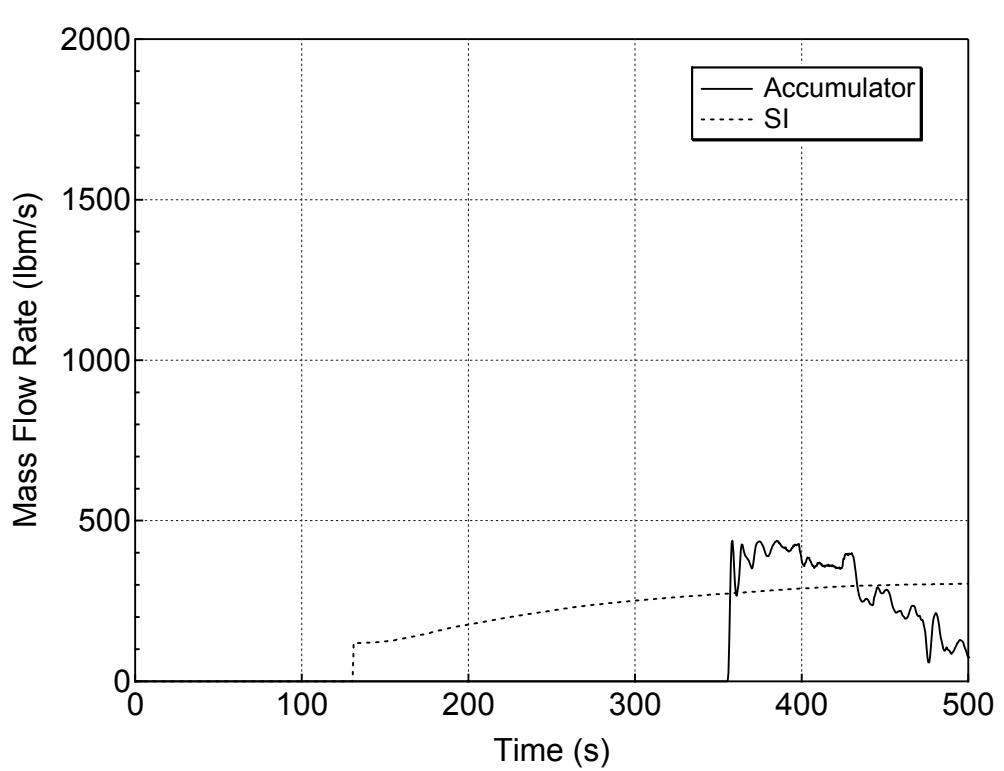
**Figure 5.2.g-4 Accumulator and Safety Injection Mass Flowrates
