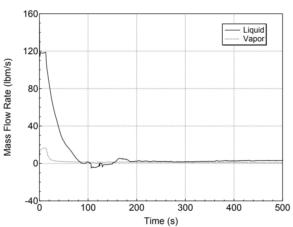
**Figure 5.3.1.c-18 Hot Assembly Exit Vapor and Liquid Mass Flowrates
