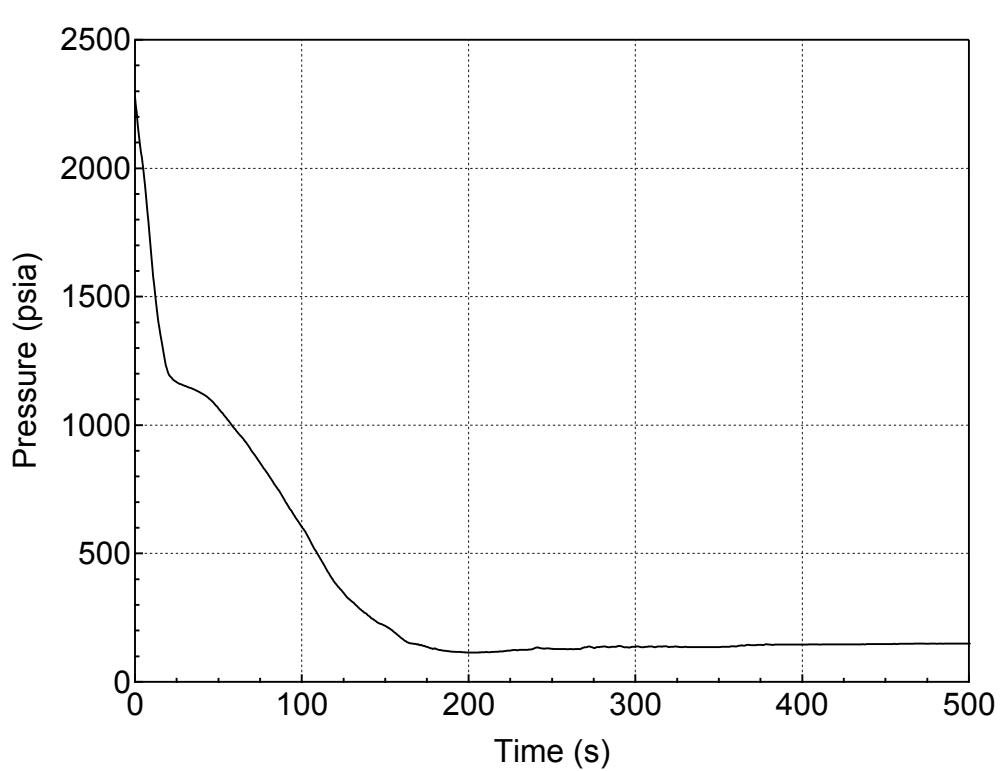
**Figure 5.3.2.b-10 RCS (Pressurizer) Pressure Transient for 13-inch Break (Side)
