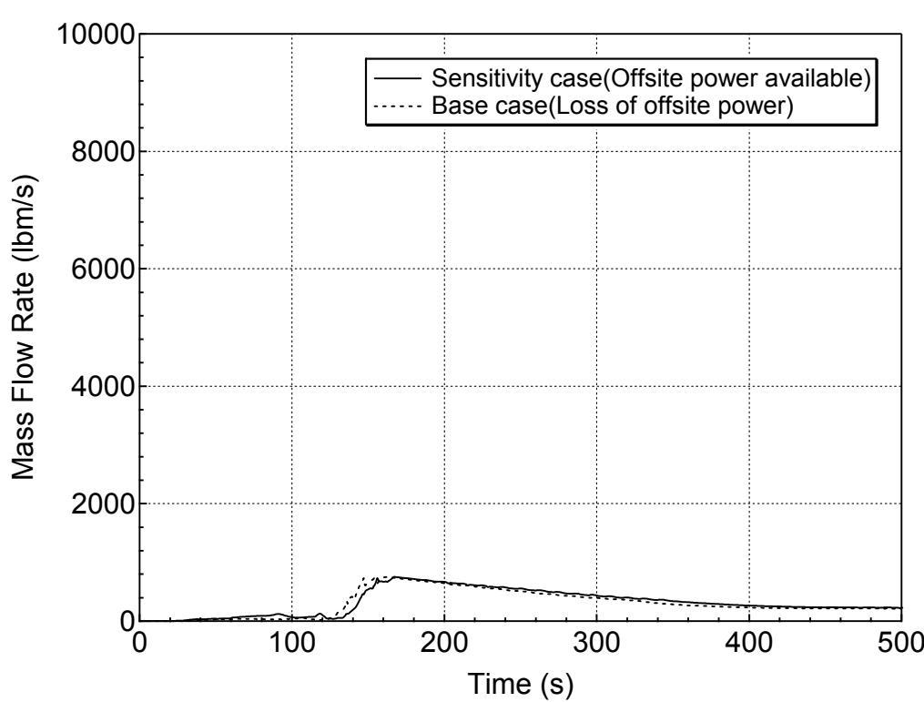
**Figure 5.6.2-4 Vapor Discharge through the Break for 7.5-inch Break (Top)
