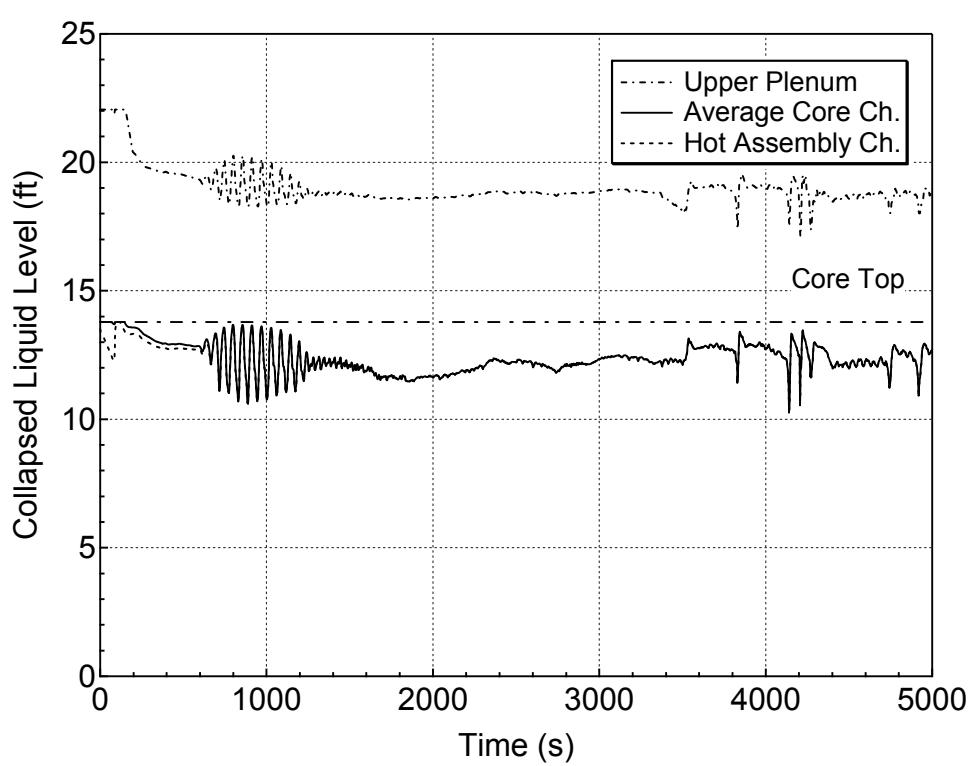
**Figure 5.2.b-7 Core and Upper Plenum Collapsed Levels for 2-inch Break (Bottom) (Spectrum Analysis)**
