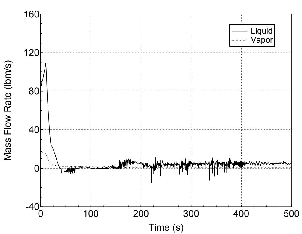
**Figure 5.3.2.b-9 Hot Assembly Exit Vapor and Liquid Mass Flowrates
