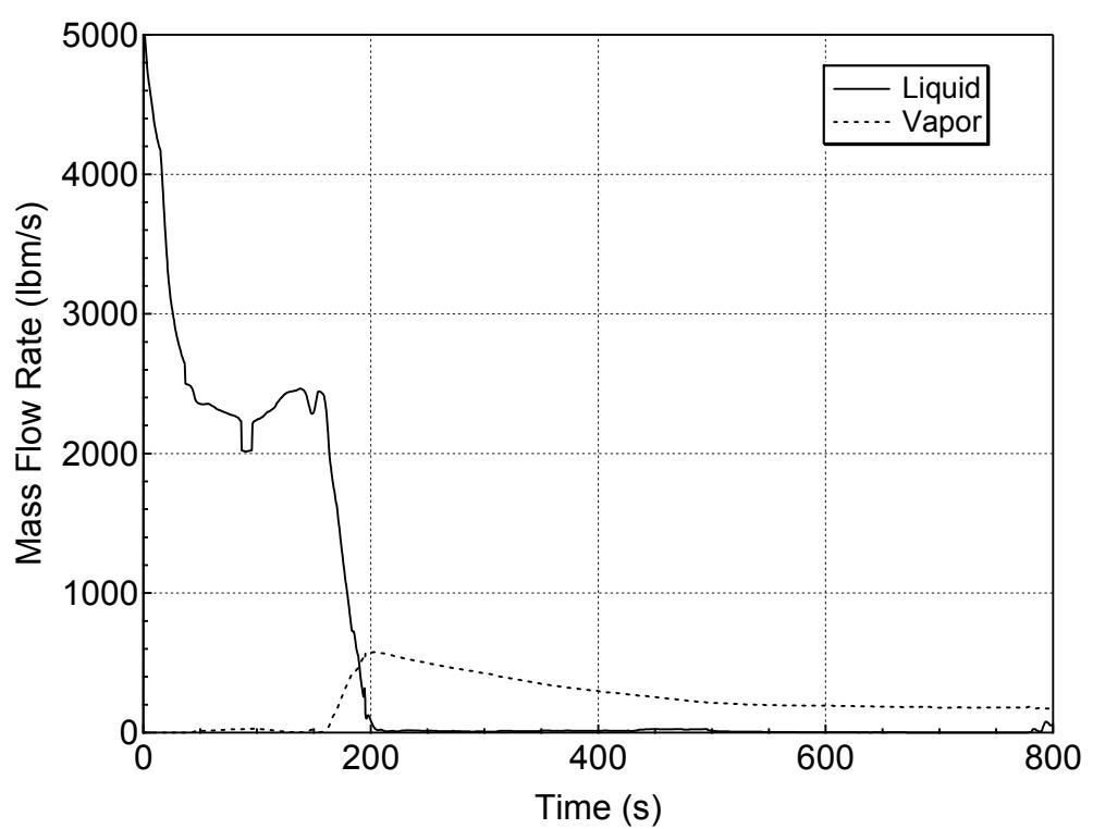
**Figure 5.3.1.b-30 Liquid and Vapor Discharges through the Break
