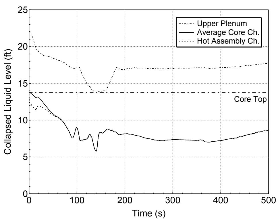
**Figure 5.3.1.c-7 Core and Upper Plenum Collapsed Levels for 7-inch Break (Top)
