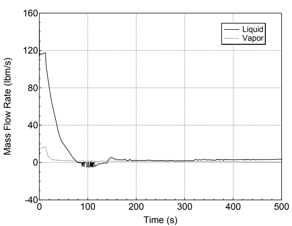
**Figure 5.3.1.d-27 Hot Assembly Exit Vapor and Liquid Mass Flowrates
