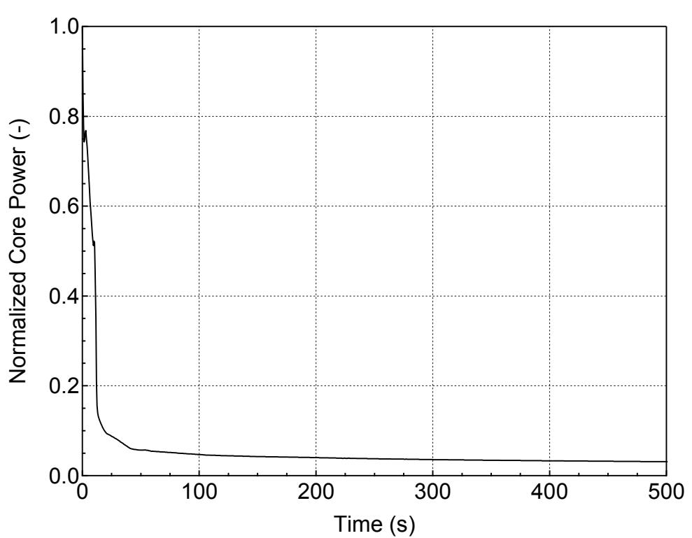
**Figure 5.3.2.b-2 Normalized Core Power for 13-inch Break (Top)
