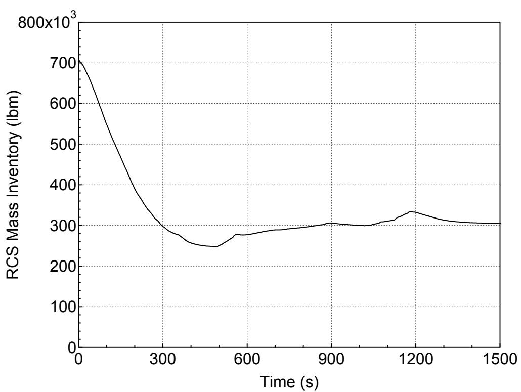
**Figure 5.1.3-5 RCS Mass Inventory for Pressurizer Steam Phase Break
