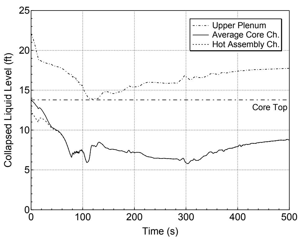
**Figure 5.2.h-7 Core and Upper Plenum Collapsed Levels for 8-inch Break (Bottom)
