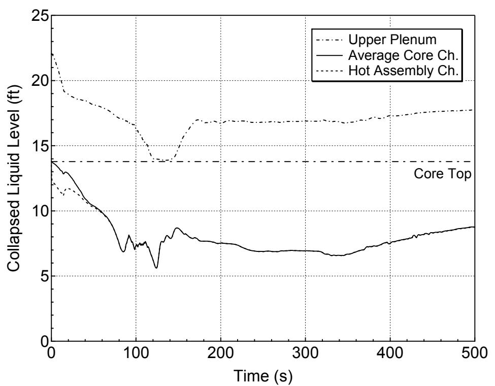
**Figure 5.3.1.d-7 Core and Upper Plenum Collapsed Levels for 7.5-inch Break (Bottom)
