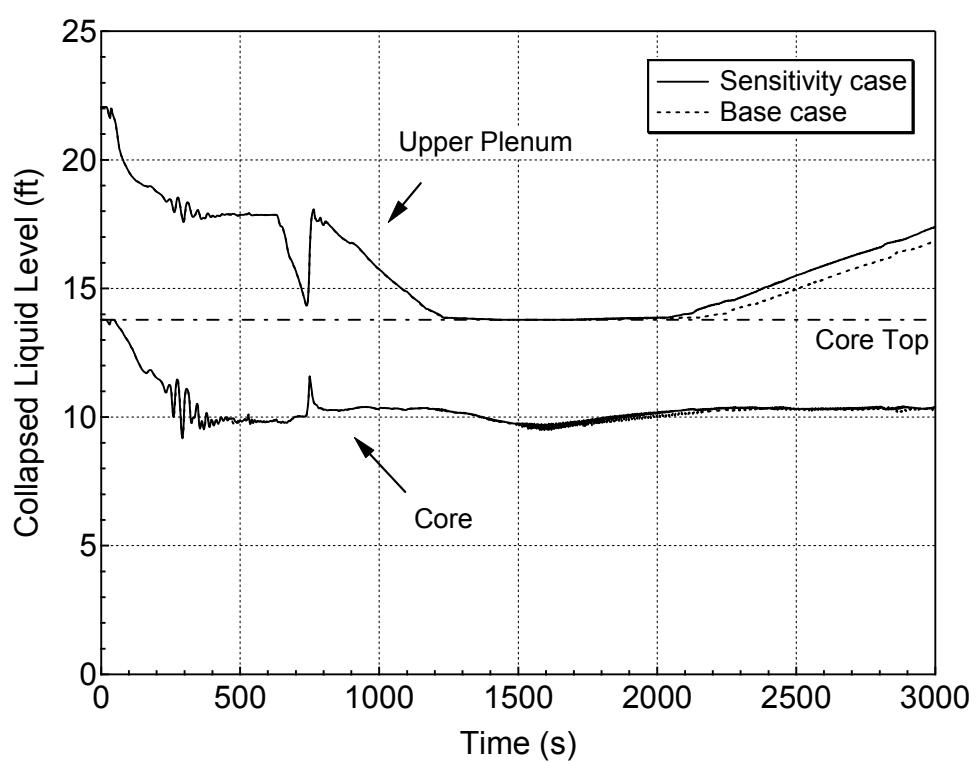
**Figure 5.5.c-9 Average Core and Upper Plenum Collapsed Levels for DVI-line Break
