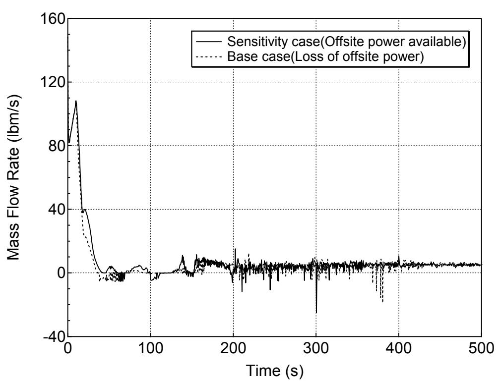
**Figure 5.6.2-25 Hot Assembly Exit Liquid Mass Flowrate for 1-ft<sup>2</sup> Break (Top)
