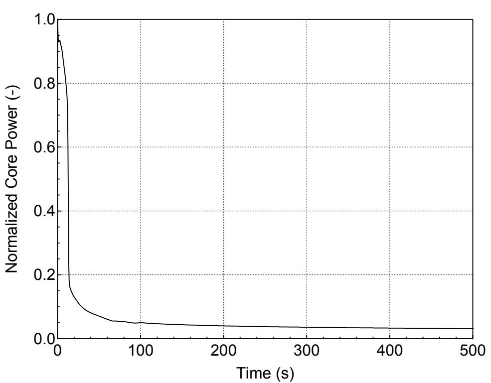
**Figure 5.2.i-2 Normalized Core Power for 9-inch Break (Bottom)
