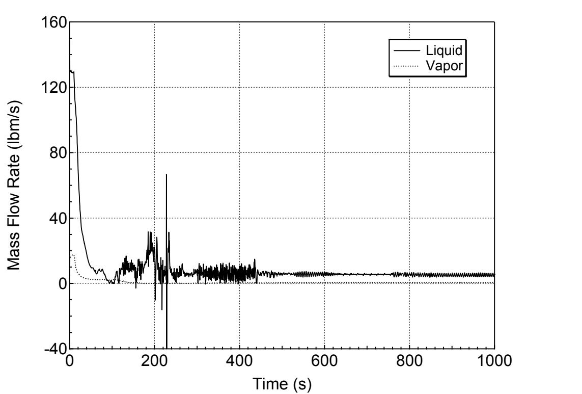
**Figure 5.1.1.b-18 Hot Assembly Exit Vapor and Liquid Mass Flowrates
