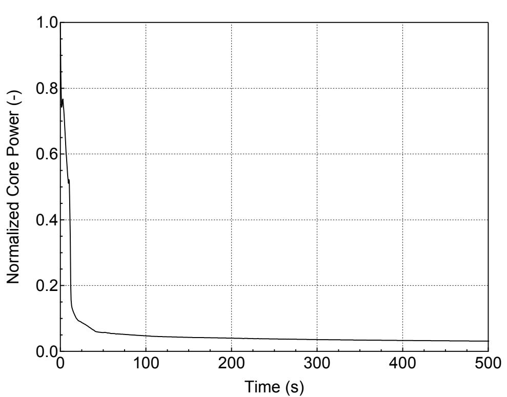
**Figure 5.2.m-2 Normalized Core Power for 13-inch Break (Bottom)
