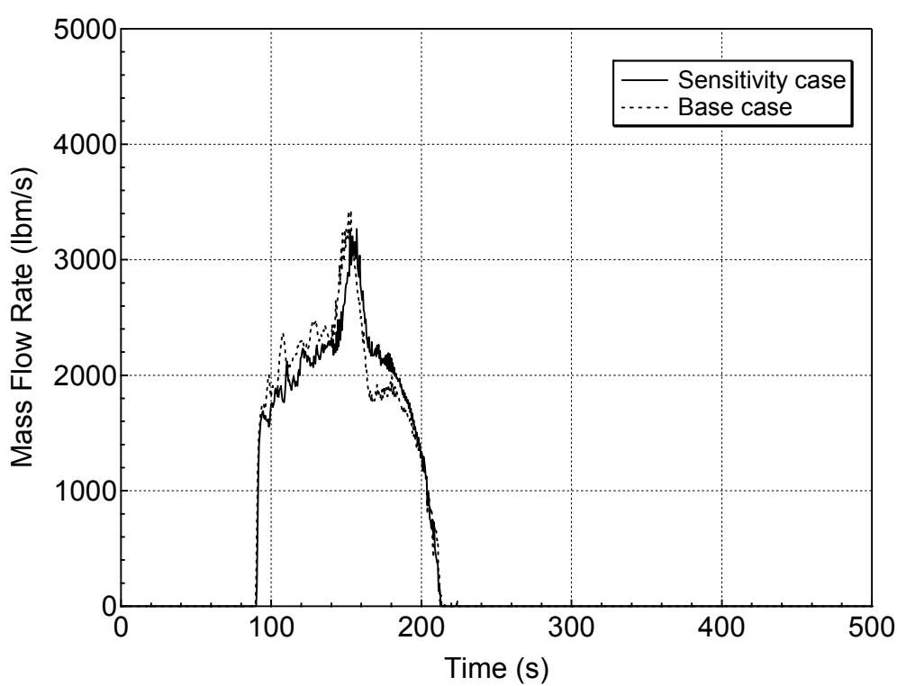
**Figure 5.4.1-18 Accumulator Injection Mass Flowrate for 1-ft<sup>2</sup> Break (Top)
