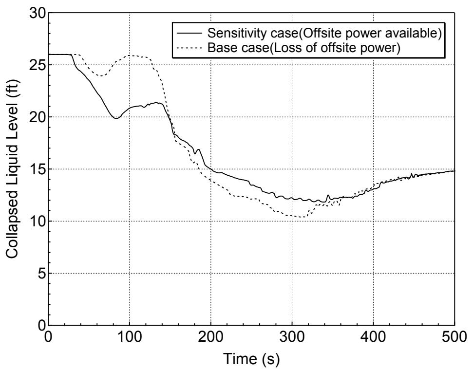
**Figure 5.6.2-8 Downcomer Collapsed Level for 7.5-inch Break (Top)
