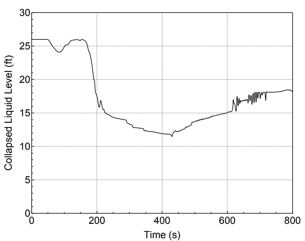
**Figure 5.3.1.b-15 Downcomer Collapsed Level for 6.5-inch Break (Top)
