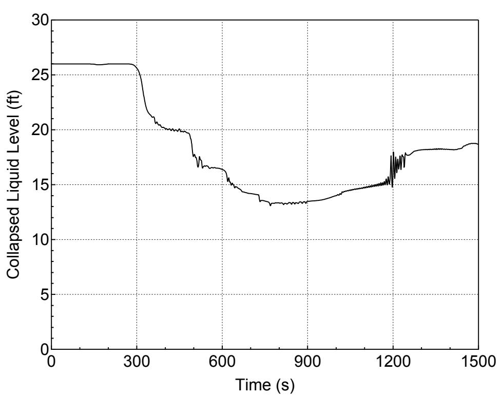
**Figure 5.2.d-6 Downcomer Collapsed Level for 4-inch Break (Bottom)
