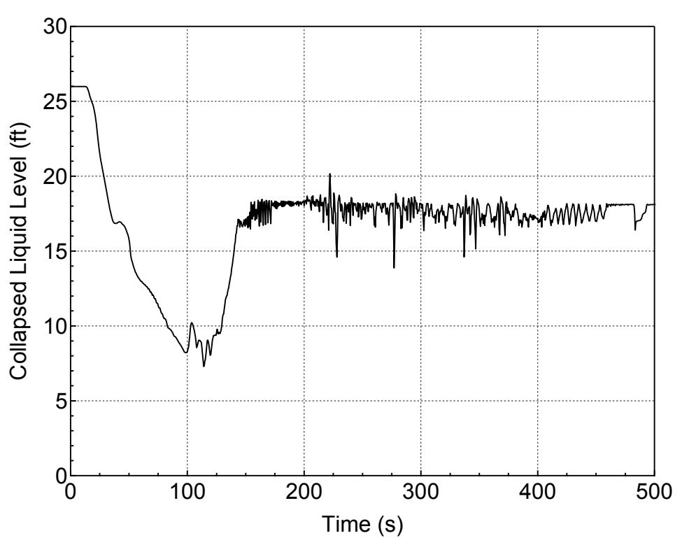
**Figure 5.3.2.b-6 Downcomer Collapsed Level for 13-inch Break (Top)
