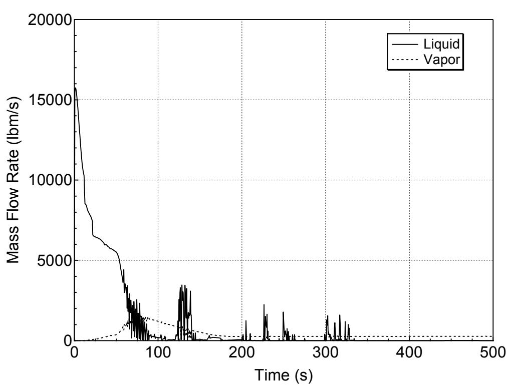
**Figure 5.3.2.a-3 Liquid and Vapor Discharges through the Break
