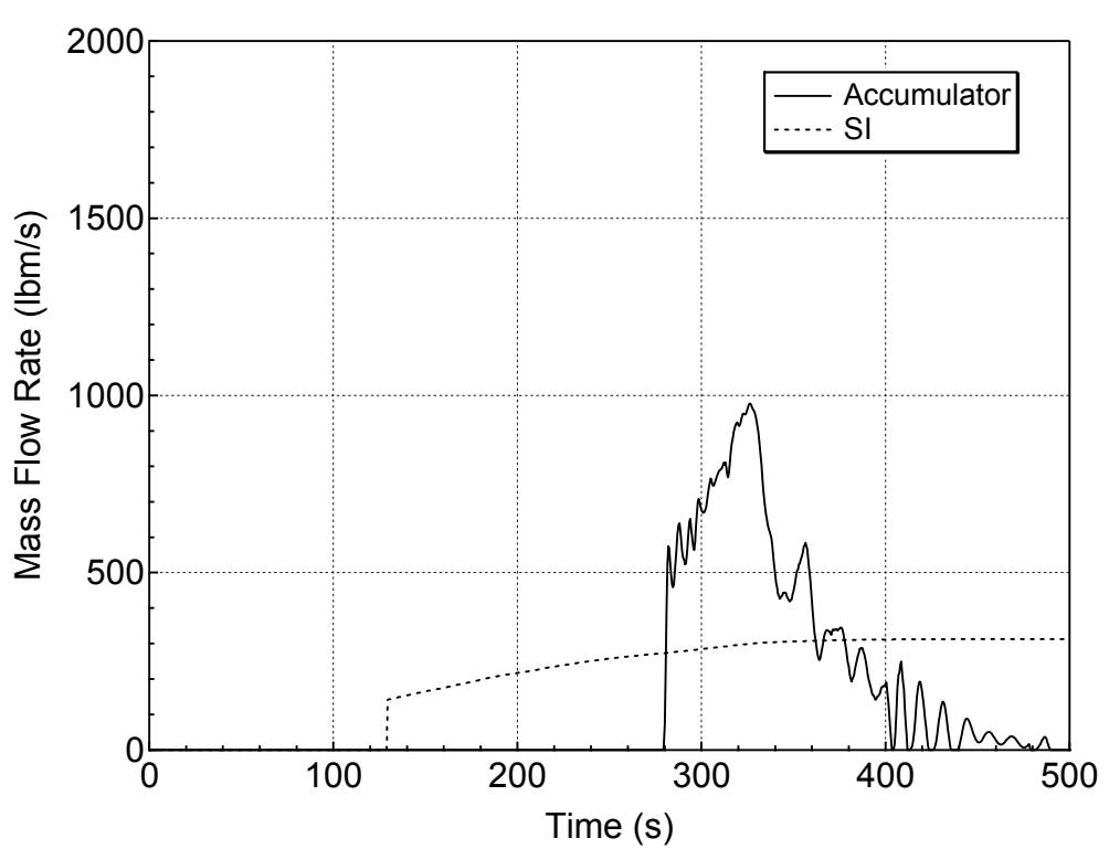
**Figure 5.2.h-4 Accumulator and Safety Injection Mass Flowrates
