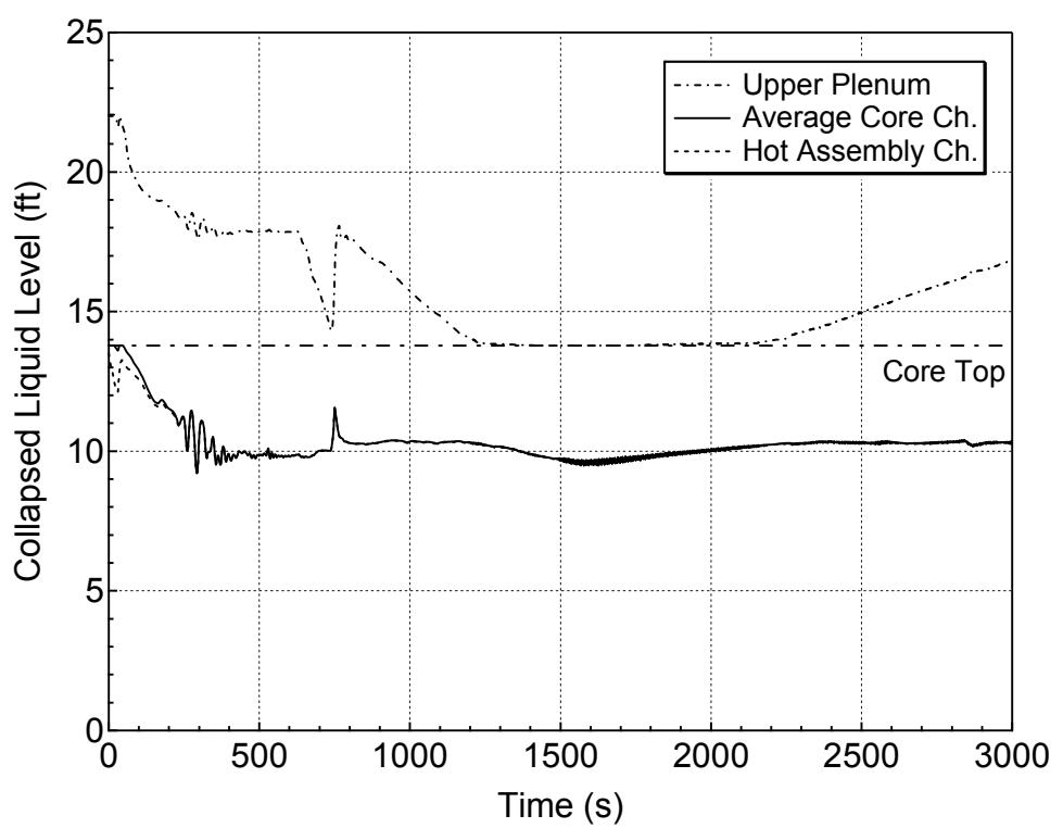
**Figure 5.1.2-7 Core and Upper Plenum Collapsed Levels for DVI-line Break
