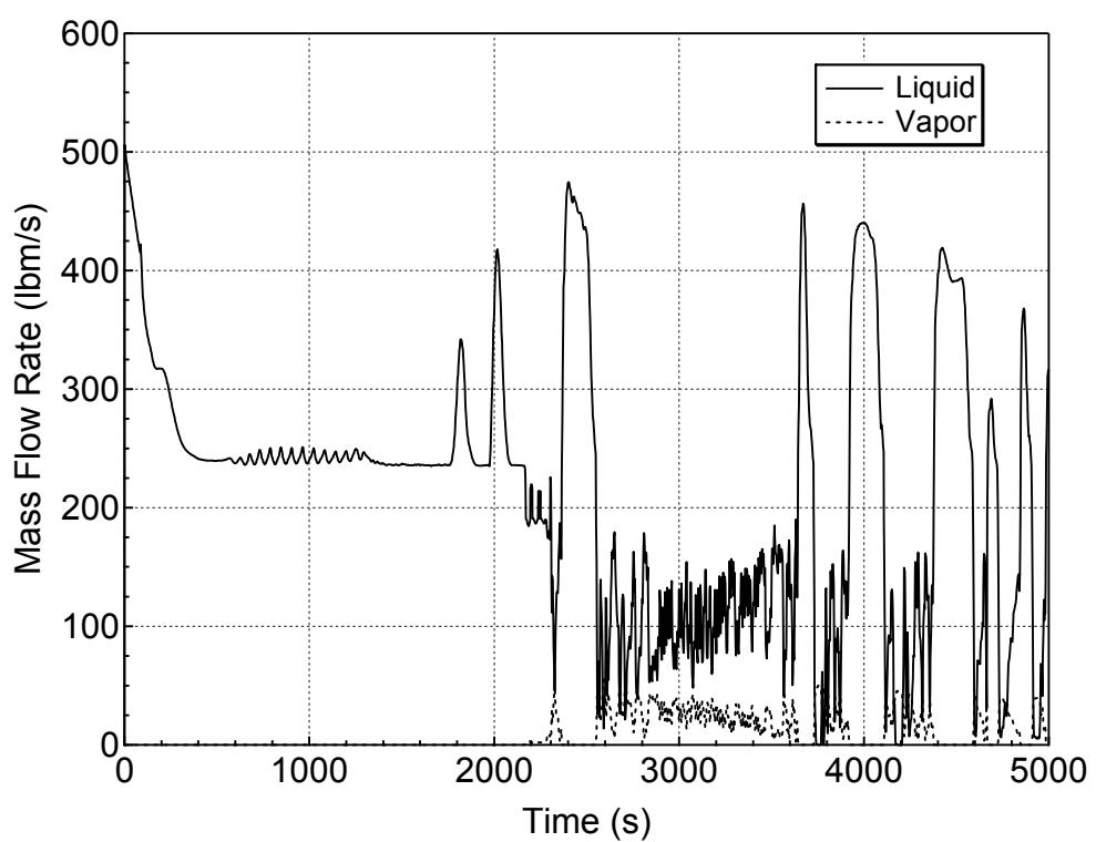
**Figure 5.1.1.c-3 Liquid and Vapor Discharges through the Break
