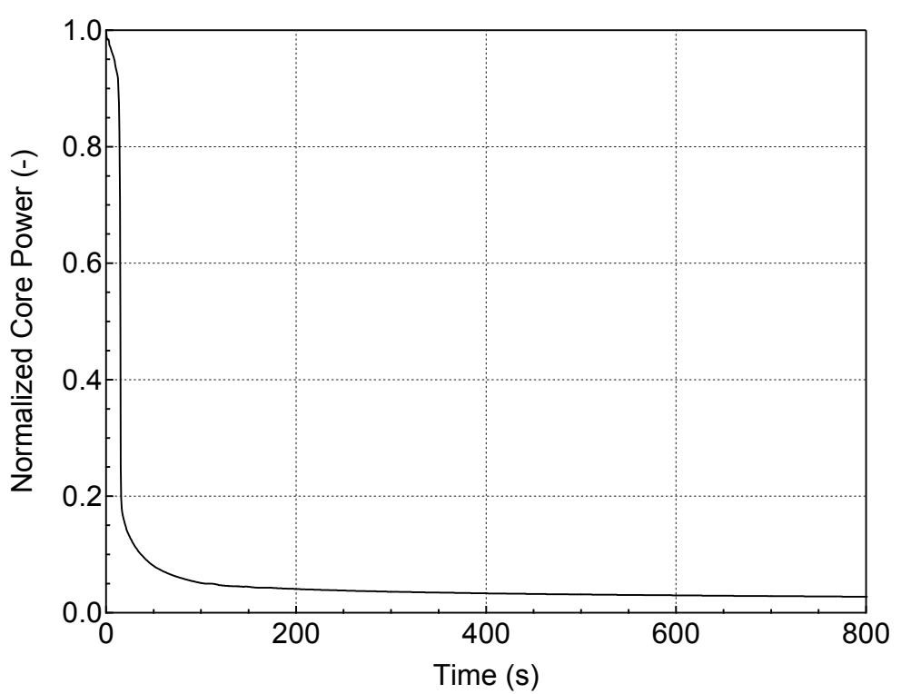
**Figure 5.3.1.b-29 Normalized Core Power for 6.5-inch Break (Homogeneous)
