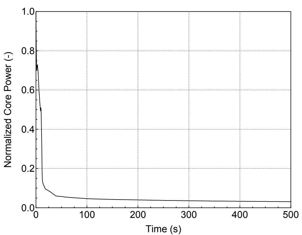
**Figure 5.3.2.c-11 Normalized Core Power for 1-ft<sup>2</sup> Break (Side)
