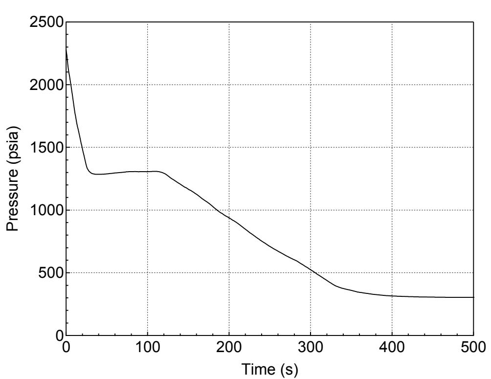
**Figure 5.2.h-1 RCS (Pressurizer) Pressure Transient for 8-inch Break (Bottom)
