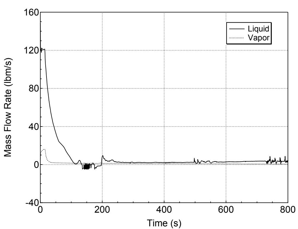
**Figure 5.3.1.a-27 Hot Assembly Exit Vapor and Liquid Mass Flowrates
