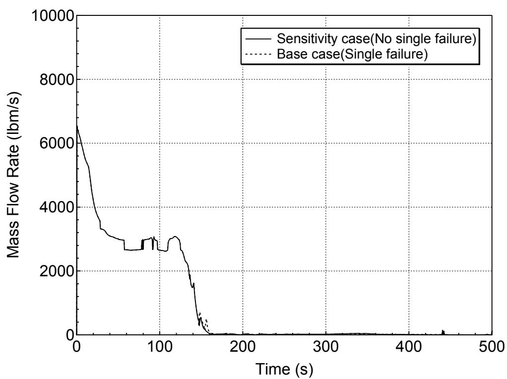
**Figure 5.6.1-3 Liquid Discharge through the Break for 7.5-inch Break (Top)
