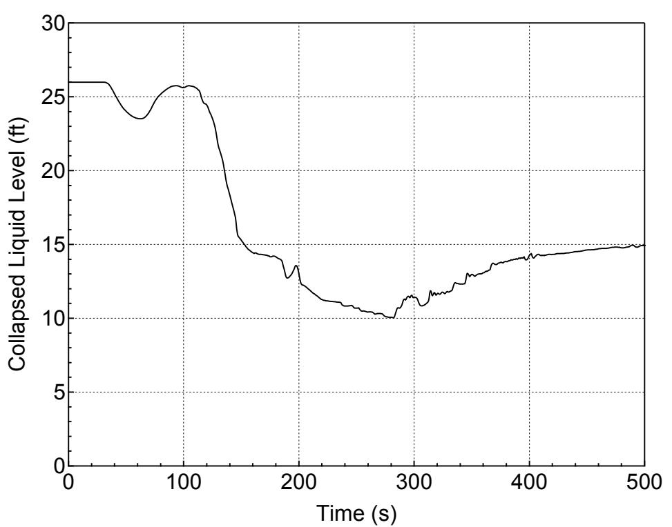
**Figure 5.3.1.e-15 Downcomer Collapsed Level for 8-inch Break (Side)
