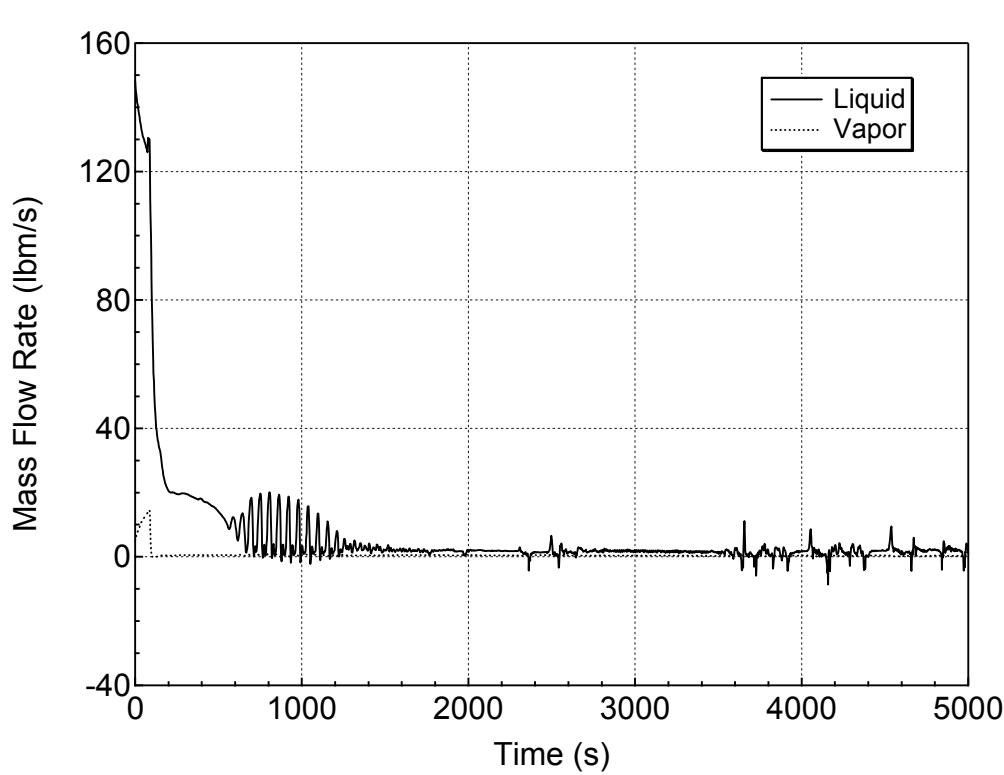
**Figure 5.1.1.c-9 Hot Assembly Exit Vapor and Liquid Mass Flowrates
