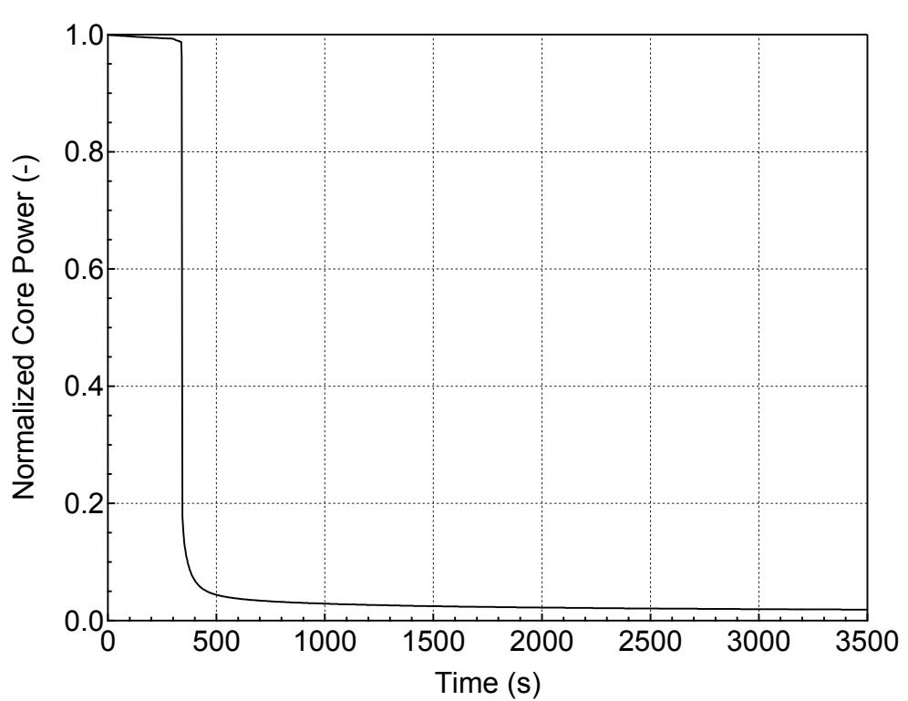
**Figure 5.2.a-2 Normalized Core Power for 1-inch Break (Bottom)
