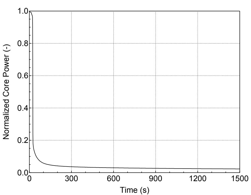
**Figure 5.2.d-2 Normalized Core Power for 4-inch Break (Bottom)
