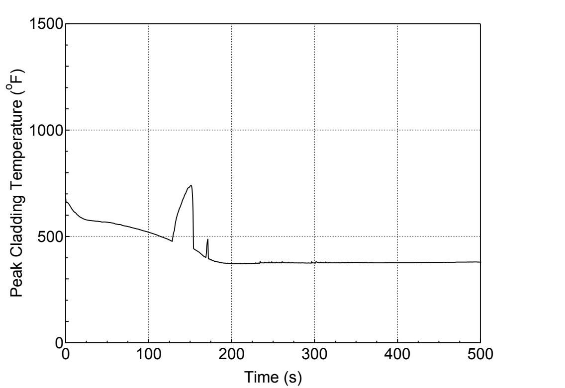
**Figure 5.2.I-8 PCT at All Elevations for Hot Rod in Hot Assembly
