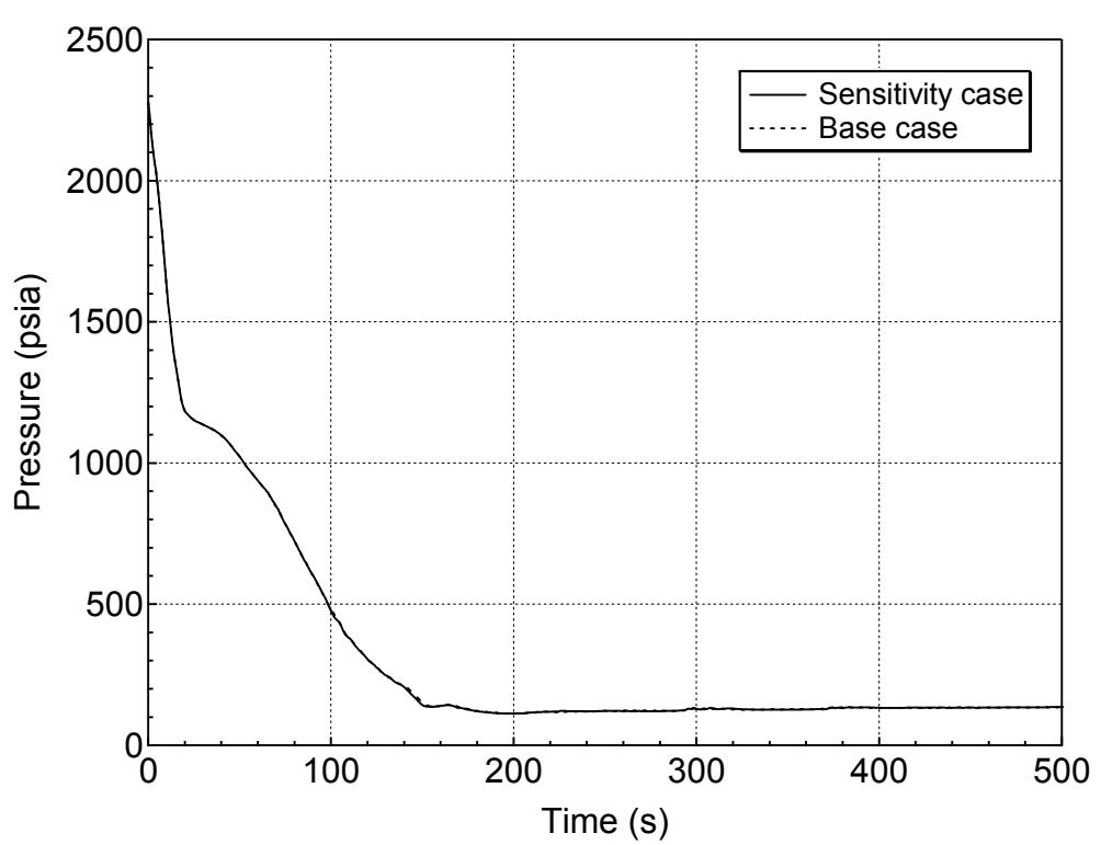
**Figure 5.5.b-1 RCS (Pressurizer) Pressure Transient for 1-ft<sup>2</sup> Break (Top)
