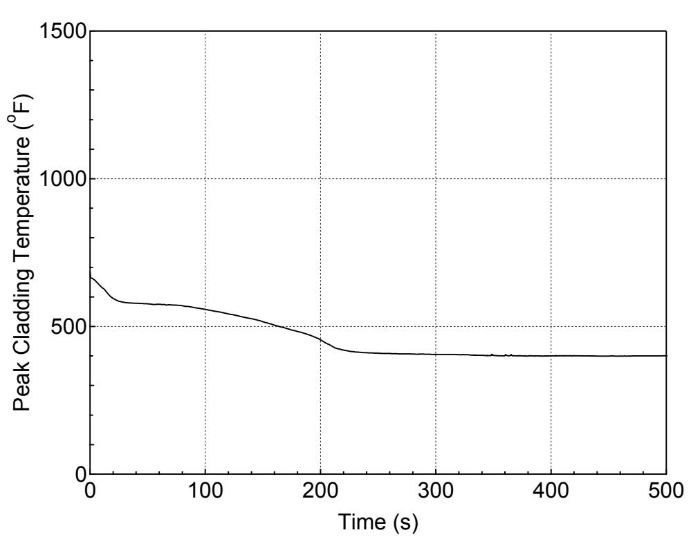
**Figure 5.2.j-8 PCT at All Elevations for Hot Rod in Hot Assembly
