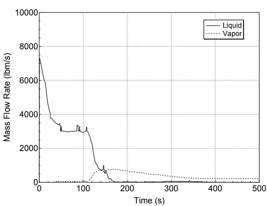
**Figure 5.2.h-3 Liquid and Vapor Discharges through the Break
