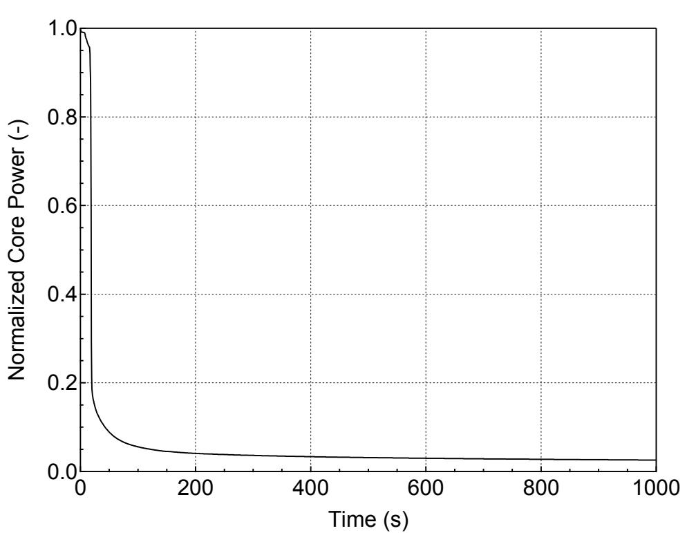
**Figure 5.2.e-2 Normalized Core Power for 5-inch Break (Bottom)
