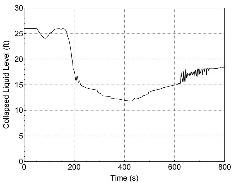
**Figure 5.3.1.b-33 Downcomer Collapsed Level for 6.5-inch Break (Homogeneous)
