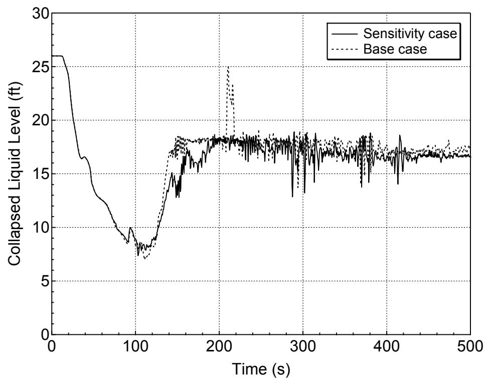
**Figure 5.4.3-21 Downcomer Collapsed Level for 1-ft<sup>2</sup> Break (Top)
