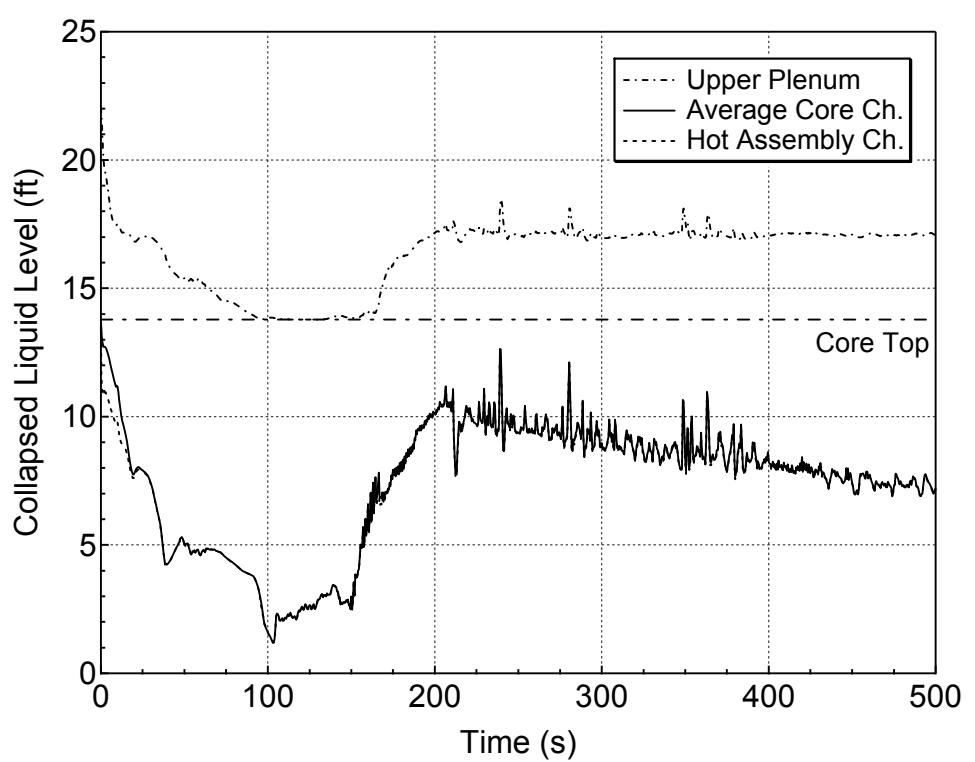
**Figure 5.2.n-7 Core and Upper Plenum Collapsed Levels for 1-ft<sup>2</sup> Break (Bottom)
