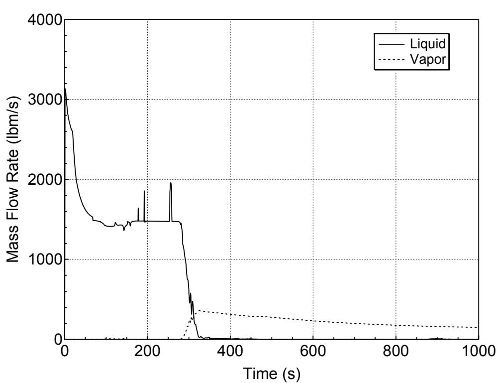
**Figure 5.2.e-3 Liquid and Vapor Discharges through the Break
