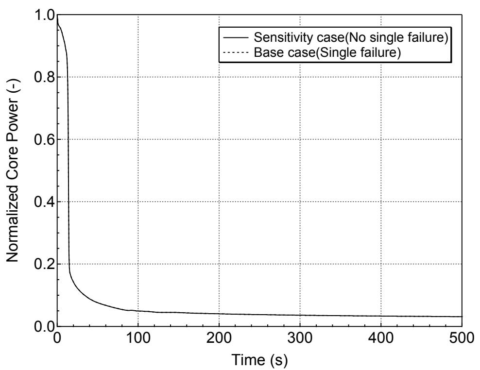
**Figure 5.6.1-2 Normalized Core Power for 7.5-inch Break (Top)
