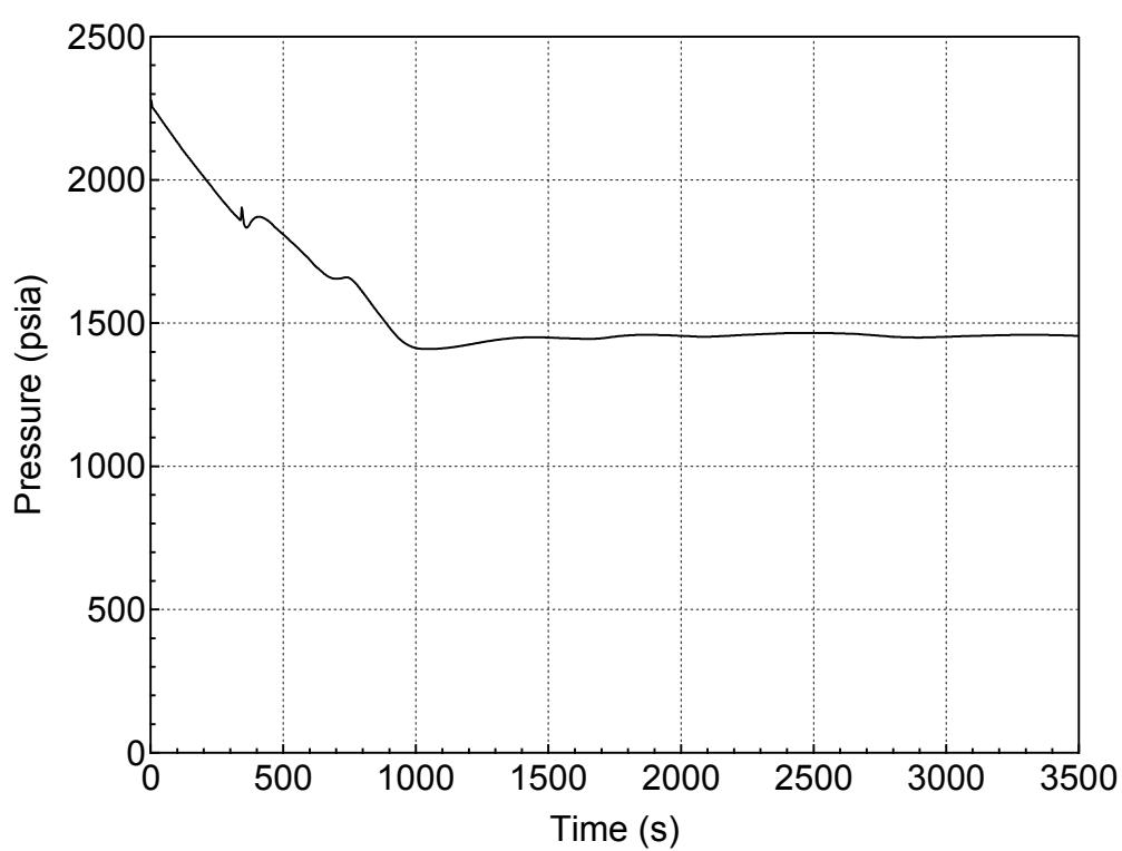
**Figure 5.2.a-1 RCS (Pressurizer) Pressure Transient for 1-inch Break (Bottom)
