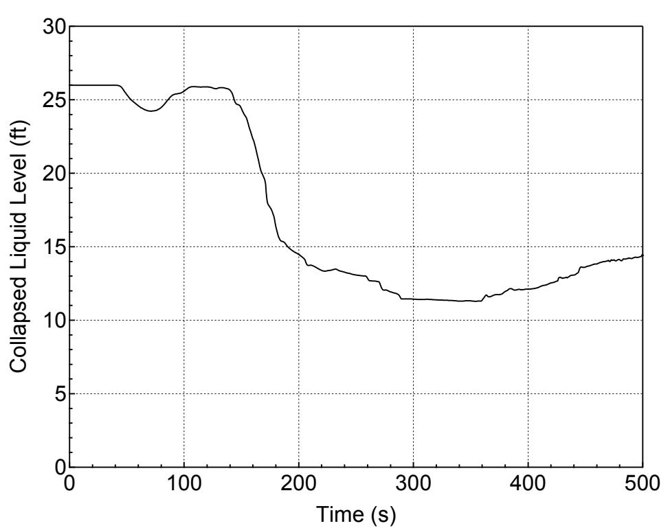
**Figure 5.3.1.c-15 Downcomer Collapsed Level for 7-inch Break (Side)
