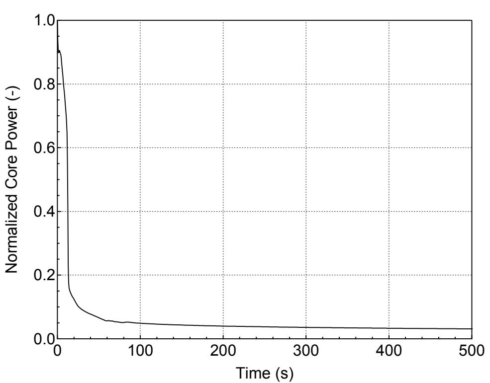
**Figure 5.2.j-2 Normalized Core Power for 10-inch Break (Bottom)
