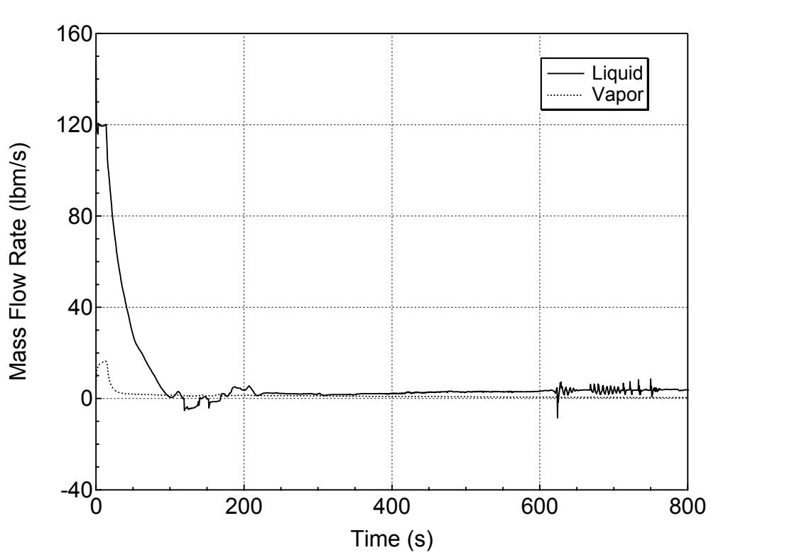
**Figure 5.3.1.b-9 Hot Assembly Exit Vapor and Liquid Mass Flowrates
