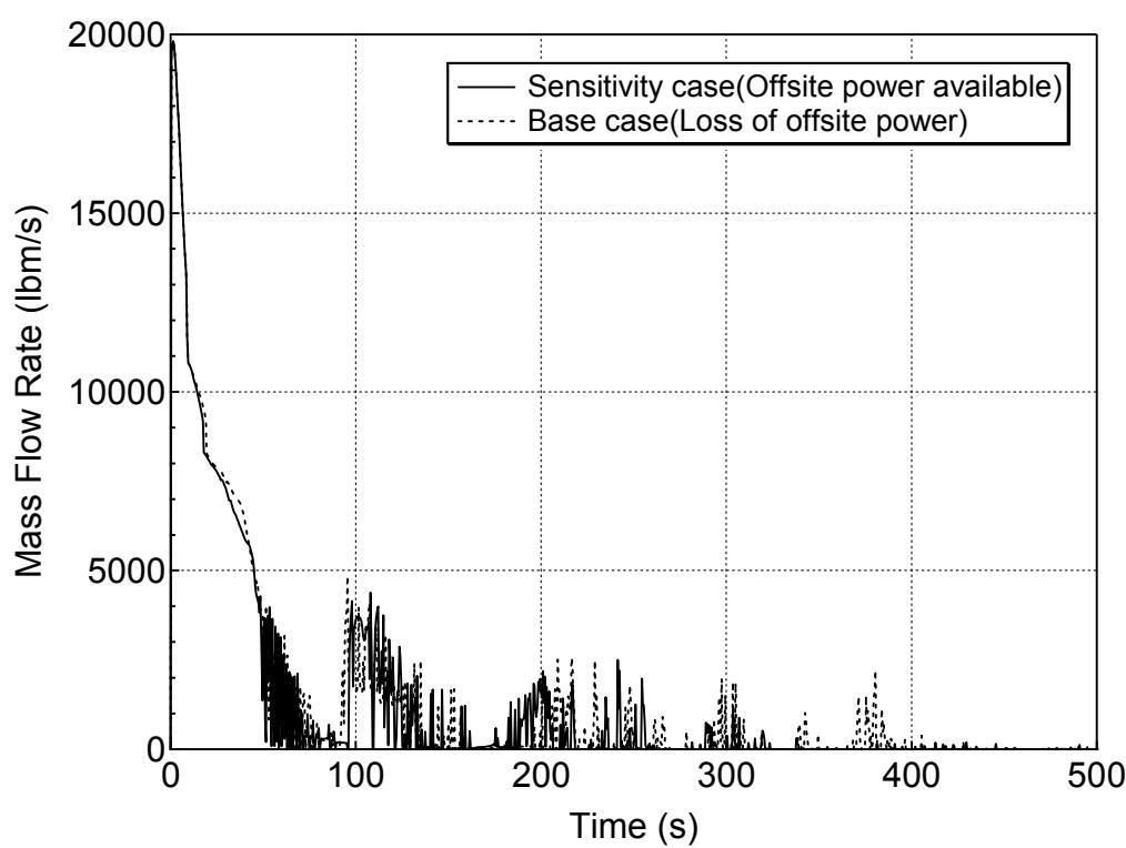
**Figure 5.6.2-16 Liquid Discharge through the Break for 1-ft<sup>2</sup> Break (Top)
