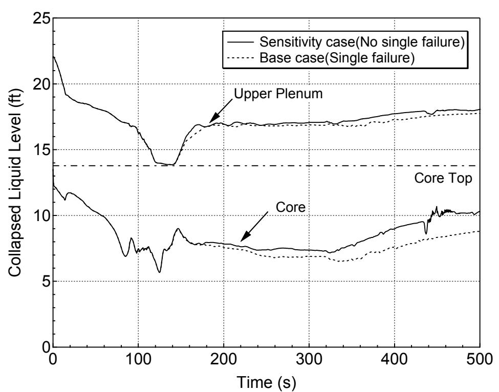
**Figure 5.6.1-10 Hot Assembly Core and Upper Plenum Collapsed Levels
