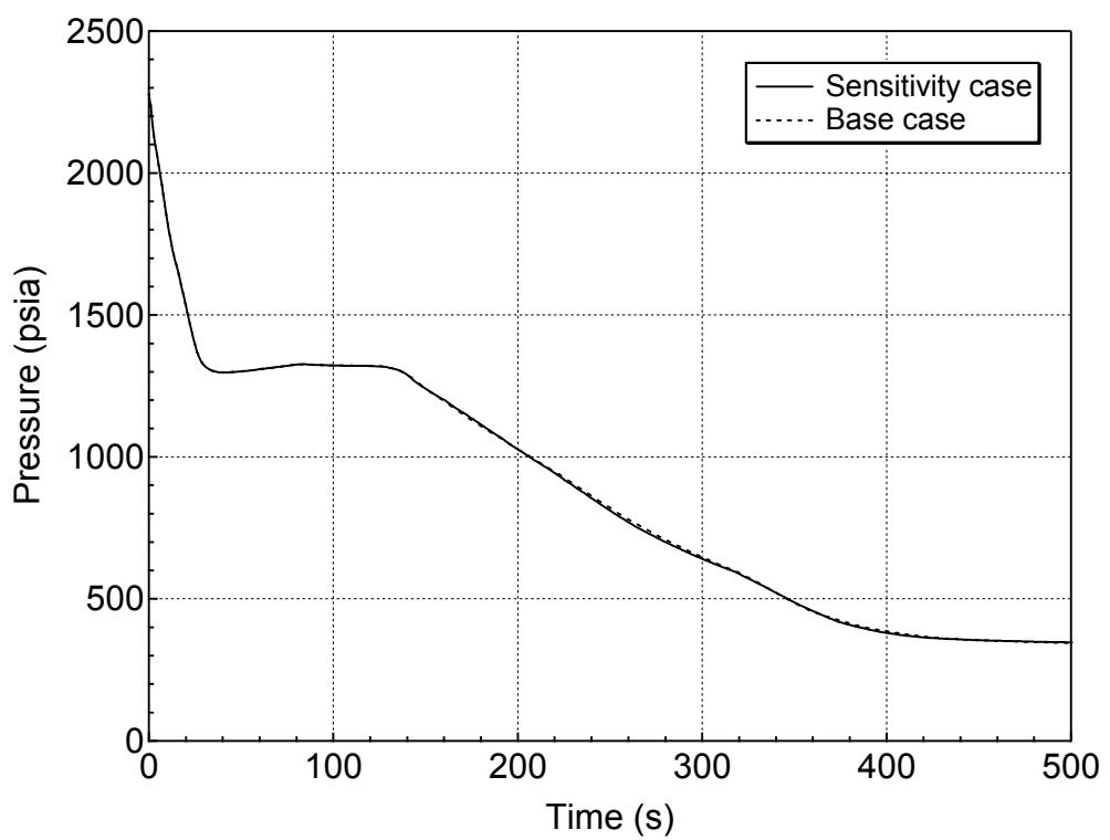
**Figure 5.4.3-1 RCS (Pressurizer) Pressure Transient for 7.5-inch Break (Top)
