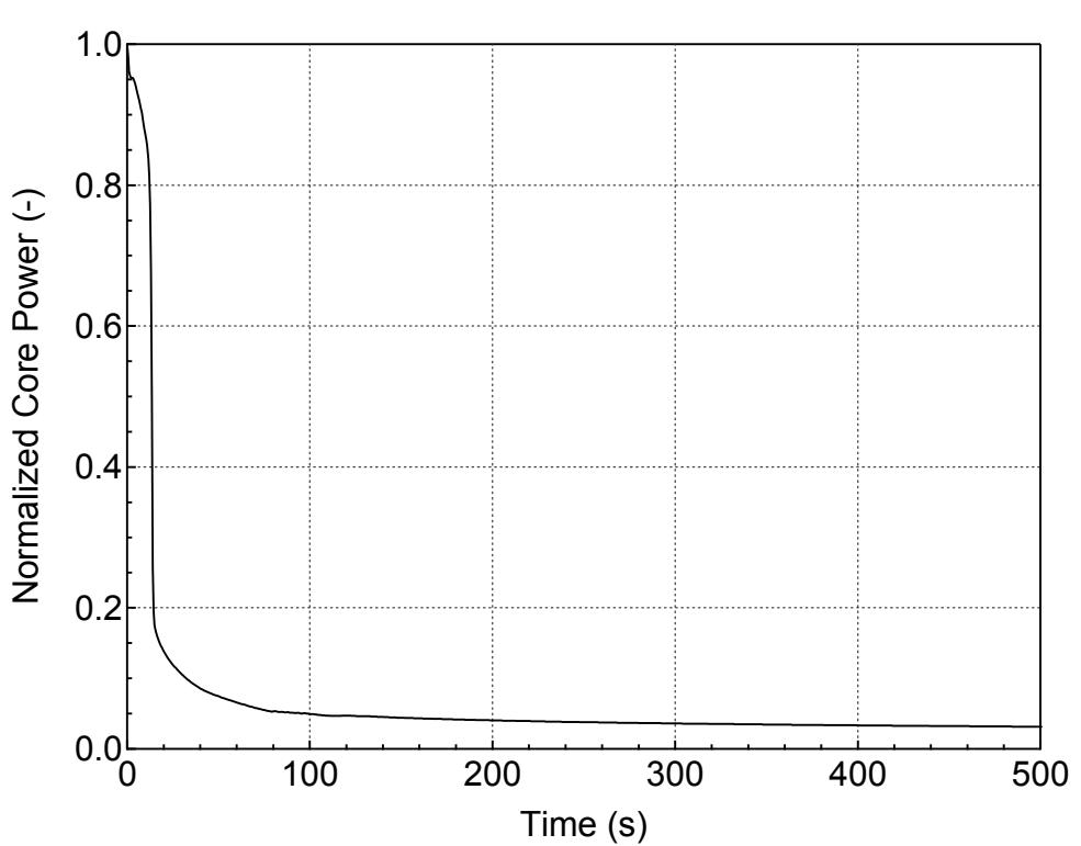
**Figure 5.3.1.e-2 Normalized Core Power for 8-inch Break (Top)
