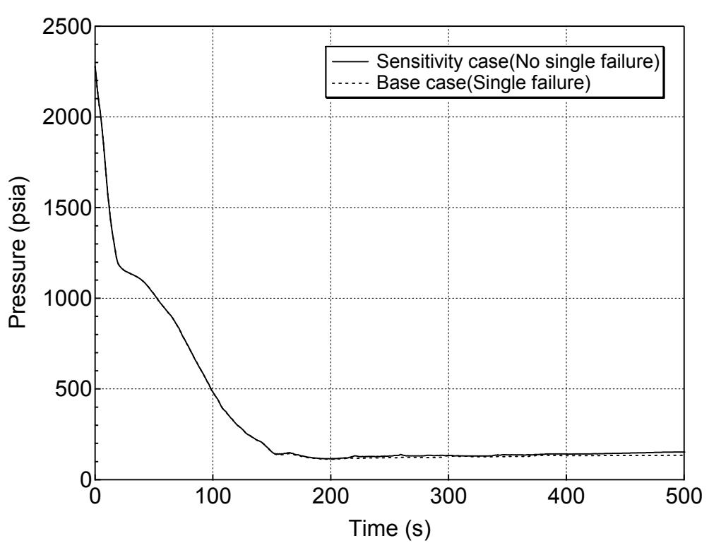
**Figure 5.6.1-14 RCS (Pressurizer) Pressure Transient for 1-ft<sup>2</sup> Break (Top)
