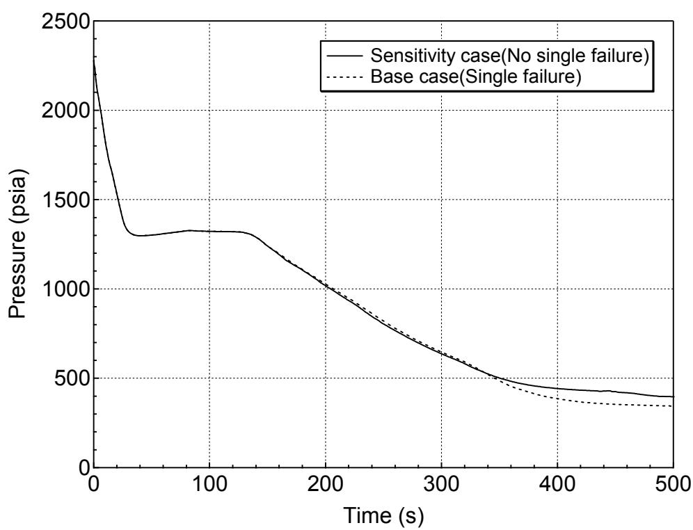
**Figure 5.6.1-1 RCS (Pressurizer) Pressure Transient for 7.5-inch Break (Top)
