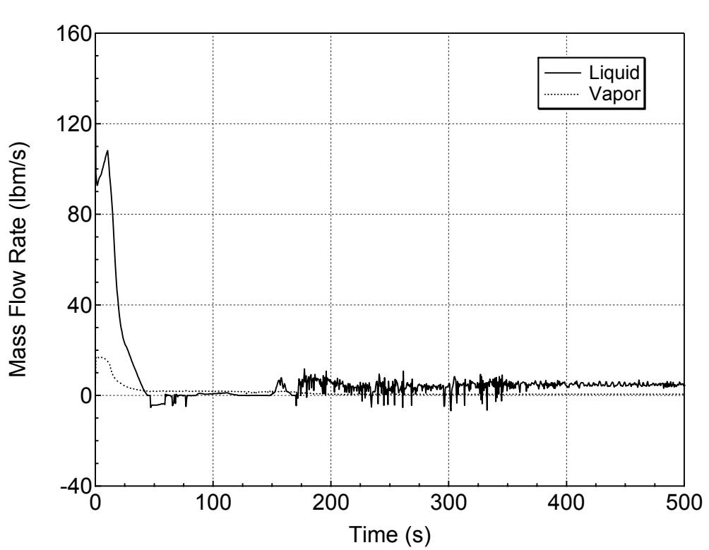
**Figure 5.2.I-9 Hot Assembly Exit Vapor and Liquid Mass Flowrates
