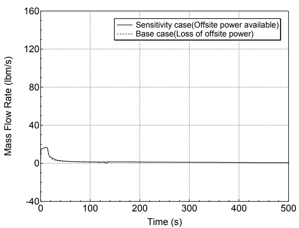
**Figure 5.6.2-13 Hot Assembly Exit Vapor Mass Flowrate for 7.5-inch Break (Top)
