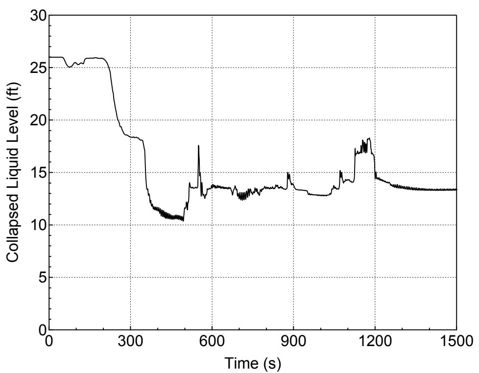
**Figure 5.1.3-6 Downcomer Collapsed Level for Pressurizer Steam Phase Break
