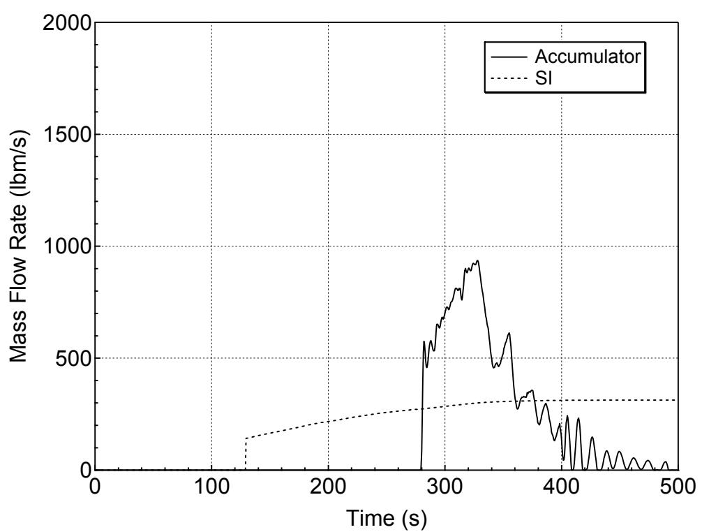
**Figure 5.3.1.e-22 Accumulator and Safety Injection Mass Flowrates
