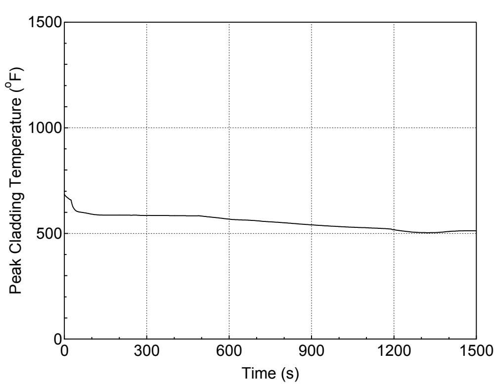
**Figure 5.2.d-8 PCT at All Elevations for Hot Rod in Hot Assembly
