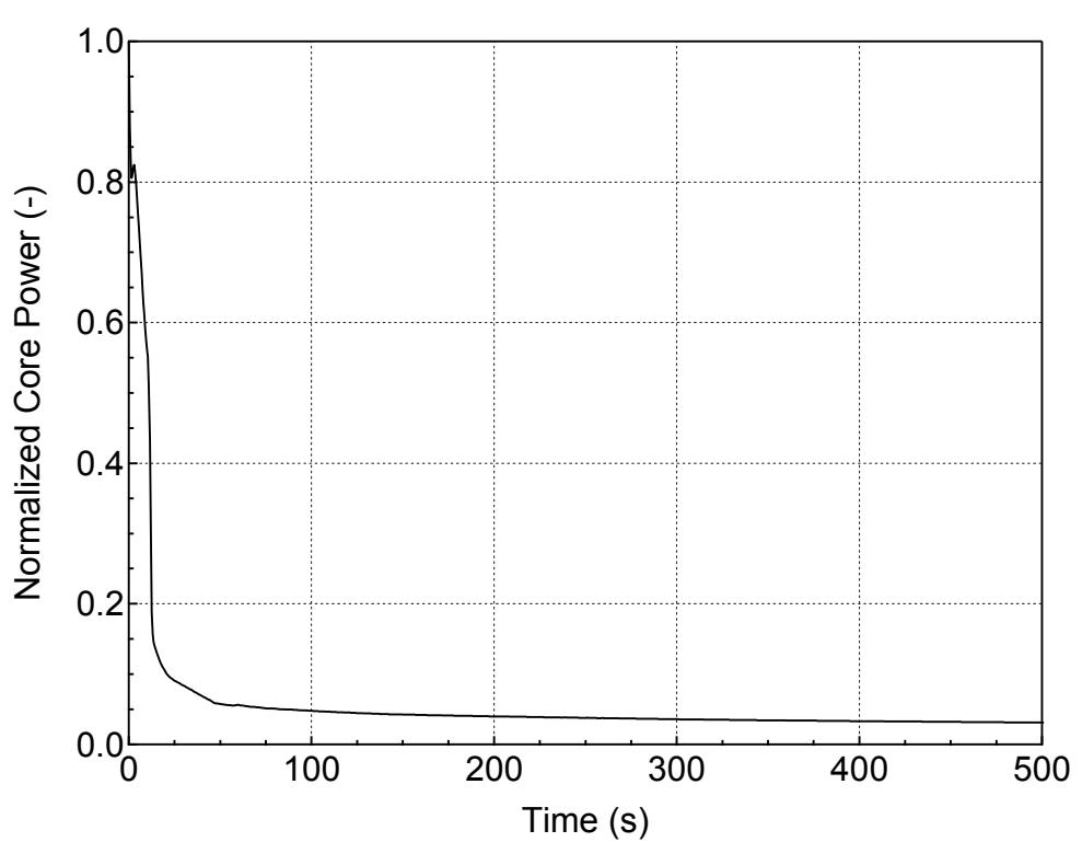
**Figure 5.3.2.a-11 Normalized Core Power for 12-inch Break (Side)
