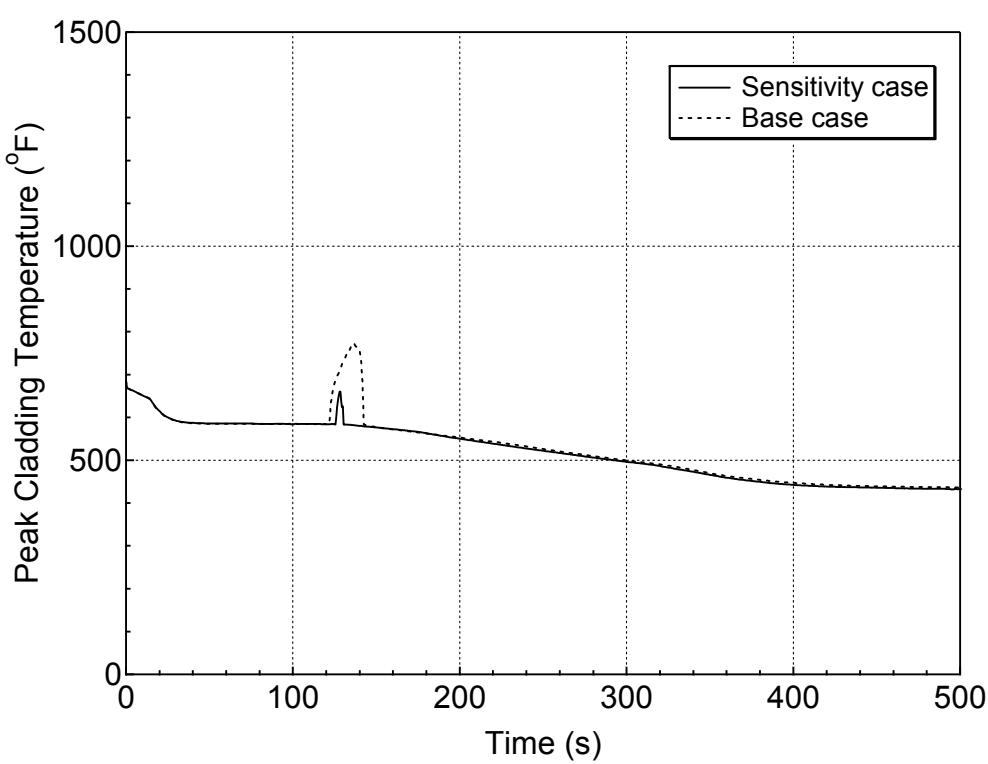
**Figure 5.4.2-11 PCT at All Elevations for Hot Rod in Hot Assembly
