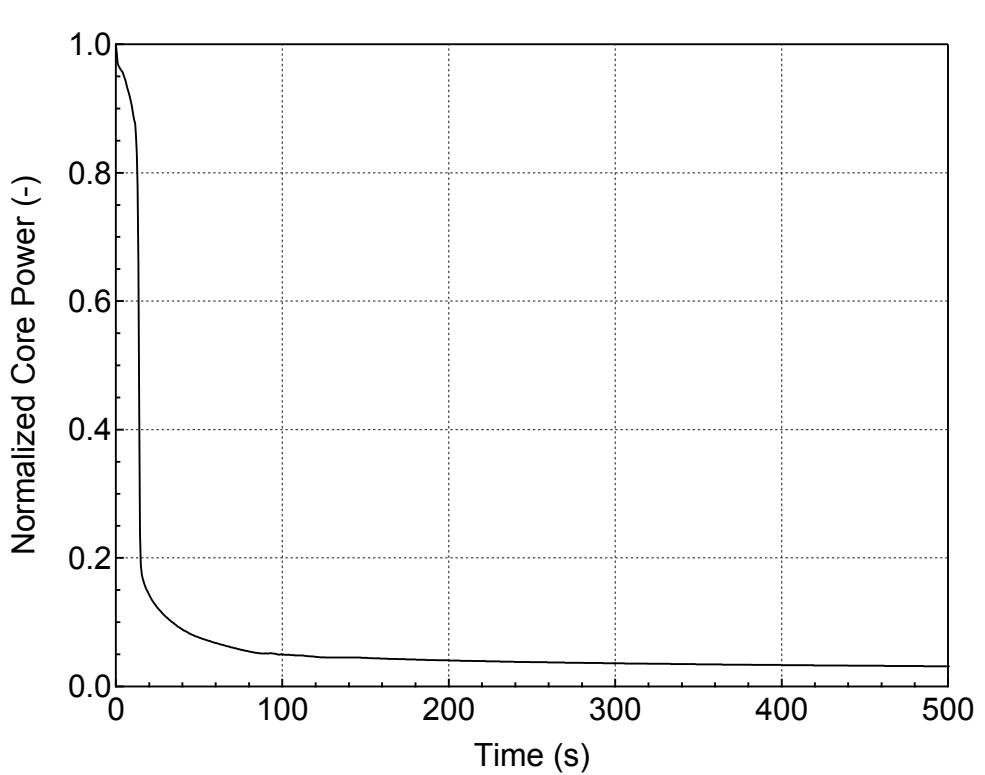
**Figure 5.3.1.d-20 Normalized Core Power for 7.5-inch Break (Side)
