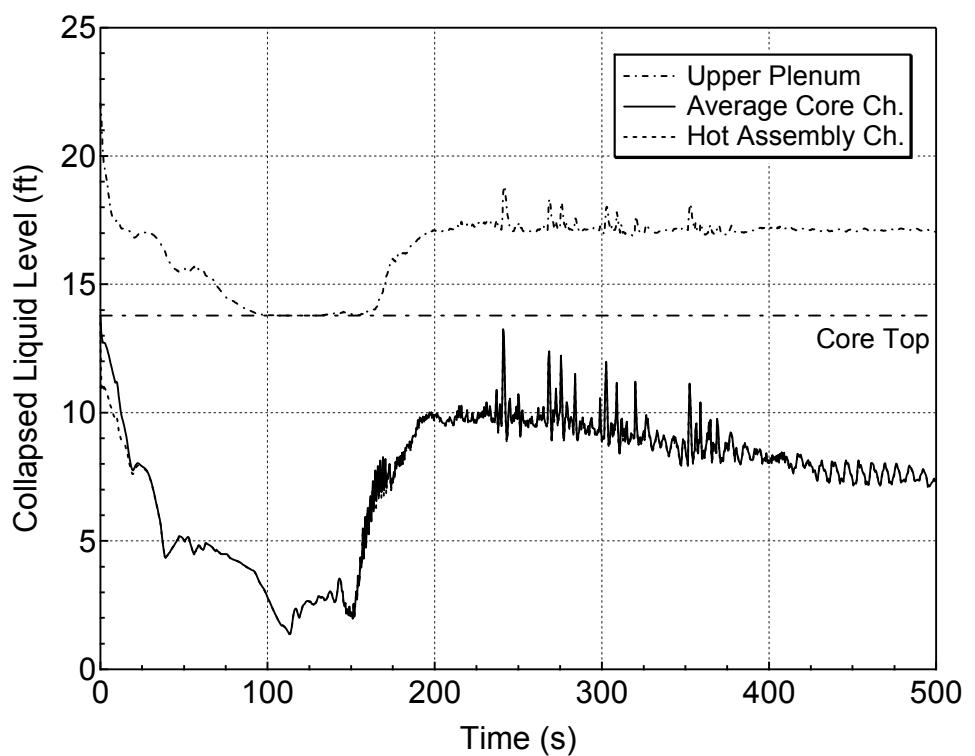
**Figure 5.3.2.c-25 Core and Upper Plenum Collapsed Levels
