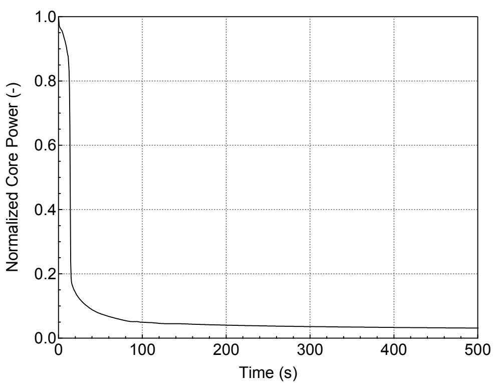
**Figure 5.3.1.d-29 Normalized Core Power for 7.5-inch Break (Homogeneous)
