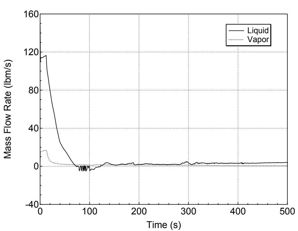
**Figure 5.2.h-9 Hot Assembly Exit Vapor and Liquid Mass Flowrates
