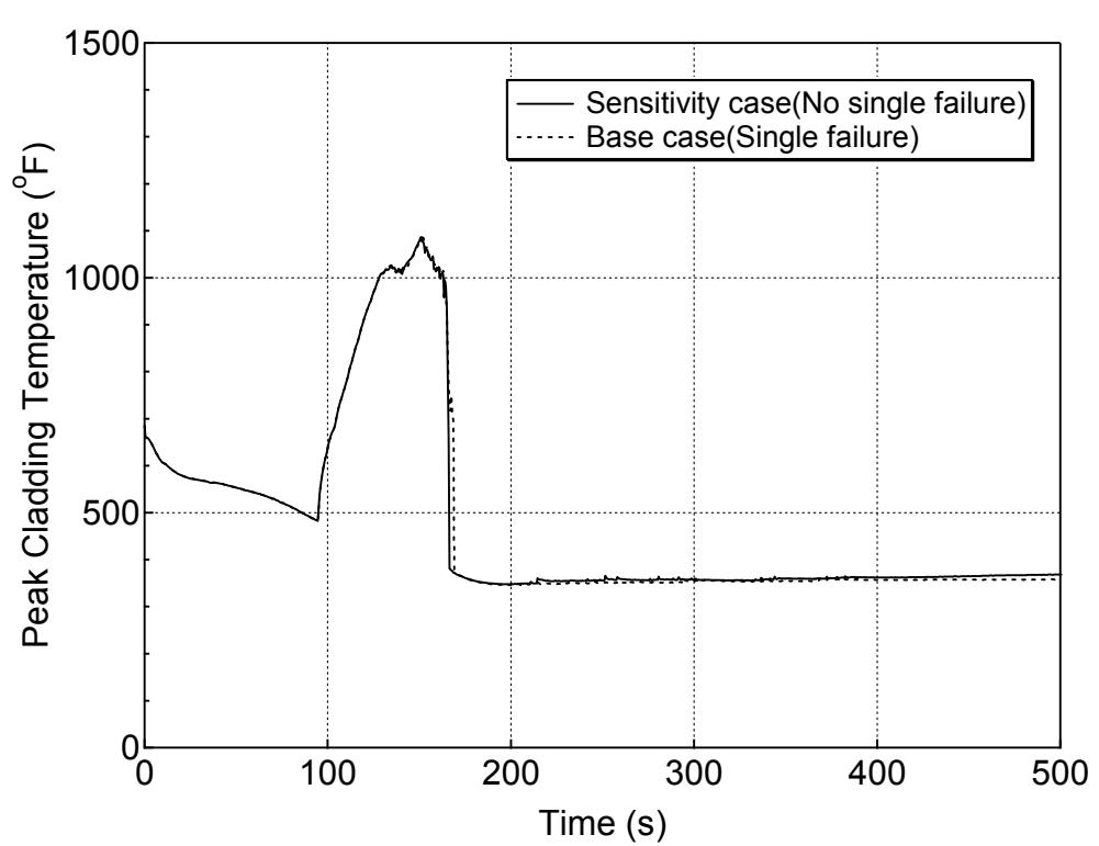
**Figure 5.6.1-24 PCT at All Elevations for Hot Rod in Hot Assembly for 1-ft<sup>2</sup> Break (Top)
