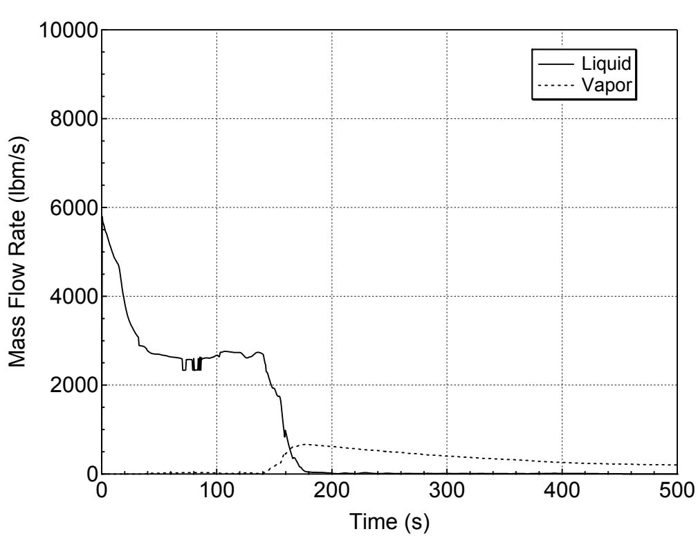
**Figure 5.3.1.c-3 Liquid and Vapor Discharges through the Break for 7-inch Break (Top)
