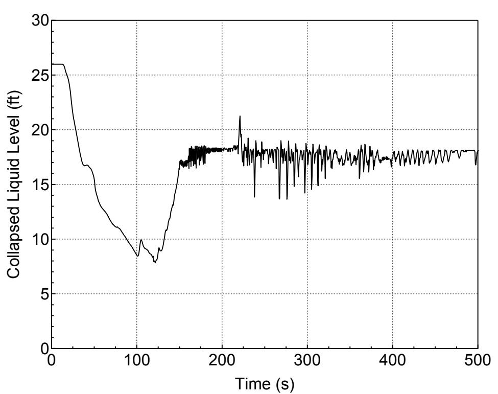
**Figure 5.3.2.b-15 Downcomer Collapsed Level for 13-inch Break (Side)
