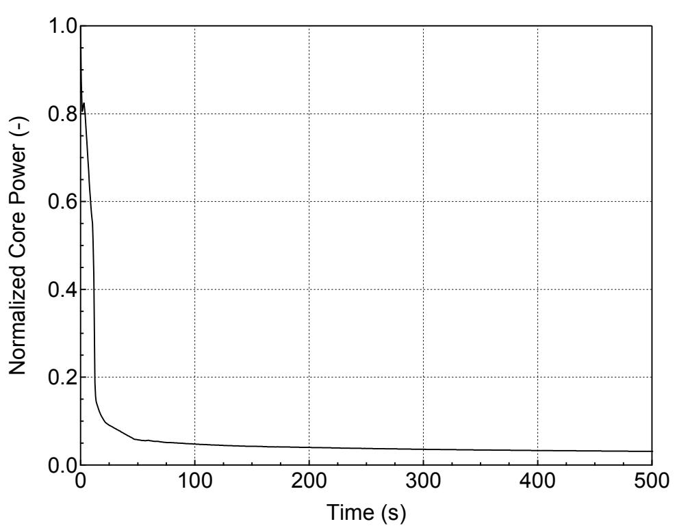
**Figure 5.2.I-2 Normalized Core Power for 12-inch Break (Bottom)
