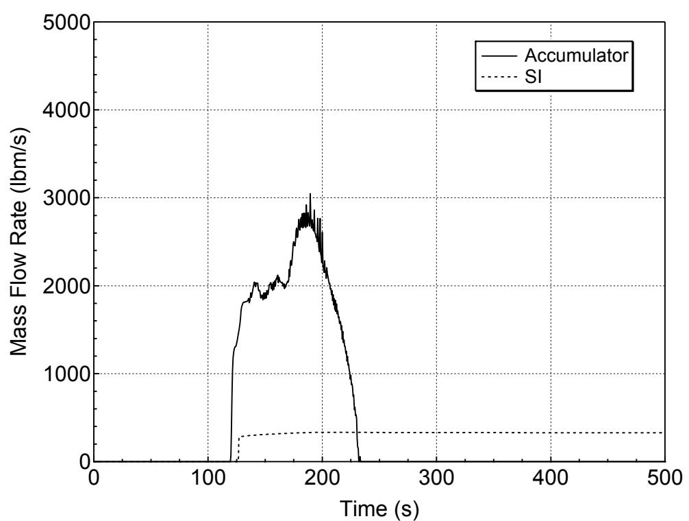
**Figure 5.3.2.a-22 Accumulator and Safety Injection Mass Flowrates
