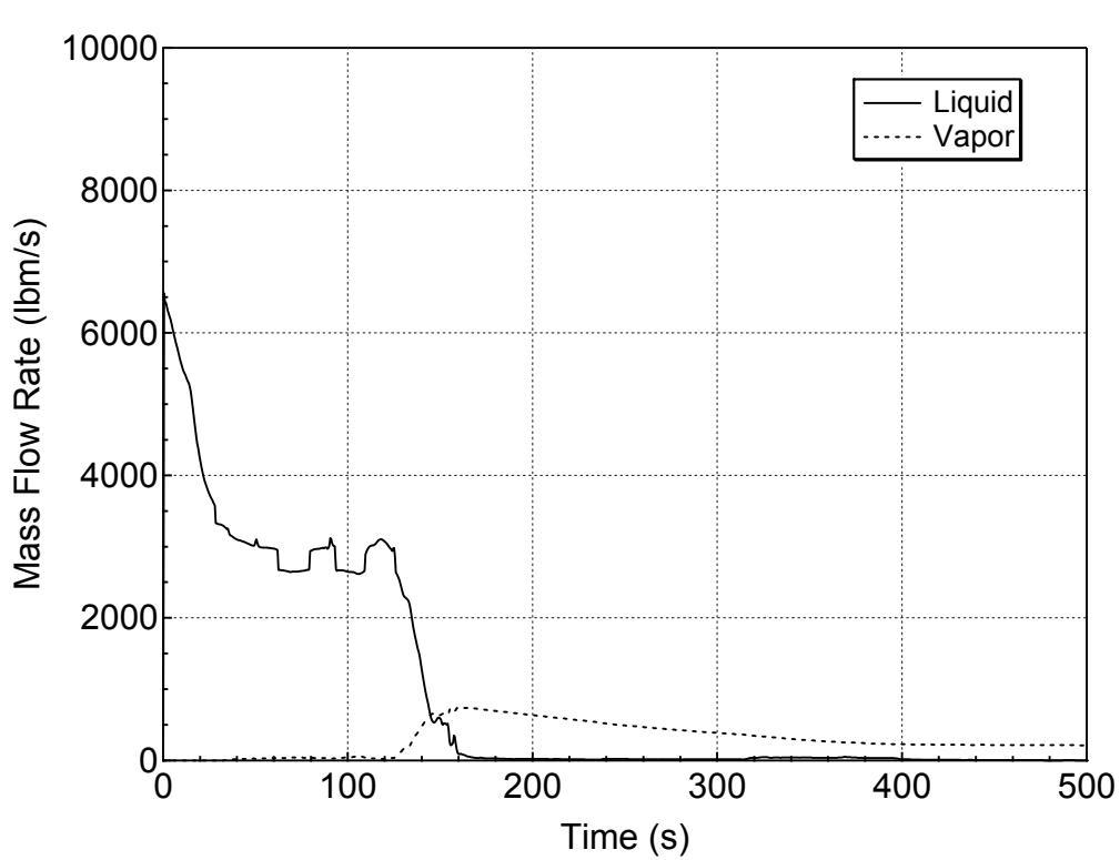
**Figure 5.3.1.d-3 Liquid and Vapor Discharges through the Break
