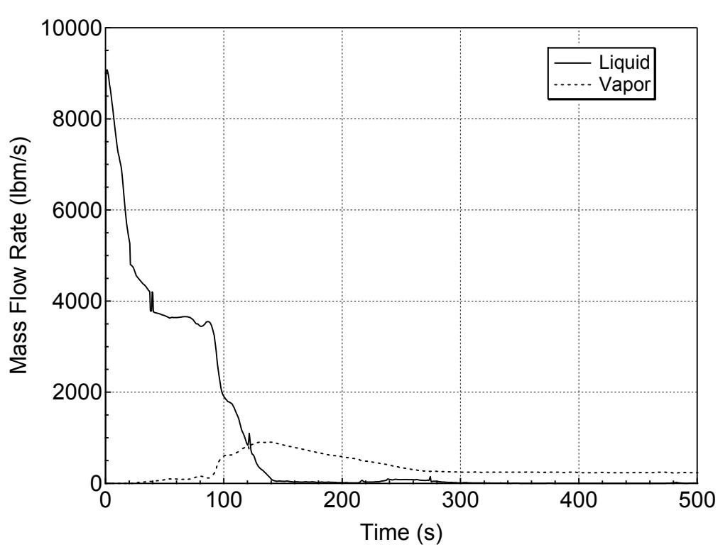
**Figure 5.2.i-3 Liquid and Vapor Discharges through the Break
