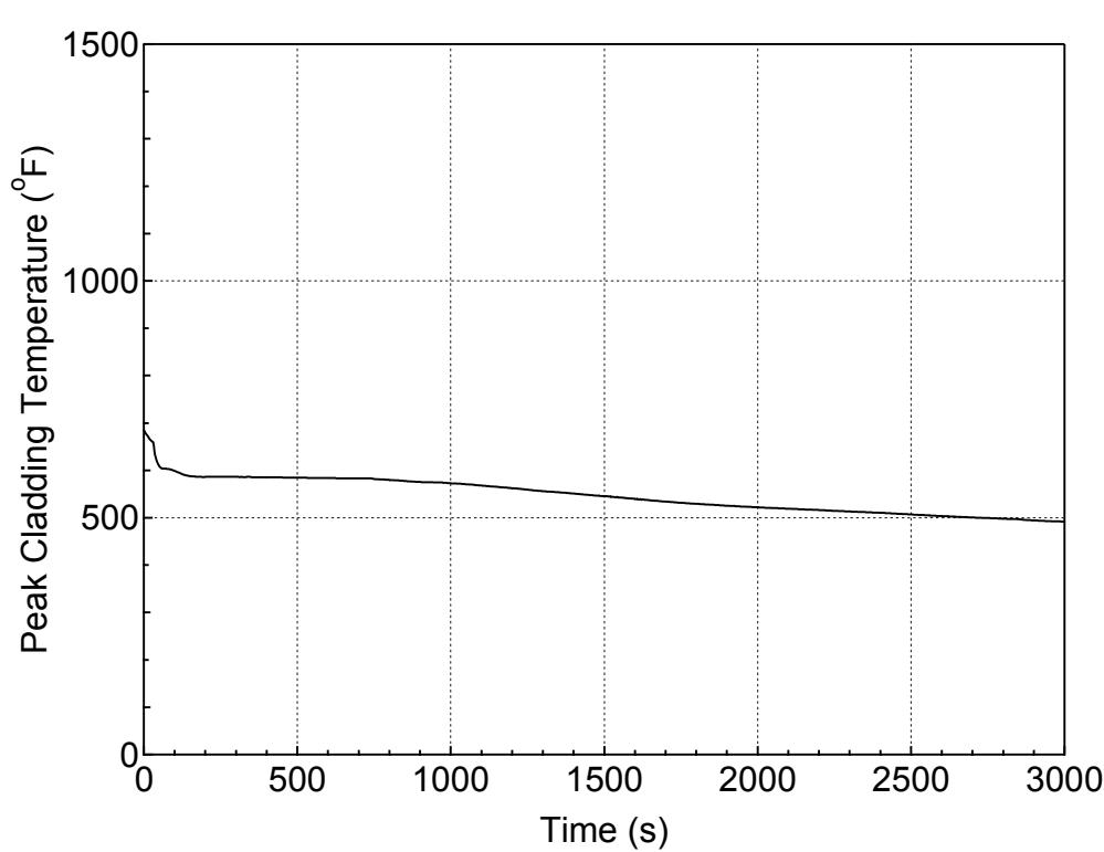
**Figure 5.1.2-8 PCT at All Elevations for Hot Rod in Hot Assembly for DVI-line Break
