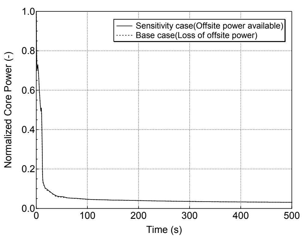
**Figure 5.6.2-15 Normalized Core Power for 1-ft<sup>2</sup> Break (Top)
