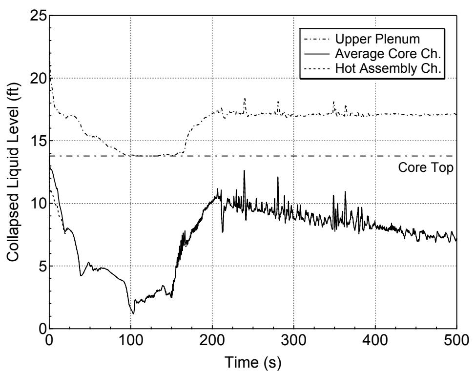
**Figure 5.1.1.a-16 Core and Upper Plenum Collapsed Levels for 1-ft<sup>2</sup> Break (Bottom)
