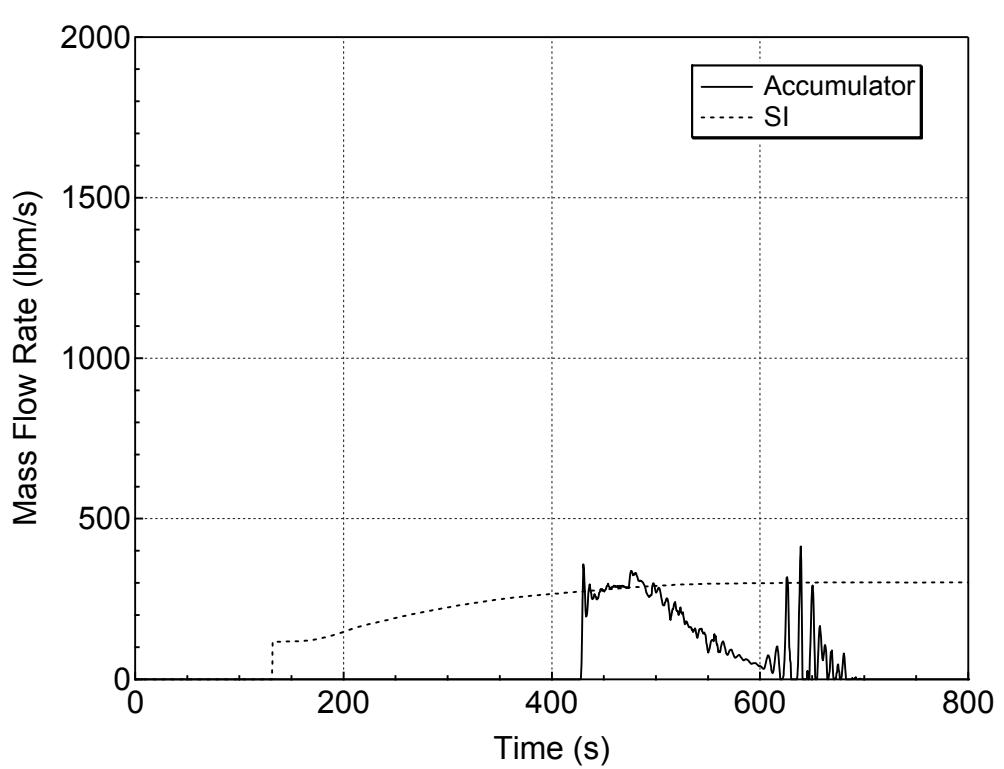
**Figure 5.3.1.b-22 Accumulator and Safety Injection Mass Flowrates
