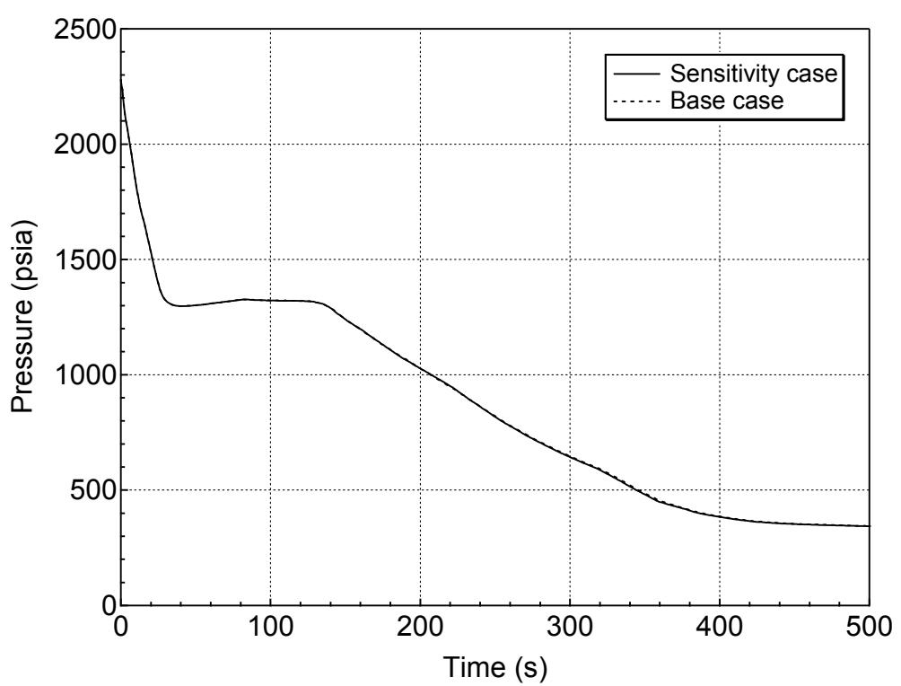
**Figure 5.5.a-1 RCS (Pressurizer) Pressure Transient for 7.5-inch Break (Top)
