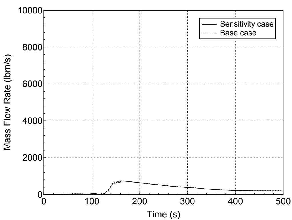
**Figure 5.4.3-4 Vapor Discharge through the Break for 7.5-inch Break (Top)
