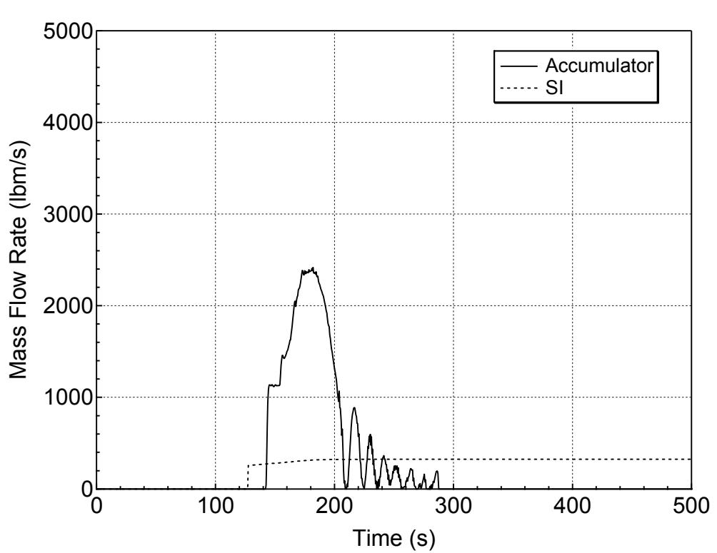
**Figure 5.2.k-4 Accumulator and Safety Injection Mass Flowrates
