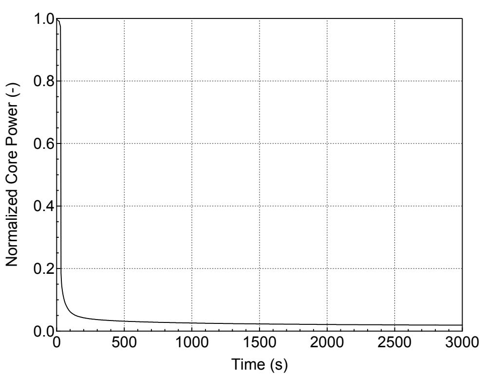
**Figure 5.1.2-2 Normalized Core Power for DVI-line Break
