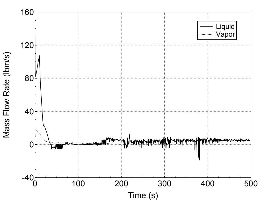
**Figure 5.3.2.c-9 Hot Assembly Exit Vapor and Liquid Mass Flowrates
