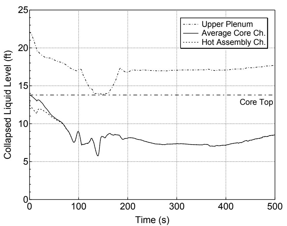
**Figure 5.2.g-7 Core and Upper Plenum Collapsed Levels for 7-inch Break (Bottom)
