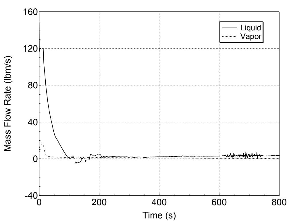
**Figure 5.3.1.b-36 Hot Assembly Exit Vapor and Liquid Mass Flowrates for 6.5-inch Break (Homogeneous) (Break Orientation Sensitivity Study)**
