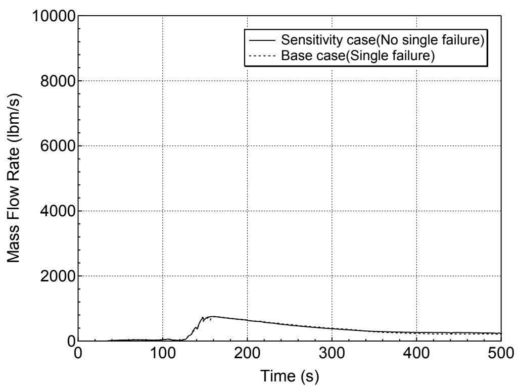
**Figure 5.6.1-4 Vapor Discharge through the Break for 7.5-inch Break (Top)
