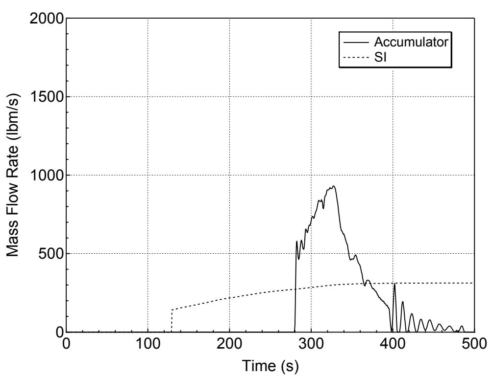
**Figure 5.3.1.e-13 Accumulator and Safety Injection Mass Flowrates
