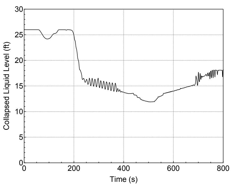
**Figure 5.3.1.a-6 Downcomer Collapsed Level for 6-inch Break (Top)
