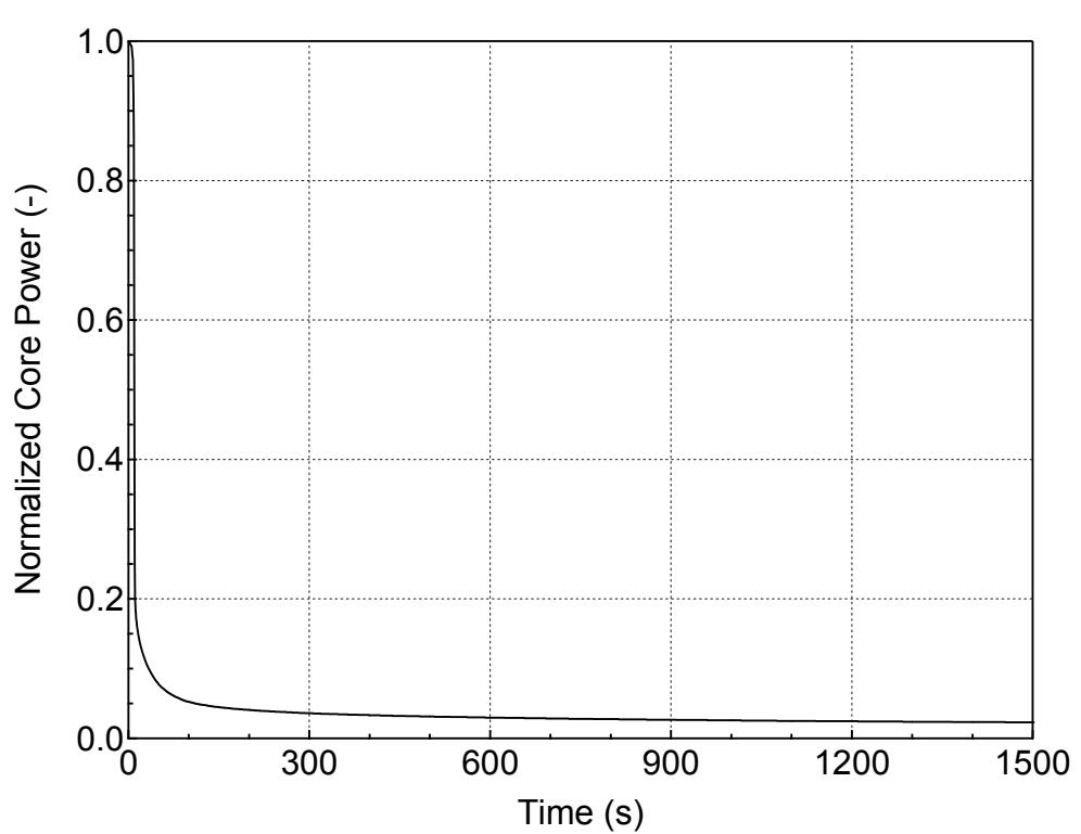
**Figure 5.1.3-2 Normalized Core Power for Pressurizer Steam Phase Break
