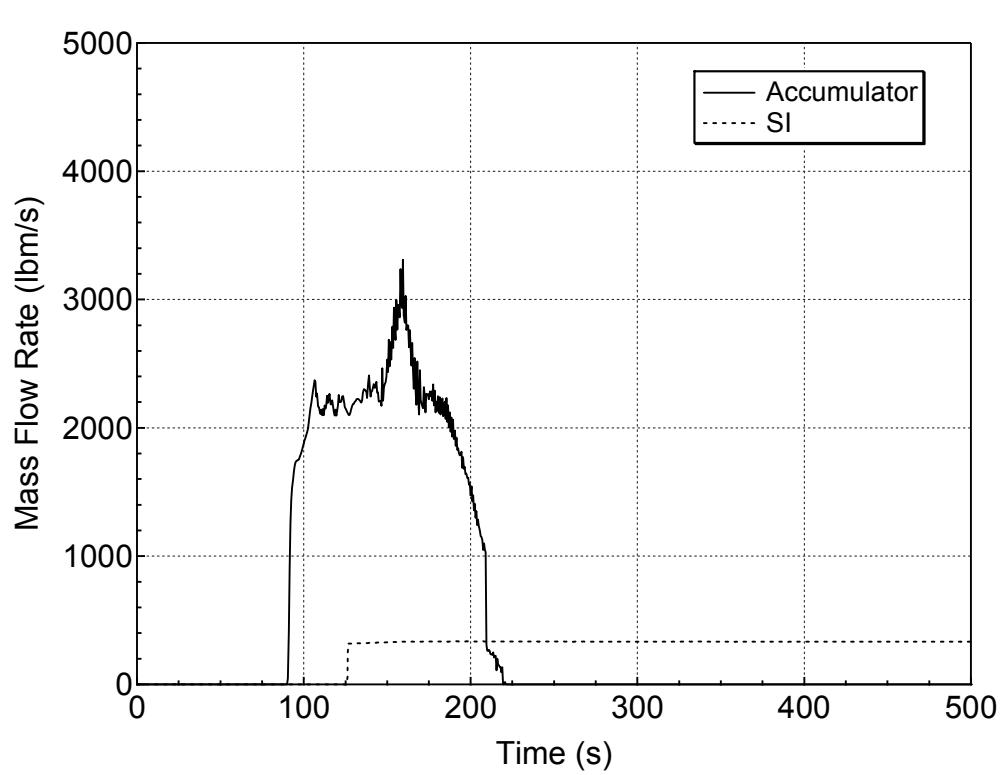
**Figure 5.3.2.c-13 Accumulator and Safety Injection Mass Flowrates
