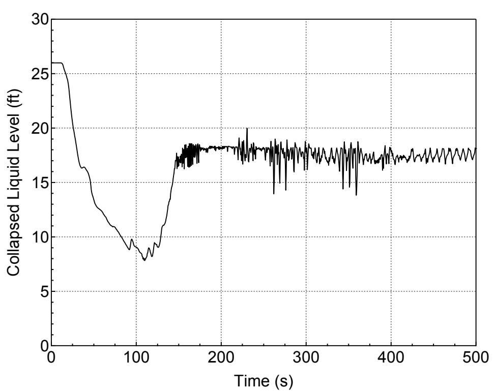
**Figure 5.3.2.c-15 Downcomer Collapsed Level for 1-ft<sup>2</sup> Break (Side)
