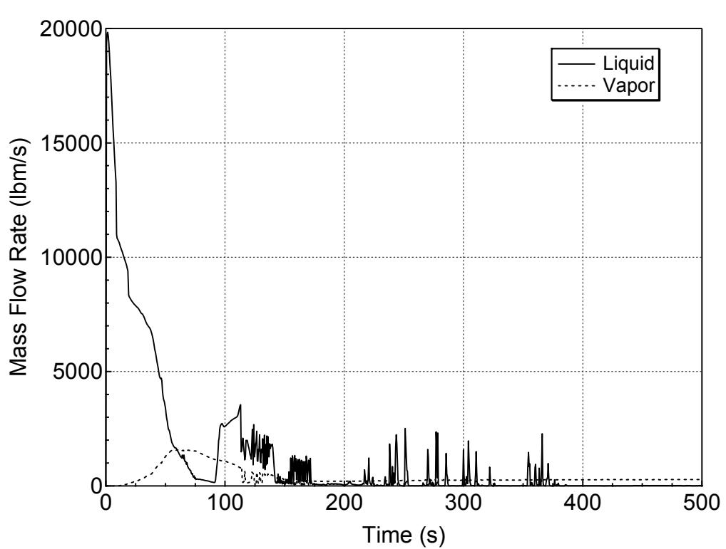
**Figure 5.3.2.c-21 Liquid and Vapor Discharges through the Break
