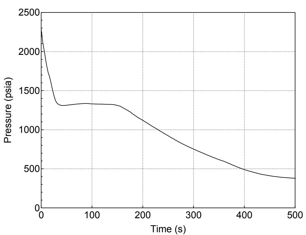
**Figure 5.2.g-1 RCS (Pressurizer) Pressure Transient for 7-inch Break (Bottom)
