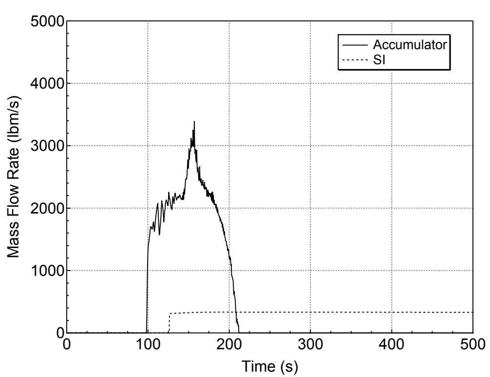
**Figure 5.3.2.b-4 Accumulator and Safety Injection Mass Flowrates
