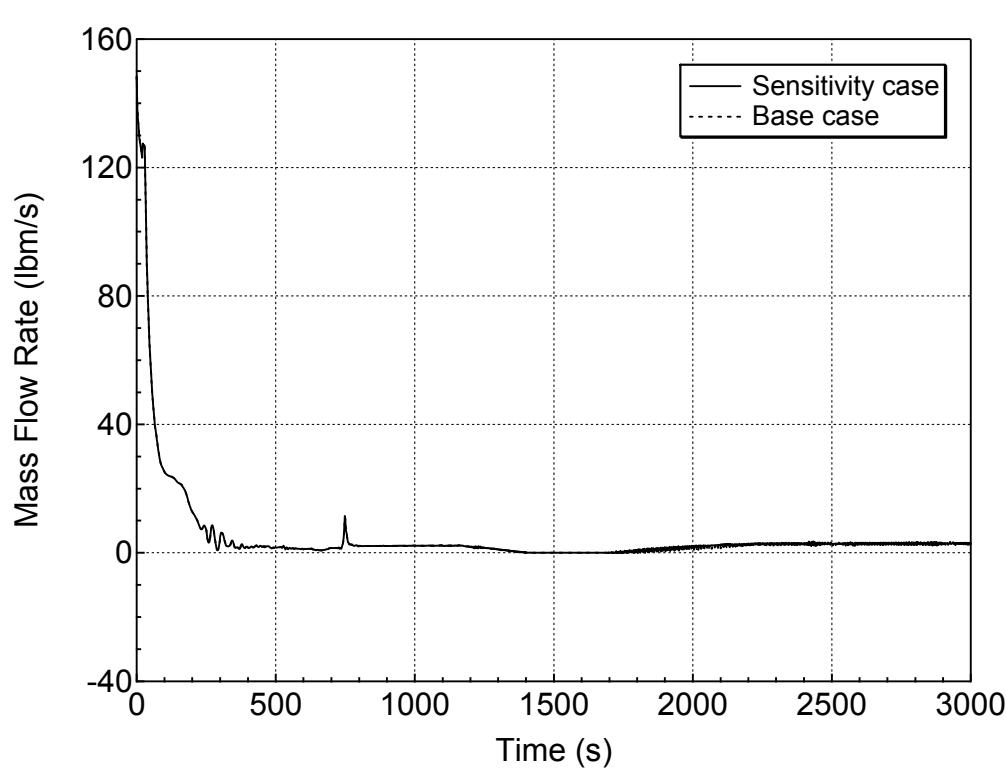
**Figure 5.5.c-12 Hot Assembly Exit Liquid Mass Flowrate for DVI-line Break
