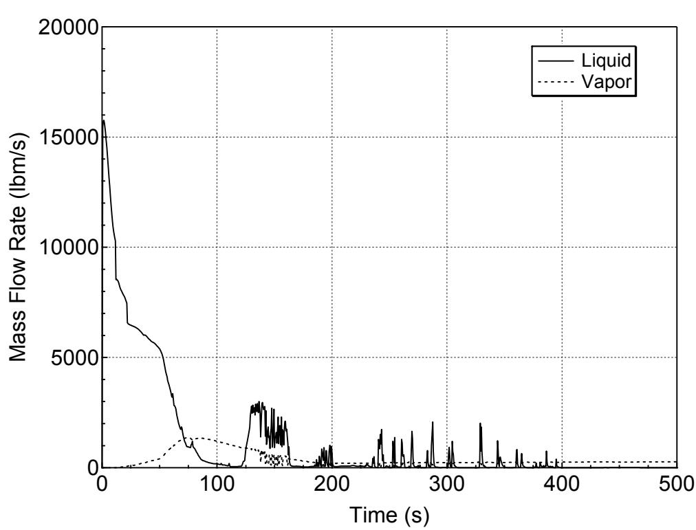
**Figure 5.3.2.a-12 Liquid and Vapor Discharges through the Break
