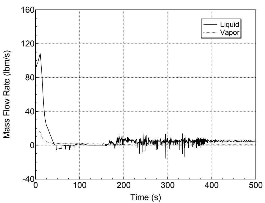
**Figure 5.3.2.a-27 Hot Assembly Exit Vapor and Liquid Mass Flowrates for 12-inch Break (Homogeneous) (Break Orientation Sensitivity Study)**
