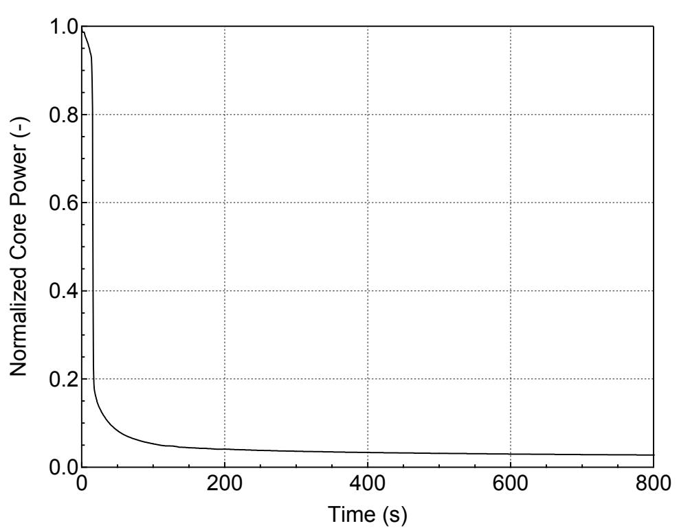
**Figure 5.3.1.a-2 Normalized Core Power for 6-inch Break (Top)
