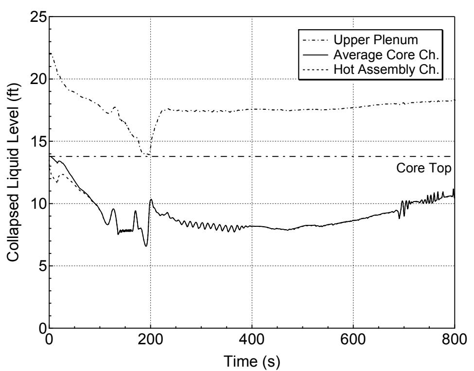
**Figure 5.3.1.a-7 Core and Upper Plenum Collapsed Levels for 6-inch Break (Top)
