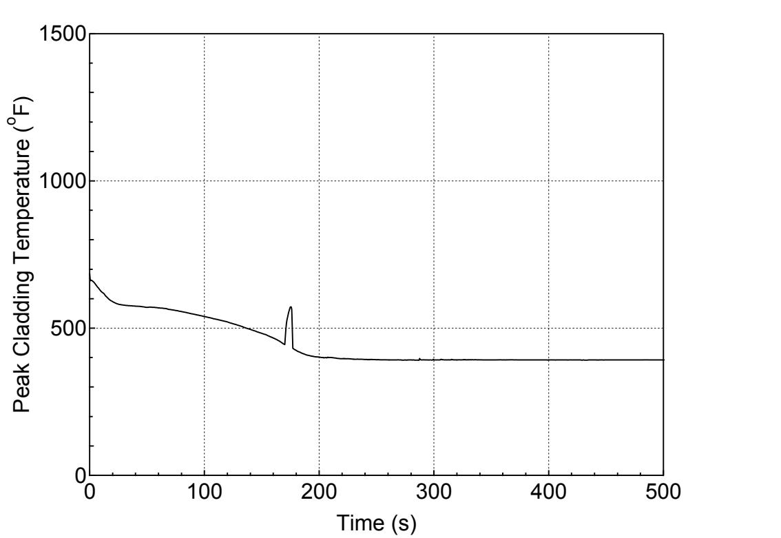
**Figure 5.2.k-8 PCT at All Elevations for Hot Rod in Hot Assembly
