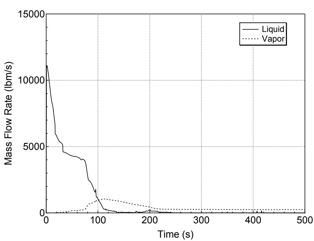
**Figure 5.2.j-3 Liquid and Vapor Discharges through the Break
