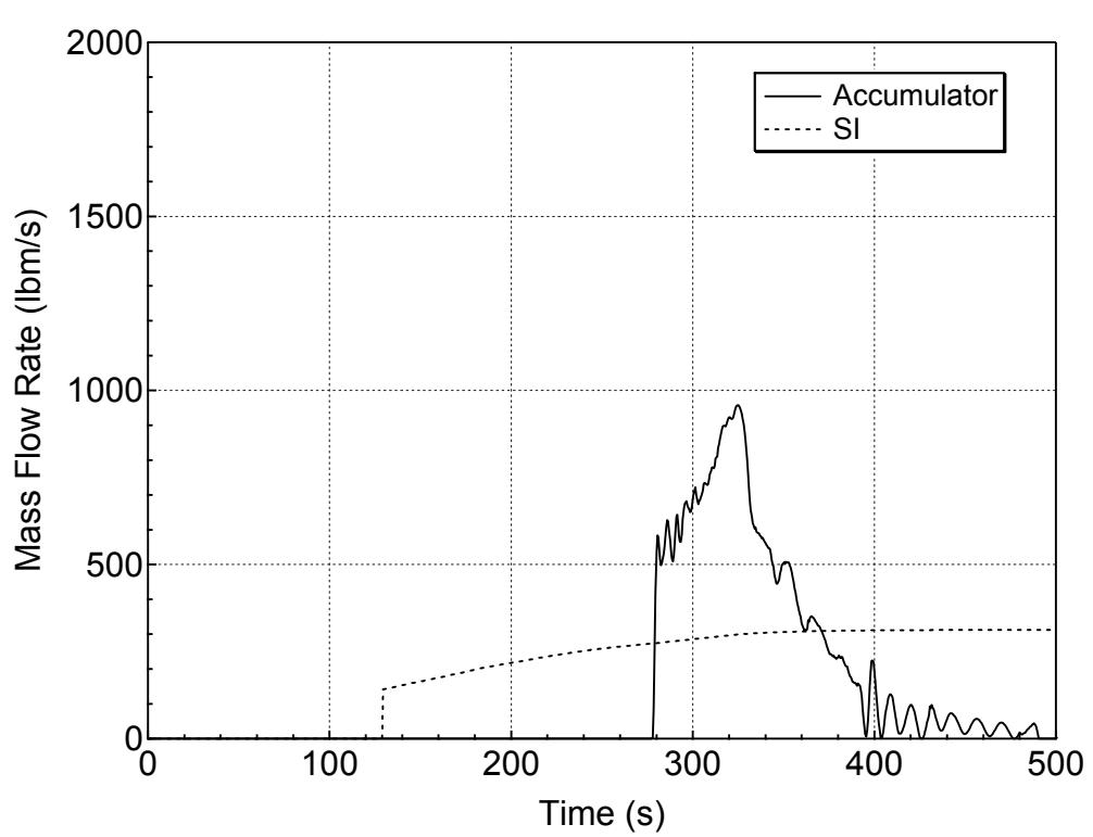
**Figure 5.3.1.e-4 Accumulator and Safety Injection Mass Flowrates
