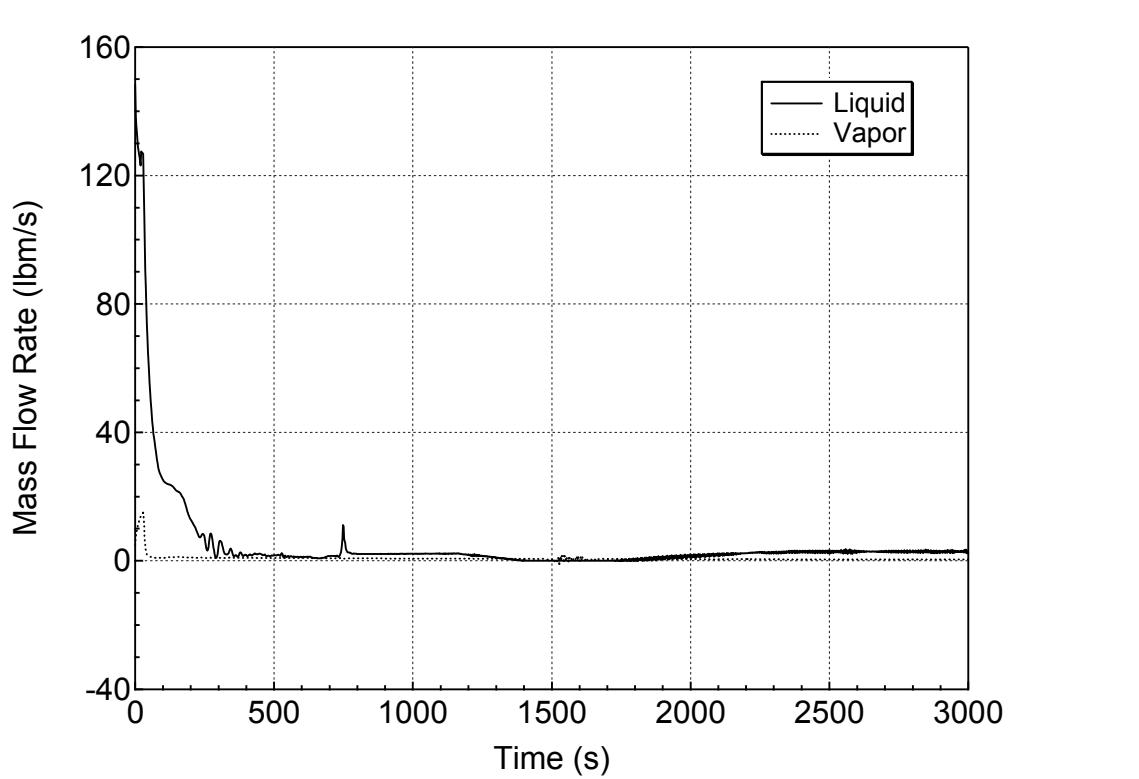
**Figure 5.1.2-9 Hot Assembly Exit Vapor and Liquid Mass Flowrates for DVI-line Break
