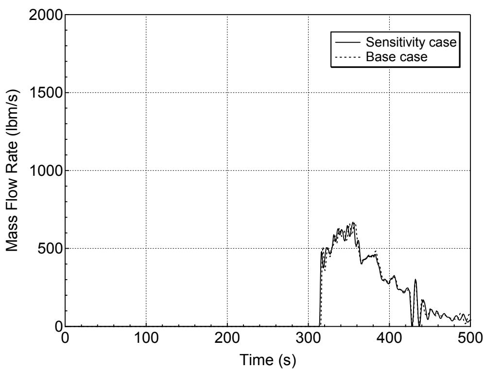
**Figure 5.4.1-5 Accumulator Injection Mass Flowrate for 7.5-inch Break (Top)
