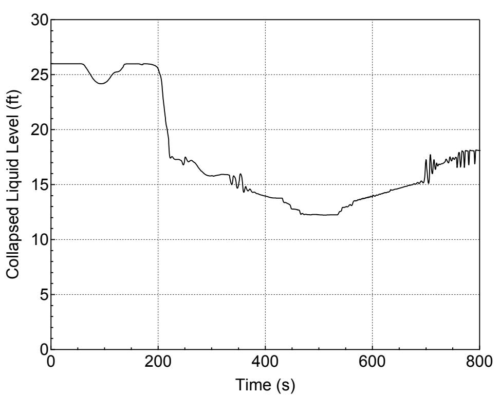
**Figure 5.3.1.a-15 Downcomer Collapsed Level for 6-inch Break (Side)
