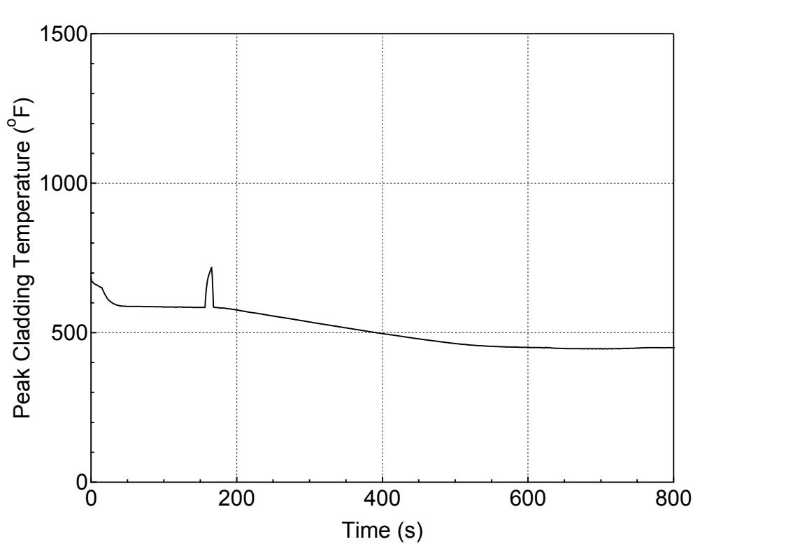
**Figure 5.3.1.b-8 PCT at All Elevations for Hot Rod in Hot Assembly
