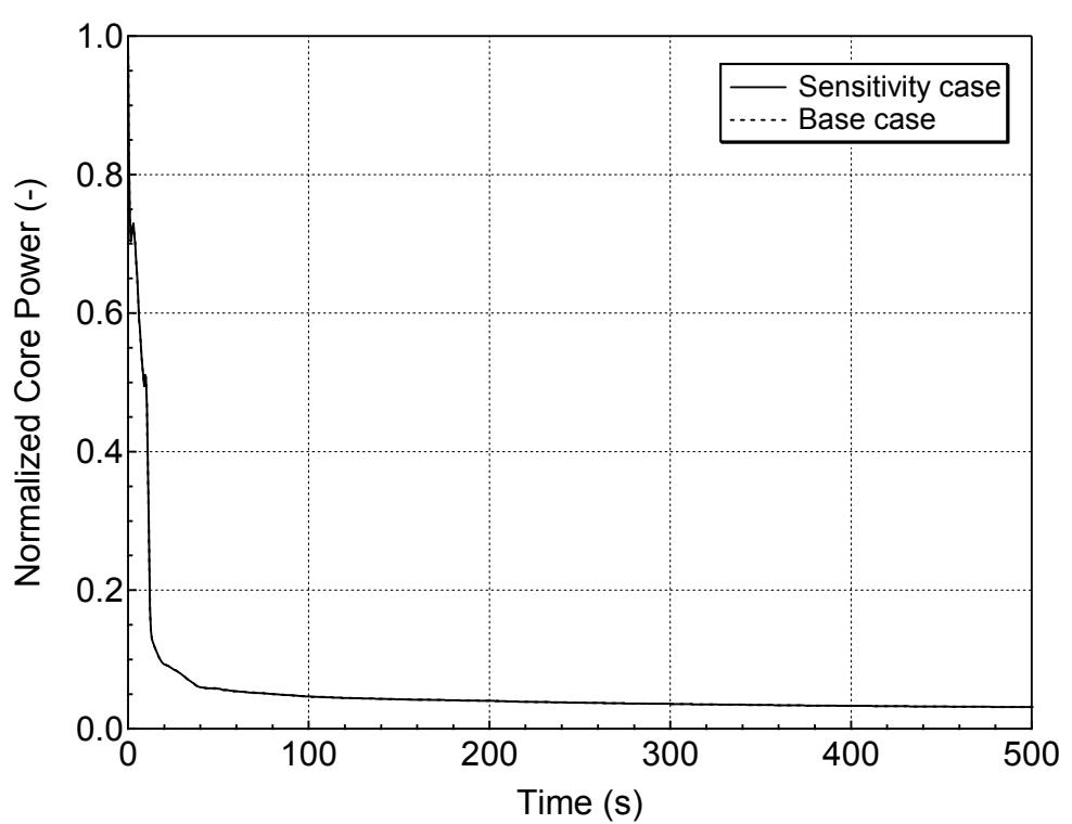
**Figure 5.4.1-15 Normalized Core Power for 1-ft<sup>2</sup> Break (Top)
