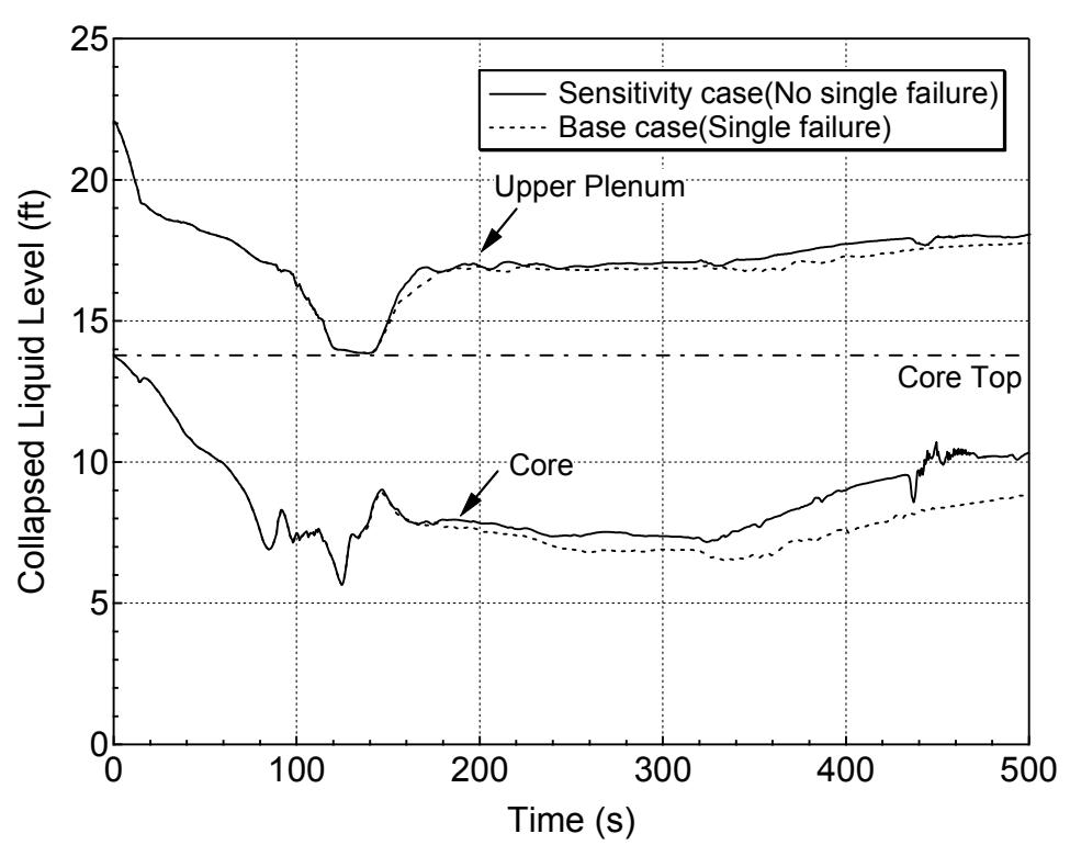
**Figure 5.6.1-9 Average Core and Upper Plenum Collapsed Levels
