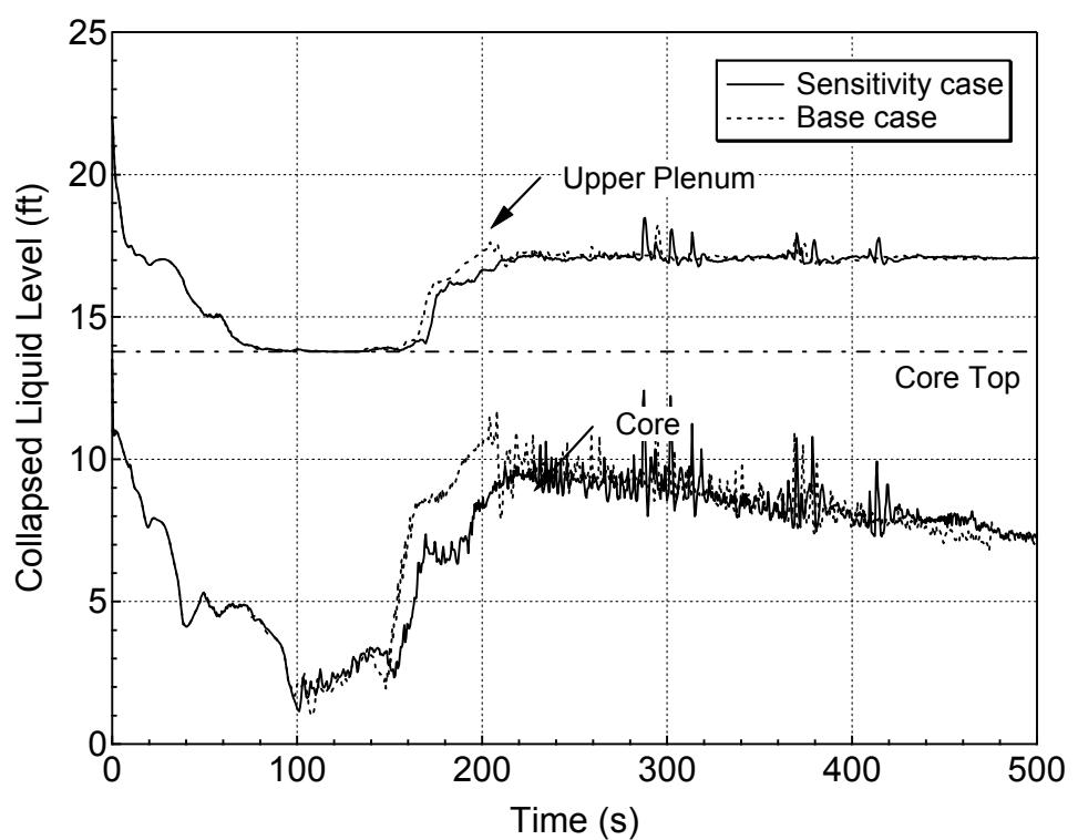
**Figure 5.4.3-23 Hot Assembly Core and Upper Plenum Collapsed Levels
