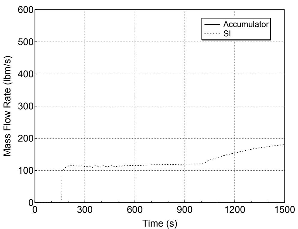
**Figure 5.2.c-4 Accumulator and Safety Injection Mass Flowrates
