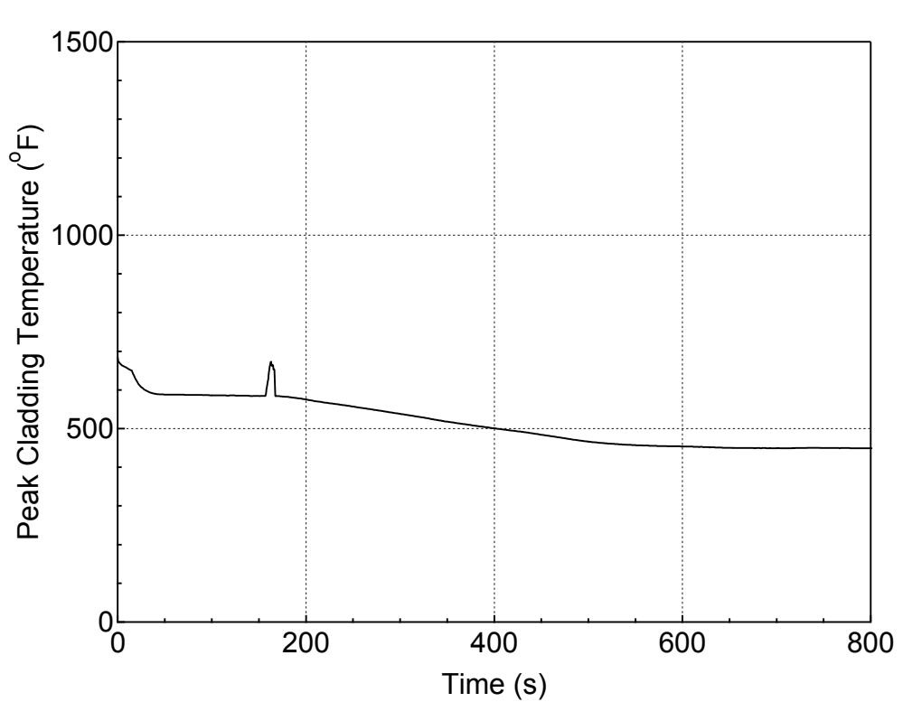
**Figure 5.3.1.b-17 PCT at All Elevations for Hot Rod in Hot Assembly
