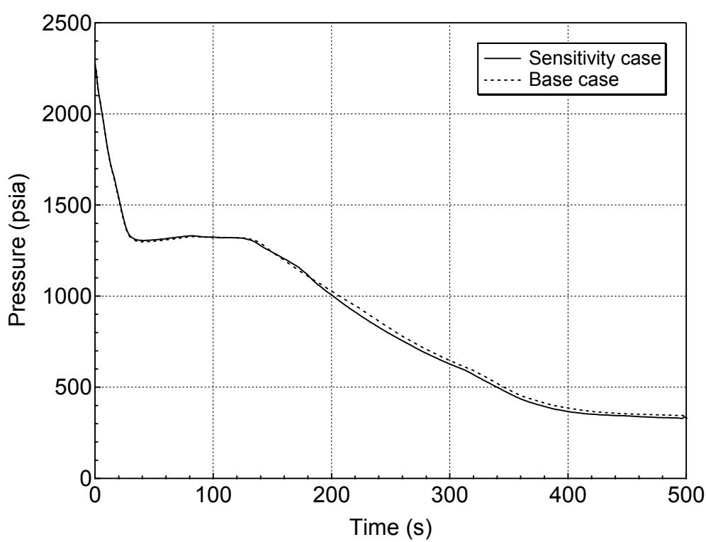
**Figure 5.4.2-1 RCS (Pressurizer) Pressure Transient for 7.5-inch Break (Top)
