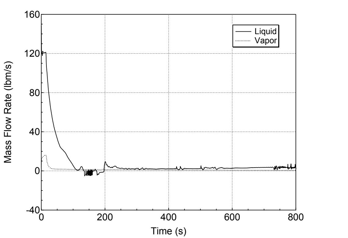
**Figure 5.2.f-9 Hot Assembly Exit Vapor and Liquid Mass Flowrates
