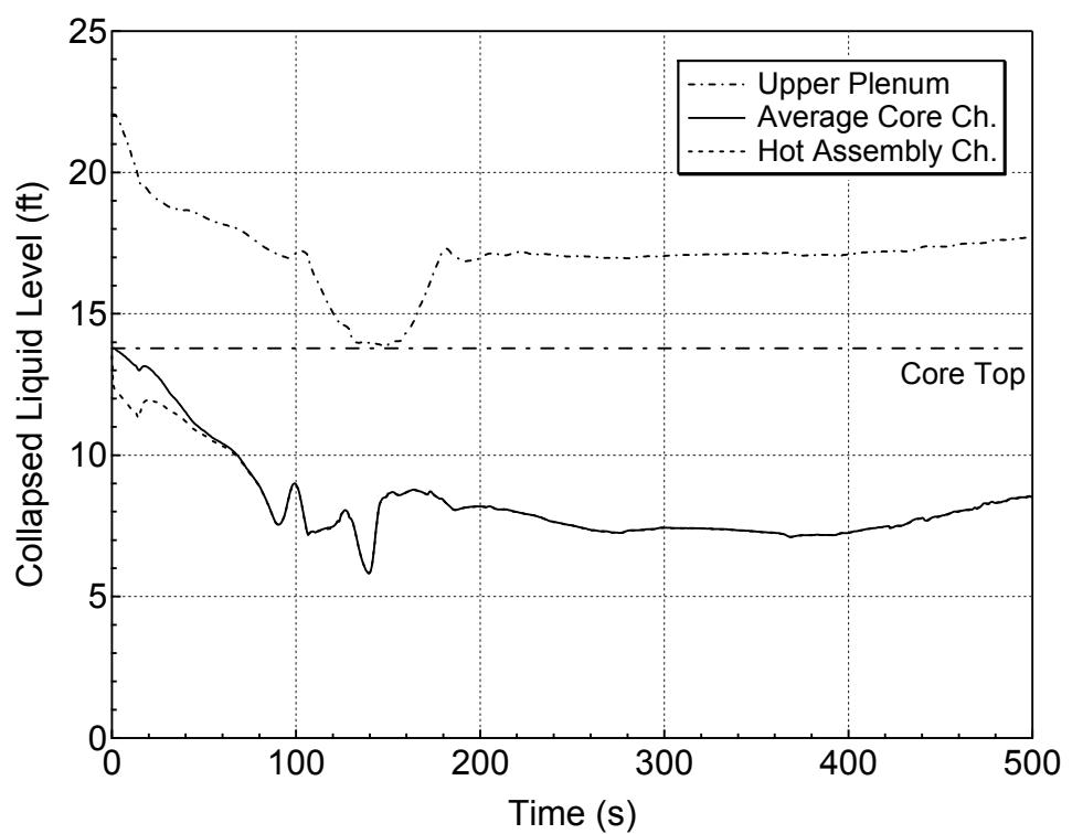
**Figure 5.3.1.c-25 Core and Upper Plenum Collapsed Levels
