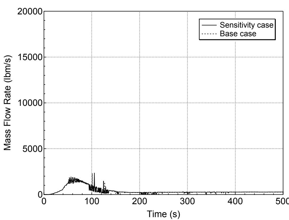
**Figure 5.4.1-17 Vapor Discharge through the Break for 1-ft<sup>2</sup> Break (Top)
