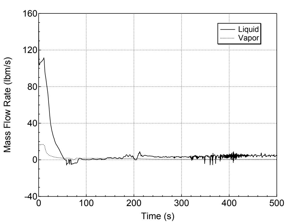
**Figure 5.2.j-9 Hot Assembly Exit Vapor and Liquid Mass Flowrates
