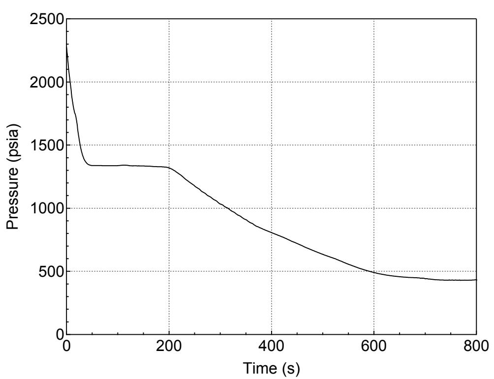
**Figure 5.3.1.a-1 RCS (Pressurizer) Pressure Transient for 6-inch Break (Top)
