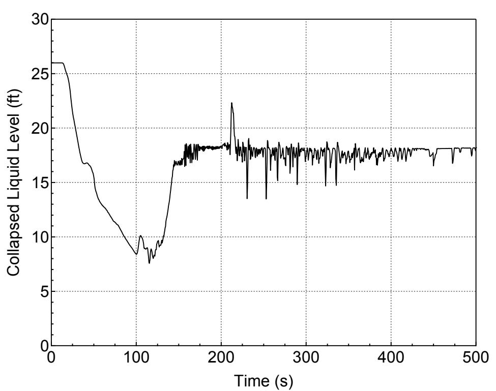
**Figure 5.2.m-6 Downcomer Collapsed Level for 13-inch Break (Bottom)
