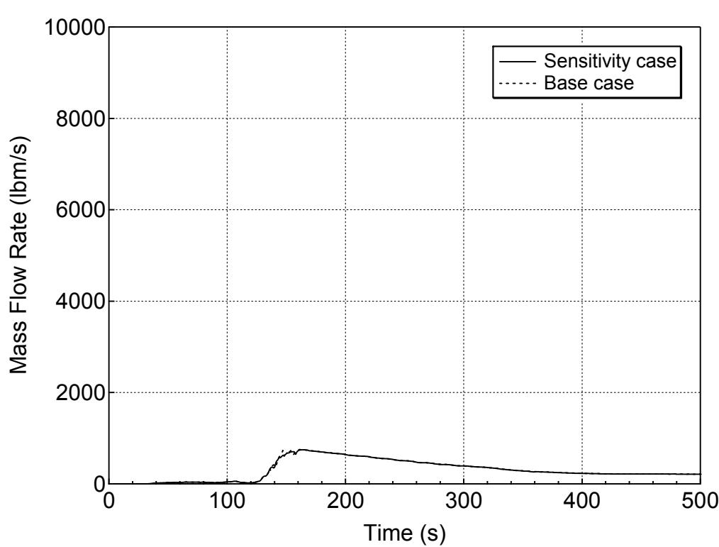
**Figure 5.5.a-4 Vapor Discharge through the Break for 7.5-inch Break (Top)
