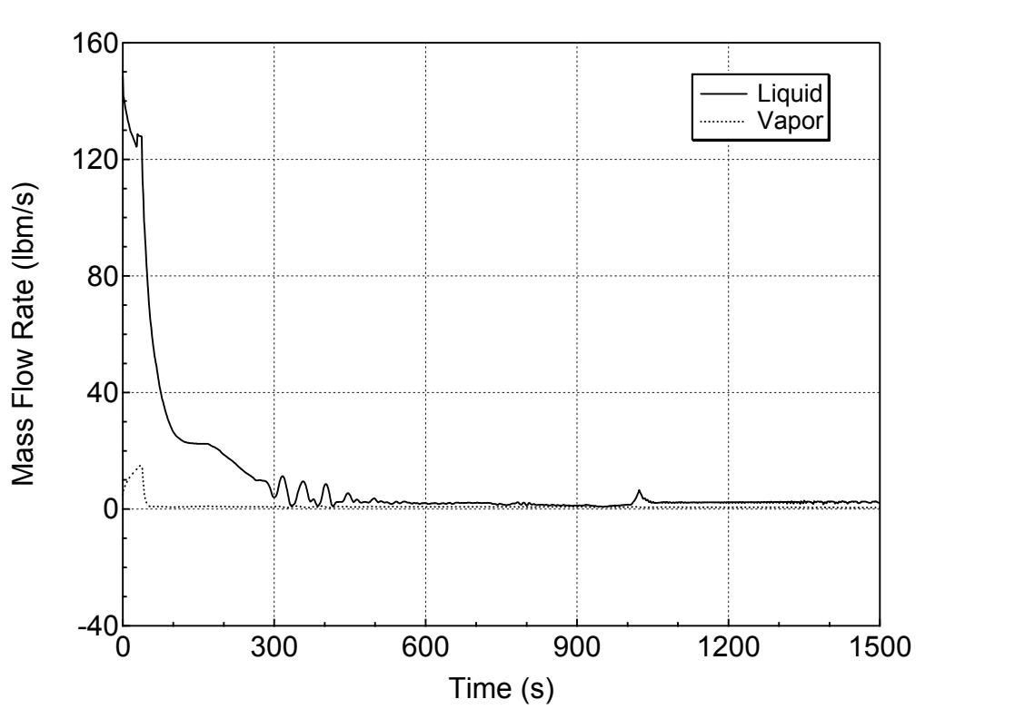
**Figure 5.2.c-9 Hot Assembly Exit Vapor and Liquid Mass Flowrates
