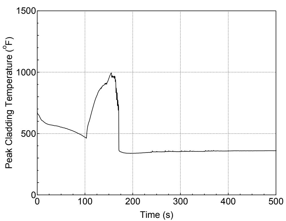
**Figure 5.3.2.c-26 PCT at All Elevations for Hot Rod in Hot Assembly
