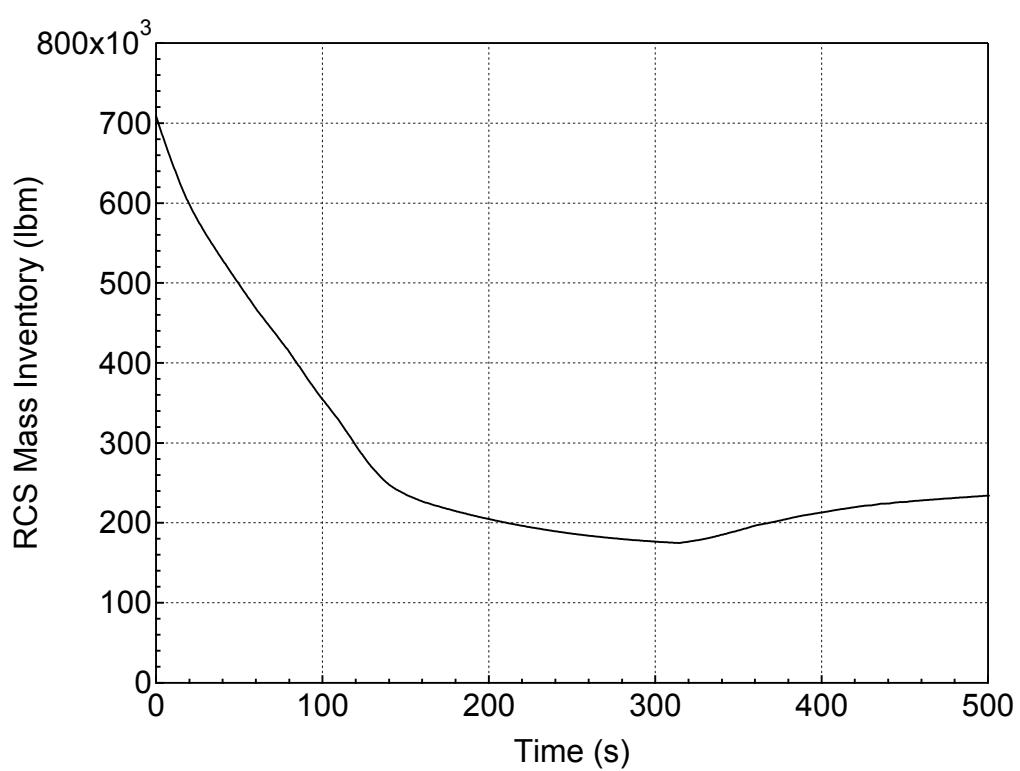
**Figure 5.3.1.d-32 RCS Mass Inventory for 7.5-inch Break (Homogeneous)
