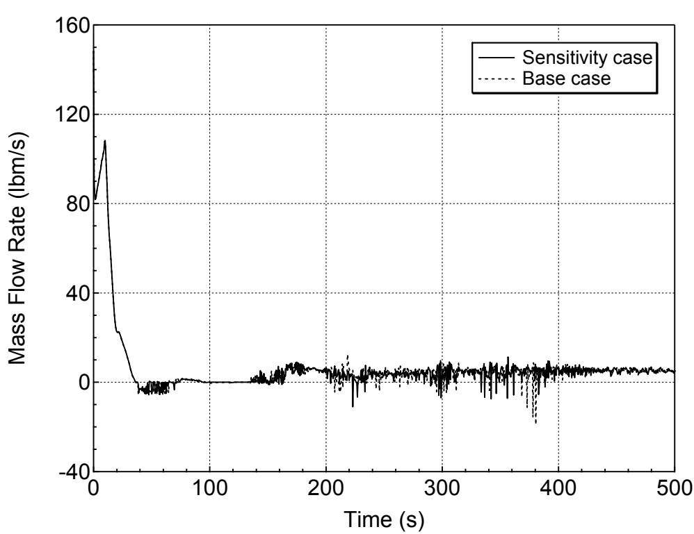
**Figure 5.4.1-25 Hot Assembly Exit Liquid Mass Flowrate for 1-ft<sup>2</sup> Break (Top)
