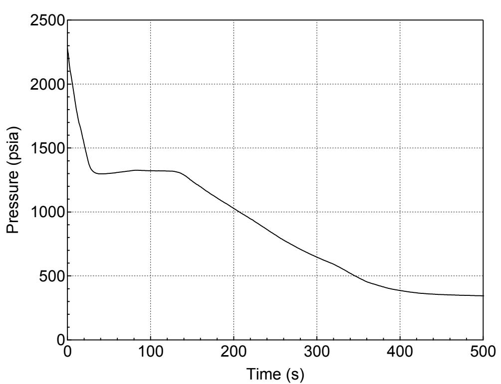
**Figure 5.3.1.d-10 RCS (Pressurizer) Pressure Transient for 7.5-inch Break (Top)
