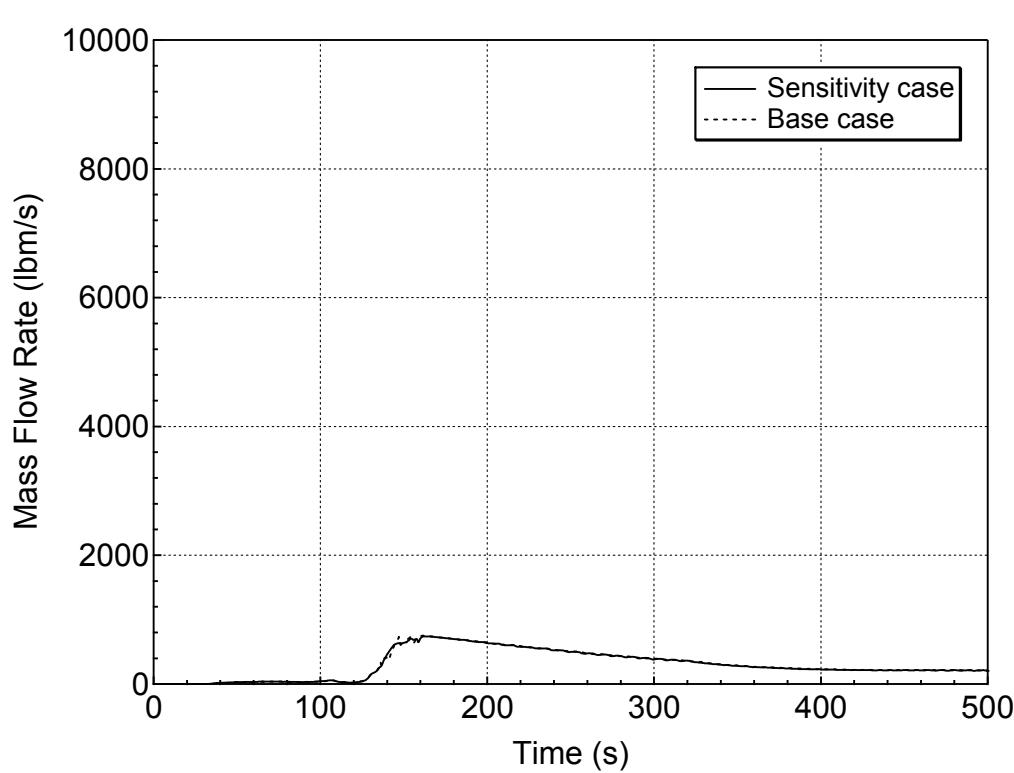
**Figure 5.4.1-4 Vapor Discharge through the Break for 7.5-inch Break (Top)
