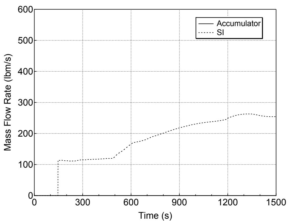
**Figure 5.2.d-4 Accumulator and Safety Injection Mass Flowrates
