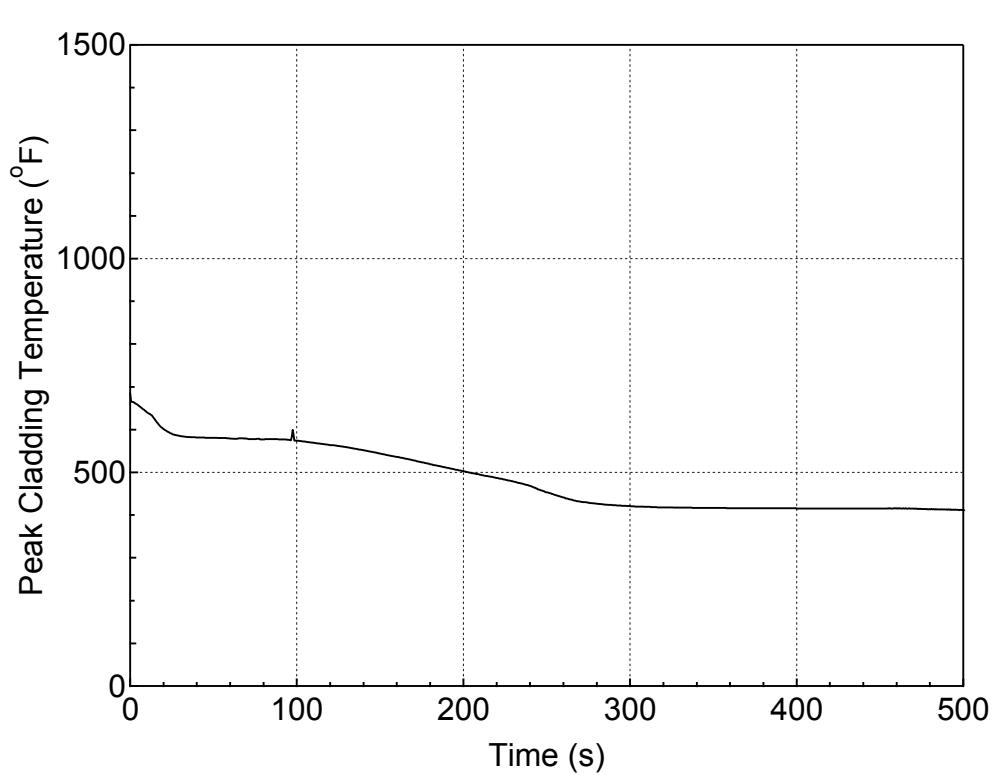
**Figure 5.2.i-8 PCT at All Elevations for Hot Rod in Hot Assembly
