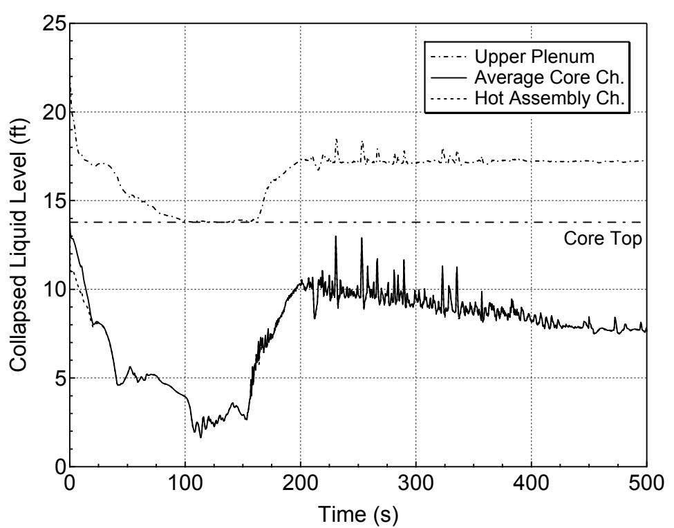
**Figure 5.2.m-7 Core and Upper Plenum Collapsed Levels for 13-inch Break (Bottom)
