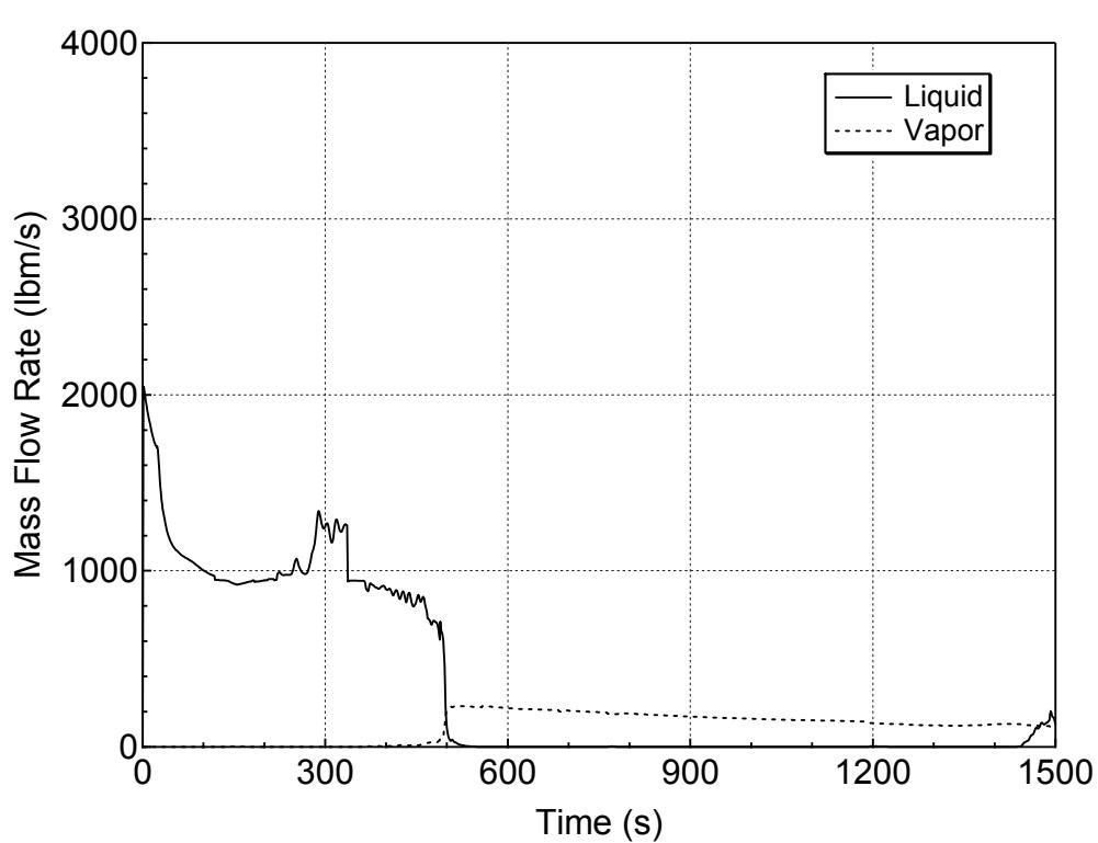
**Figure 5.2.d-3 Liquid and Vapor Discharges through the Break
