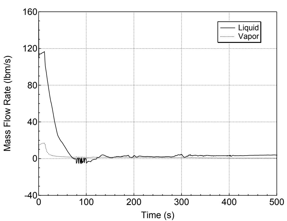
**Figure 5.3.1.e-18 Hot Assembly Exit Vapor and Liquid Mass Flowrates
