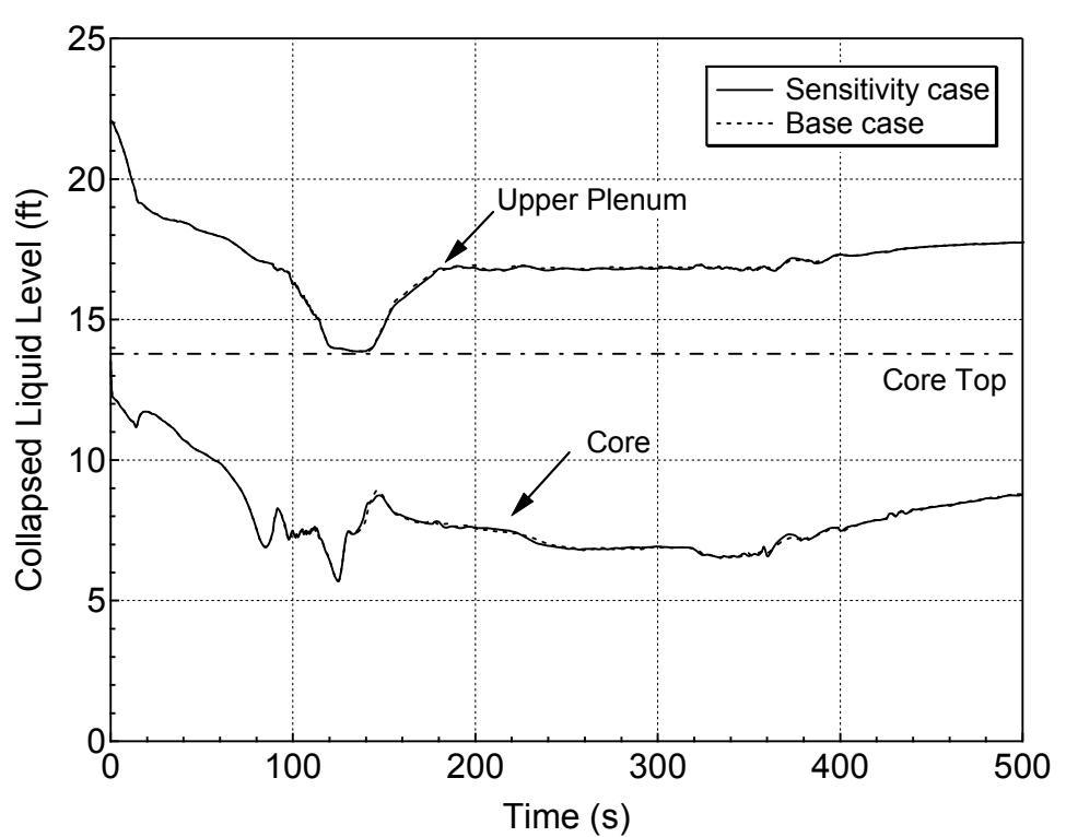
**Figure 5.5.a-10 Hot Assembly Core and Upper Plenum Collapsed Levels
