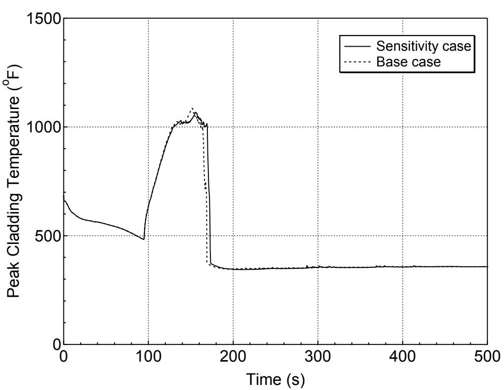
**Figure 5.4.3-24 PCT at All Elevations for Hot Rod in Hot Assembly for 1-ft<sup>2</sup> Break (Top)
