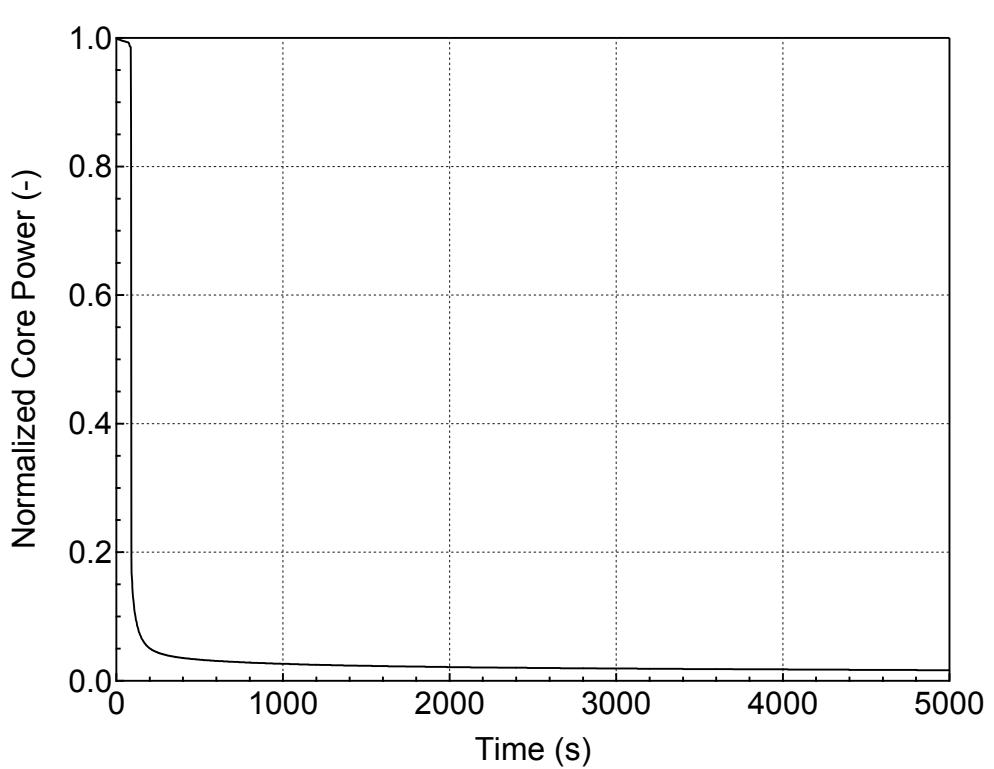
**Figure 5.1.1.c-2 Normalized Core Power for 2-inch Break (Bottom)
