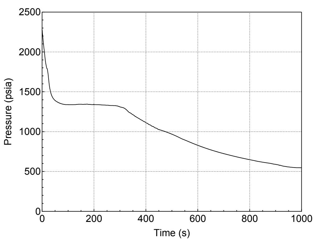
**Figure 5.2.e-1 RCS (Pressurizer) Pressure Transient for 5-inch Break (Bottom)
