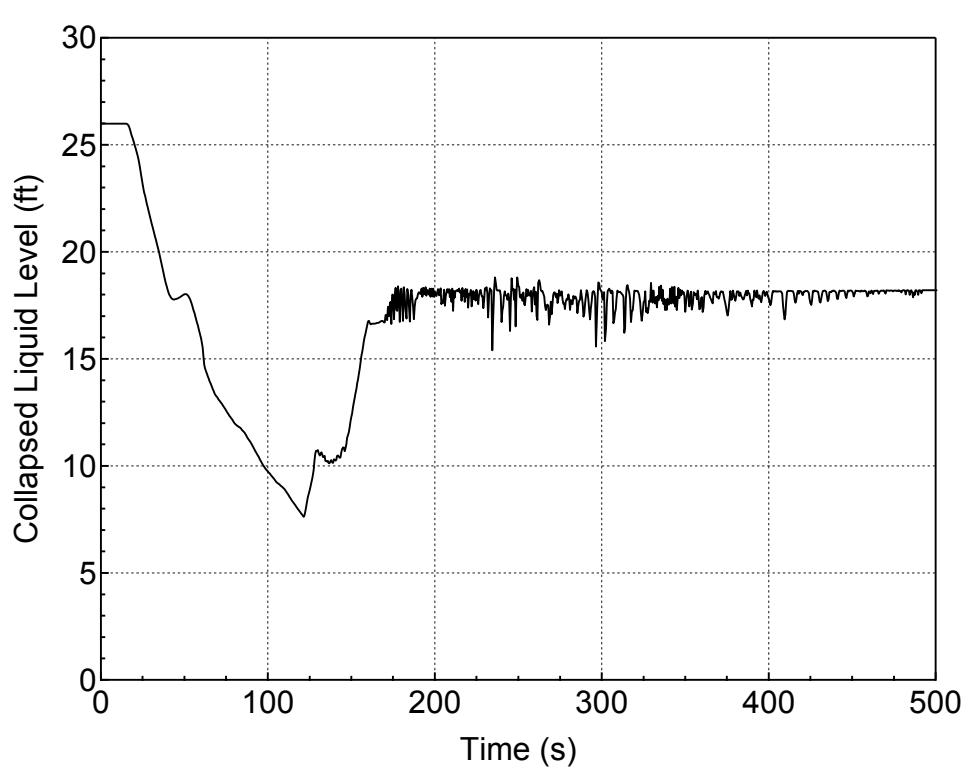
**Figure 5.2.I-6 Downcomer Collapsed Level for 12-inch Break (Bottom)
