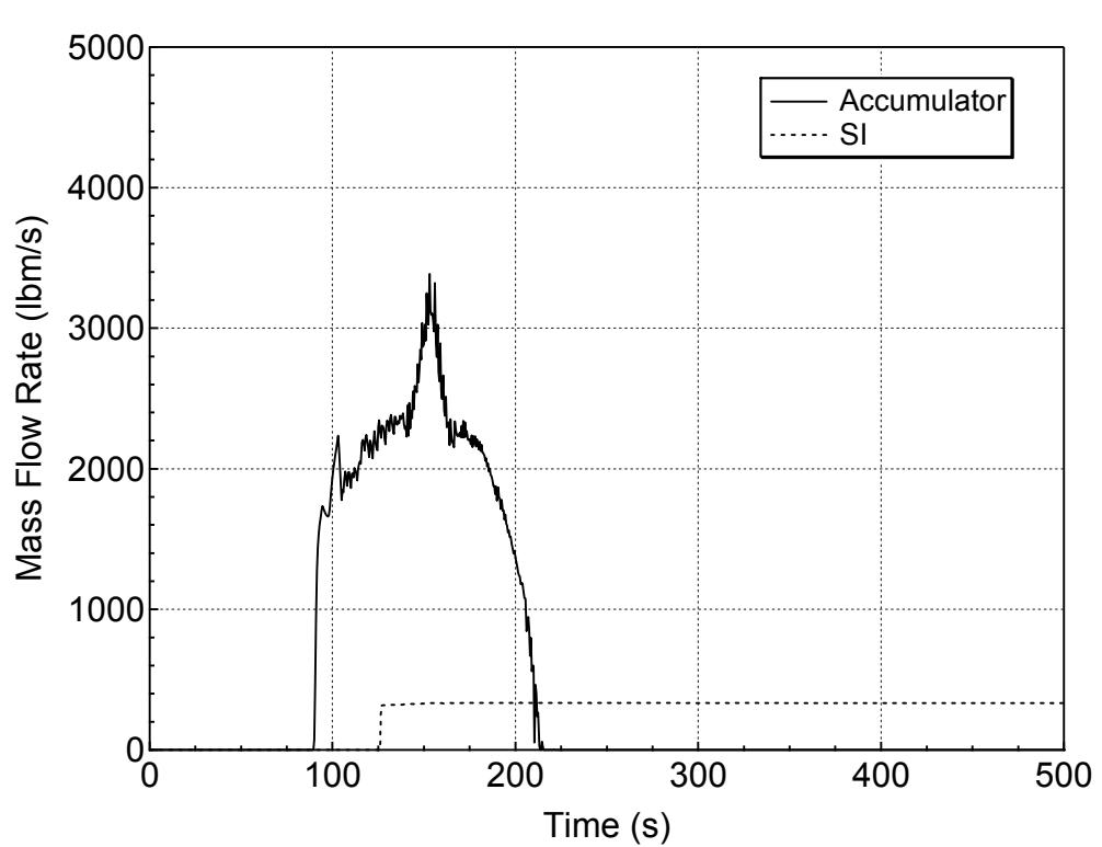
**Figure 5.2.n-4 Accumulator and Safety Injection Mass Flowrates
