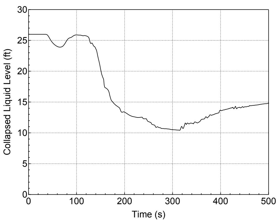
**Figure 5.3.1.d-6 Downcomer Collapsed Level for 7.5-inch Break (Bottom)
