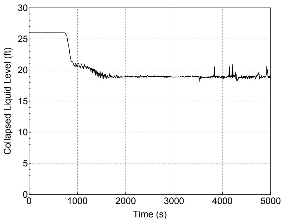
**Figure 5.1.1.a-6 Downcomer Collapsed Level for 2-inch Break (Bottom)
