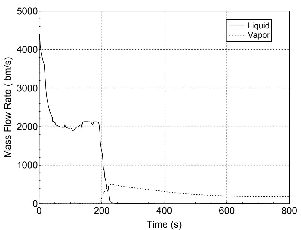
**Figure 5.2.f-3 Liquid and Vapor Discharges through the Break
