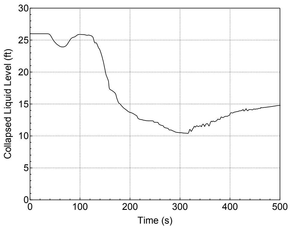
**Figure 5.3.1.d-33 Downcomer Collapsed Level for 7.5-inch Break (Homogeneous)
