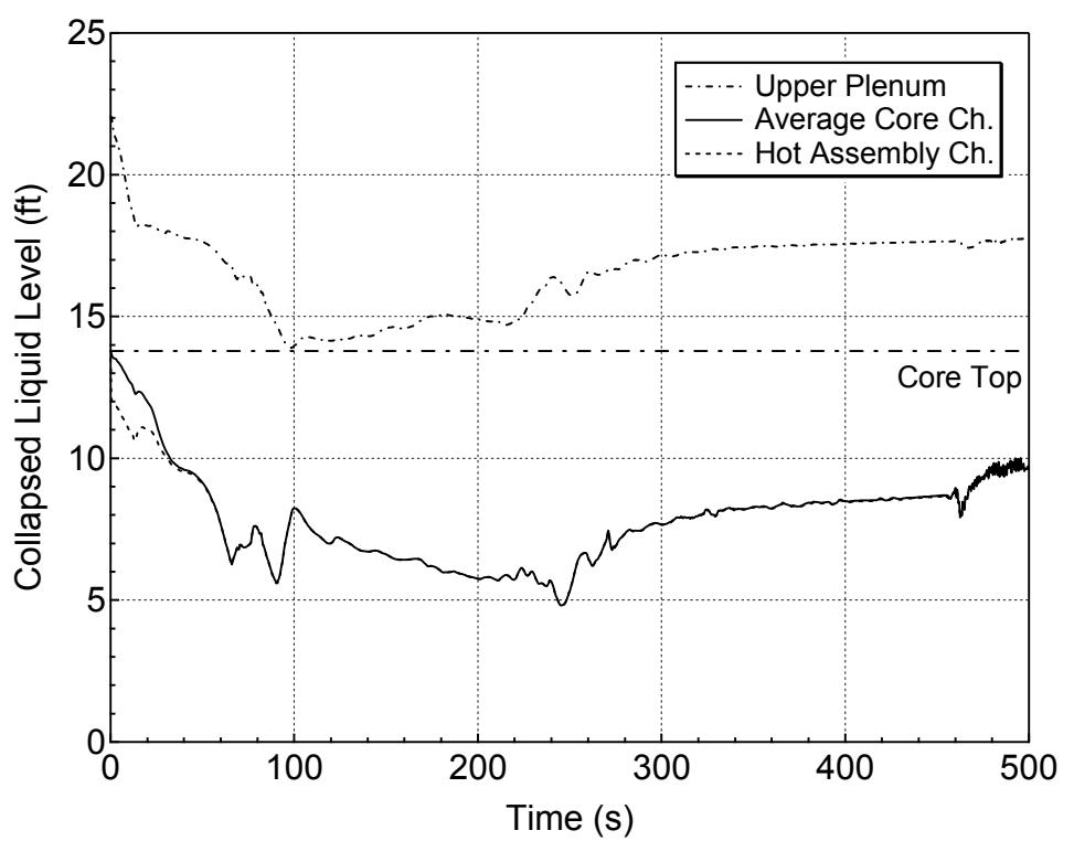
**Figure 5.2.i-7 Core and Upper Plenum Collapsed Levels for 9-inch Break (Bottom)
