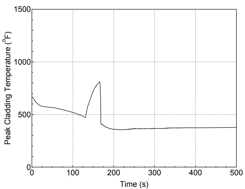
**Figure 5.3.2.a-26 PCT at All Elevations for Hot Rod in Hot Assembly
