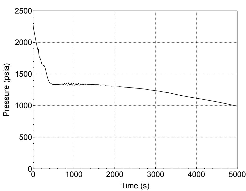
**Figure 5.1.1.b-1 RCS (Pressurizer) Pressure Transient for 2-inch Break (Bottom)
