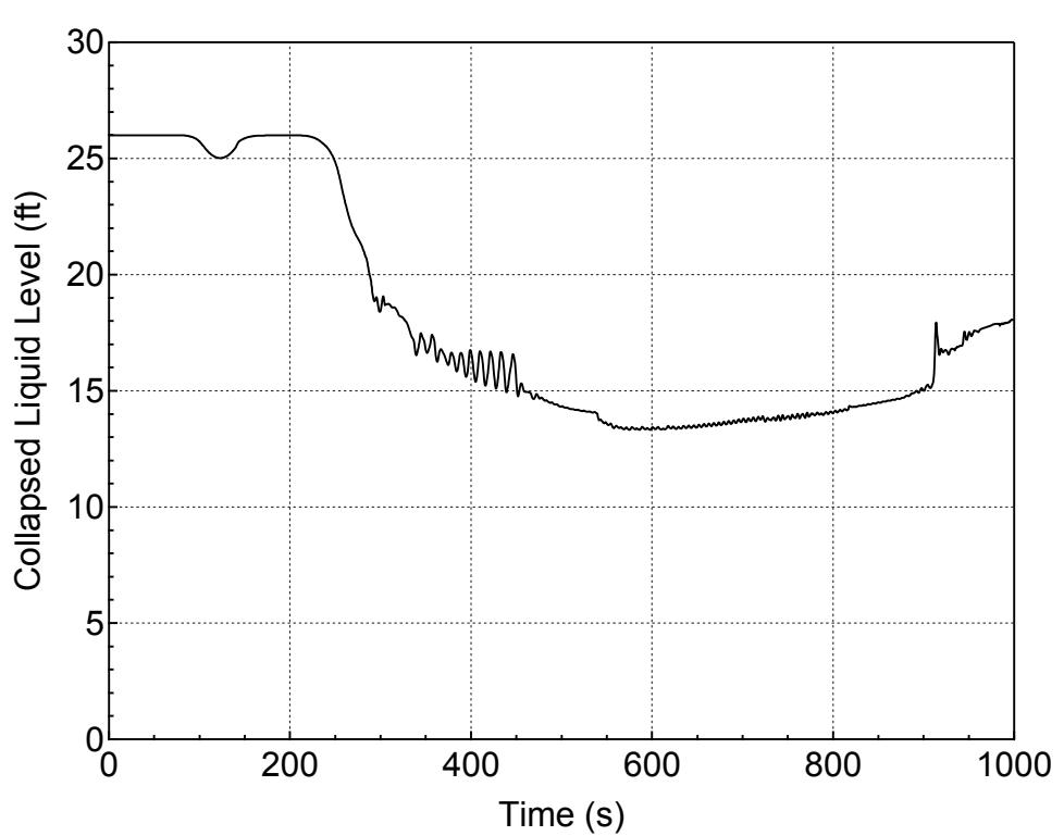
**Figure 5.2.e-6 Downcomer Collapsed Level for 5-inch Break (Bottom)
