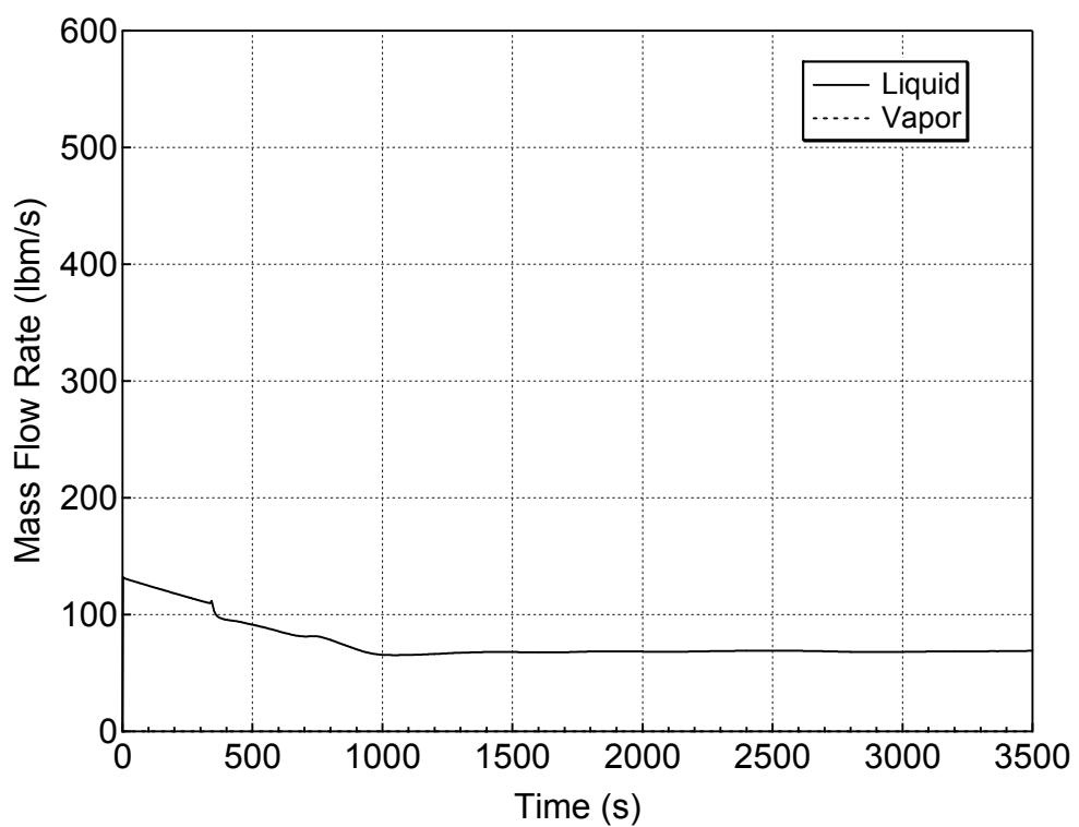
**Figure 5.2.a-3 Liquid and Vapor Discharges through the Break
