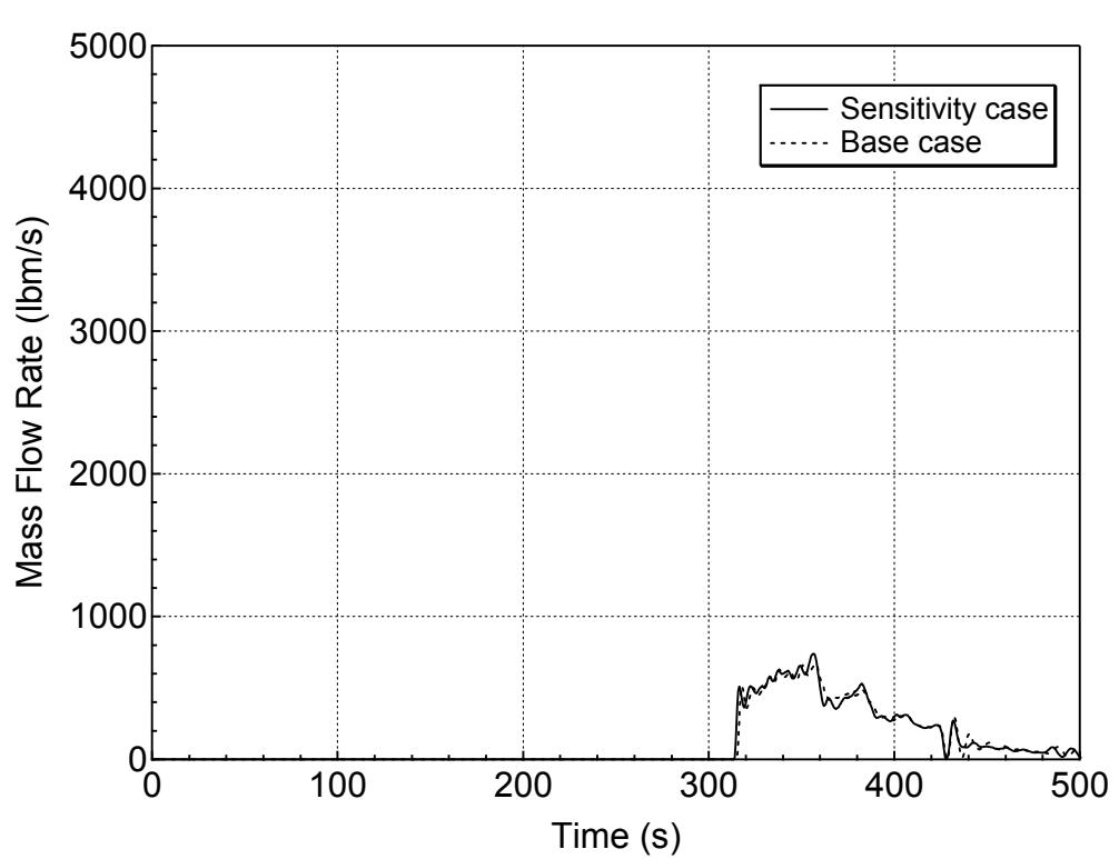
**Figure 5.5.a-5 Accumulator Injection Mass Flowrate for 7.5-inch Break (Top)
