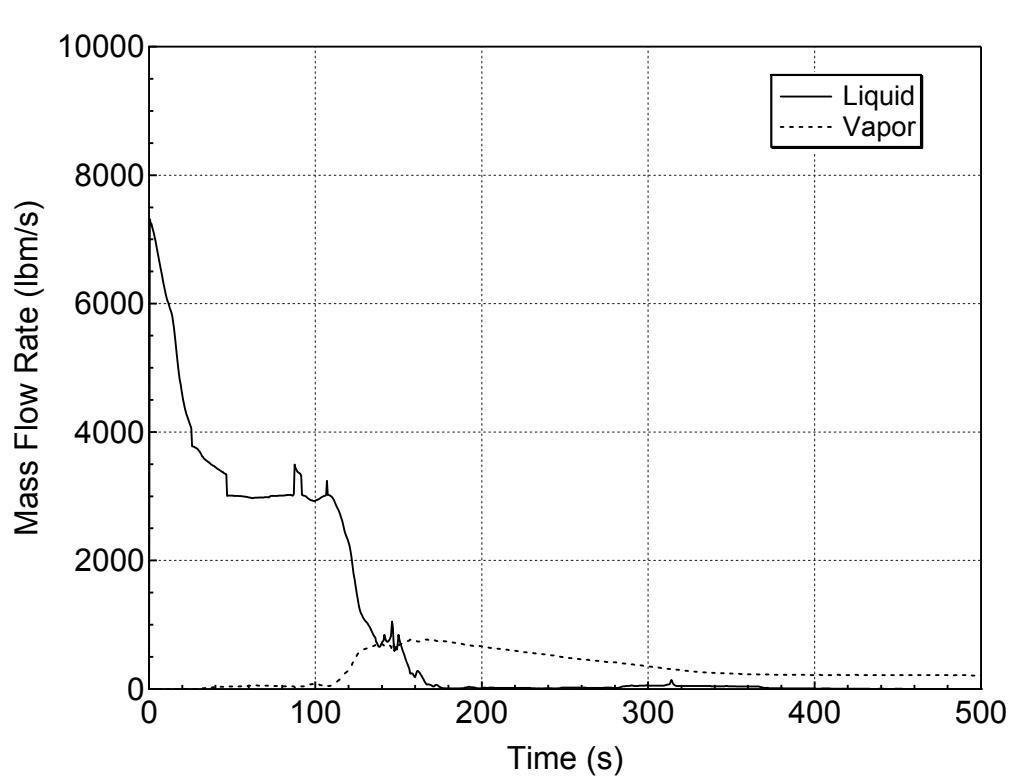
**Figure 5.3.1.e-12 Liquid and Vapor Discharges through the Break
