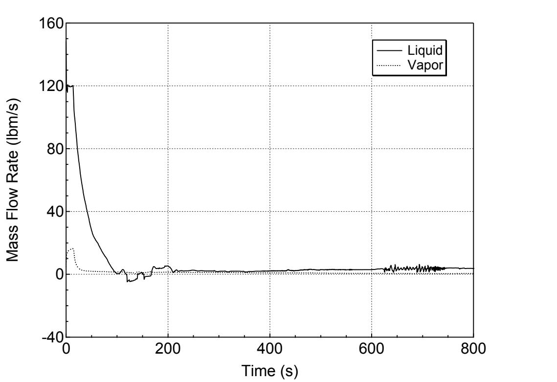
**Figure 5.3.1.b-27 Hot Assembly Exit Vapor and Liquid Mass Flowrates
