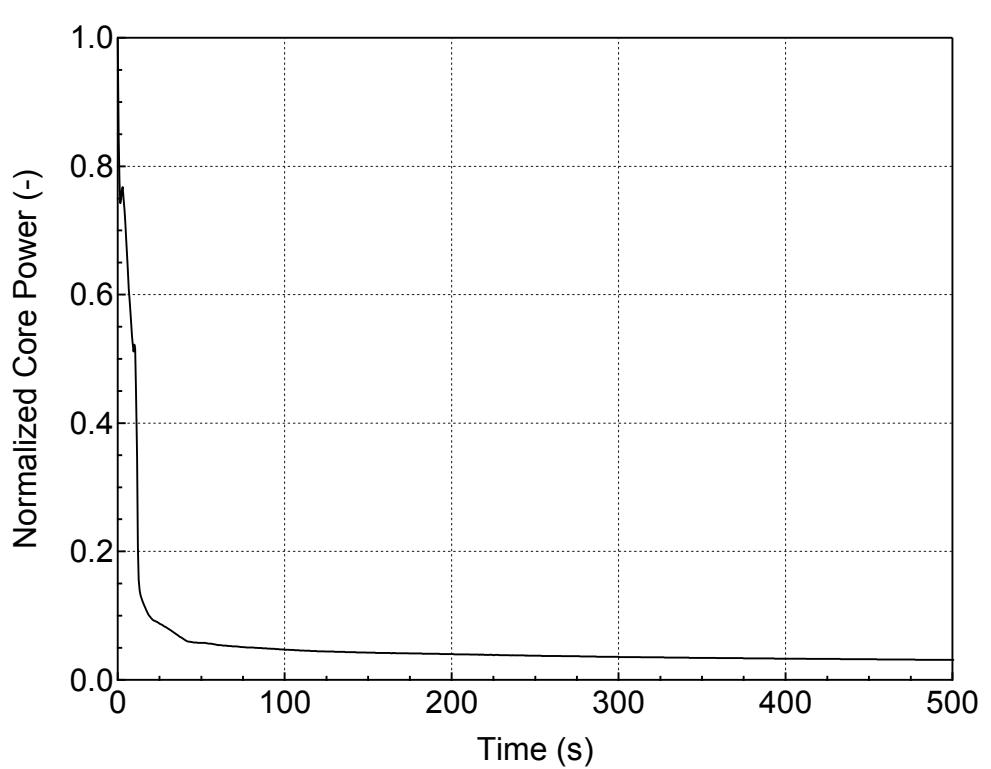
**Figure 5.3.2.b-20 Normalized Core Power for 13-inch Break (Homogeneous)
