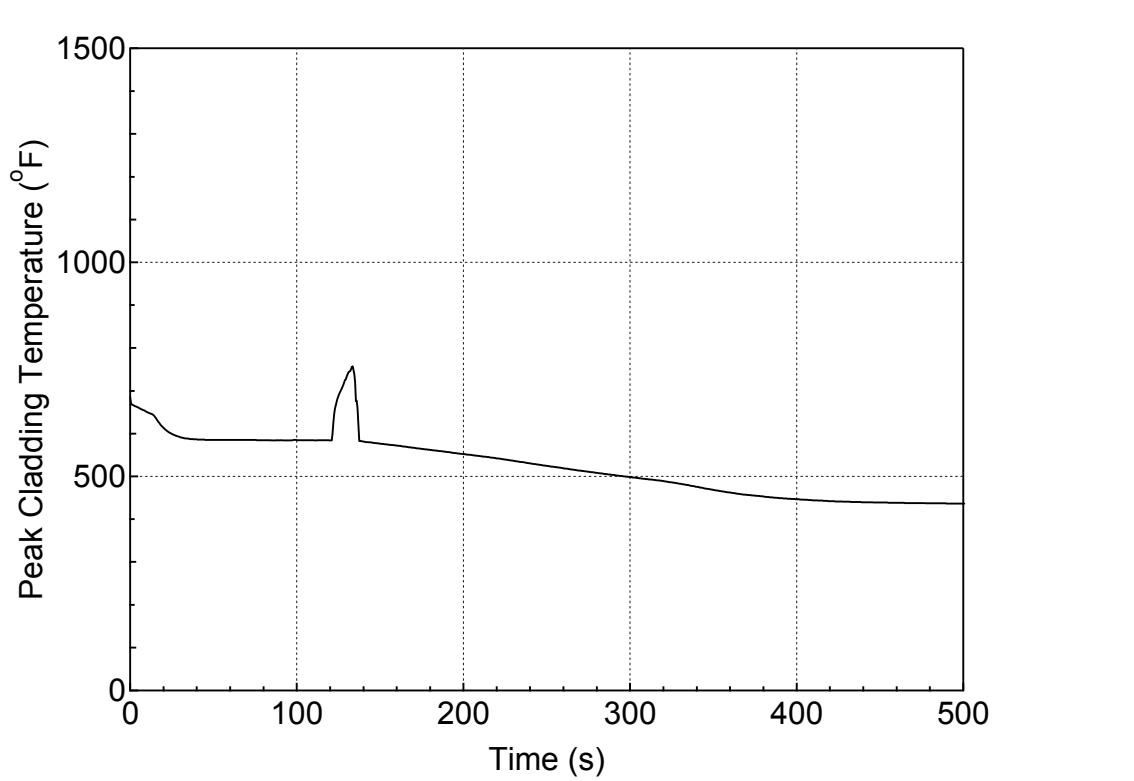
**Figure 5.3.1.d-8 PCT at All Elevations for Hot Rod in Hot Assembly
