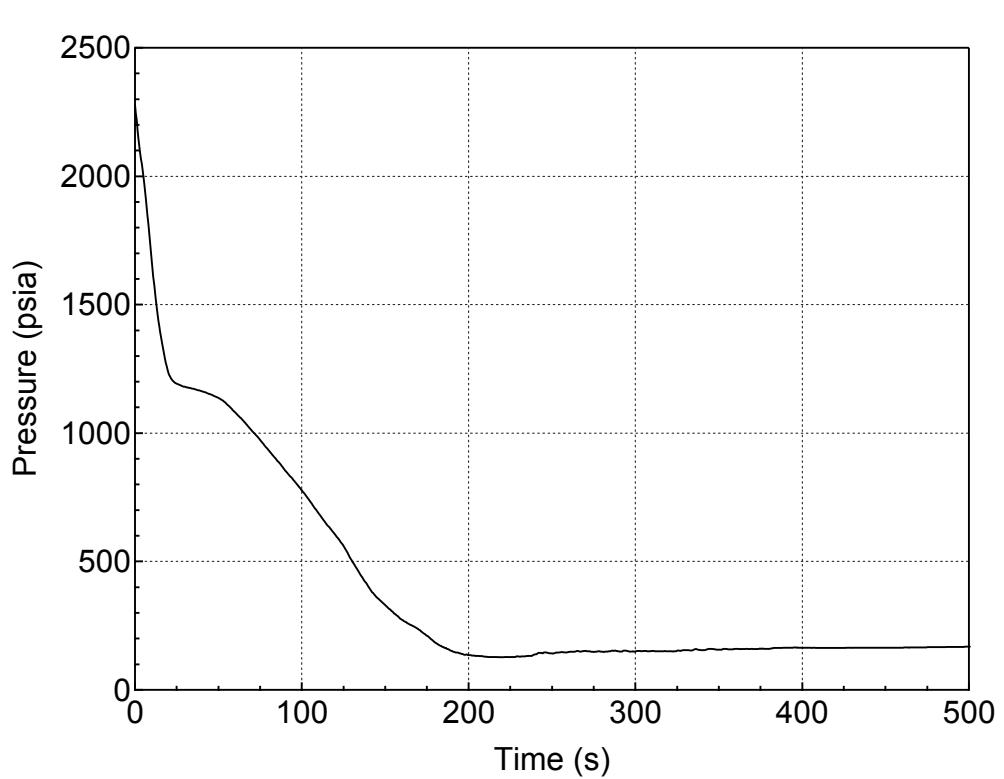
**Figure 5.3.2.a-10 RCS (Pressurizer) Pressure Transient for 12-inch Break (Side)
