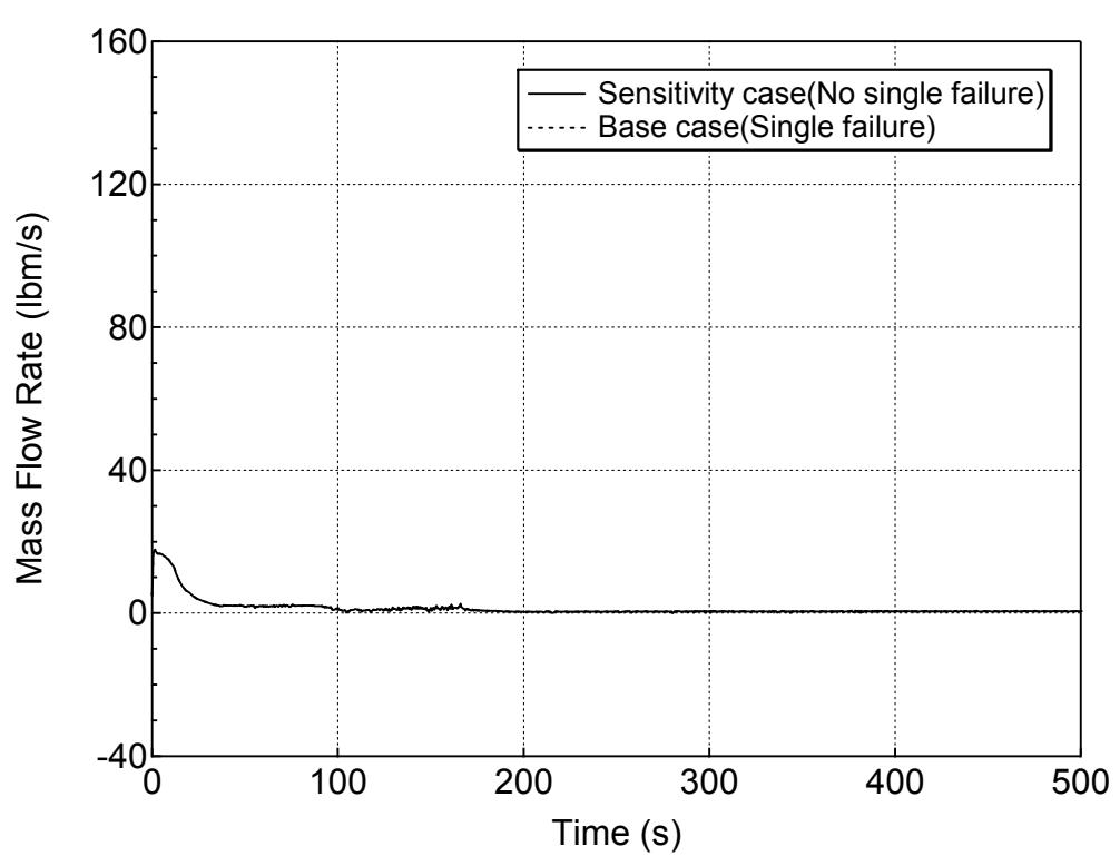
**Figure 5.6.1-26 Hot Assembly Exit Vapor Mass Flowrate for 1-ft<sup>2</sup> Break (Top)
