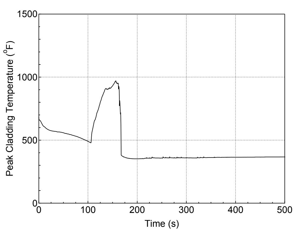
**Figure 5.2.m-8 PCT at All Elevations for Hot Rod in Hot Assembly
