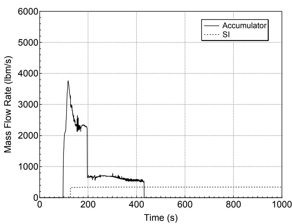
**Figure 5.1.1.b-13 Accumulator and Safety Injection Mass Flowrates
