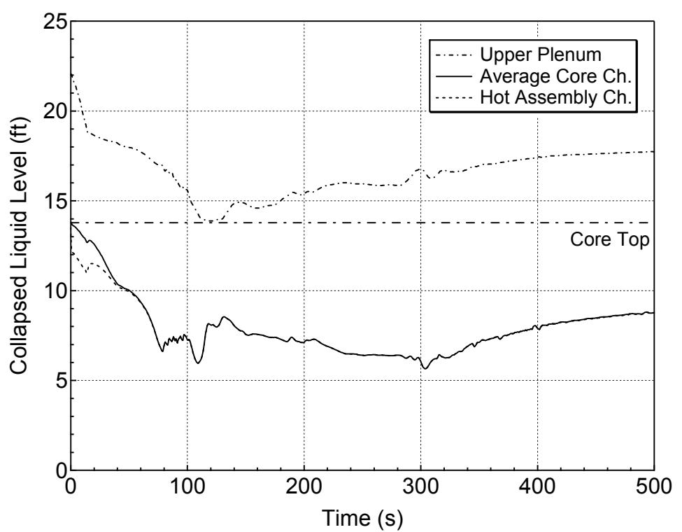
**Figure 5.3.1.e-16 Core and Upper Plenum Collapsed Levels for 8-inch Break (Side)
