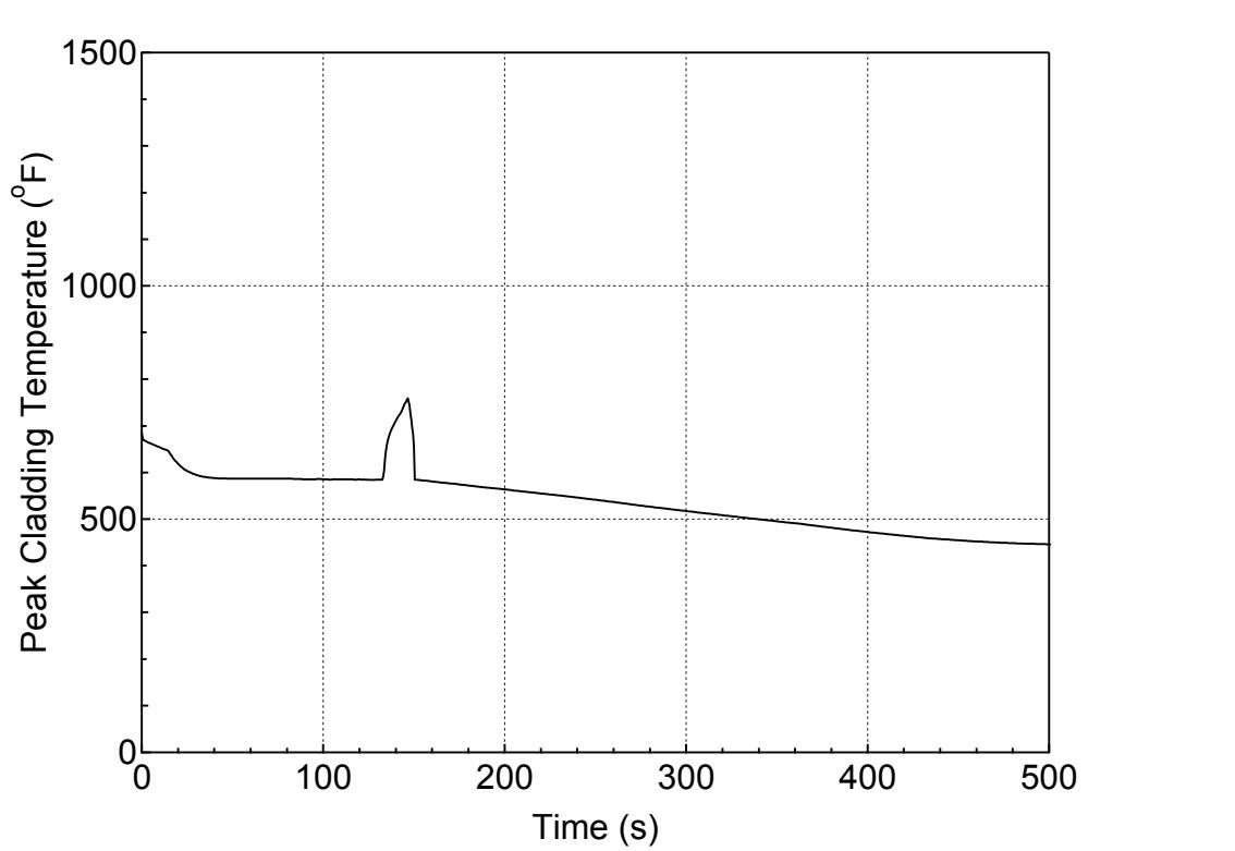
**Figure 5.3.1.c-17 PCT at All Elevations for Hot Rod in Hot Assembly
