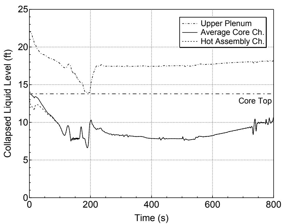
**Figure 5.2.f-7 Core and Upper Plenum Collapsed Levels for 6-inch Break (Bottom)
