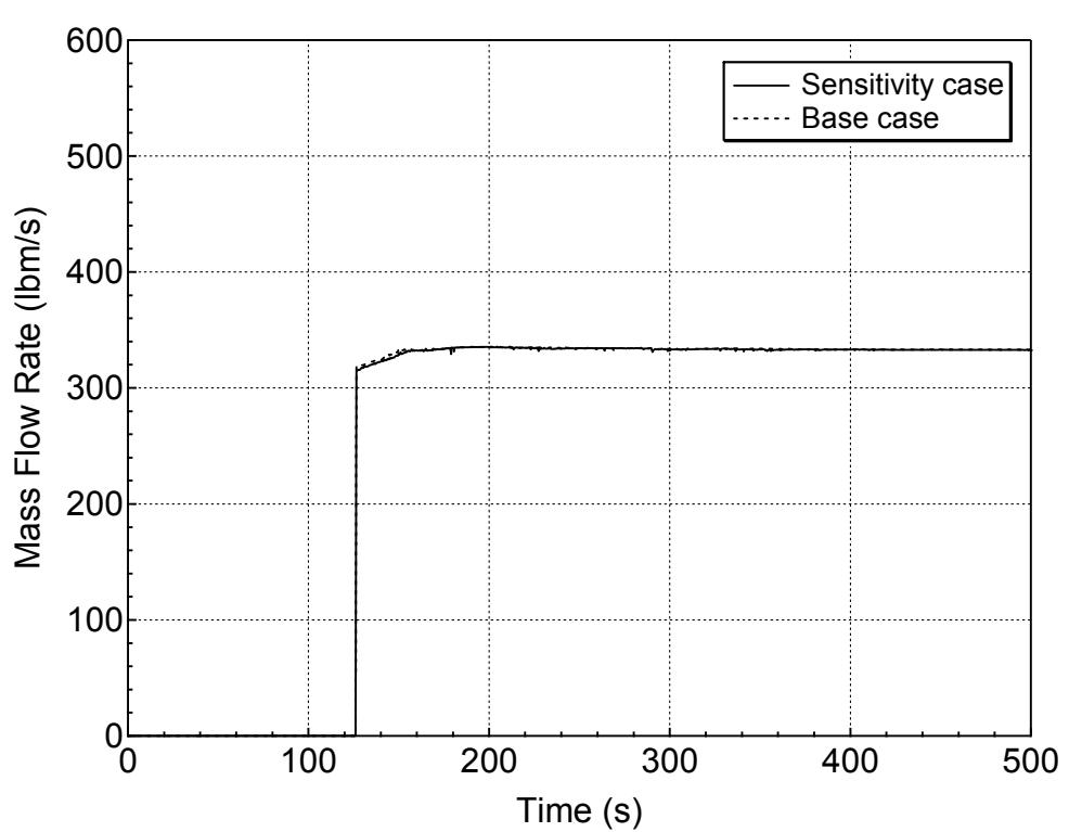
**Figure 5.4.1-19 Safety Injection Mass Flowrate for 1-ft<sup>2</sup> Break (Top)
