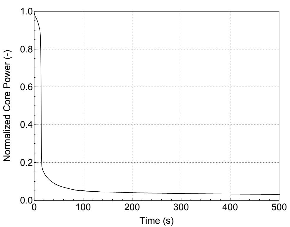
**Figure 5.3.1.c-11 Normalized Core Power for 7-inch Break (Side)
