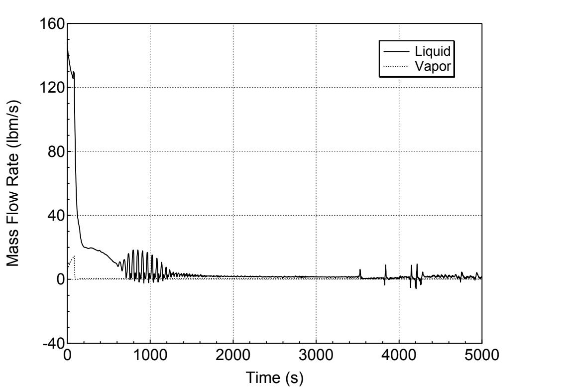
**Figure 5.2.b-9 Hot Assembly Exit Vapor and Liquid Mass Flowrates
