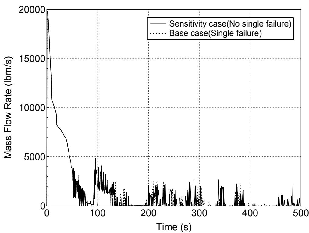
**Figure 5.6.1-16 Liquid Discharge through the Break for 1-ft<sup>2</sup> Break (Top)
