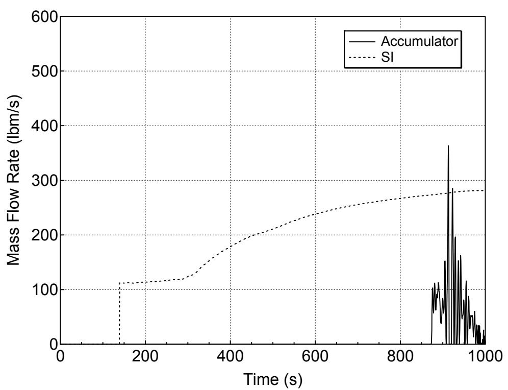
**Figure 5.2.e-4 Accumulator and Safety Injection Mass Flowrates
