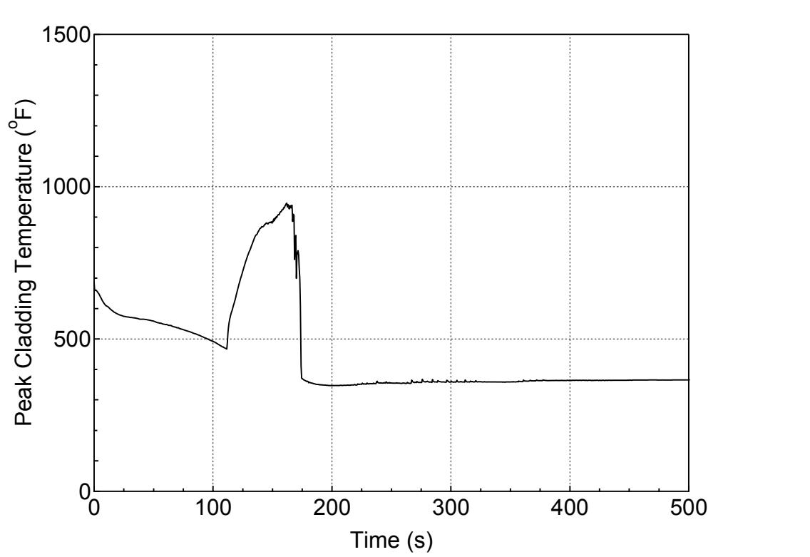
**Figure 5.3.2.b-17 PCT at All Elevations for Hot Rod in Hot Assembly
