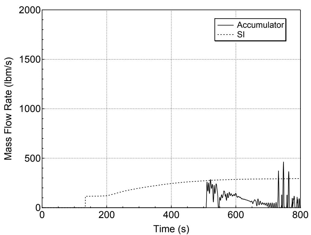
**Figure 5.3.1.a-22 Accumulator and Safety Injection Mass Flowrates
