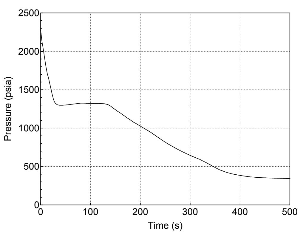
**Figure 5.3.1.d-19 RCS (Pressurizer) Pressure Transient for 7.5-inch Break (Side)
