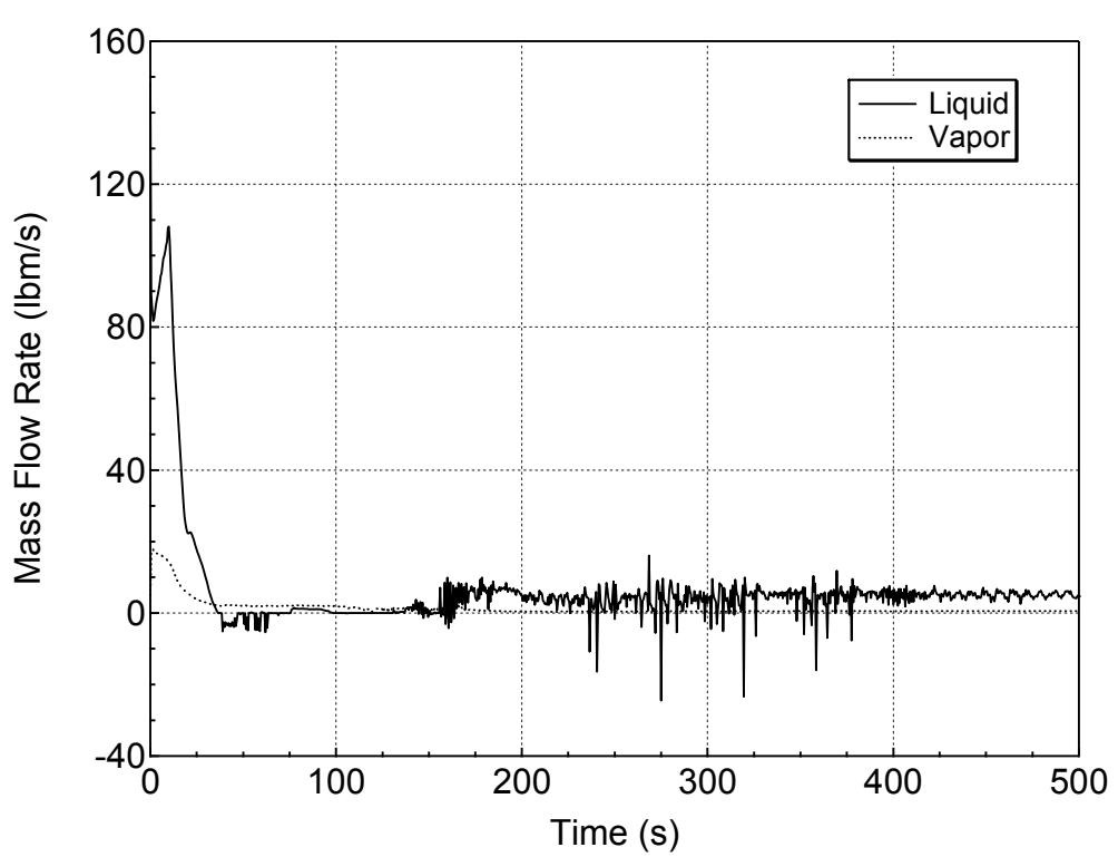
**Figure 5.3.2.c-27 Hot Assembly Exit Vapor and Liquid Mass Flowrates
