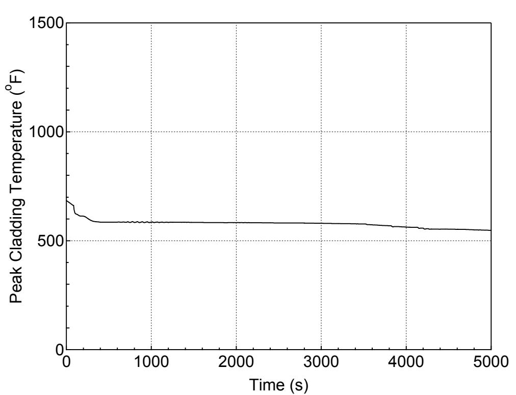
**Figure 5.2.b-8 PCT at All Elevations for Hot Rod in Hot Assembly
