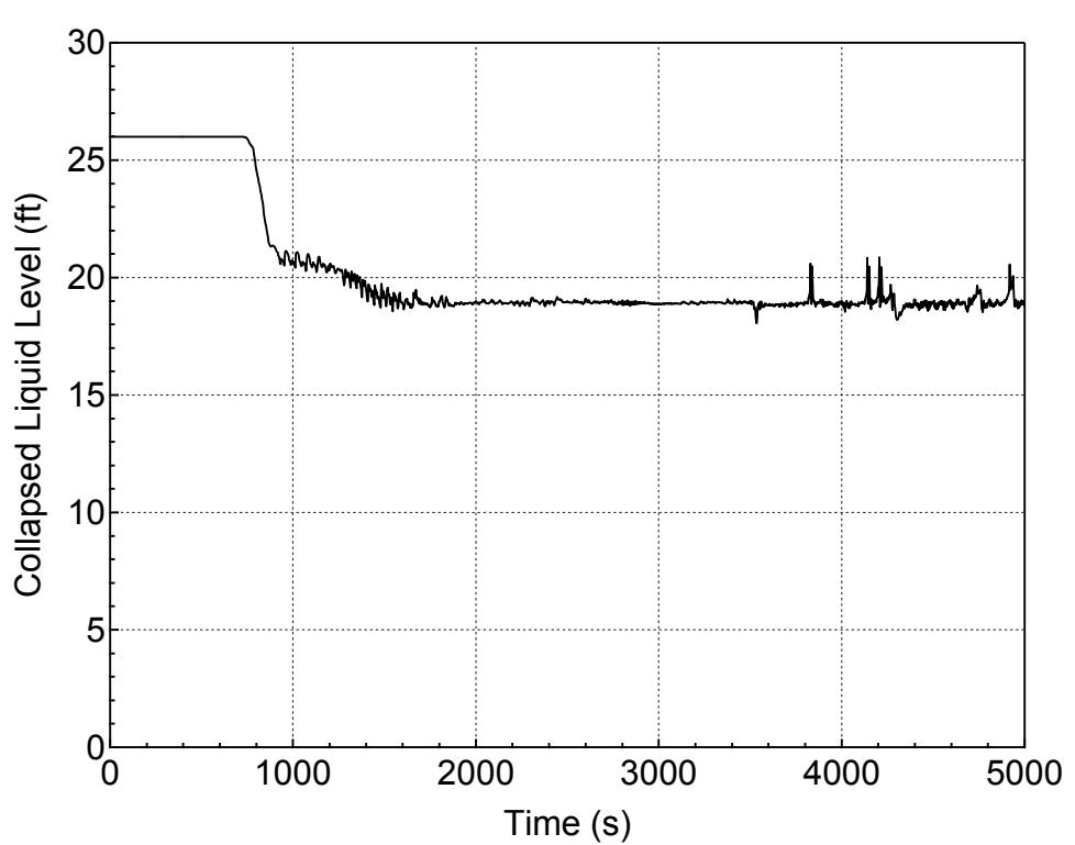
**Figure 5.2.b-6 Downcomer Collapsed Level for 2-inch Break (Bottom)
