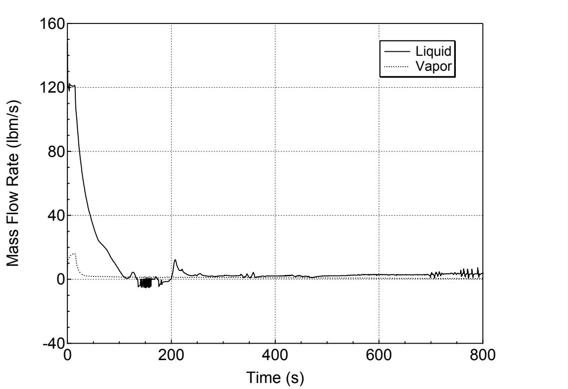
**Figure 5.3.1.a-18 Hot Assembly Exit Vapor and Liquid Mass Flowrates
