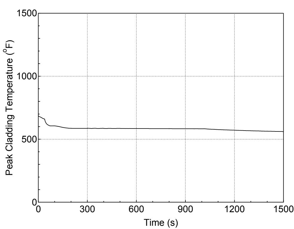
**Figure 5.2.c-8 PCT at All Elevations for Hot Rod in Hot Assembly
