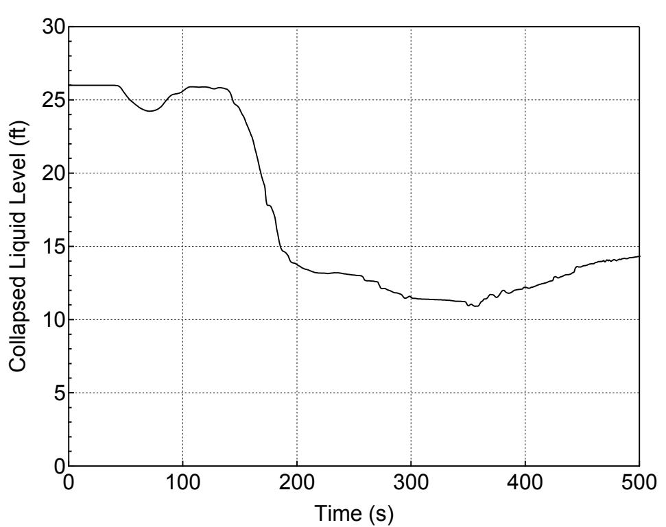
**Figure 5.2.g-6 Downcomer Collapsed Level for 7-inch Break (Bottom)
