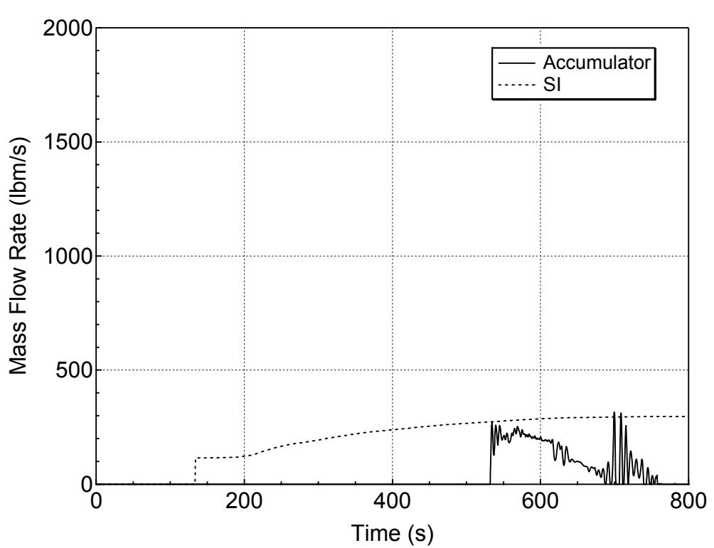
**Figure 5.3.1.a-13 Accumulator and Safety Injection Mass Flowrates
