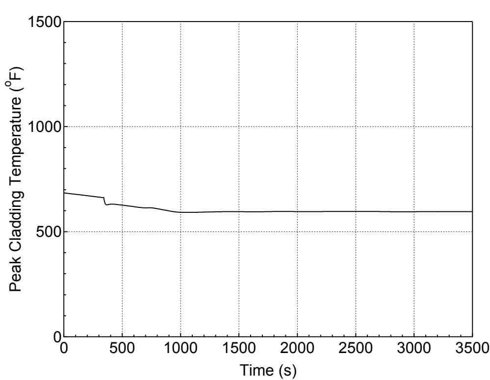
**Figure 5.2.a-8 PCT at All Elevations for Hot Rod in Hot Assembly
