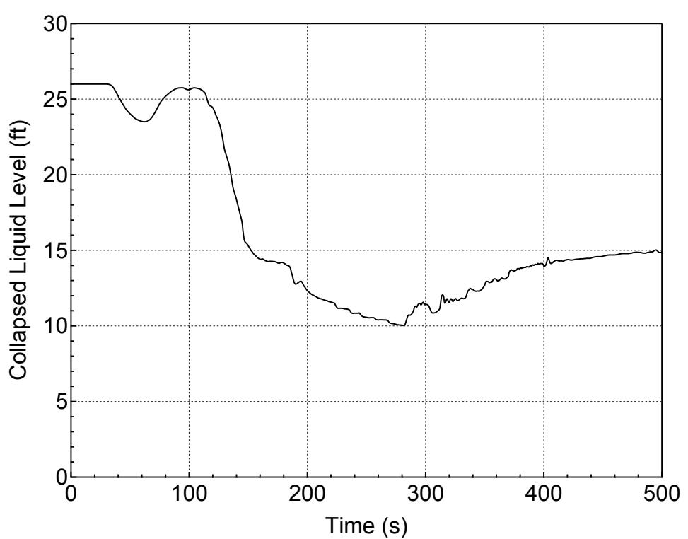
**Figure 5.3.1.e-24 Downcomer Collapsed Level for 8-inch Break (Homogeneous)
