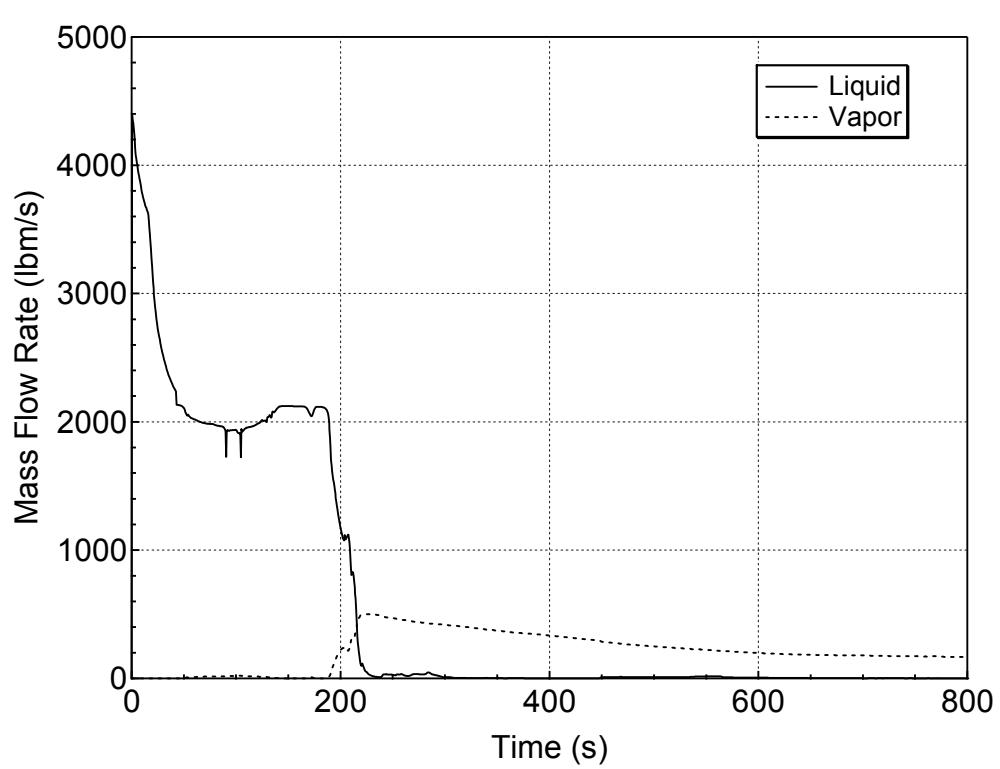
**Figure 5.3.1.a-12 Liquid and Vapor Discharges through the Break
