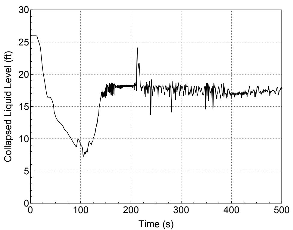
**Figure 5.1.1.a-15 Downcomer Collapsed Level for 1-ft<sup>2</sup> Break (Bottom)
