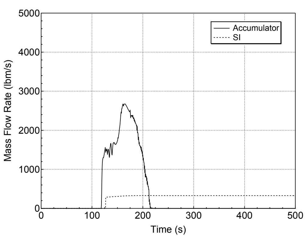
**Figure 5.3.2.a-4 Accumulator and Safety Injection Mass Flowrates
