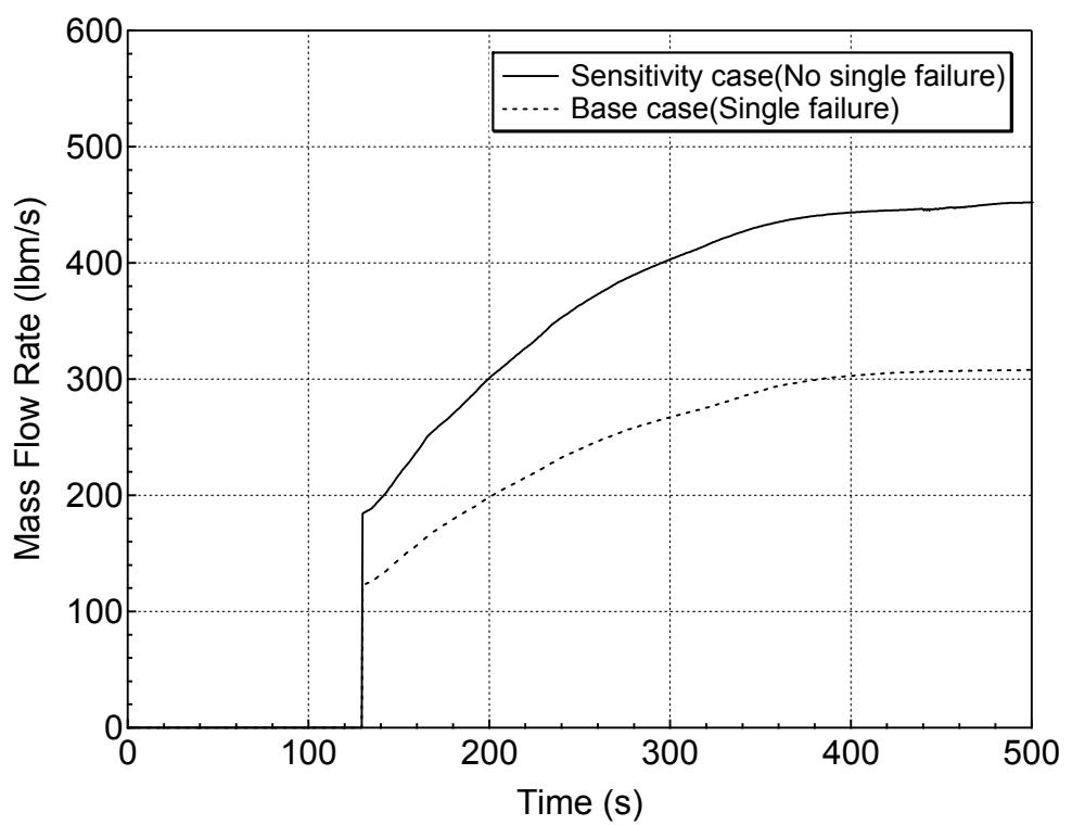
**Figure 5.6.1-6 Safety Injection Mass Flowrate for 7.5-inch Break (Top)
