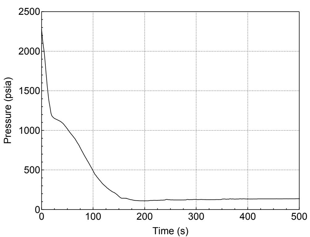
**Figure 5.1.1.a-10 RCS (Pressurizer) Pressure Transient for 1-ft<sup>2</sup> Break (Bottom)
