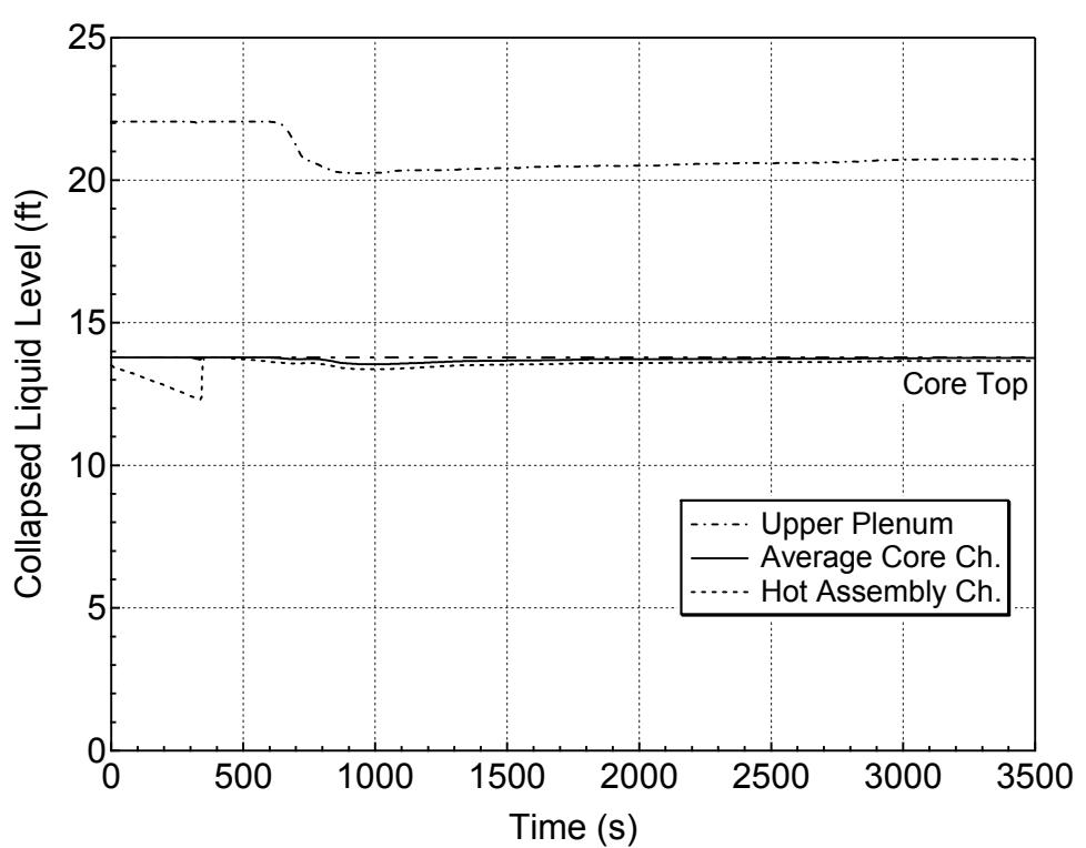
**Figure 5.2.a-7 Core and Upper Plenum Collapsed Levels for 1-inch Break (Bottom)
