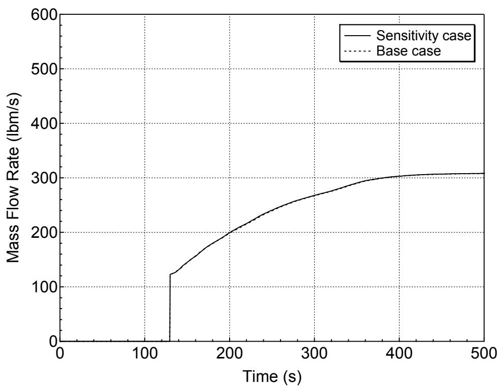
**Figure 5.4.1-6 Safety Injection Mass Flowrate for 7.5-inch Break (Top)
