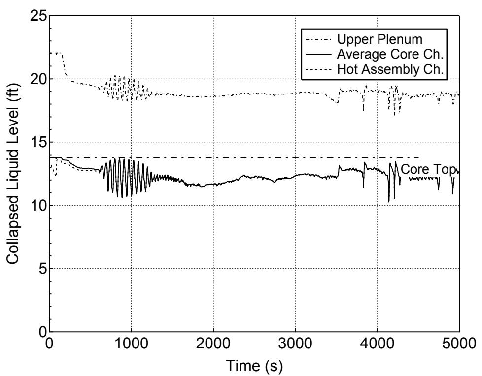
**Figure 5.1.1.a-7 Core and Upper Plenum Collapsed Levels for 2-inch Break (Bottom)
