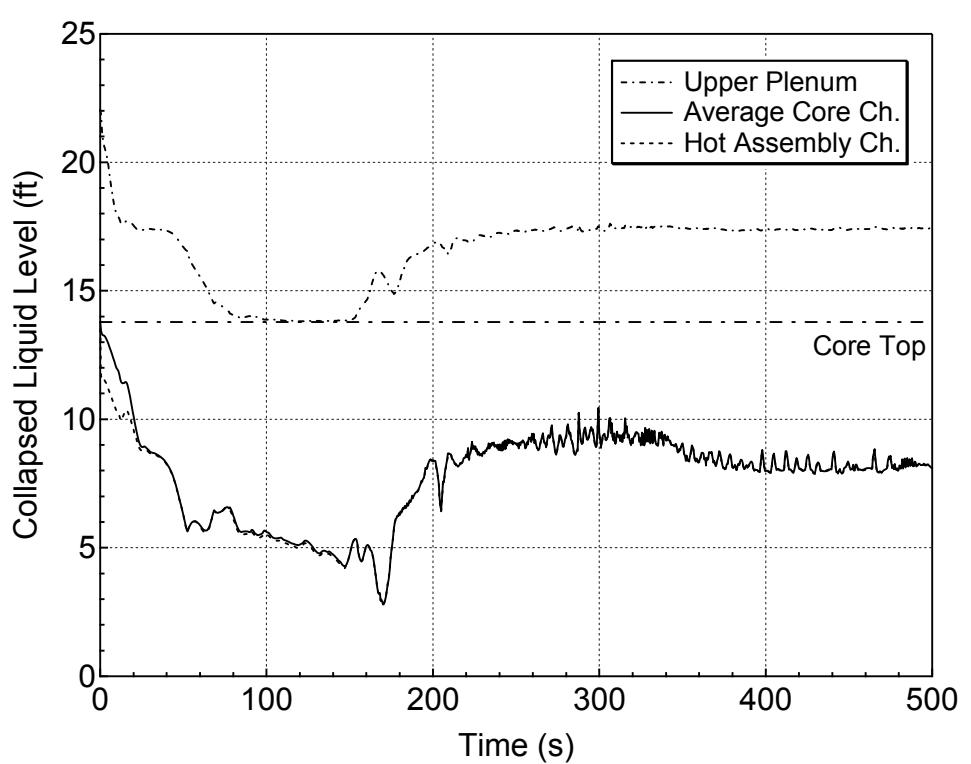
**Figure 5.2.k-7 Core and Upper Plenum Collapsed Levels for 11-inch Break (Bottom) (Spectrum Analysis)**
