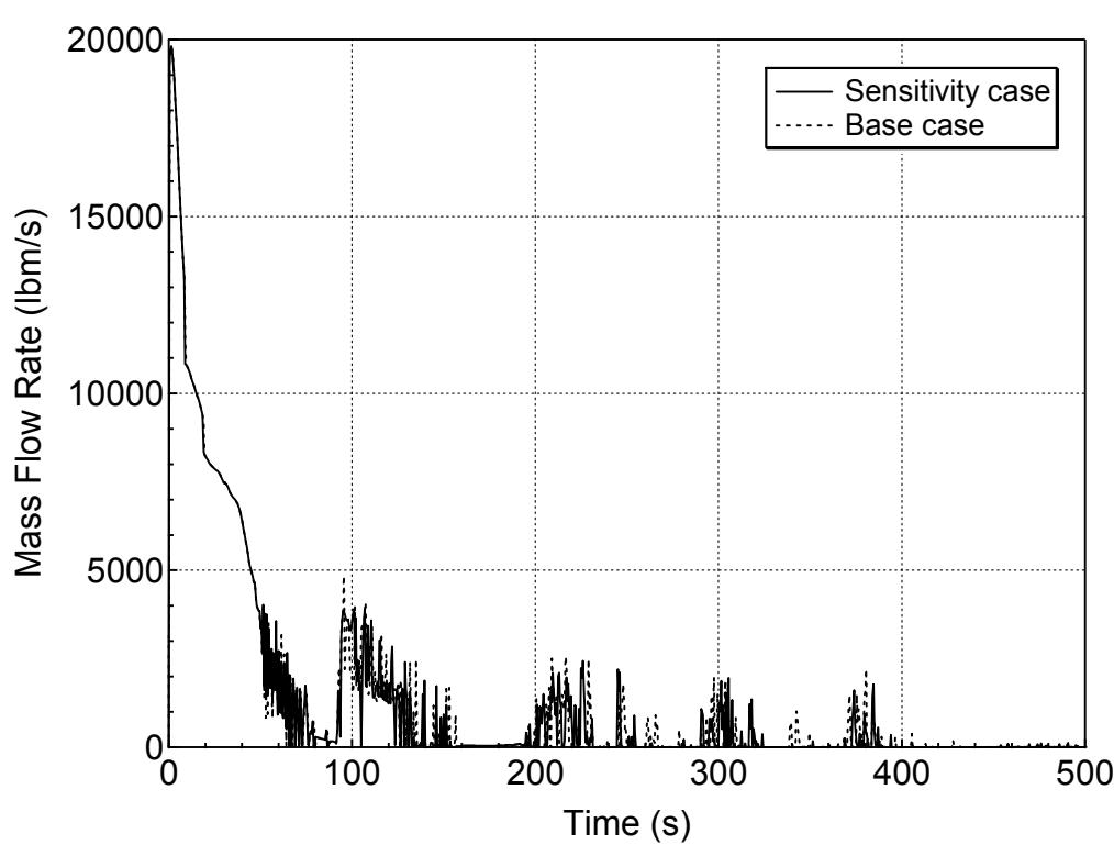
**Figure 5.5.b-3 Liquid Discharge through the Break for 1-ft<sup>2</sup> Break (Top)
