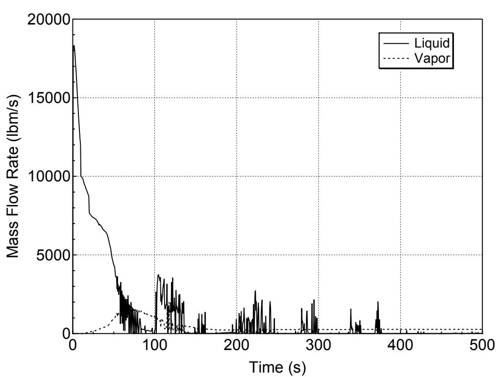
**Figure 5.3.2.b-3 Liquid and Vapor Discharges through the Break
