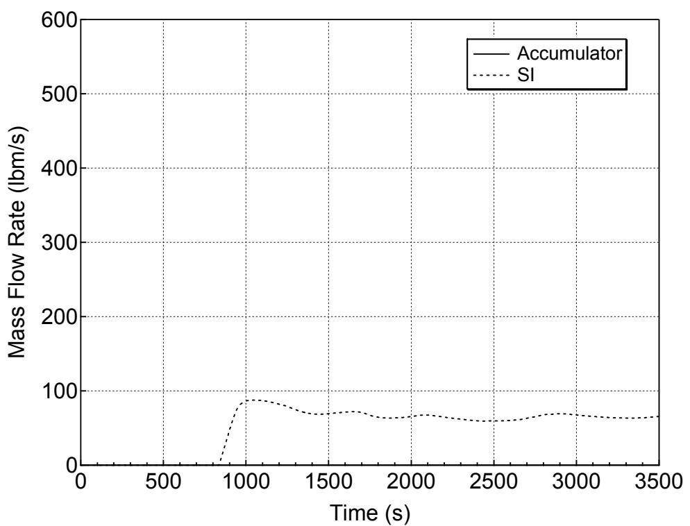
**Figure 5.2.a-4 Accumulator and Safety Injection Mass Flowrates
