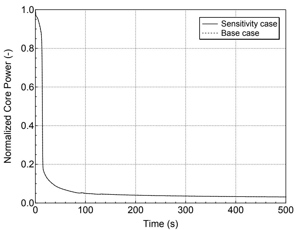
**Figure 5.4.2-2 Normalized Core Power for 7.5-inch Break (Top)
