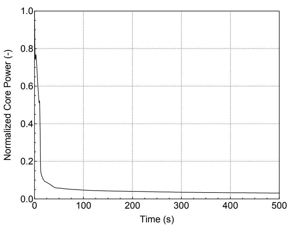
**Figure 5.3.2.b-11 Normalized Core Power for 13-inch Break (Side)
