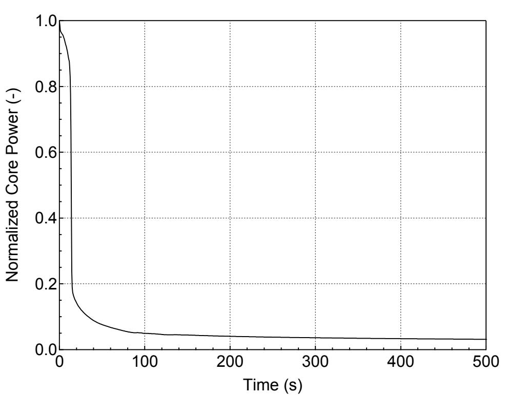
**Figure 5.3.1.d-2 Normalized Core Power for 7.5-inch Break (Bottom)
