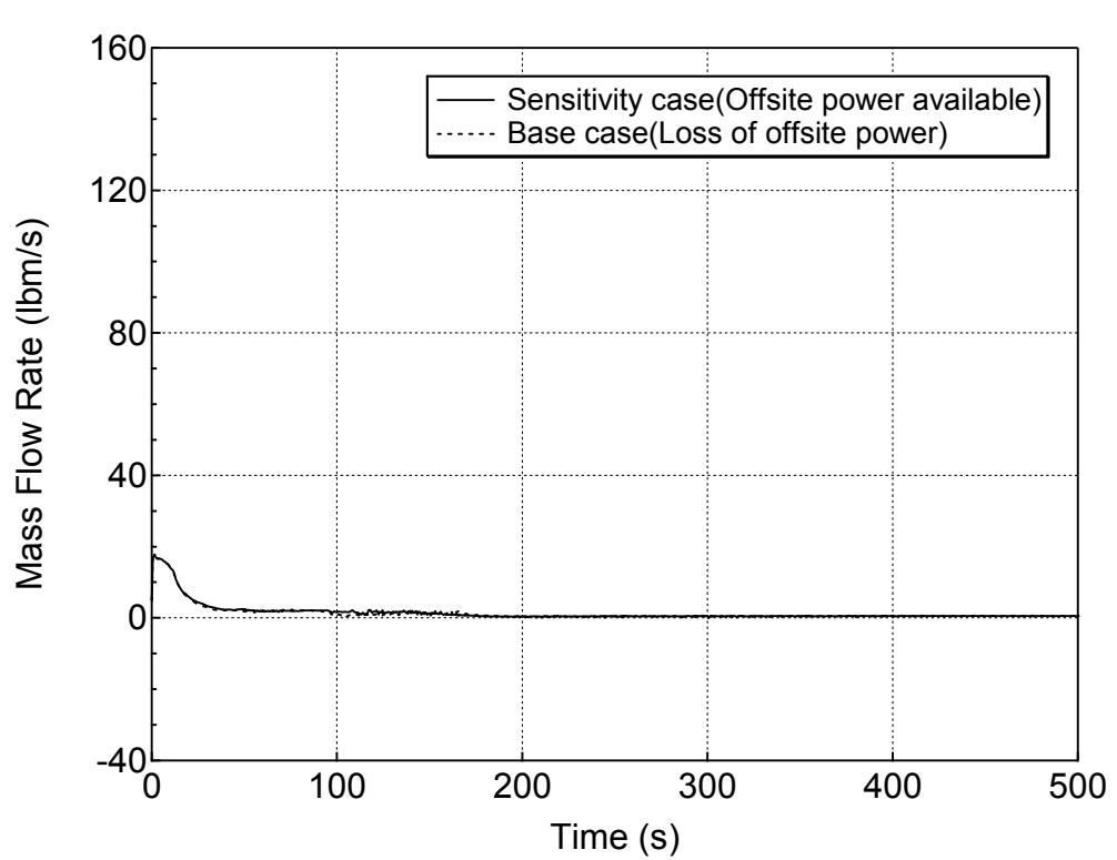
**Figure 5.6.2-26 Hot Assembly Exit Vapor Mass Flowrate for 1-ft<sup>2</sup> Break (Top)
