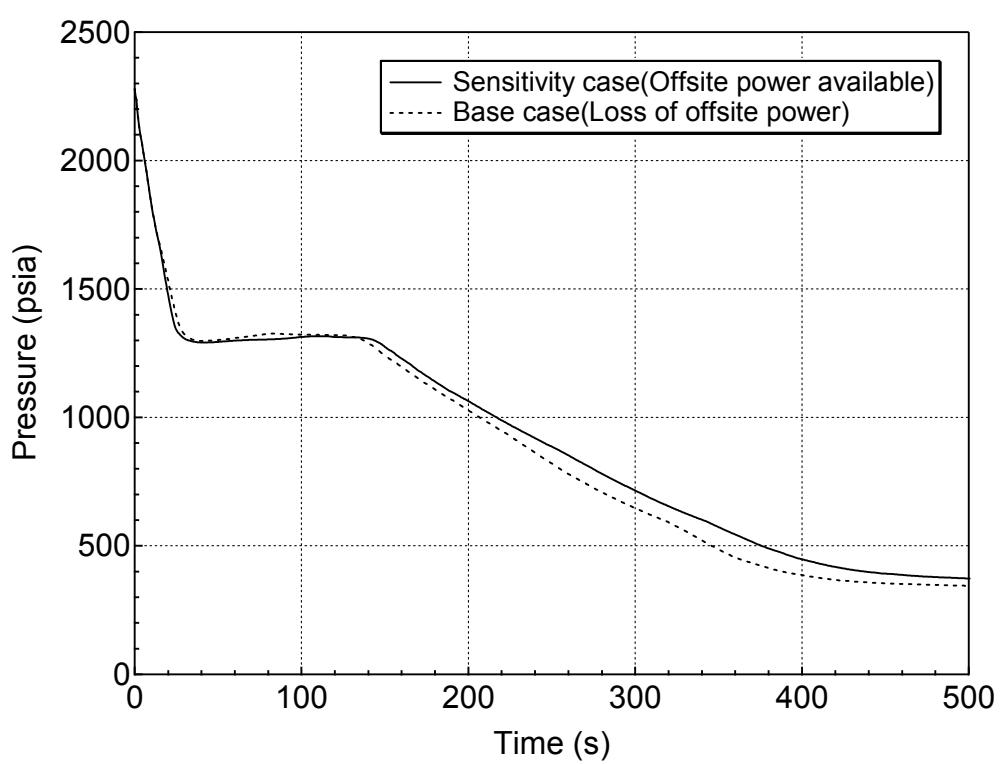
**Figure 5.6.2-1 RCS (Pressurizer) Pressure Transient for 7.5-inch Break (Top)
