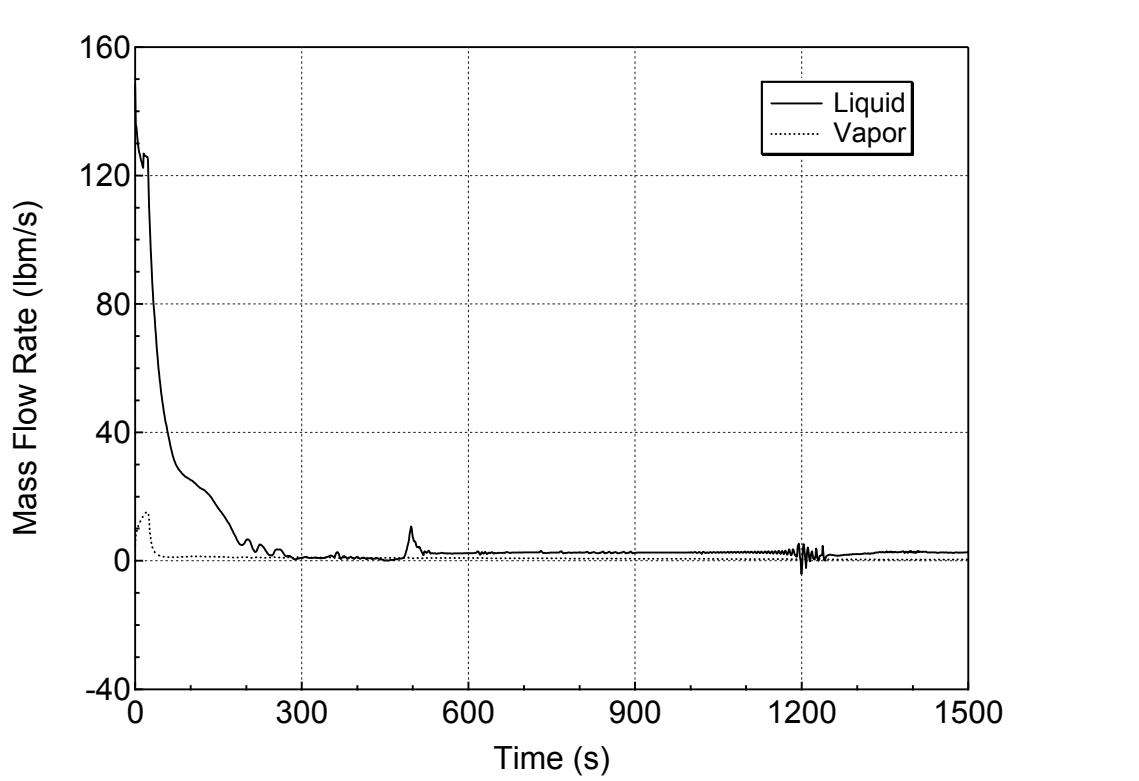
**Figure 5.2.d-9 Hot Assembly Exit Vapor and Liquid Mass Flowrates
