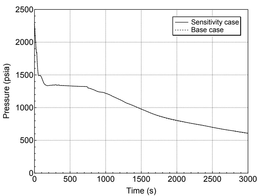
**Figure 5.5.c-1 RCS (Pressurizer) Pressure Transient for DVI-line Break
