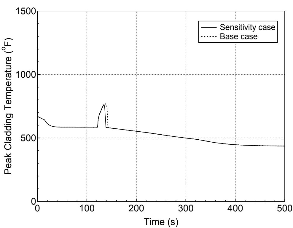
**Figure 5.4.1-11 PCT at All Elevations for Hot Rod in Hot Assembly
