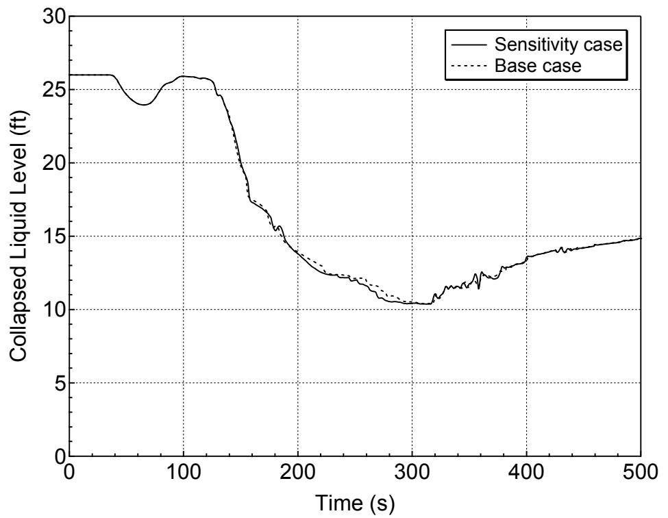
**Figure 5.5.a-8 Downcomer Collapsed Level for 7.5-inch Break (Top)
