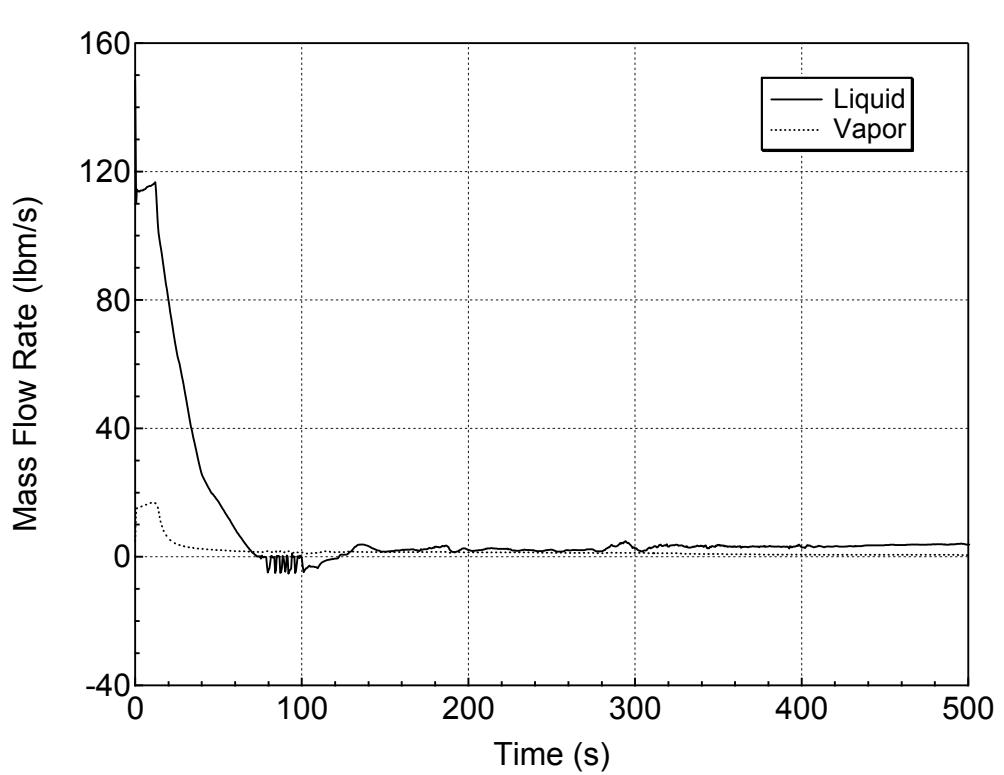
**Figure 5.3.1.e-9 Hot Assembly Exit Vapor and Liquid Mass Flowrates
