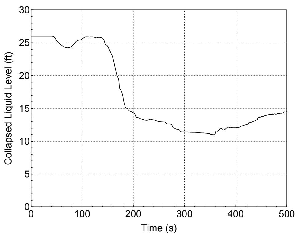
**Figure 5.3.1.c-6 Downcomer Collapsed Level for 7-inch Break (Top)
