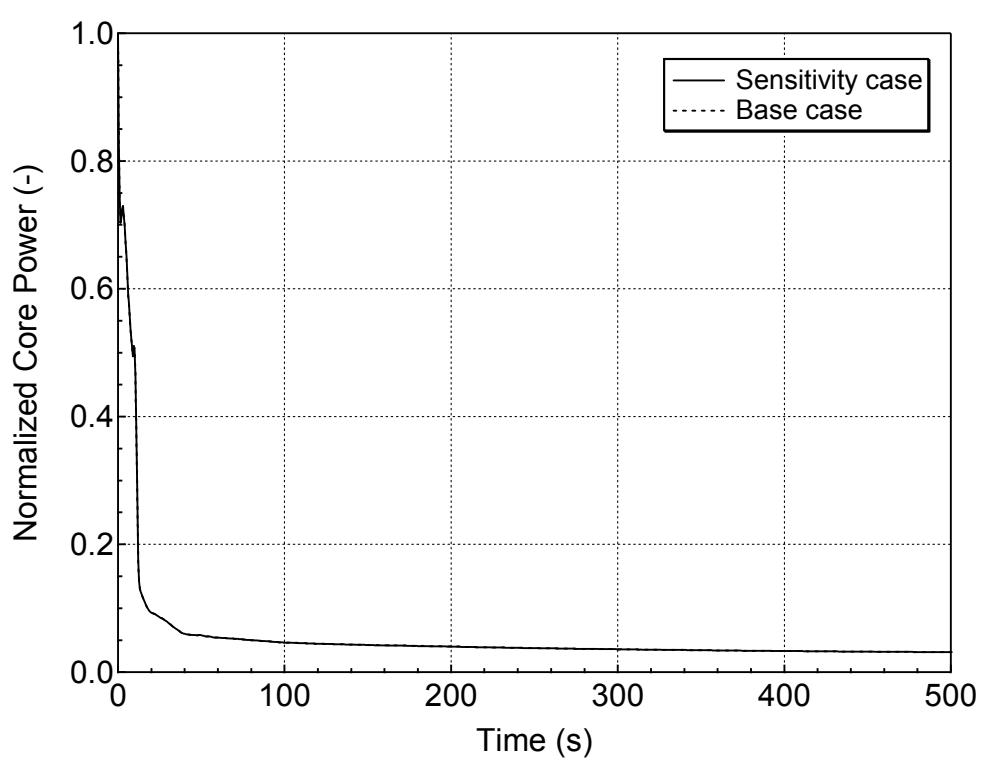
**Figure 5.4.3-15 Normalized Core Power for 1-ft<sup>2</sup> Break (Top)
