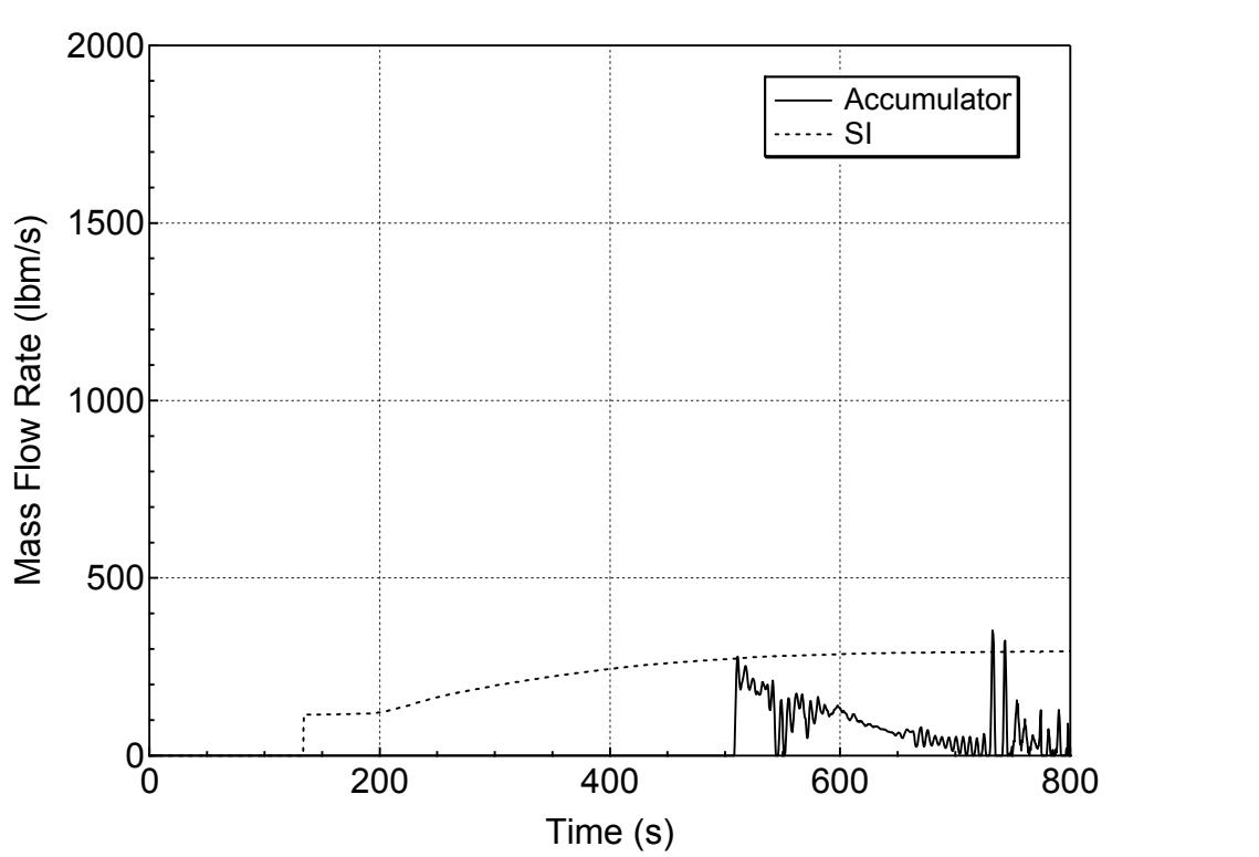
**Figure 5.2.f-4 Accumulator and Safety Injection Mass Flowrates
