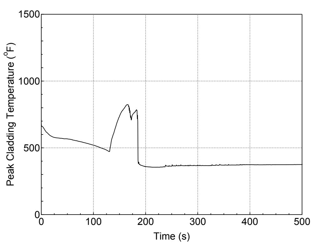
**Figure 5.3.2.a-17 PCT at All Elevations for Hot Rod in Hot Assembly
