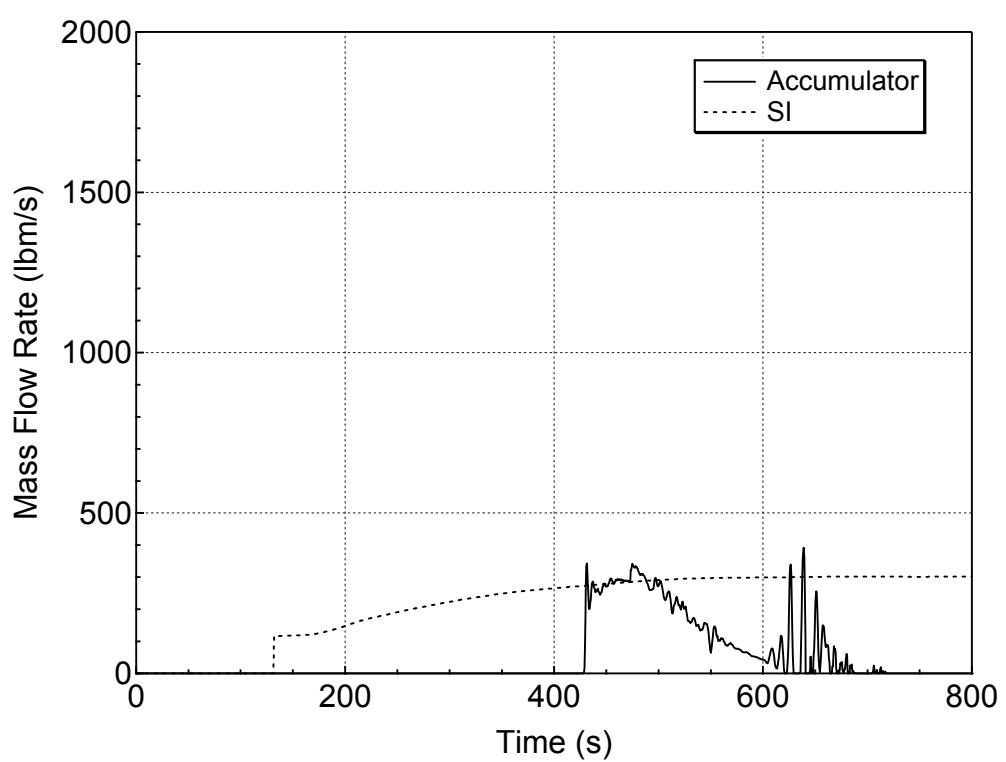
**Figure 5.3.1.b-31 Accumulator and Safety Injection Mass Flowrates
