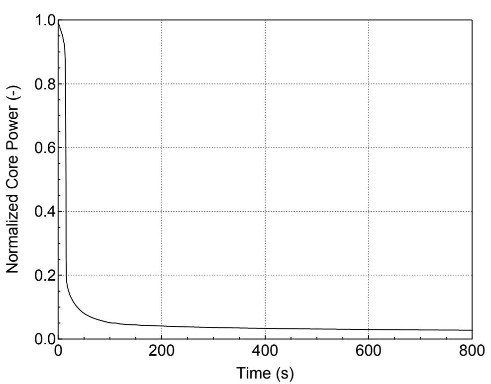
**Figure 5.3.1.b-11 Normalized Core Power for 6.5-inch Break (Top)
