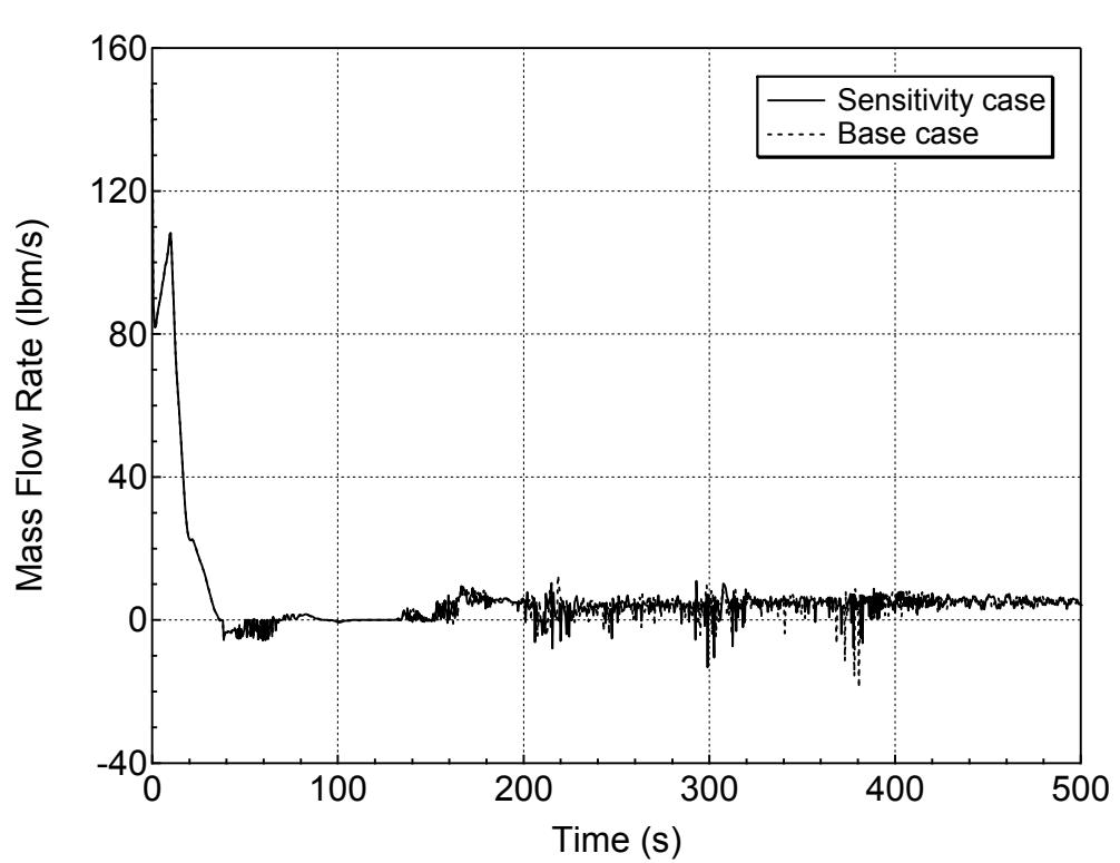
**Figure 5.5.b-12 Hot Assembly Exit Liquid Mass Flowrate for 1-ft<sup>2</sup> Break (Top)
