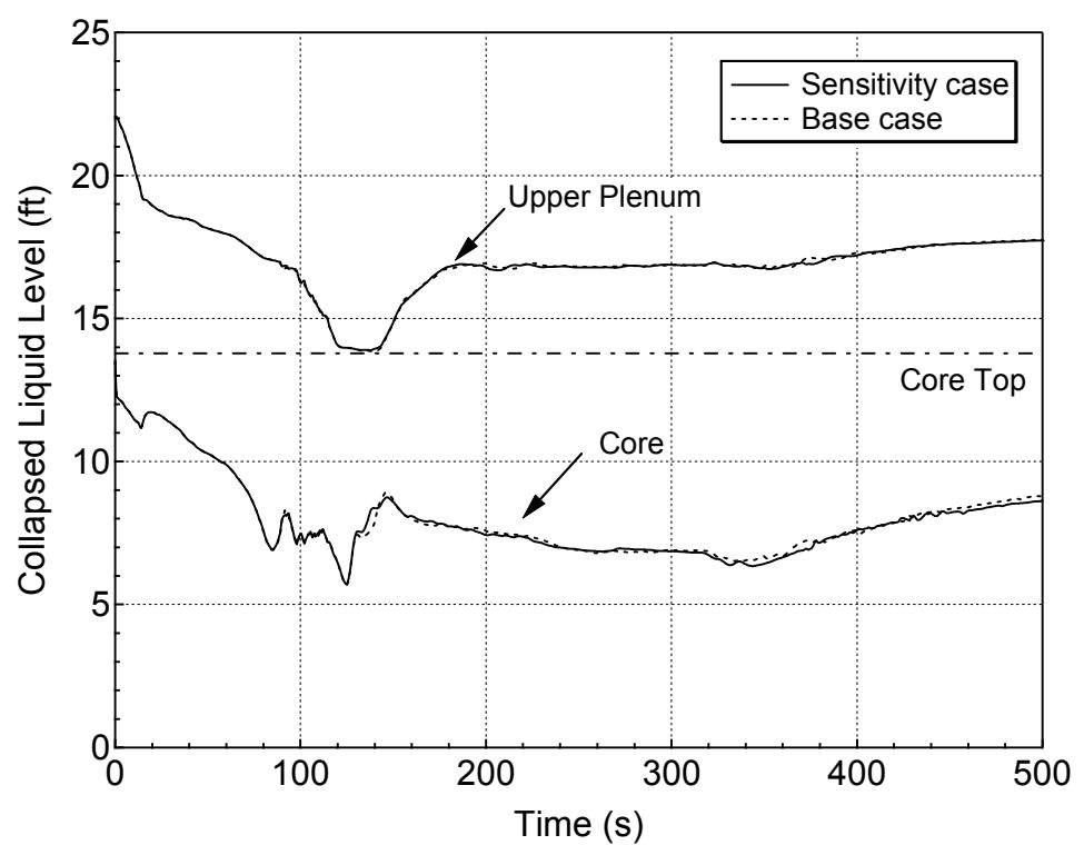
**Figure 5.4.3-10 Hot Assembly Core and Upper Plenum Collapsed Levels for 7.5-inch Break (Top)
