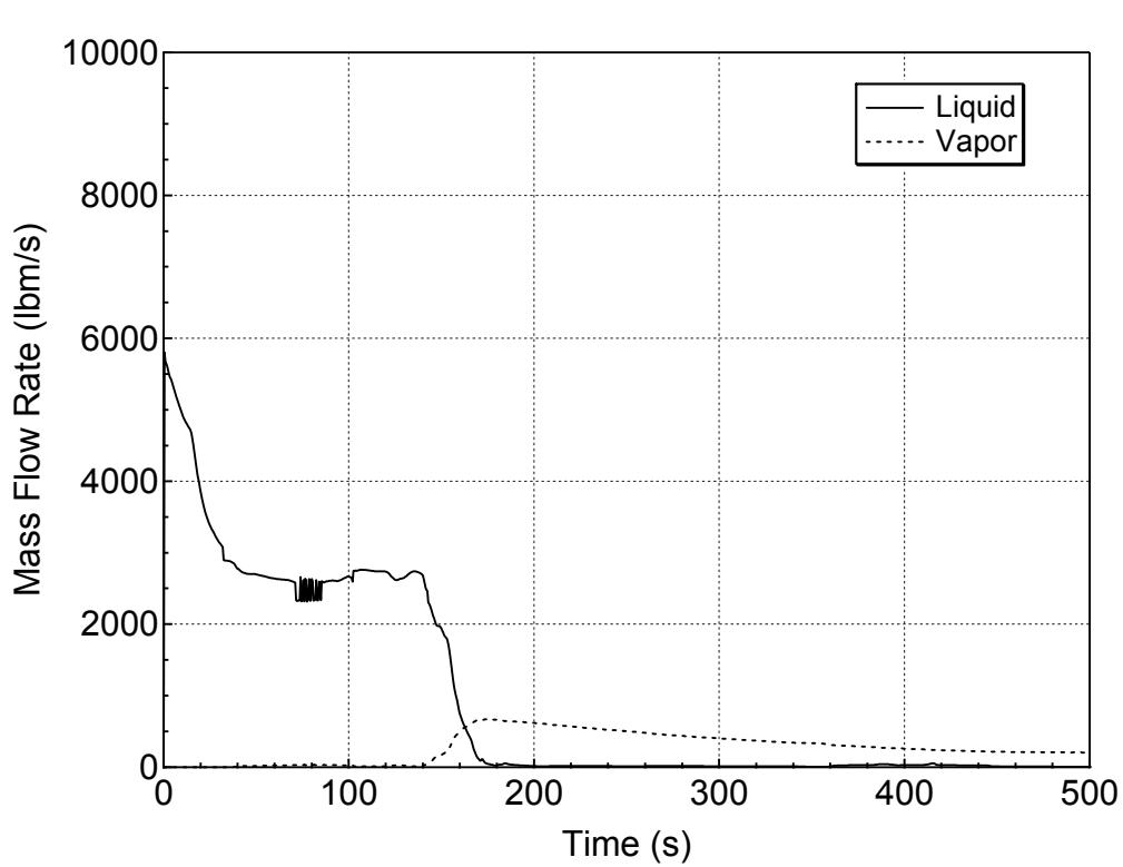
**Figure 5.3.1.c-12 Liquid and Vapor Discharges through the Break
