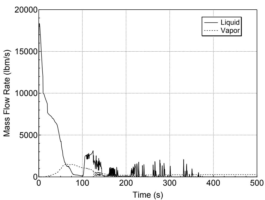
**Figure 5.3.2.b-21 Liquid and Vapor Discharges through the Break
