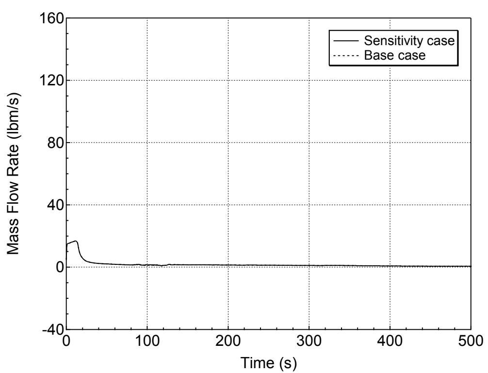
**Figure 5.5.a-13 Hot Assembly Exit Vapor Mass Flowrate for 7.5-inch Break (Top)
