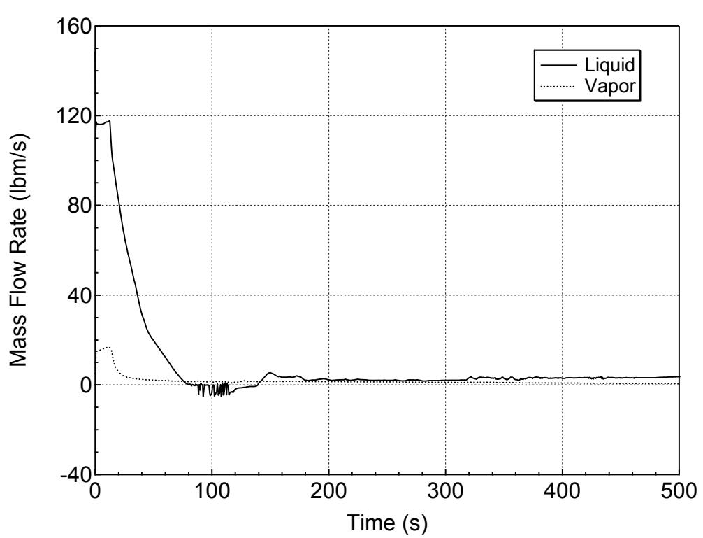
**Figure 5.3.1.d-36 Hot Assembly Exit Vapor and Liquid Mass Flowrates for 7.5-inch Break (Homogeneous) (Break Orientation Sensitivity Study)**
