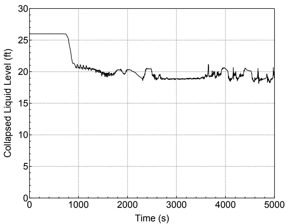
**Figure 5.1.1.c-6 Downcomer Collapsed Level for 2-inch Break (Bottom)
