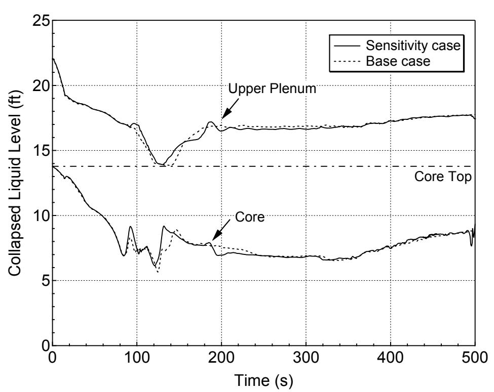
**Figure 5.4.2-9 Average Core and Upper Plenum Collapsed Levels
