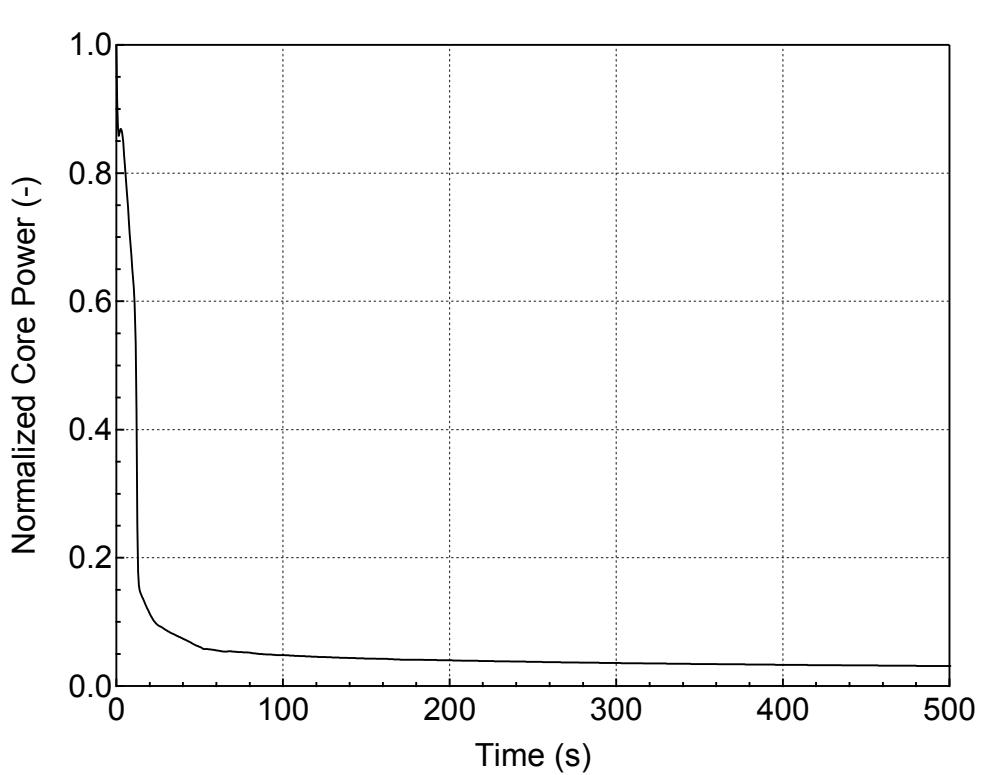
**Figure 5.2.k-2 Normalized Core Power for 11-inch Break (Bottom)
