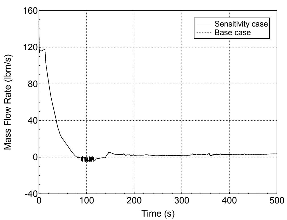
**Figure 5.5.a-12 Hot Assembly Exit Liquid Mass Flowrate for 7.5-inch Break (Top)
