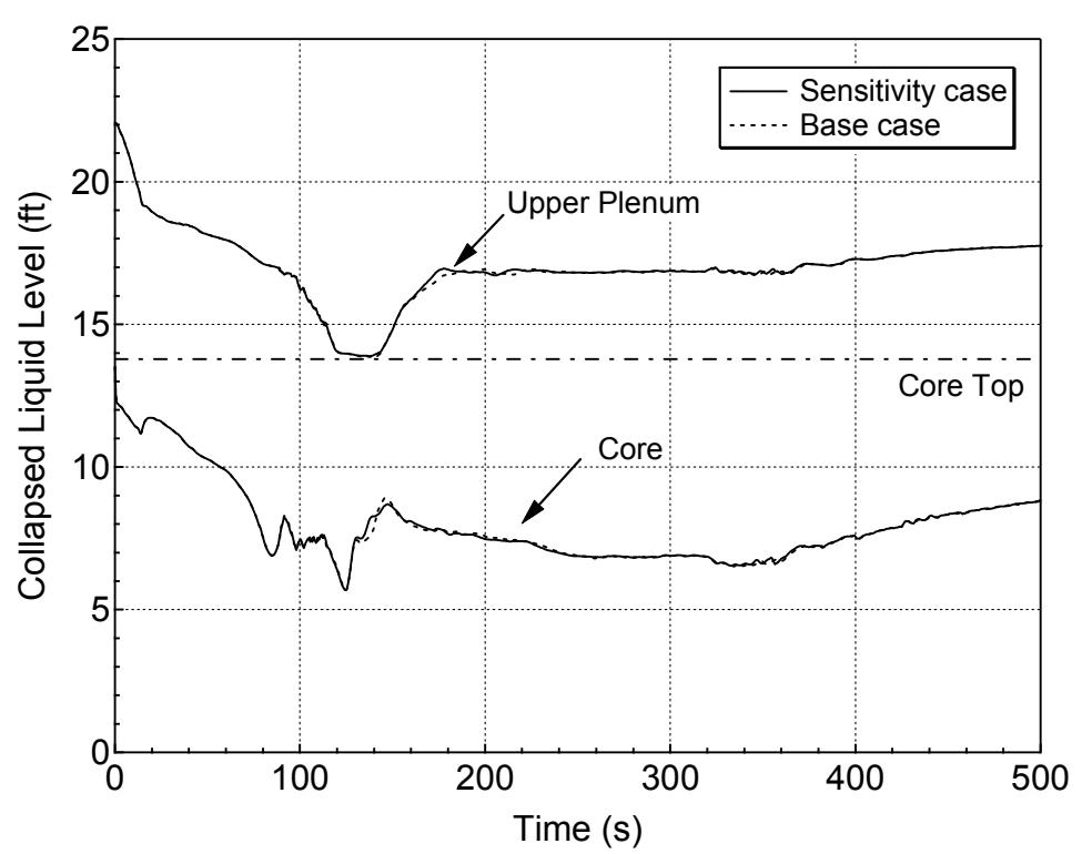
**Figure 5.4.1-10 Hot Assembly Core and Upper Plenum Collapsed Levels
