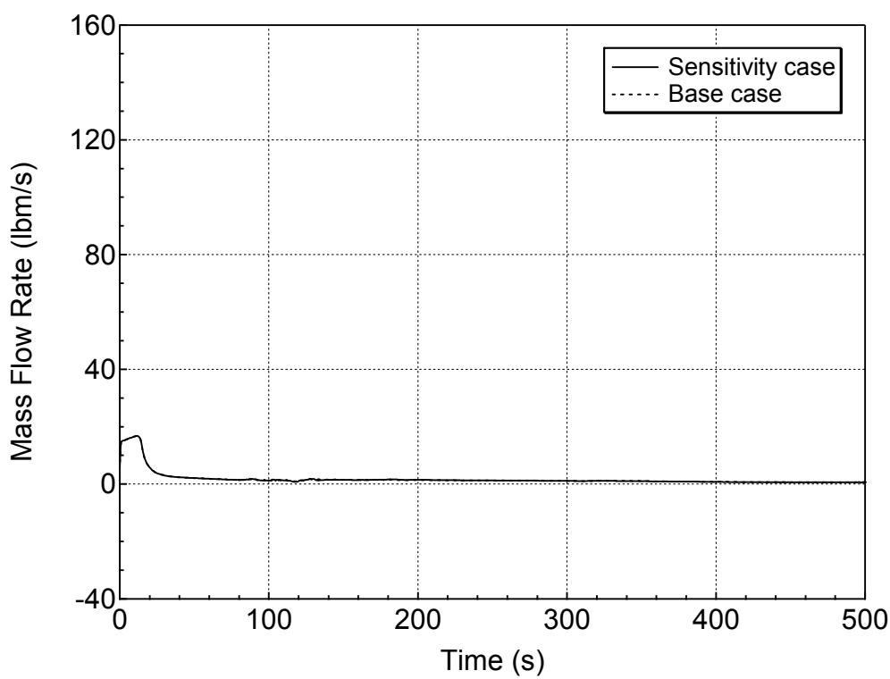
**Figure 5.4.2-13 Hot Assembly Exit Vapor Mass Flowrate for 7.5-inch Break (Top)
