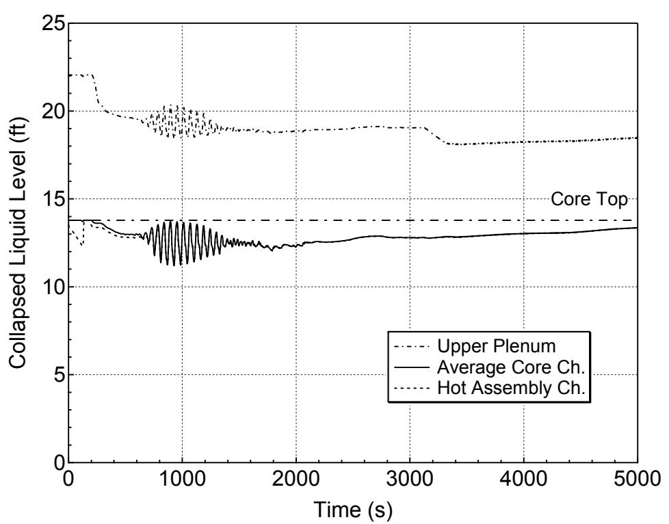
**Figure 5.1.1.b-7 Core and Upper Plenum Collapsed Levels for 2-inch Break (Bottom)
