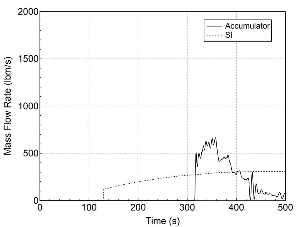
**Figure 5.3.1.d-13 Accumulator and Safety Injection Mass Flowrates
