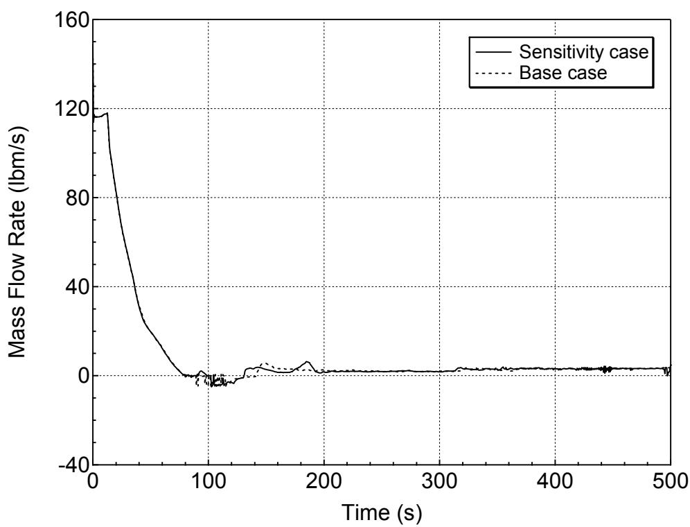
**Figure 5.4.2-12 Hot Assembly Exit Liquid Mass Flowrate for 7.5-inch Break (Top)
