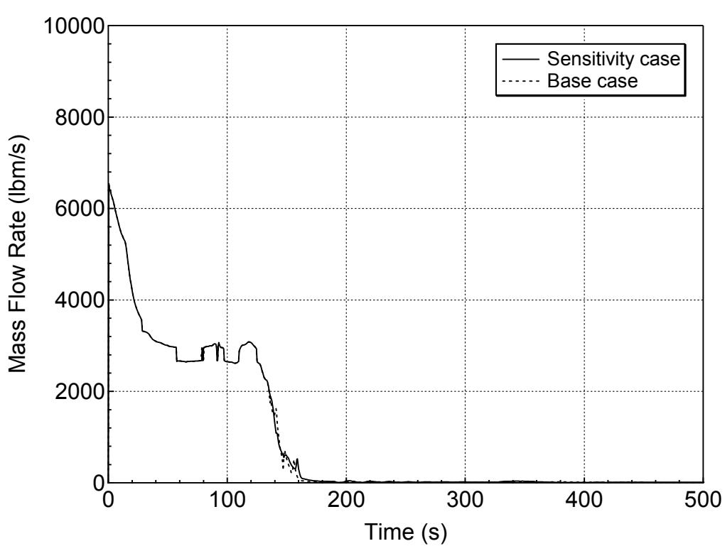
**Figure 5.4.3-3 Liquid Discharge through the Break for 7.5-inch Break (Top)
