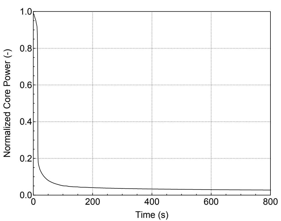
**Figure 5.3.1.b-20 Normalized Core Power for 6.5-inch Break (Side)
