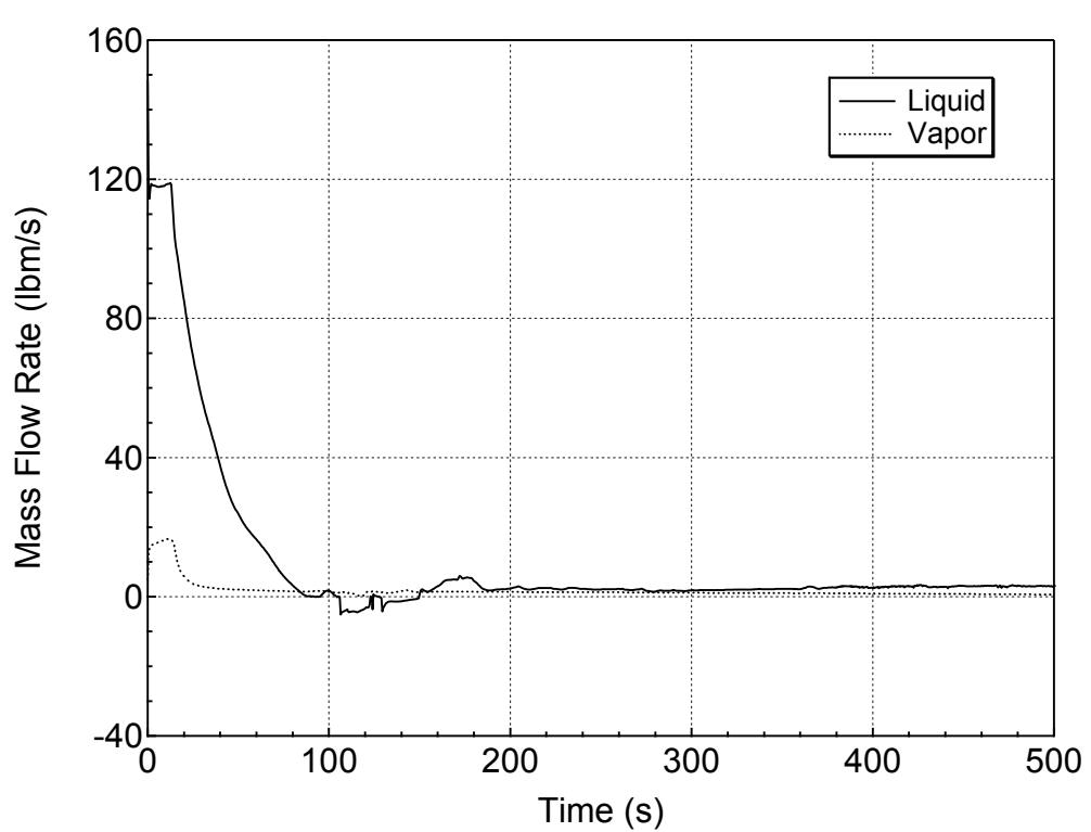
**Figure 5.3.1.c-27 Hot Assembly Exit Vapor and Liquid Mass Flowrates
