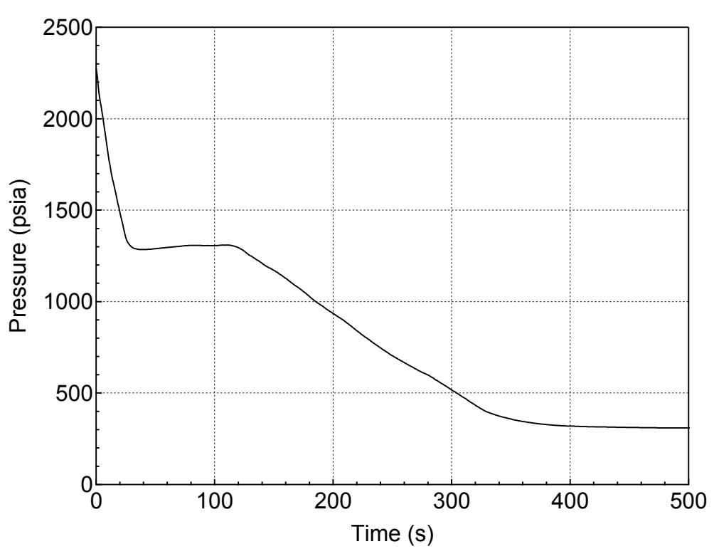
**Figure 5.3.1.e-1 RCS (Pressurizer) Pressure Transient for 8-inch Break (Top)
