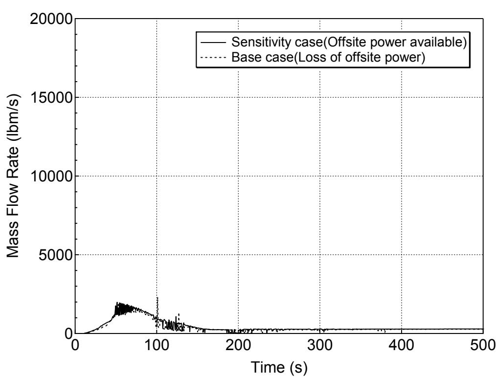
**Figure 5.6.2-17 Vapor Discharge through the Break for 1-ft<sup>2</sup> Break (Top)
