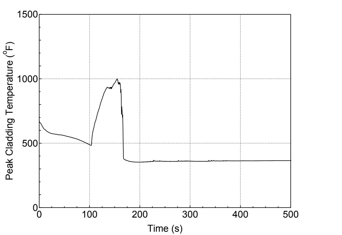
**Figure 5.3.2.b-8 PCT at All Elevations for Hot Rod in Hot Assembly
