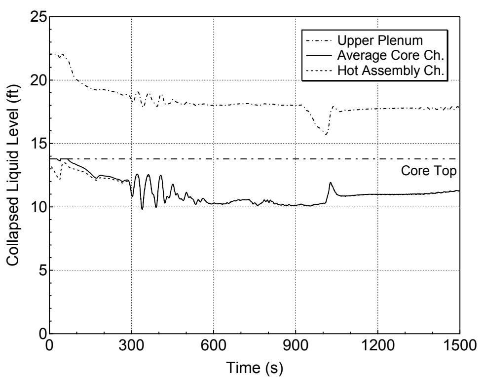
**Figure 5.2.c-7 Core and Upper Plenum Collapsed Levels for 3-inch Break (Bottom)
