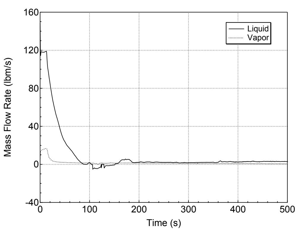
**Figure 5.3.1.c-9 Hot Assembly Exit Vapor and Liquid Mass Flowrates
