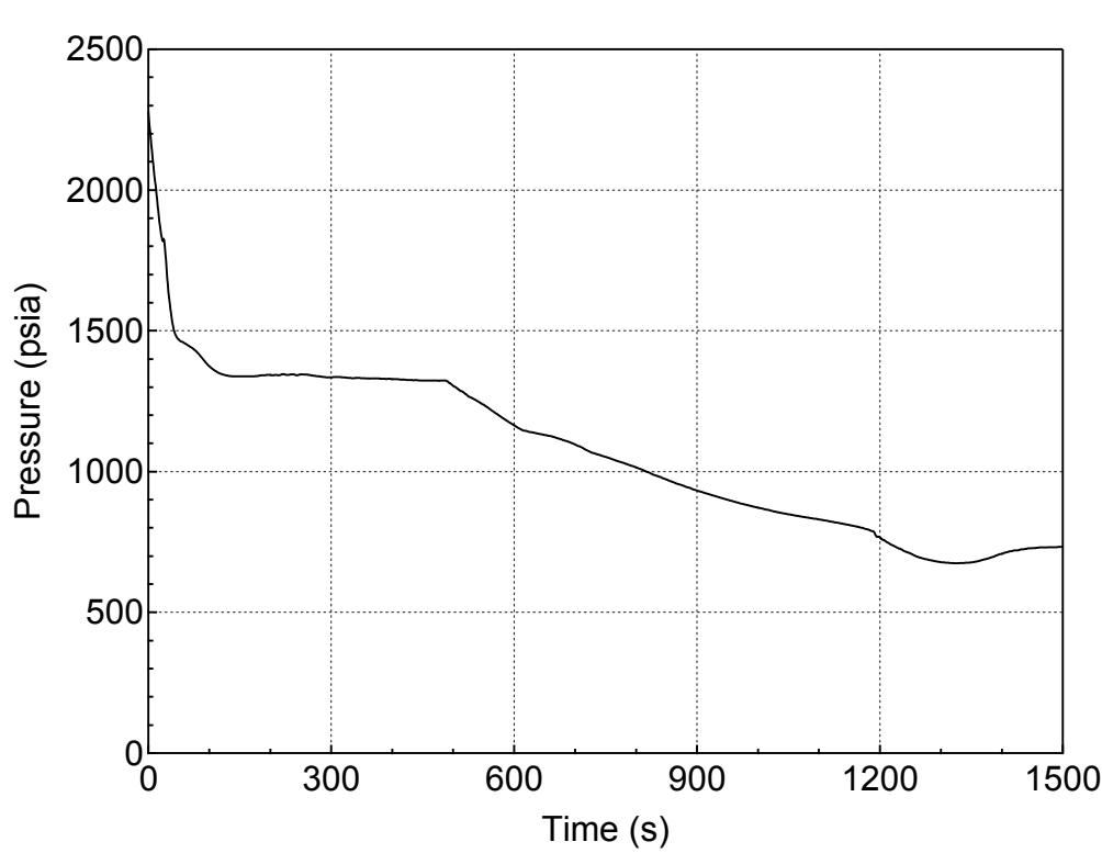
**Figure 5.2.d-1 RCS (Pressurizer) Pressure Transient for 4-inch Break (Bottom)
