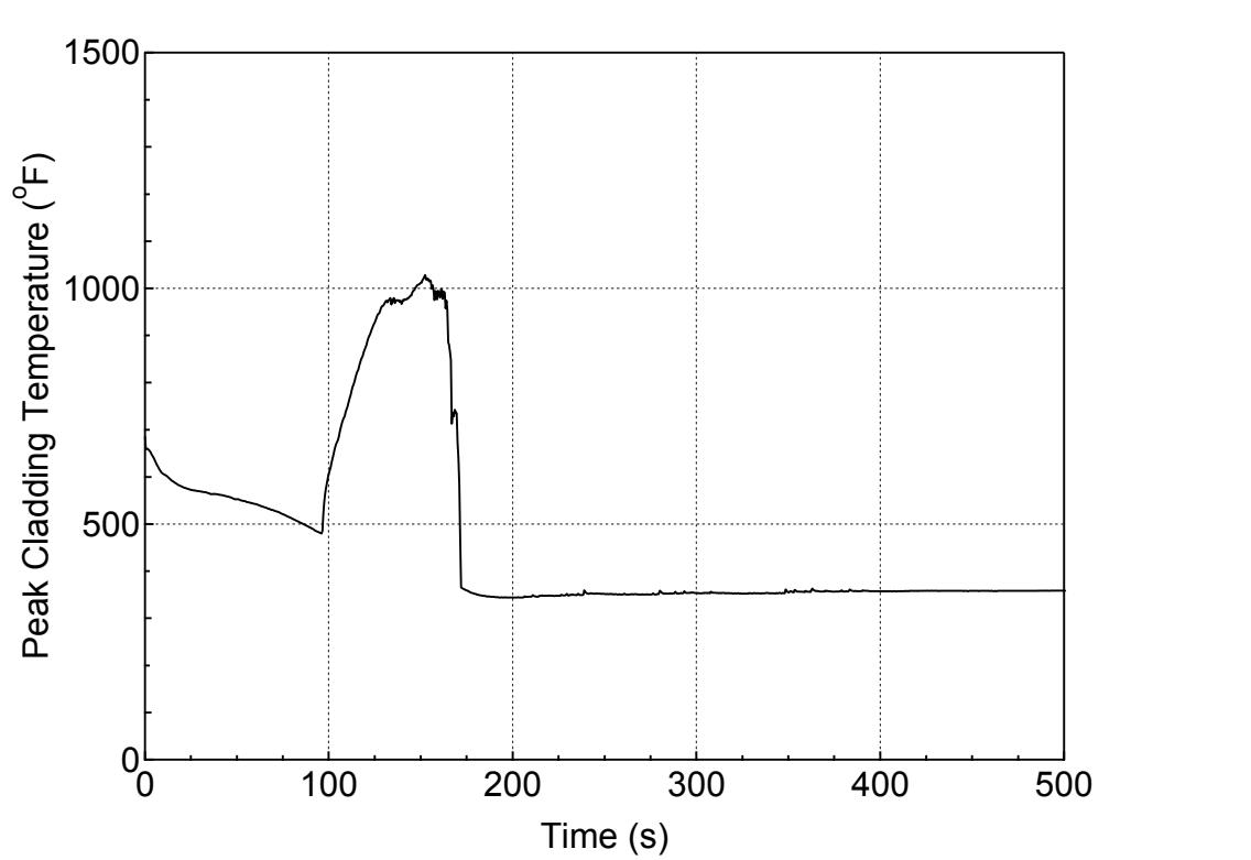
**Figure 5.2.n-8 PCT at All Elevations for Hot Rod in Hot Assembly
