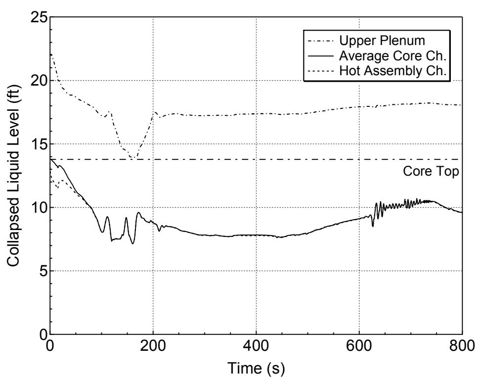
**Figure 5.3.1.b-25 Core and Upper Plenum Collapsed Levels for 6.5-inch Break (Side)
