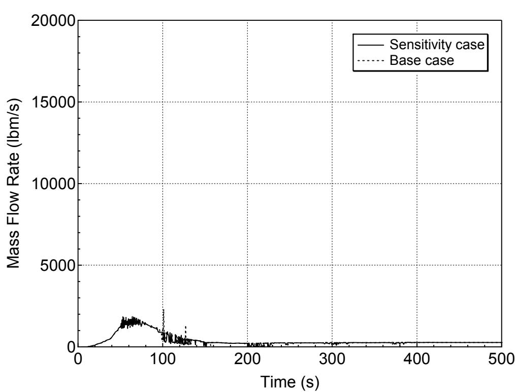
**Figure 5.5.b-4 Vapor Discharge through the Break for 1-ft<sup>2</sup> Break (Top)
