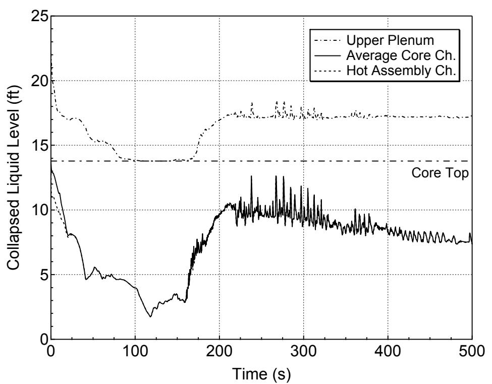
**Figure 5.3.2.b-16 Core and Upper Plenum Collapsed Levels for 13-inch Break (Side)
