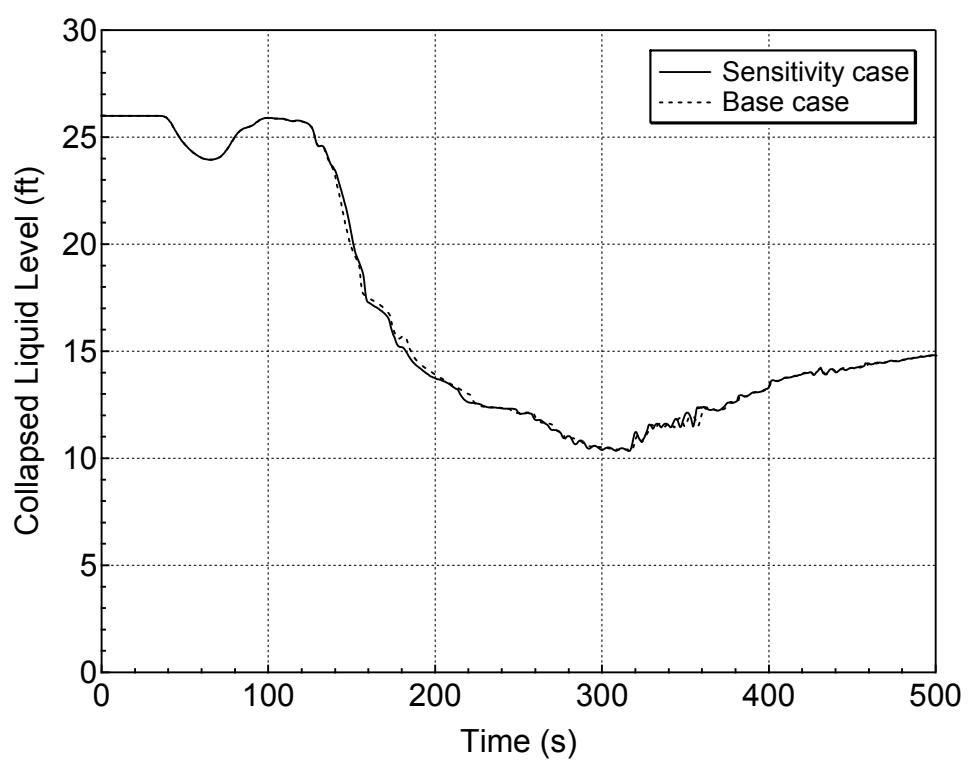
**Figure 5.4.1-8 Downcomer Collapsed Level for 7.5-inch Break (Top)
