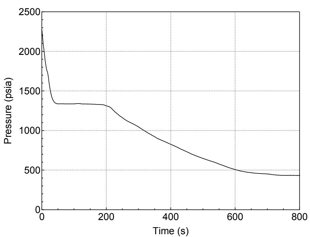
**Figure 5.3.1.a-10 RCS (Pressurizer) Pressure Transient for 6-inch Break (Side)
