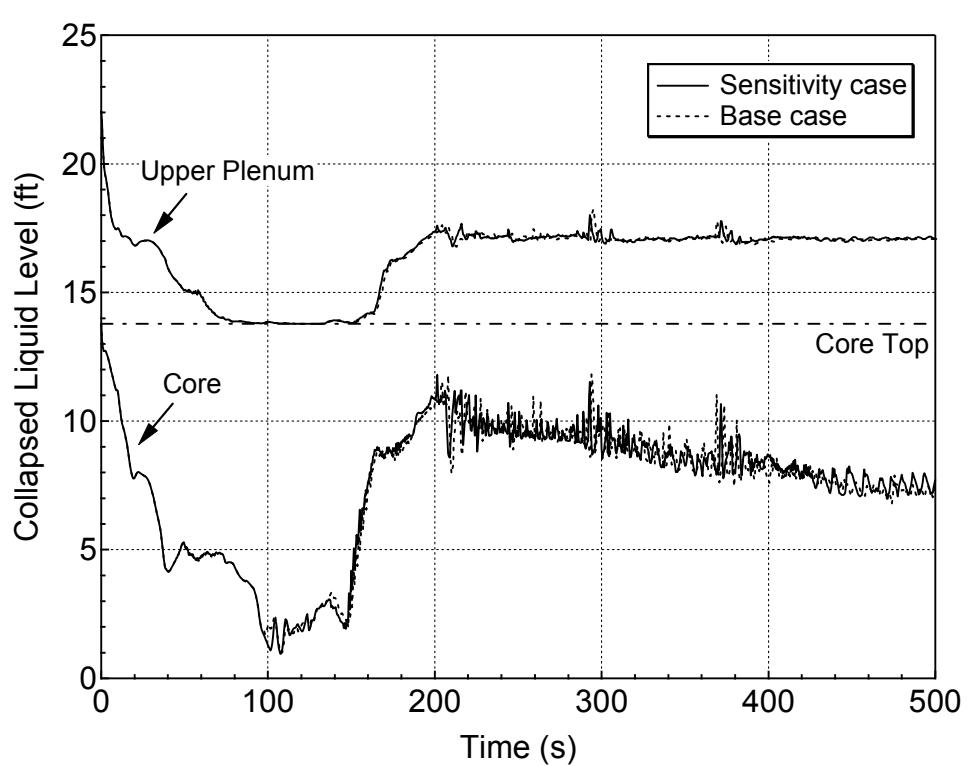
**Figure 5.5.b-9 Average Core and Upper Plenum Collapsed Levels for 1-ft<sup>2</sup> Break (Top)
