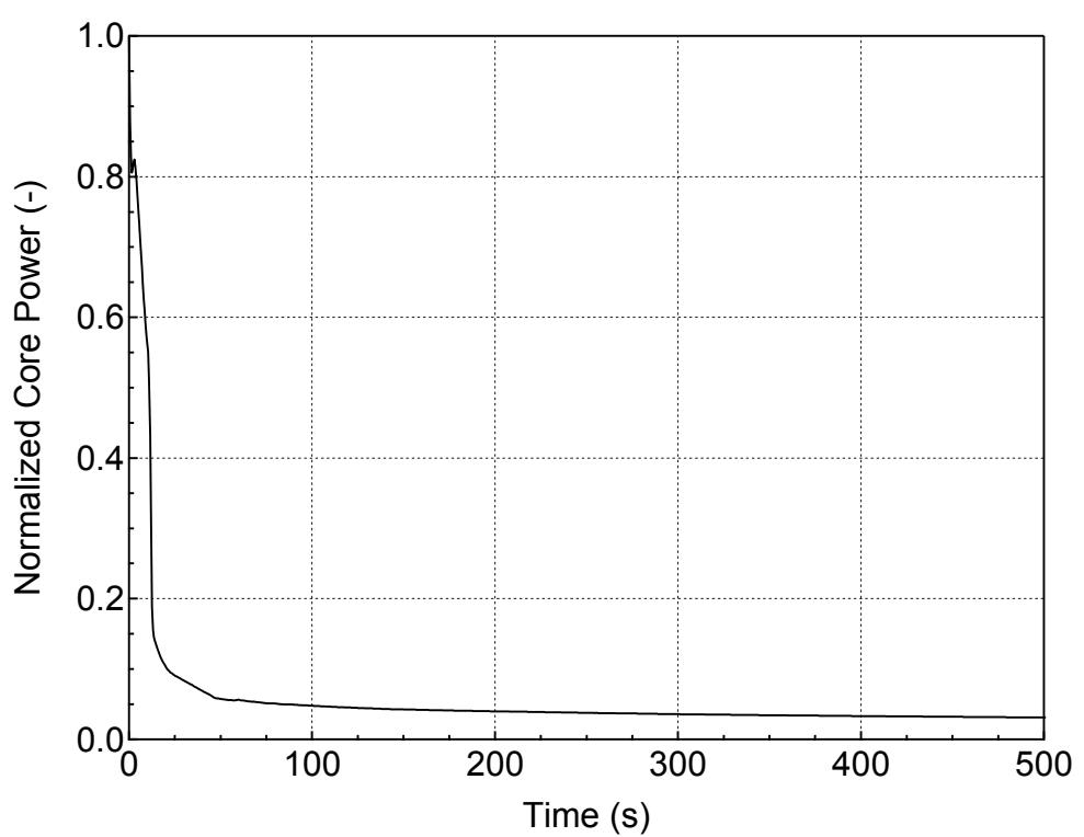
**Figure 5.3.2.a-20 Normalized Core Power for 12-inch Break (Homogeneous)
