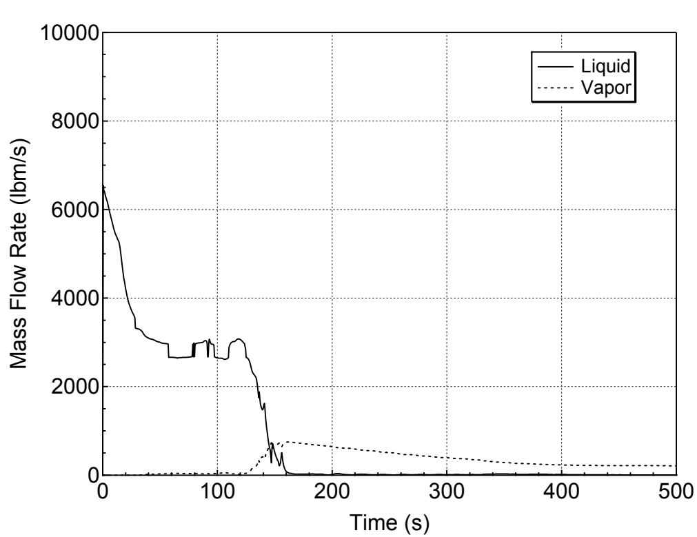
**Figure 5.3.1.d-12 Liquid and Vapor Discharges through the Break
