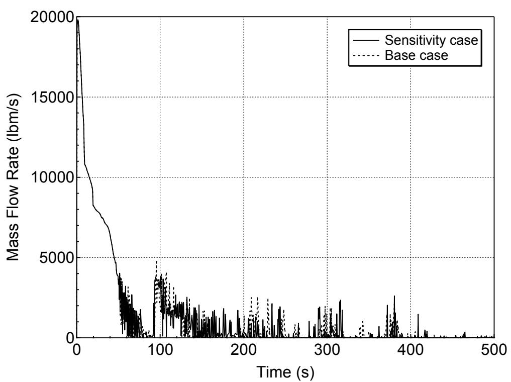
**Figure 5.4.3-16 Liquid Discharge through the Break for 1-ft<sup>2</sup> Break (Top)
