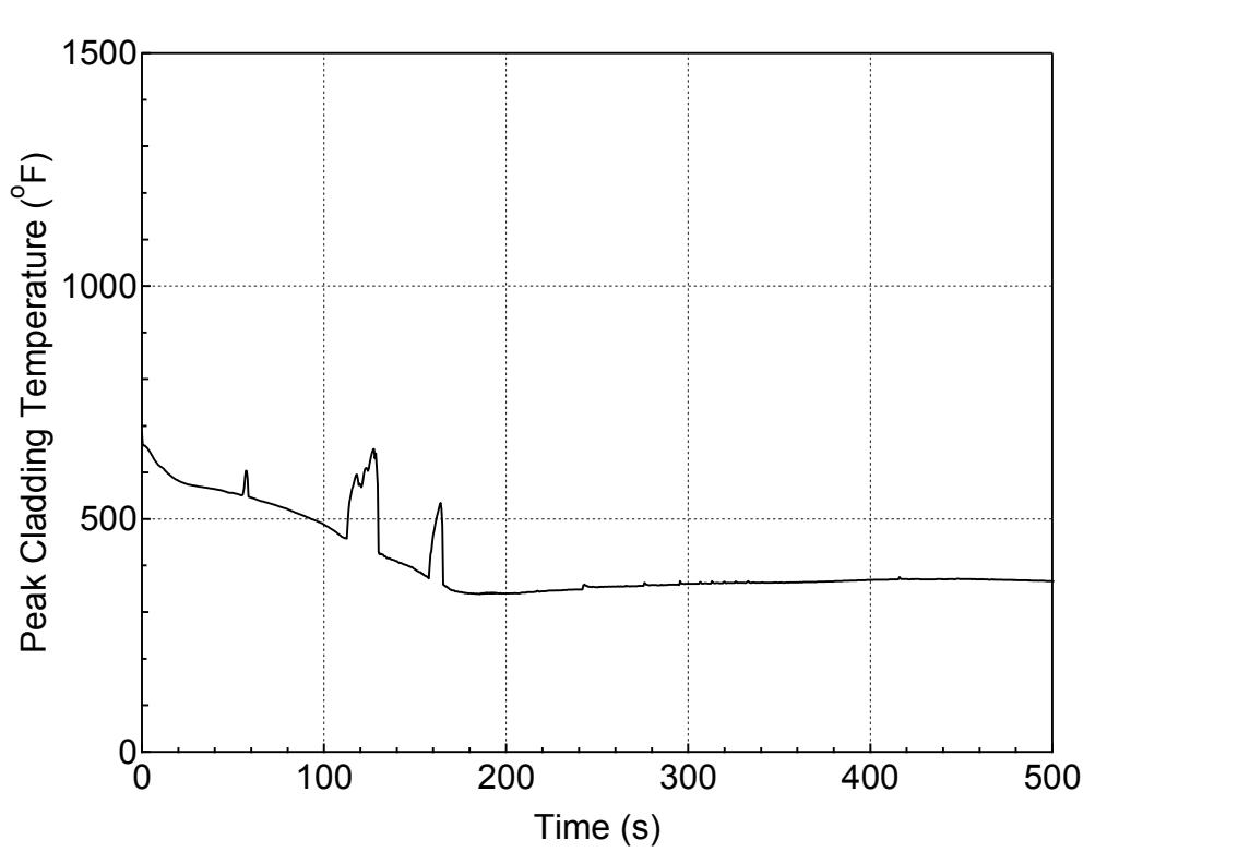
**Figure 5.1.1.c-17 PCT at All Elevations for Hot Rod in Hot Assembly
