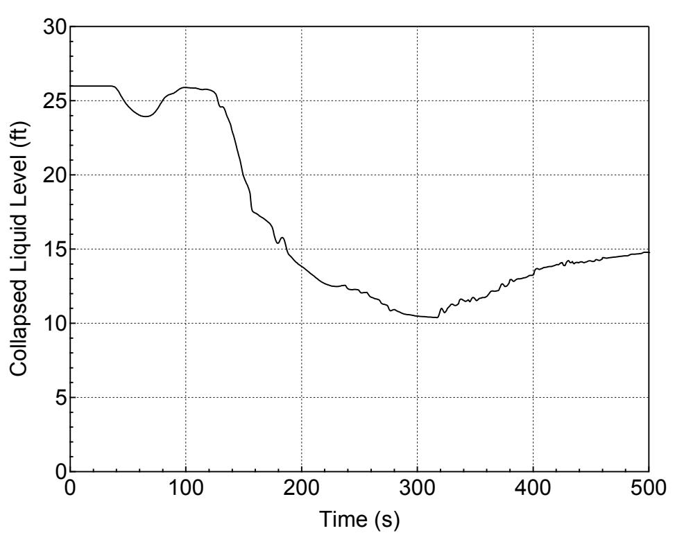
**Figure 5.3.1.d-24 Downcomer Collapsed Level for 7.5-inch Break (Side)
