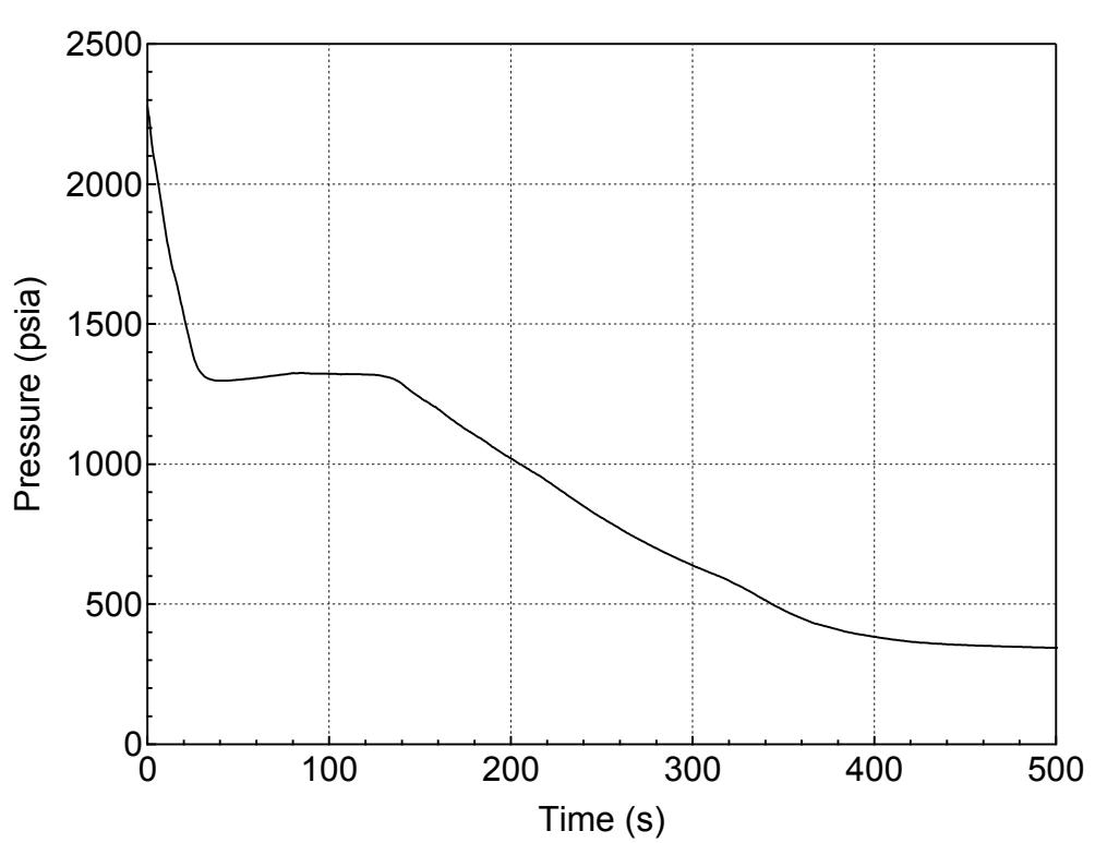
**Figure 5.3.1.d-1 RCS (Pressurizer) Pressure Transient for 7.5-inch Break (Bottom)
