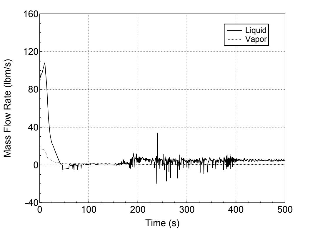
**Figure 5.3.2.a-18 Hot Assembly Exit Vapor and Liquid Mass Flowrates
