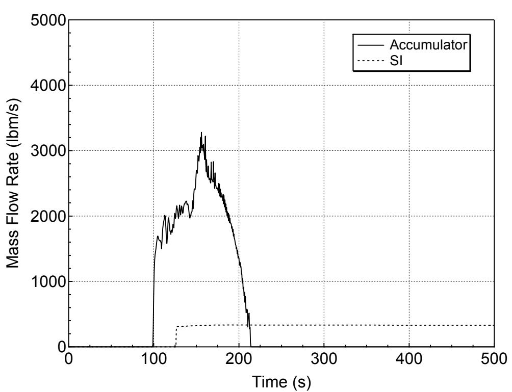
**Figure 5.2.m-4 Accumulator and Safety Injection Mass Flowrates
