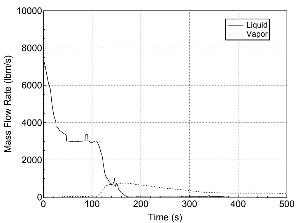
**Figure 5.3.1.e-21 Liquid and Vapor Discharges through the Break
