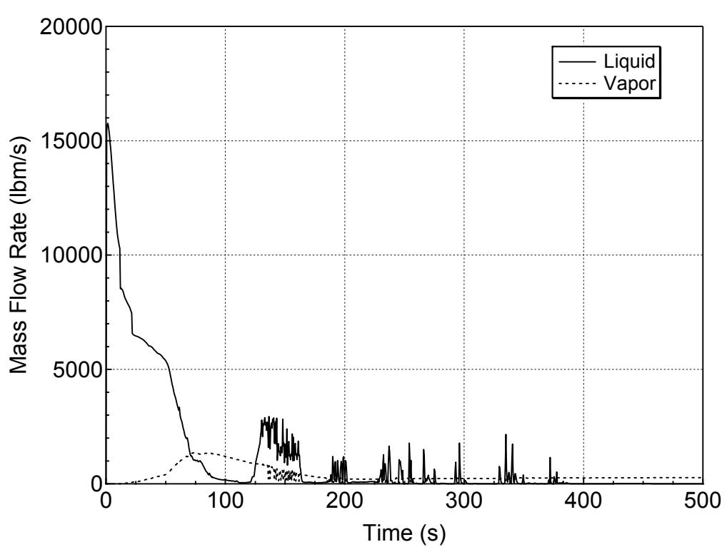
**Figure 5.3.2.a-21 Liquid and Vapor Discharges through the Break
