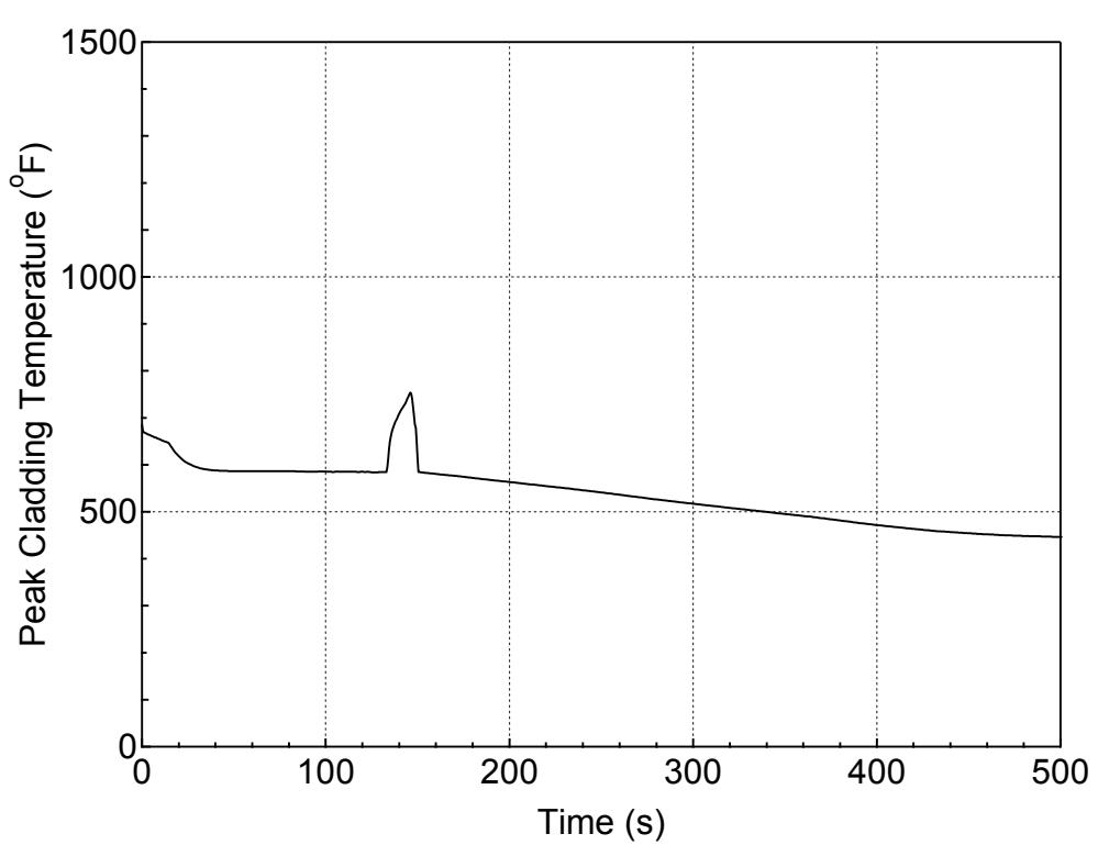
**Figure 5.3.1.c-26 PCT at All Elevations for Hot Rod in Hot Assembly
