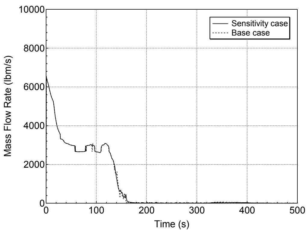
**Figure 5.4.1-3 Liquid Discharge through the Break for 7.5-inch Break (Top)
