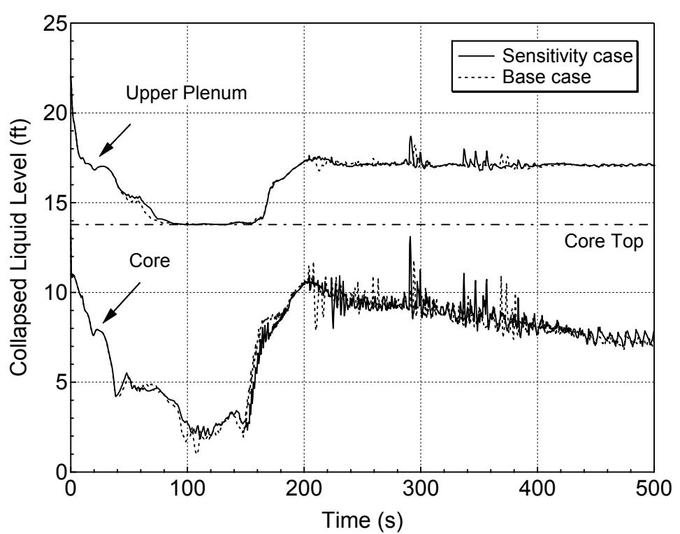
**Figure 5.4.1-23 Hot Assembly Core and Upper Plenum Collapsed Levels
