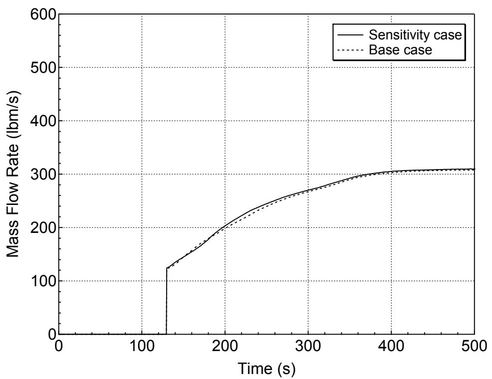
**Figure 5.4.2-6 Safety Injection Mass Flowrate for 7.5-inch Break (Top)
