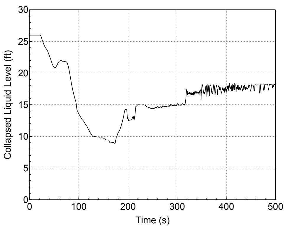
**Figure 5.2.j-6 Downcomer Collapsed Level for 10-inch Break (Bottom)
