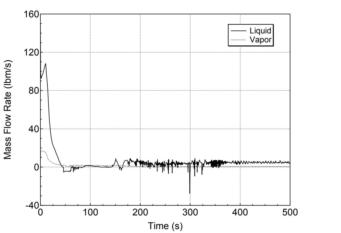
**Figure 5.3.2.a-9 Hot Assembly Exit Vapor and Liquid Mass Flowrates
