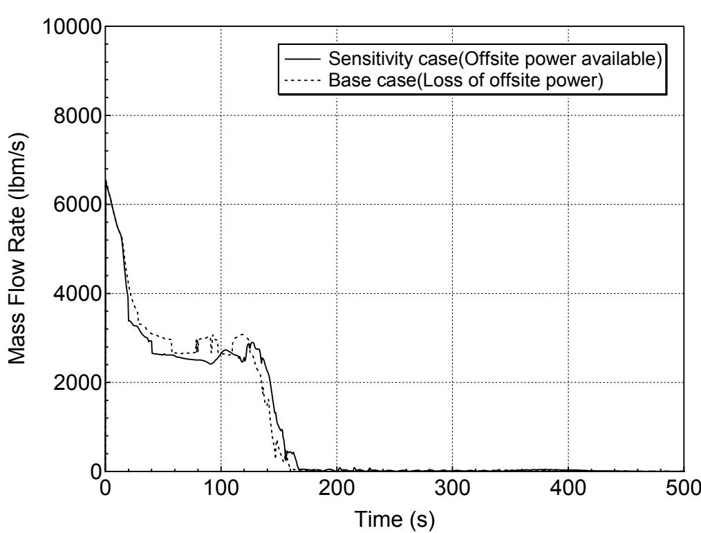
**Figure 5.6.2-3 Liquid Discharge through the Break for 7.5-inch Break (Top)
