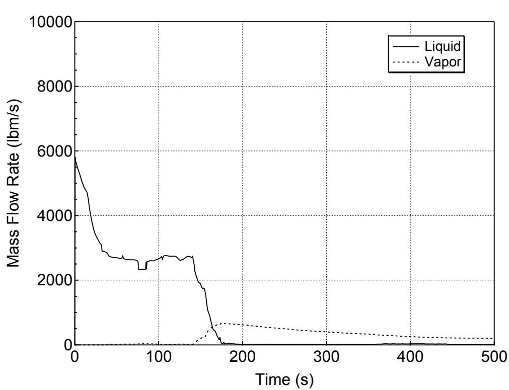
**Figure 5.2.g-3 Liquid and Vapor Discharges through the Break
