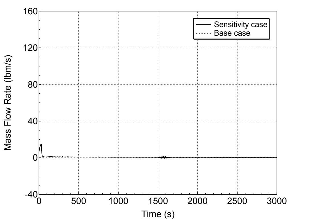
**Figure 5.5.c-13 Hot Assembly Exit Vapor Mass Flowrate for DVI-line Break
