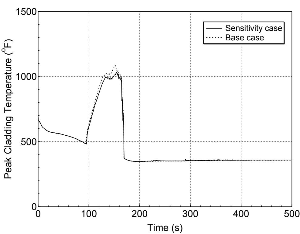
**Figure 5.4.1-24 PCT at All Elevations for Hot Rod in Hot Assembly for 1-ft<sup>2</sup> Break (Top)
