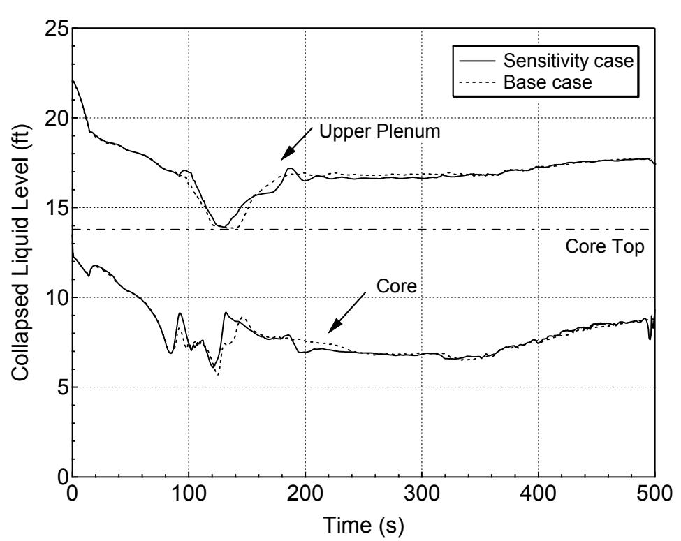
**Figure 5.4.2-10 Hot Assembly Core and Upper Plenum Collapsed Levels
