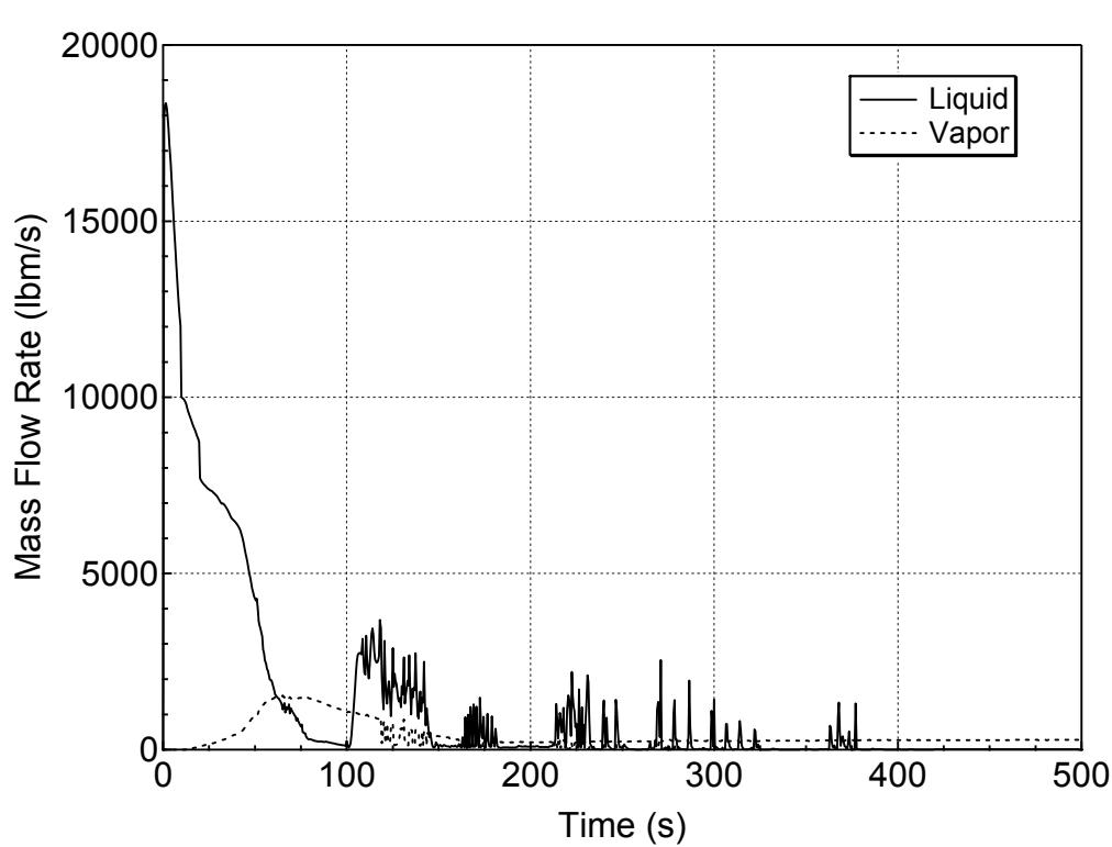
**Figure 5.3.2.b-12 Liquid and Vapor Discharges through the Break
