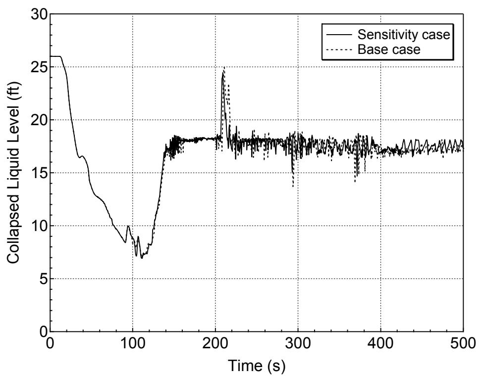
**Figure 5.5.b-8 Downcomer Collapsed Level for 1-ft<sup>2</sup> Break (Top)
