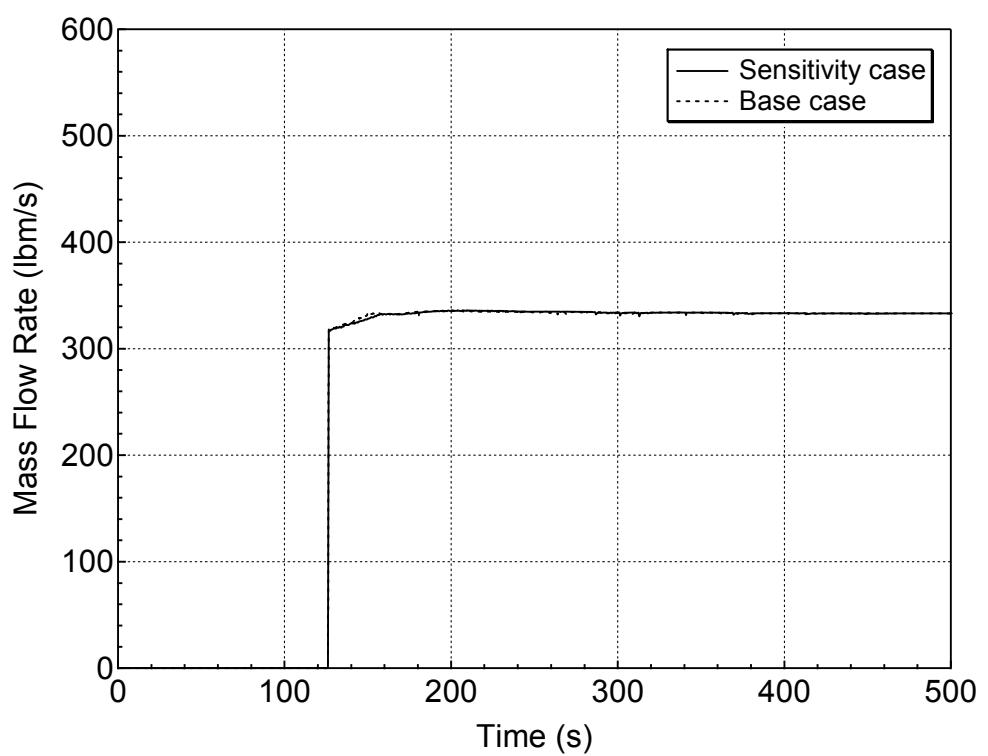
**Figure 5.4.3-19 Safety Injection Mass Flowrate for 1-ft<sup>2</sup> Break (Top)
