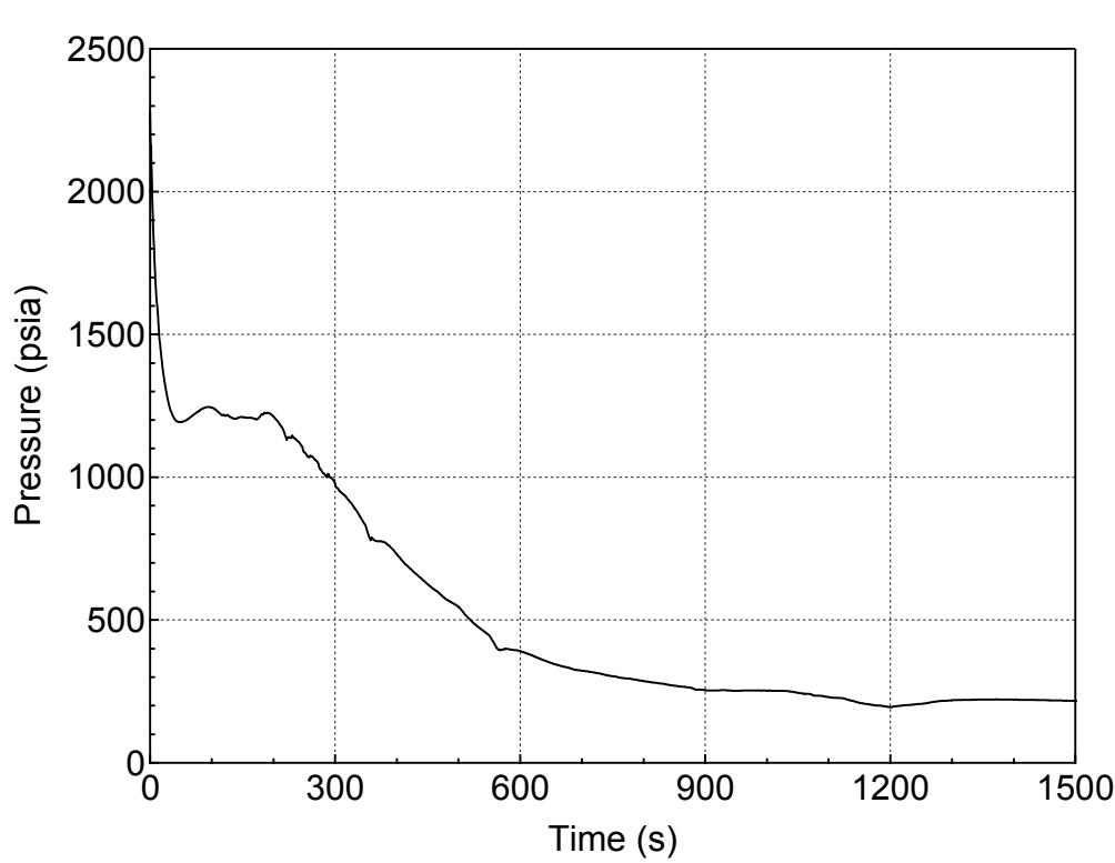
**Figure 5.1.3-1 RCS (Pressurizer) Pressure Transient
