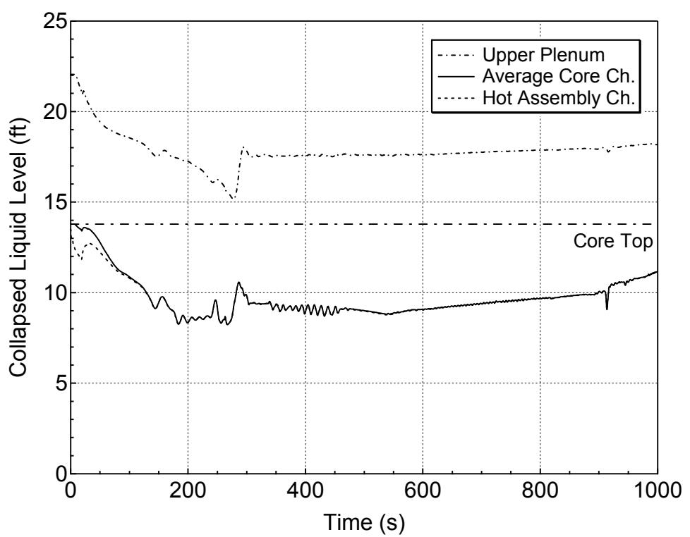
**Figure 5.2.e-7 Core and Upper Plenum Collapsed Levels for 5-inch Break (Bottom)
