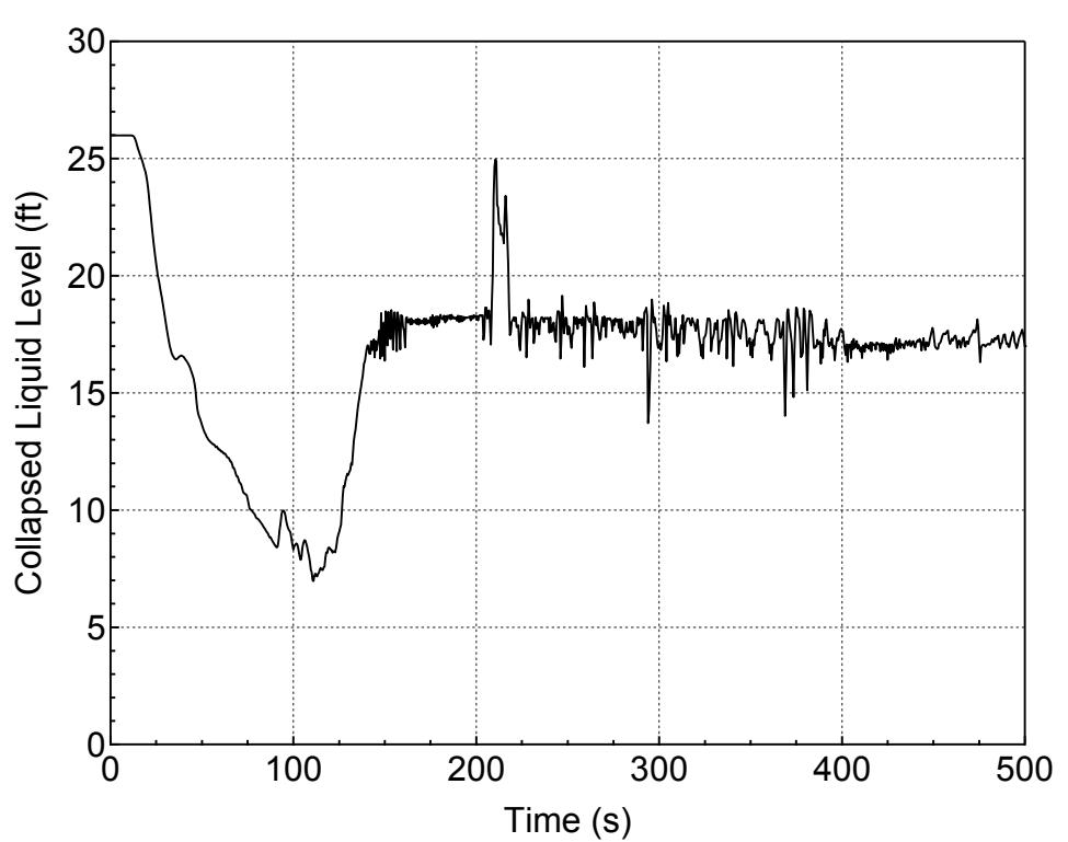
**Figure 5.3.2.c-6 Downcomer Collapsed Level for 1-ft<sup>2</sup> Break (Top)
