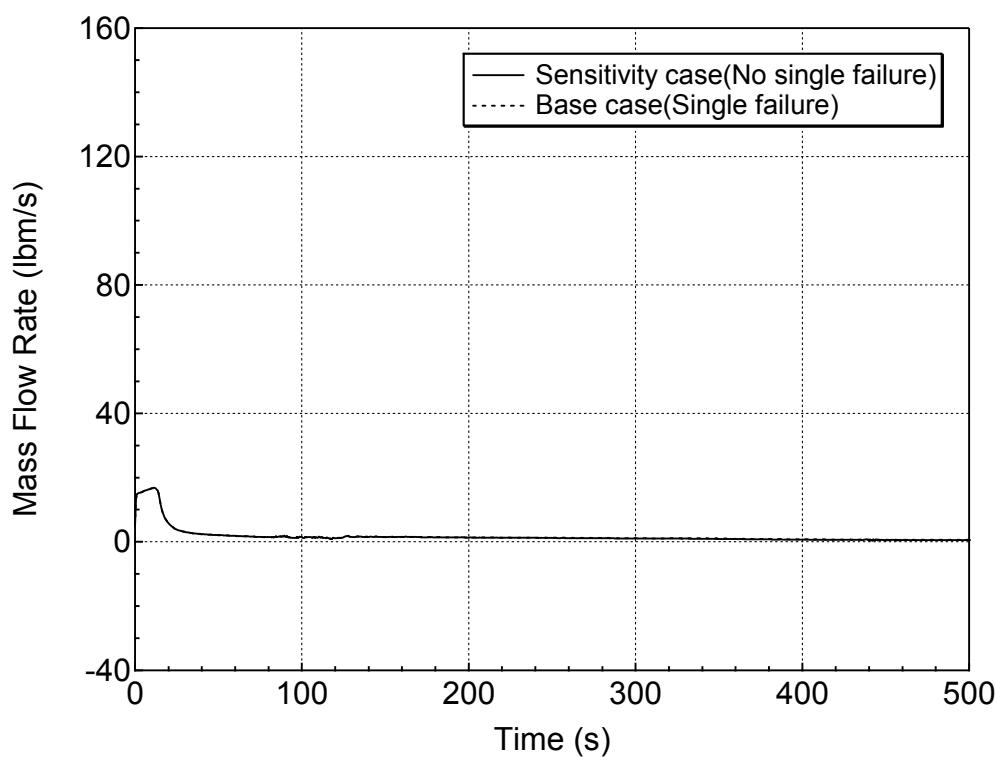
**Figure 5.6.1-13 Hot Assembly Exit Vapor Mass Flowrate for 7.5-inch Break (Top)
