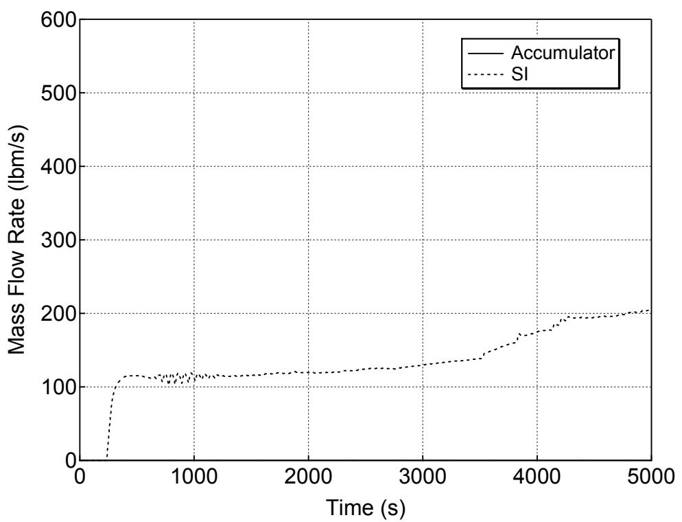
**Figure 5.1.1.a-4 Accumulator and Safety Injection Mass Flowrates
