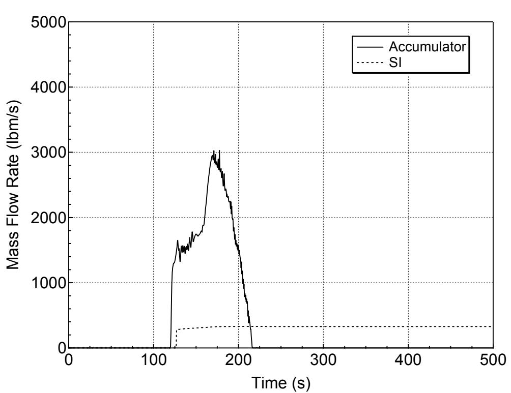
**Figure 5.2.I-4 Accumulator and Safety Injection Mass Flowrates
