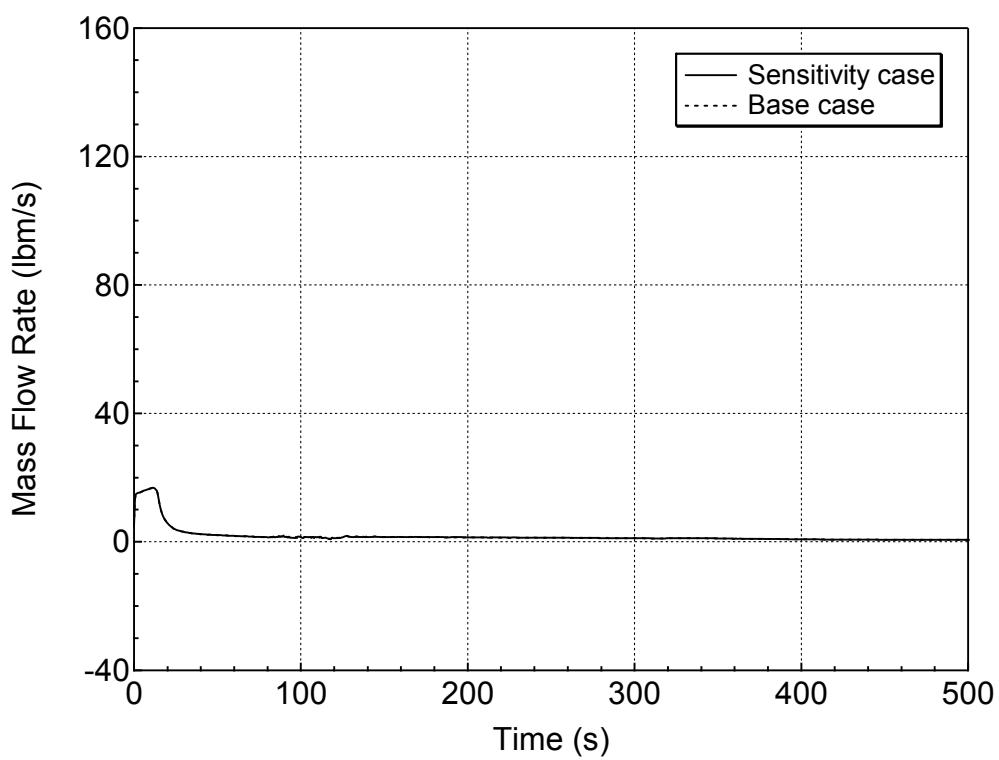
**Figure 5.4.3-13 Hot Assembly Exit Vapor Mass Flowrate for 7.5-inch Break (Top)
