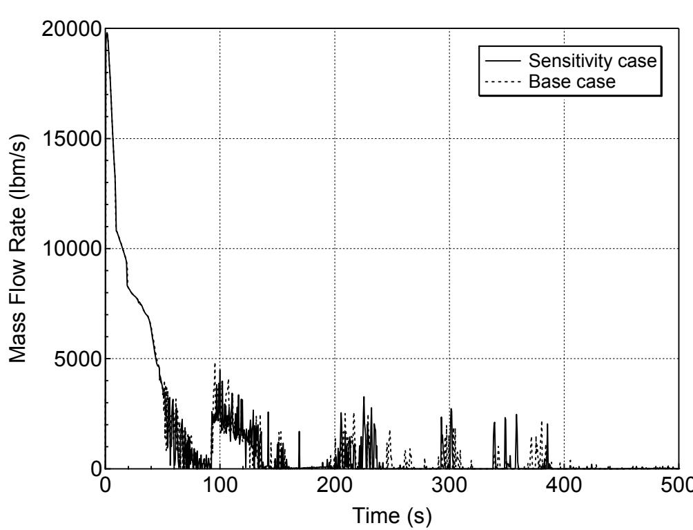
**Figure 5.4.1-16 Liquid Discharge through the Break for 1-ft<sup>2</sup> Break (Top)
