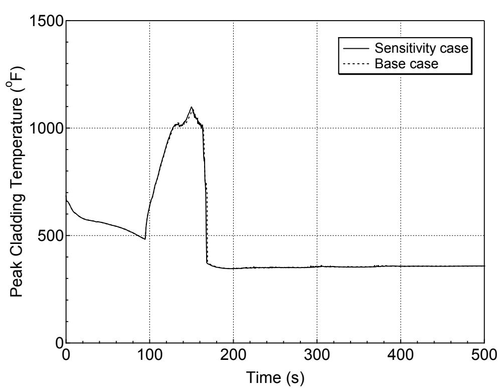
**Figure 5.5.b-11 PCT at All Elevations for Hot Rod in Hot Assembly for 1-ft<sup>2</sup> Break (Top)
