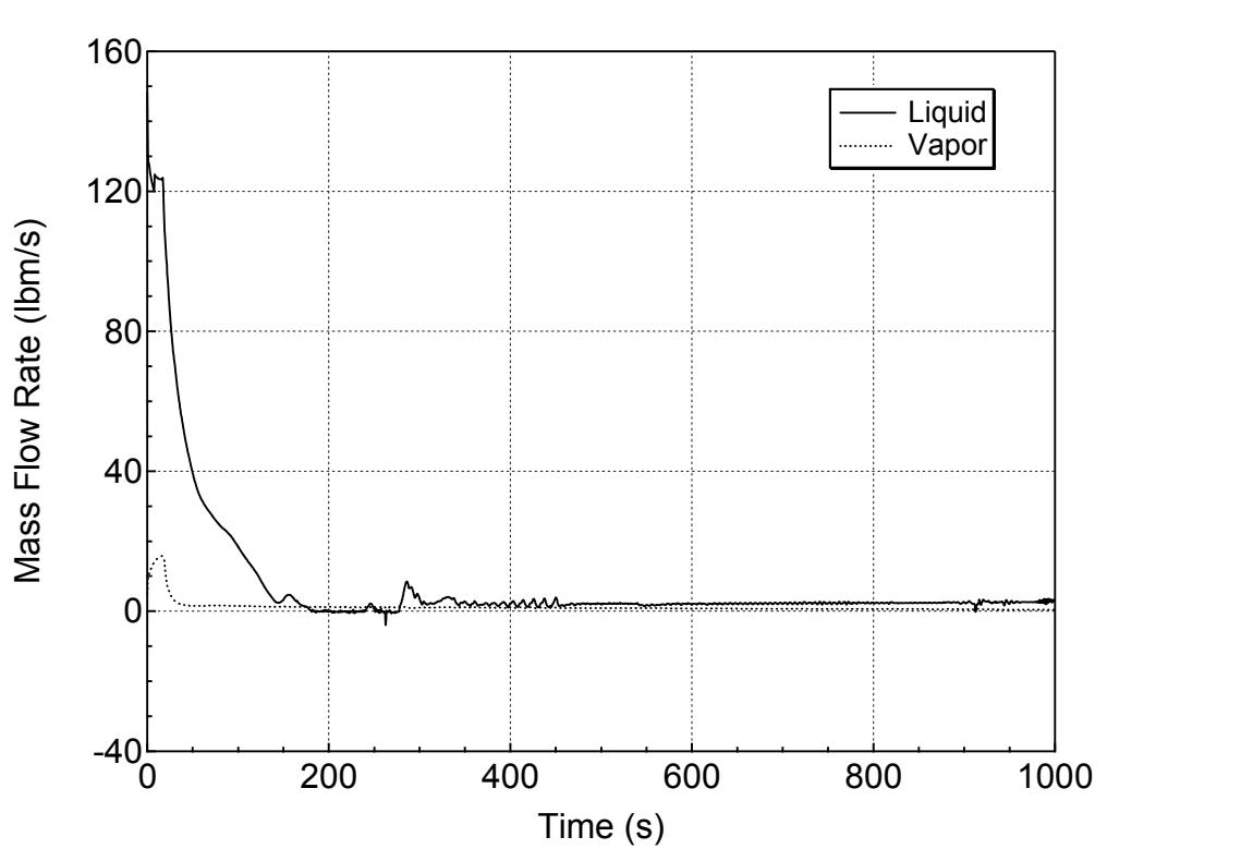
**Figure 5.2.e-9 Hot Assembly Exit Vapor and Liquid Mass Flowrates
