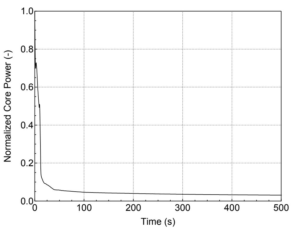
**Figure 5.1.1.a-11 Normalized Core Power for 1-ft<sup>2</sup> Break (Bottom)
