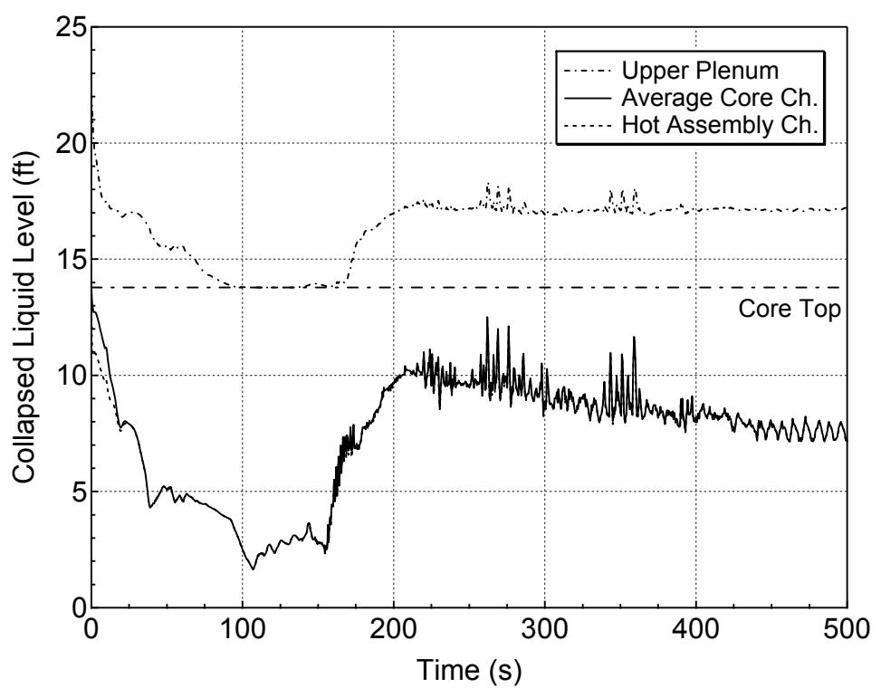
**Figure 5.3.2.c-16 Core and Upper Plenum Collapsed Levels for 1-ft<sup>2</sup> Break (Side)
