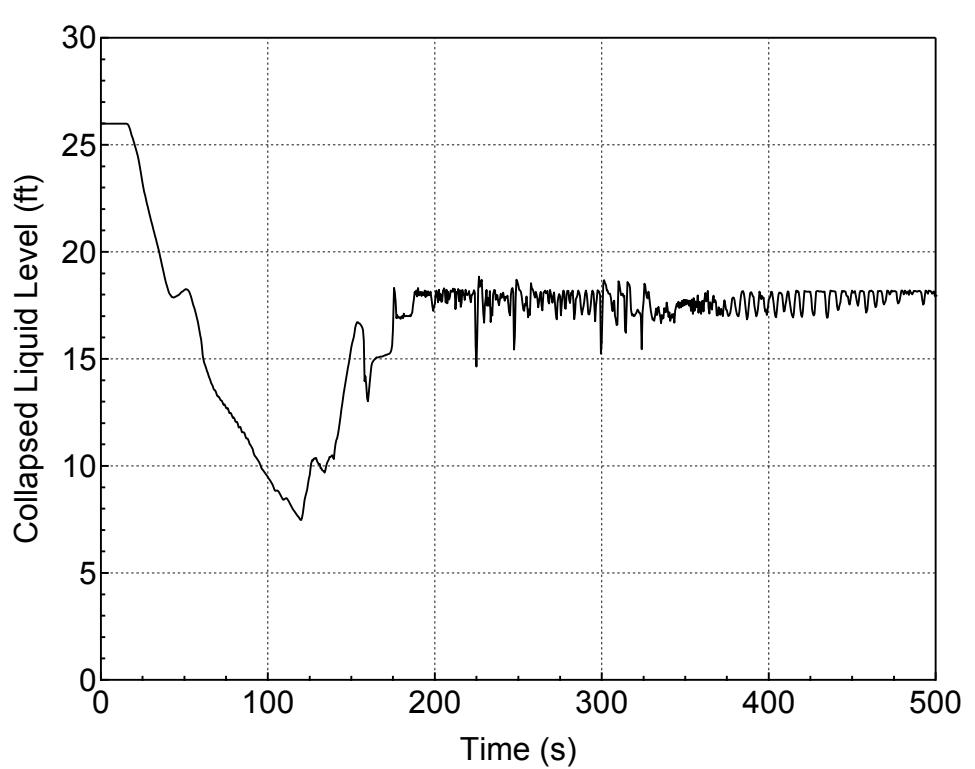
**Figure 5.3.2.a-6 Downcomer Collapsed Level for 12-inch Break (Top)
