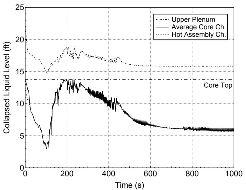
**Figure 5.1.1.b-16 Core and Upper Plenum Collapsed Levels for 1-ft<sup>2</sup> Break (Bottom)
