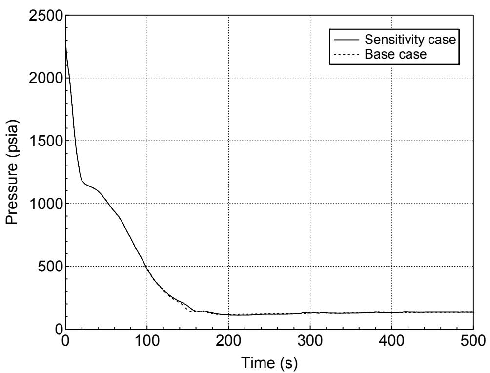
**Figure 5.4.3-14 RCS (Pressurizer) Pressure Transient for 1-ft<sup>2</sup> Break (Top)
