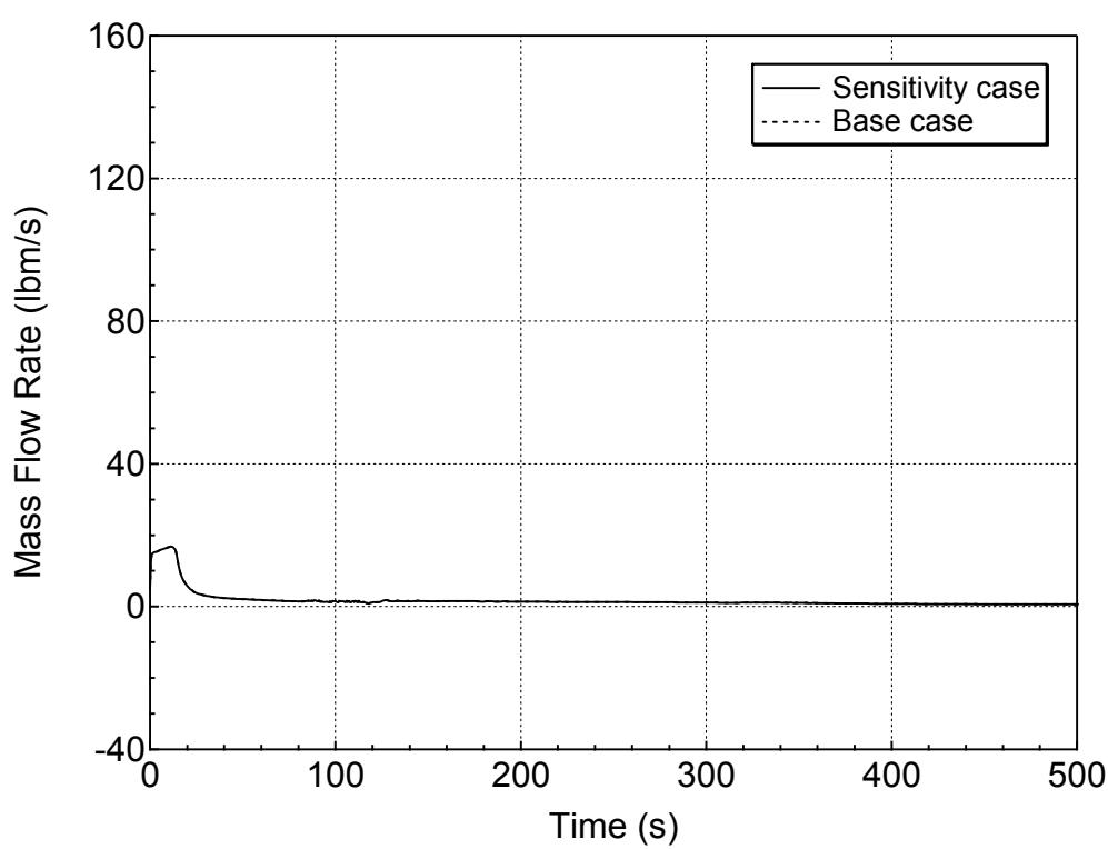
**Figure 5.4.1-13 Hot Assembly Exit Vapor Mass Flowrate for 7.5-inch Break (Top)
