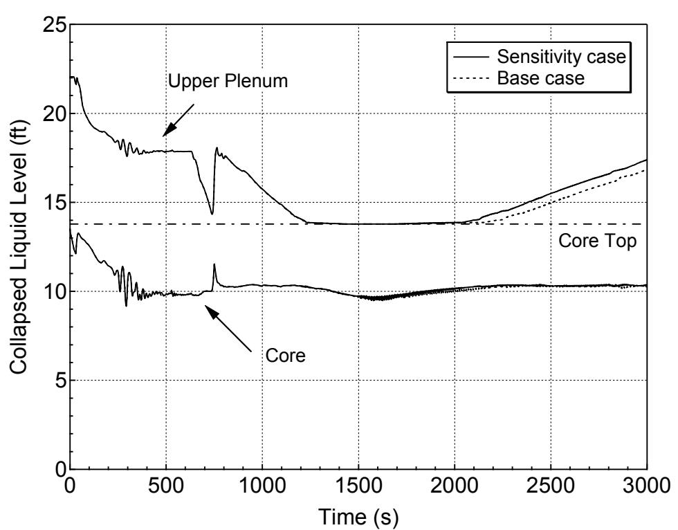
**Figure 5.5.c-10 Hot Assembly Core and Upper Plenum Collapsed Levels
