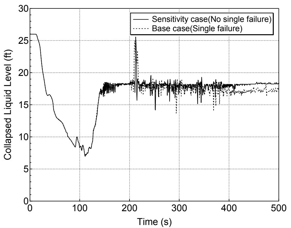
**Figure 5.6.1-21 Downcomer Collapsed Level for 1-ft<sup>2</sup> Break (Top)
