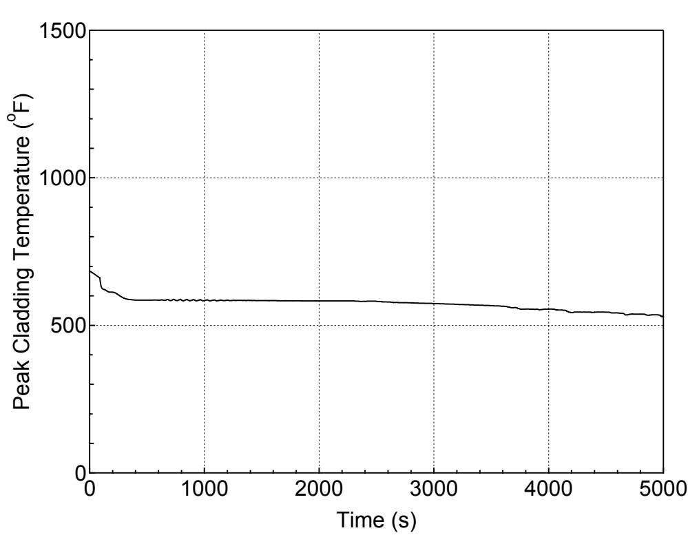
**Figure 5.1.1.c-8 PCT at All Elevations for Hot Rod in Hot Assembly
