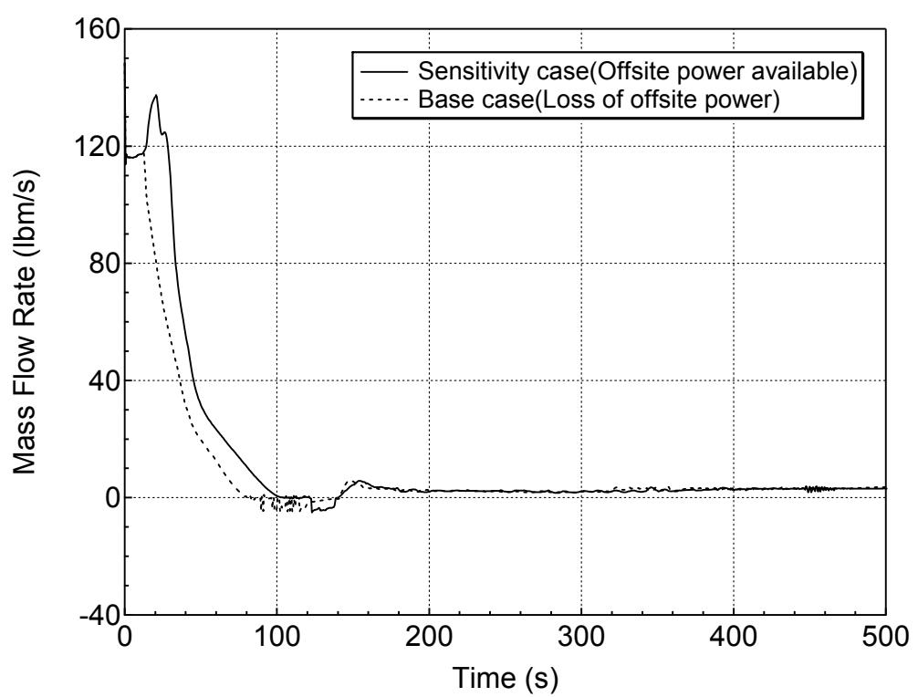
**Figure 5.6.2-12 Hot Assembly Exit Liquid Mass Flowrate for 7.5-inch Break (Top)
