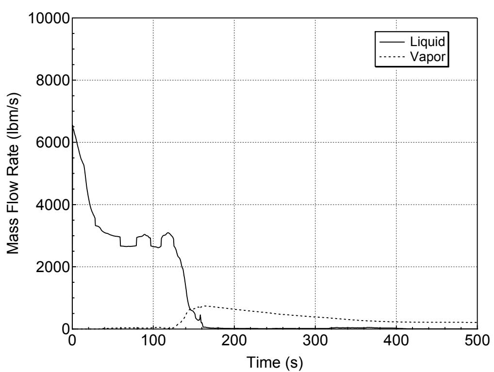
**Figure 5.3.1.d-30 Liquid and Vapor Discharges through the Break
