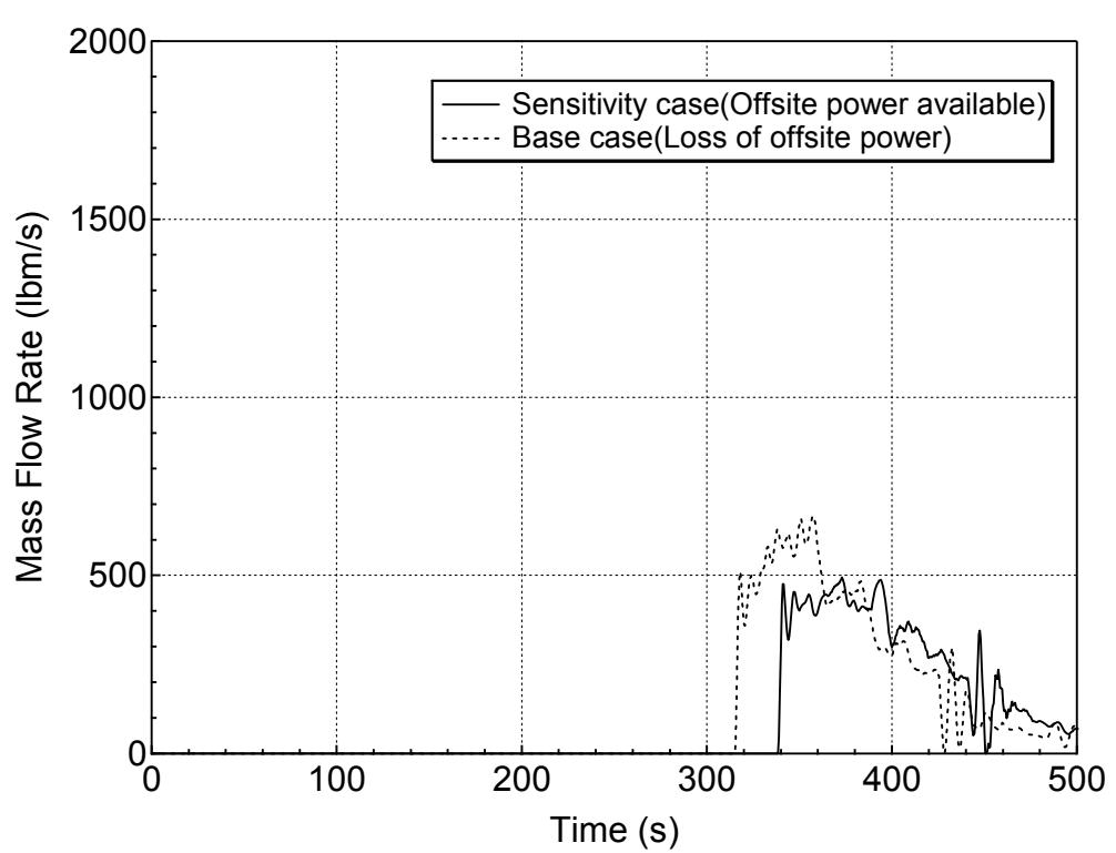
**Figure 5.6.2-5 Accumulator Mass Flowrate for 7.5-inch Break (Top)
