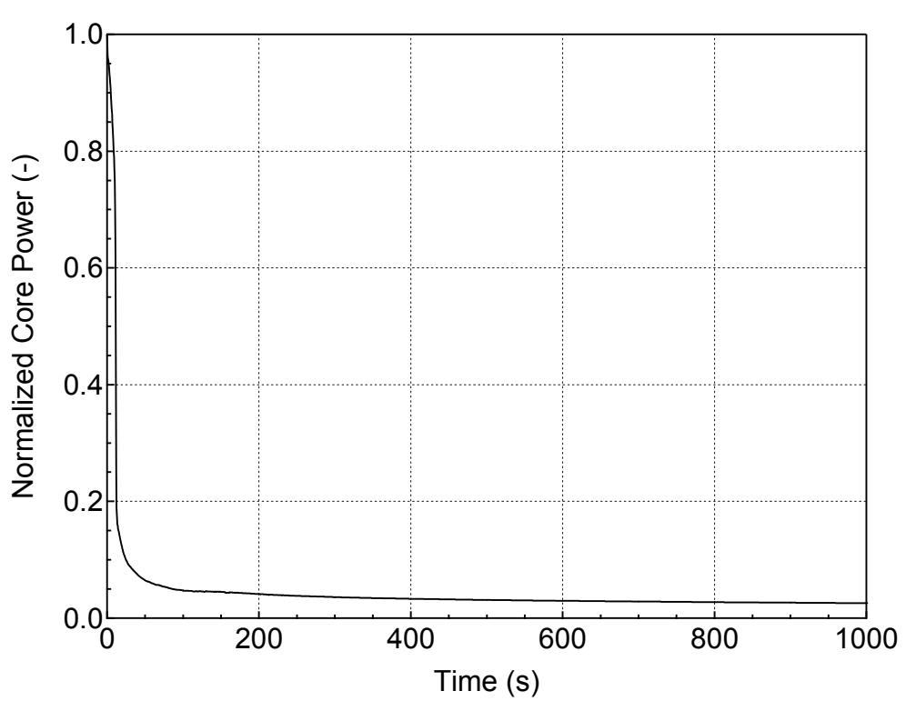
**Figure 5.1.1.b-11 Normalized Core Power for 1-ft<sup>2</sup> Break (Bottom)
