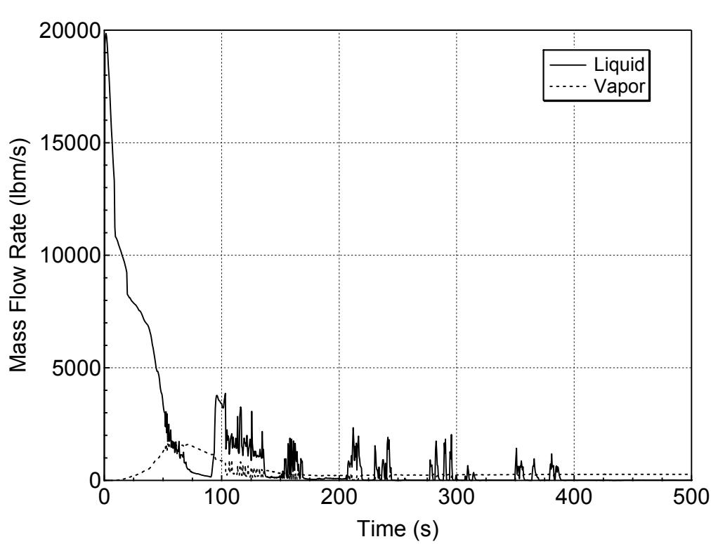
**Figure 5.2.n-3 Liquid and Vapor Discharges through the Break for 1-ft<sup>2</sup> Break (Bottom) (Spectrum Analysis)**
