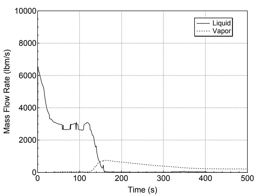
**Figure 5.3.1.d-21 Liquid and Vapor Discharges through the Break
