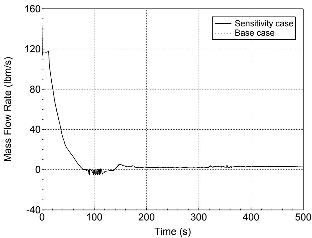
**Figure 5.4.1-12 Hot Assembly Exit Liquid Mass Flowrate for 7.5-inch Break (Top)
