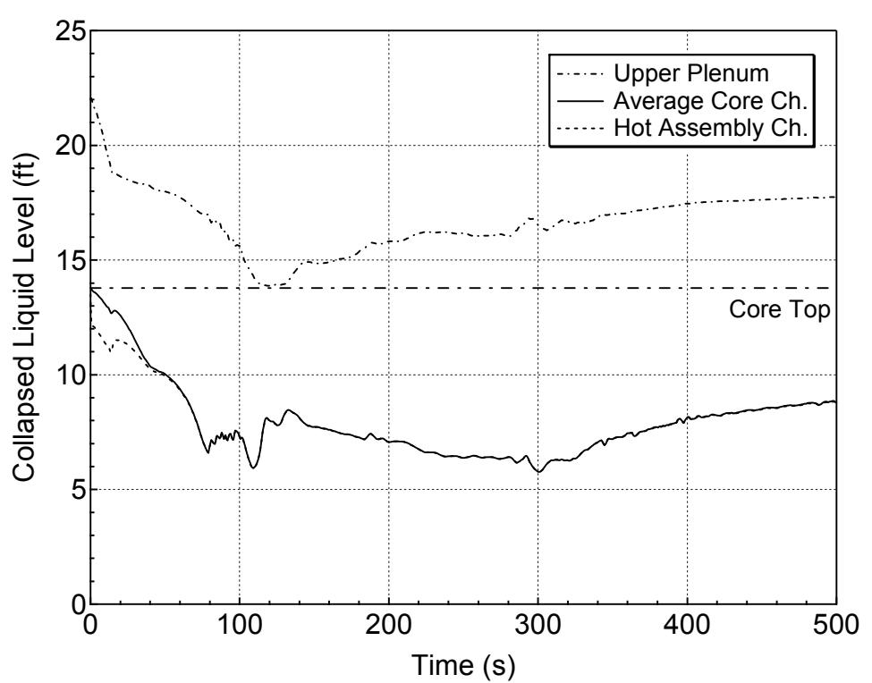
**Figure 5.3.1.e-7 Core and Upper Plenum Collapsed Levels for 8-inch Break (Top)
