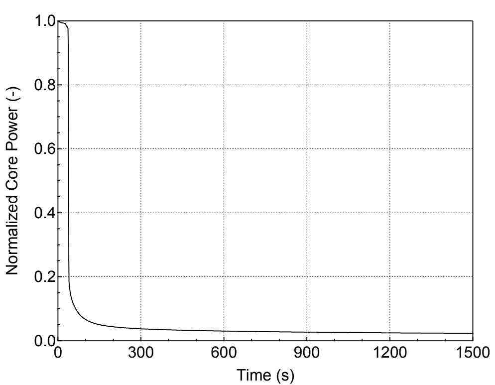
**Figure 5.2.c-2 Normalized Core Power for 3-inch Break (Bottom)
