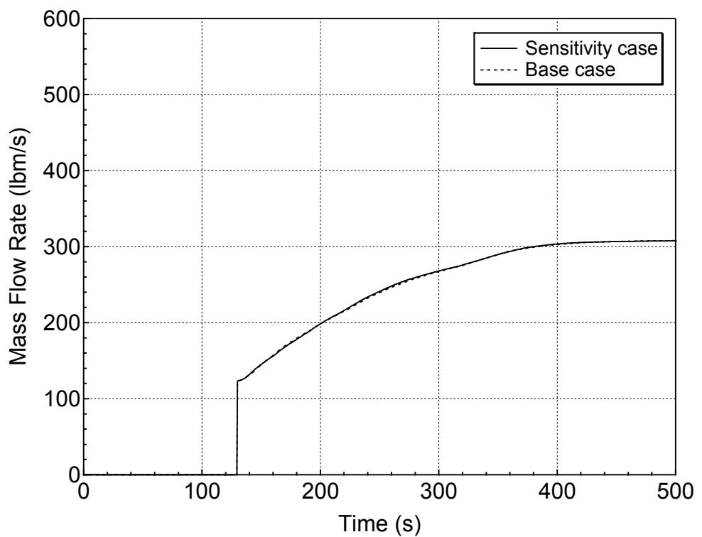
**Figure 5.4.3-6 Safety Injection Mass Flowrate for 7.5-inch Break (Top)
