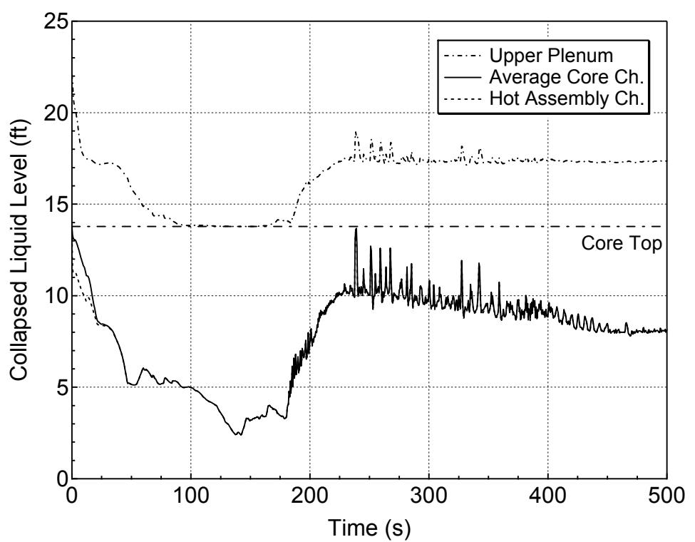
**Figure 5.3.2.a-16 Core and Upper Plenum Collapsed Levels for 12-inch Break (Side)
