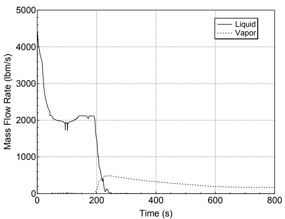
**Figure 5.3.1.a-3 Liquid and Vapor Discharges through the Break for 6-inch Break (Top)
