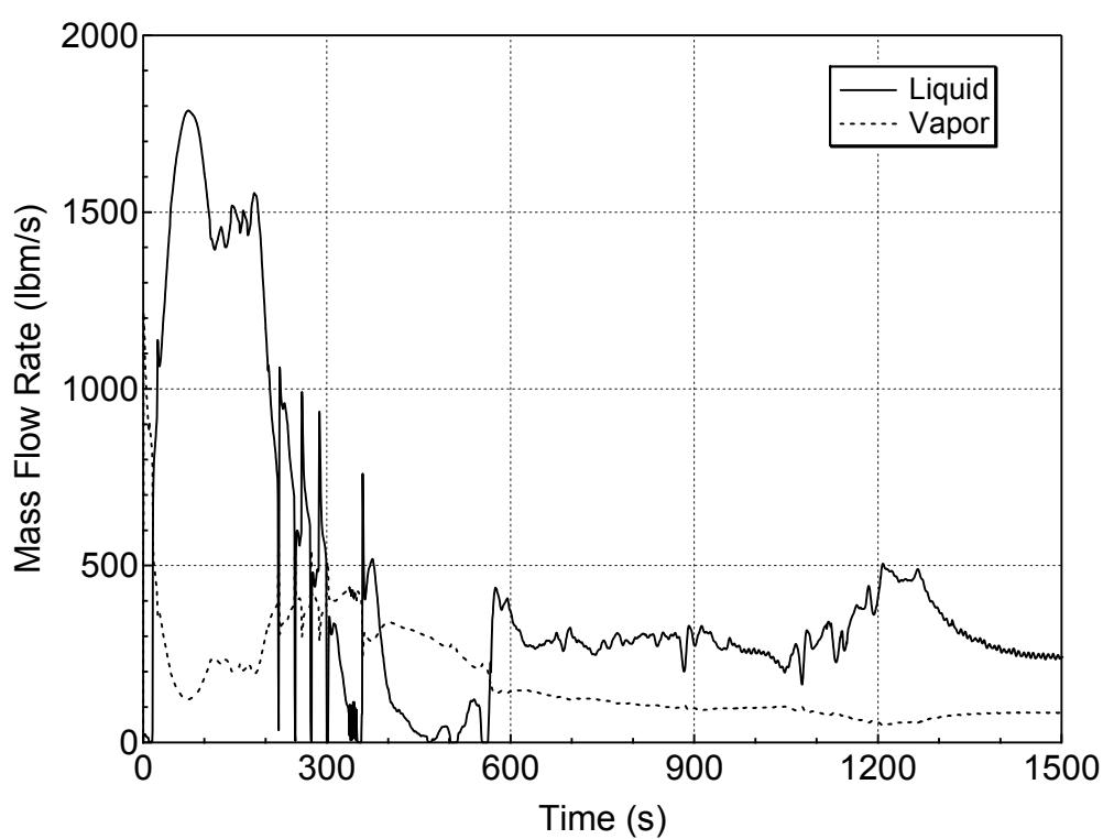
**Figure 5.1.3-3 Liquid and Vapor Discharges through the Break
