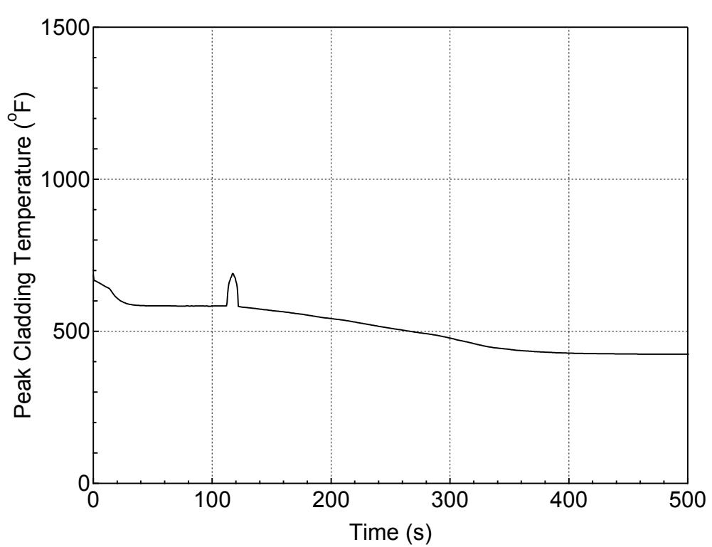
**Figure 5.3.1.e-26 PCT at All Elevations for Hot Rod in Hot Assembly
