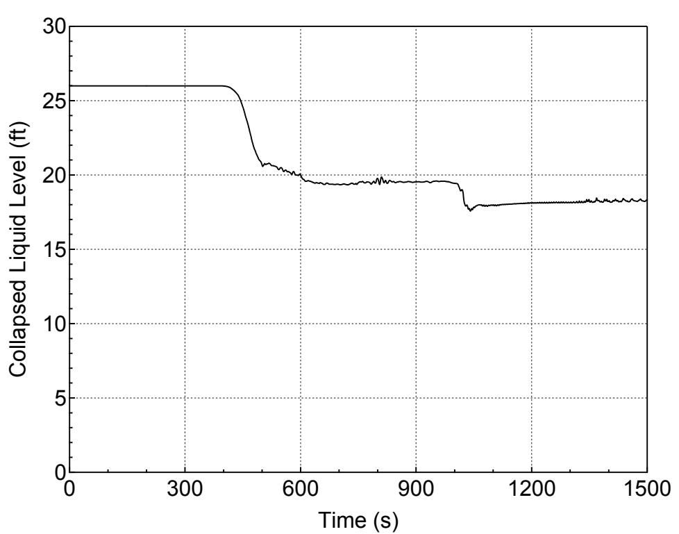
**Figure 5.2.c-6 Downcomer Collapsed Level for 3-inch Break (Bottom)
