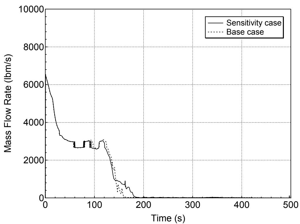
**Figure 5.4.2-3 Liquid Discharge through the Break for 7.5-inch Break (Top)
