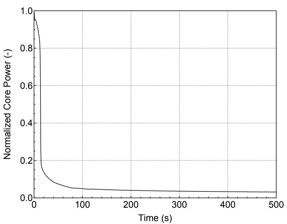
**Figure 5.3.1.e-11 Normalized Core Power for 8-inch Break (Side)
