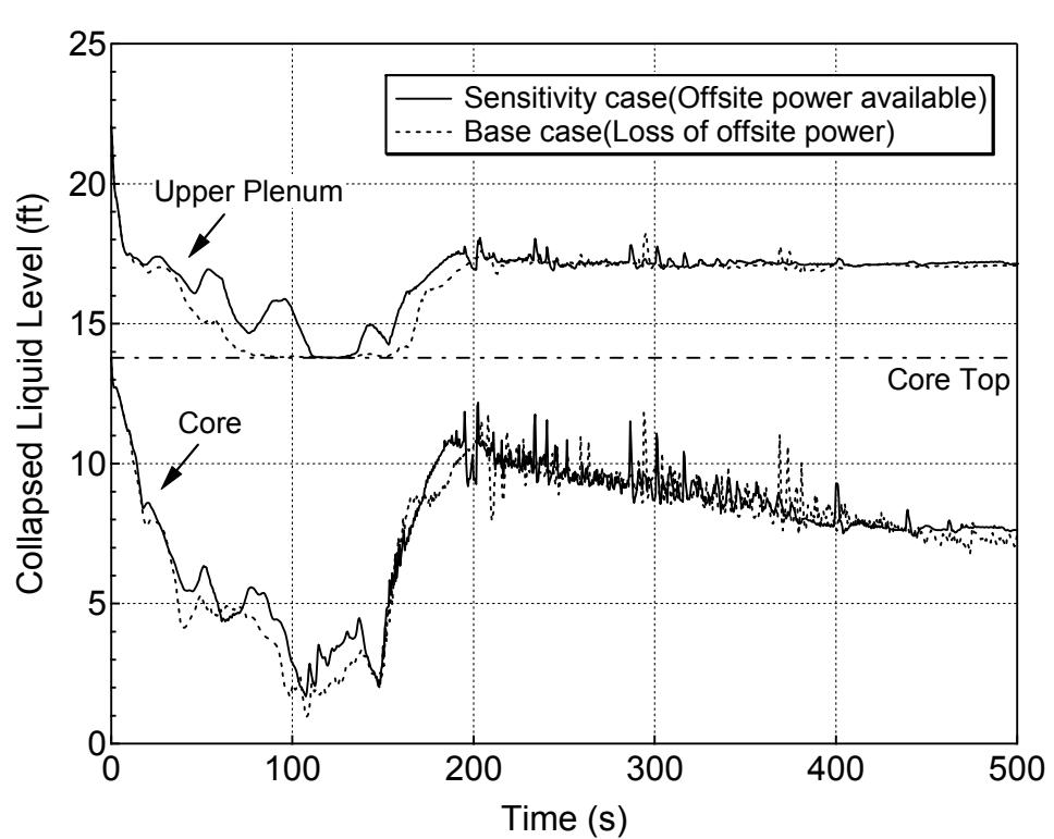
**Figure 5.6.2-22 Average Core and Upper Plenum Collapsed Levels for 1-ft<sup>2</sup> Break (Top)
