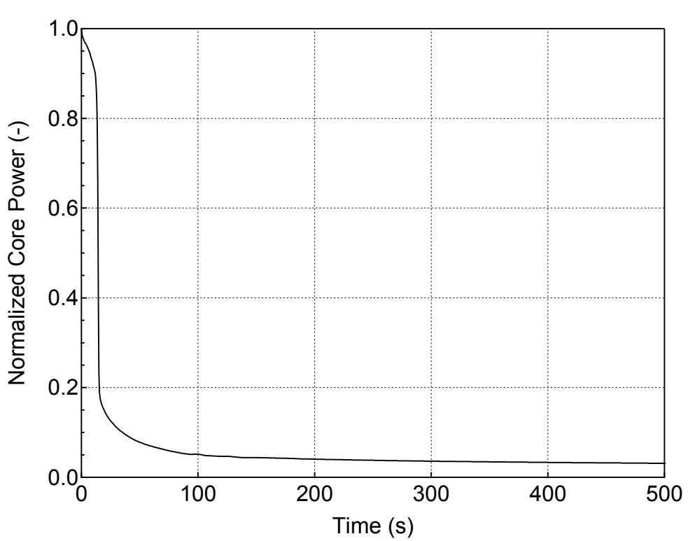
**Figure 5.2.g-2 Normalized Core Power for 7-inch Break (Bottom)
