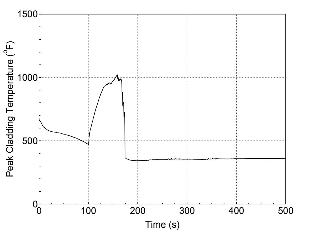
**Figure 5.3.2.c-17 PCT at All Elevations for Hot Rod in Hot Assembly
