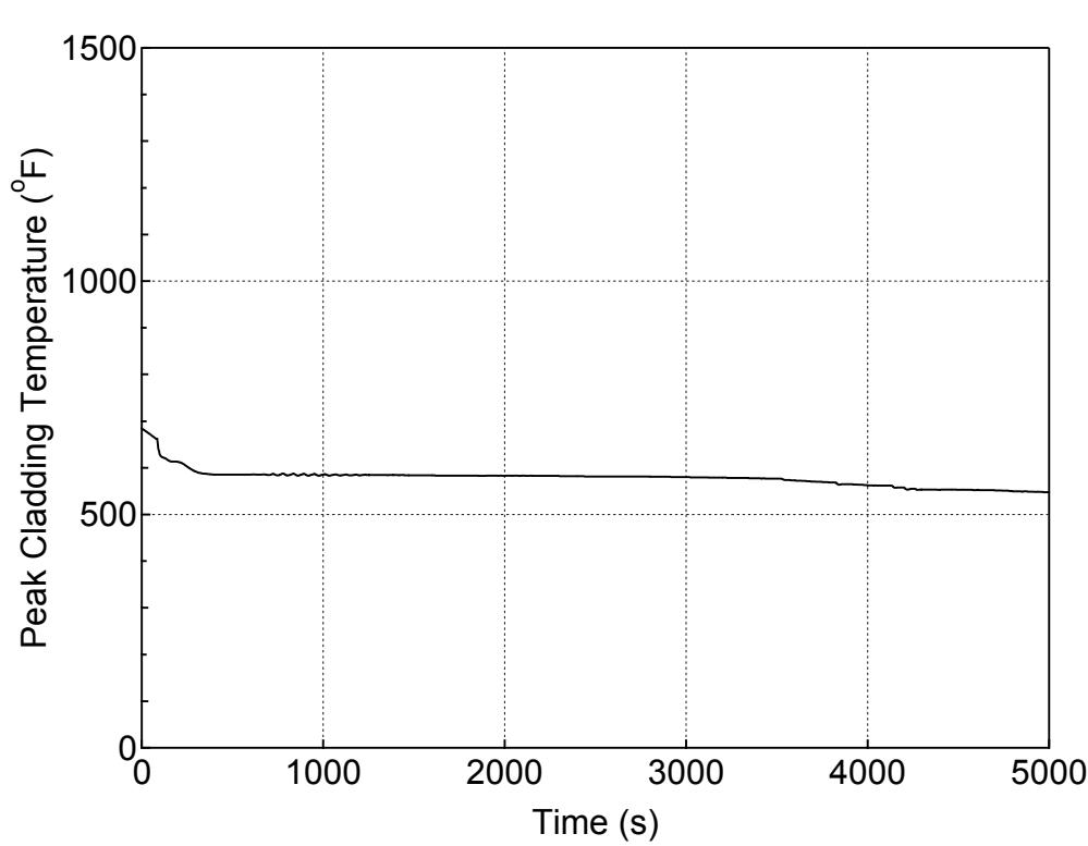
**Figure 5.1.1.a-8 PCT at All Elevations for Hot Rod in Hot Assembly
