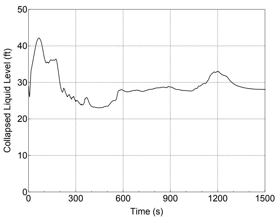
**Figure 5.1.3-10 Pressurizer Collapsed Level for Pressurizer Steam Phase Break
