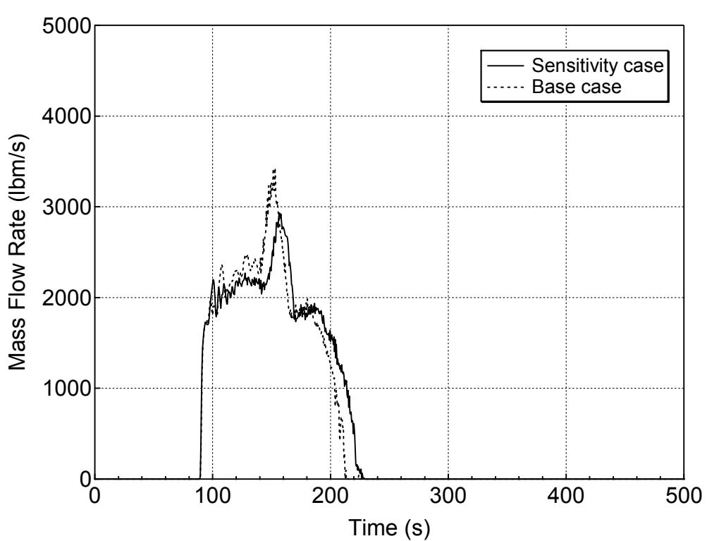
**Figure 5.4.3-18 Accumulator Injection Mass Flowrate for 1-ft<sup>2</sup> Break (Top)
