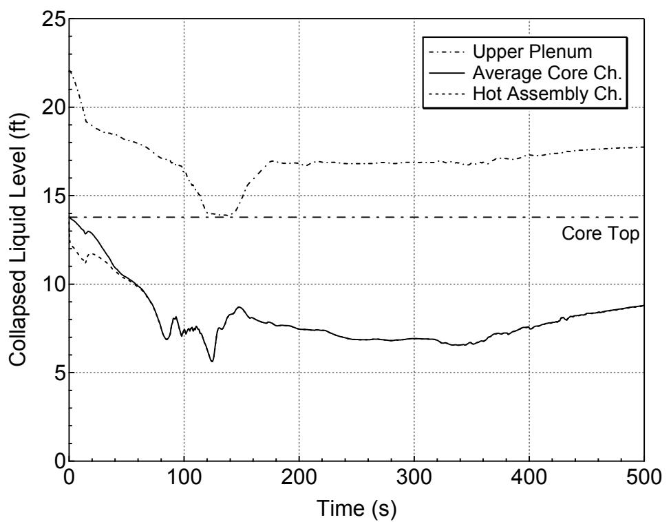
**Figure 5.3.1.d-34 Core and Upper Plenum Collapsed Levels
