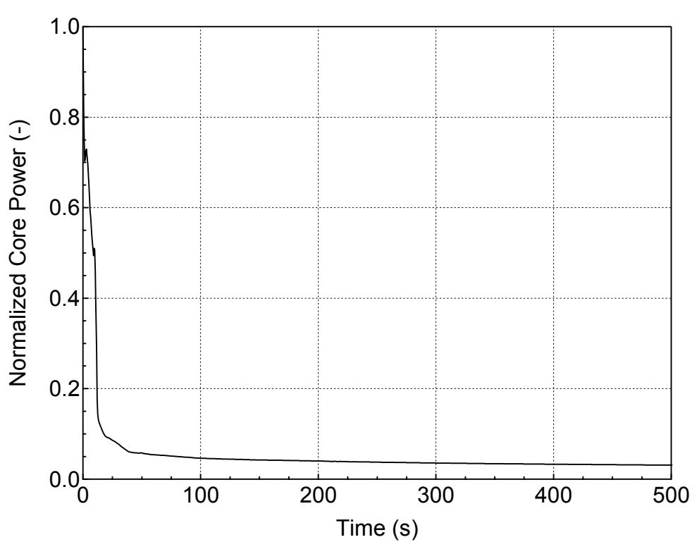
**Figure 5.3.2.c-2 Normalized Core Power for 1-ft<sup>2</sup> Break (Top)
