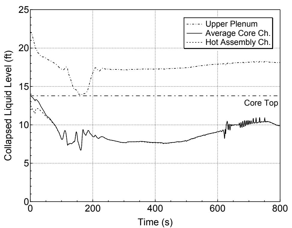
**Figure 5.3.1.b-7 Core and Upper Plenum Collapsed Levels for 6.5-inch Break (Bottom)
