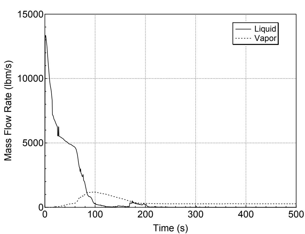
**Figure 5.2.k-3 Liquid and Vapor Discharges through the Break
