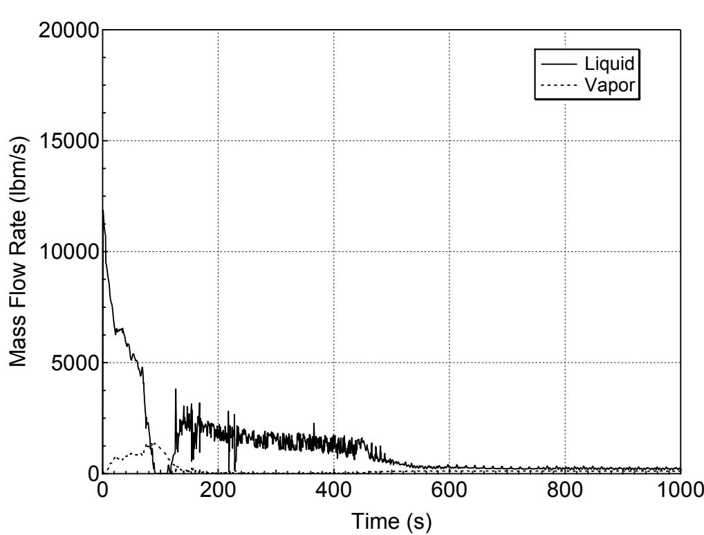
**Figure 5.1.1.b-12 Liquid and Vapor Discharges through the Break
