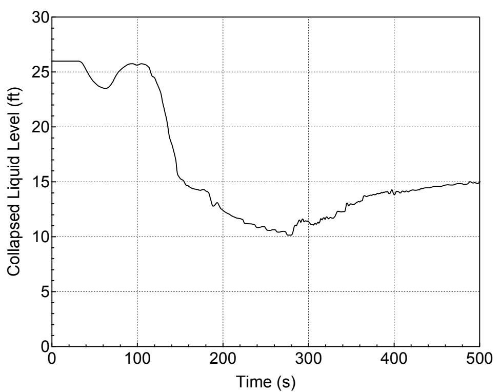
**Figure 5.3.1.e-6 Downcomer Collapsed Level for 8-inch Break (Top)
