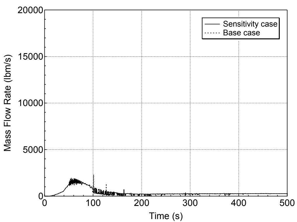
**Figure 5.4.3-17 Vapor Discharge through the Break for 1-ft<sup>2</sup> Break (Top)
