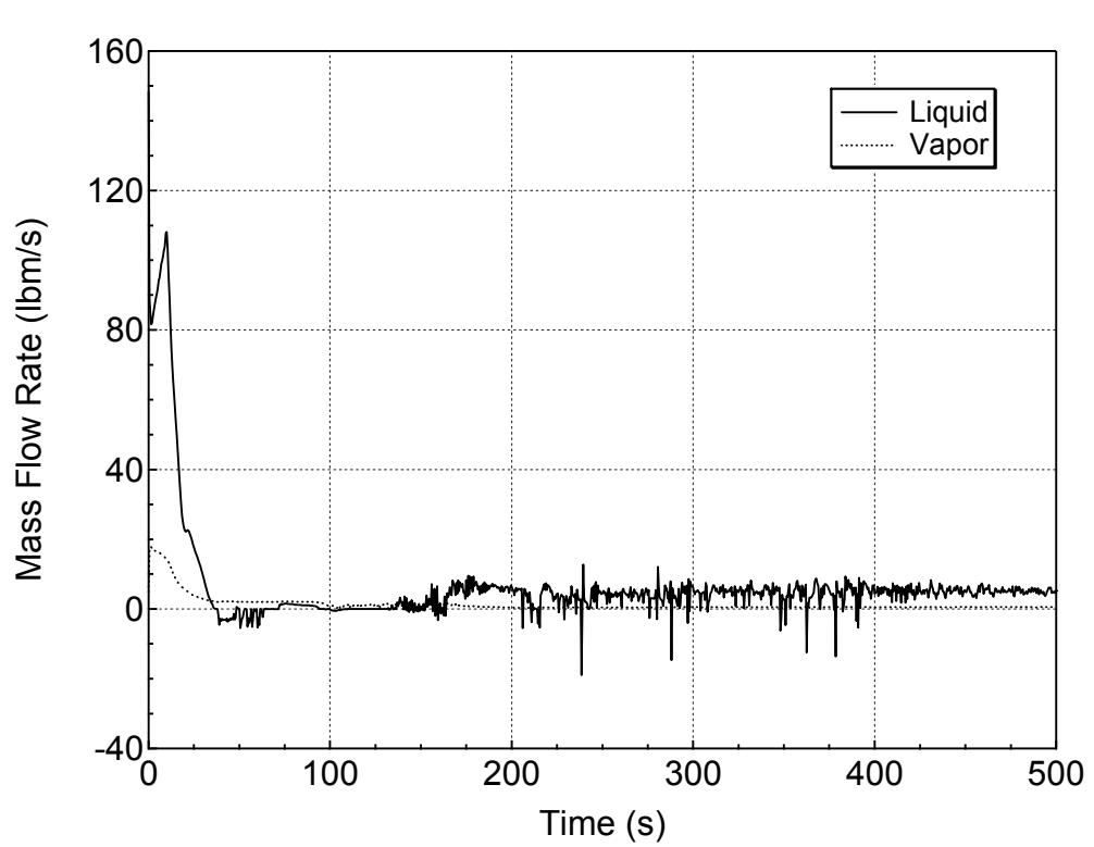
**Figure 5.2.n-9 Hot Assembly Exit Vapor and Liquid Mass Flowrates
