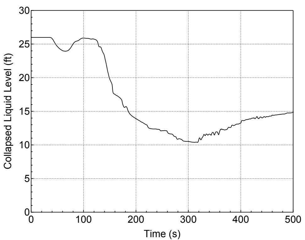
**Figure 5.3.1.d-15 Downcomer Collapsed Level for 7.5-inch Break (Top)
