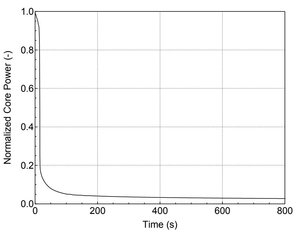
**Figure 5.3.1.b-2 Normalized Core Power for 6.5-inch Break (Bottom)
