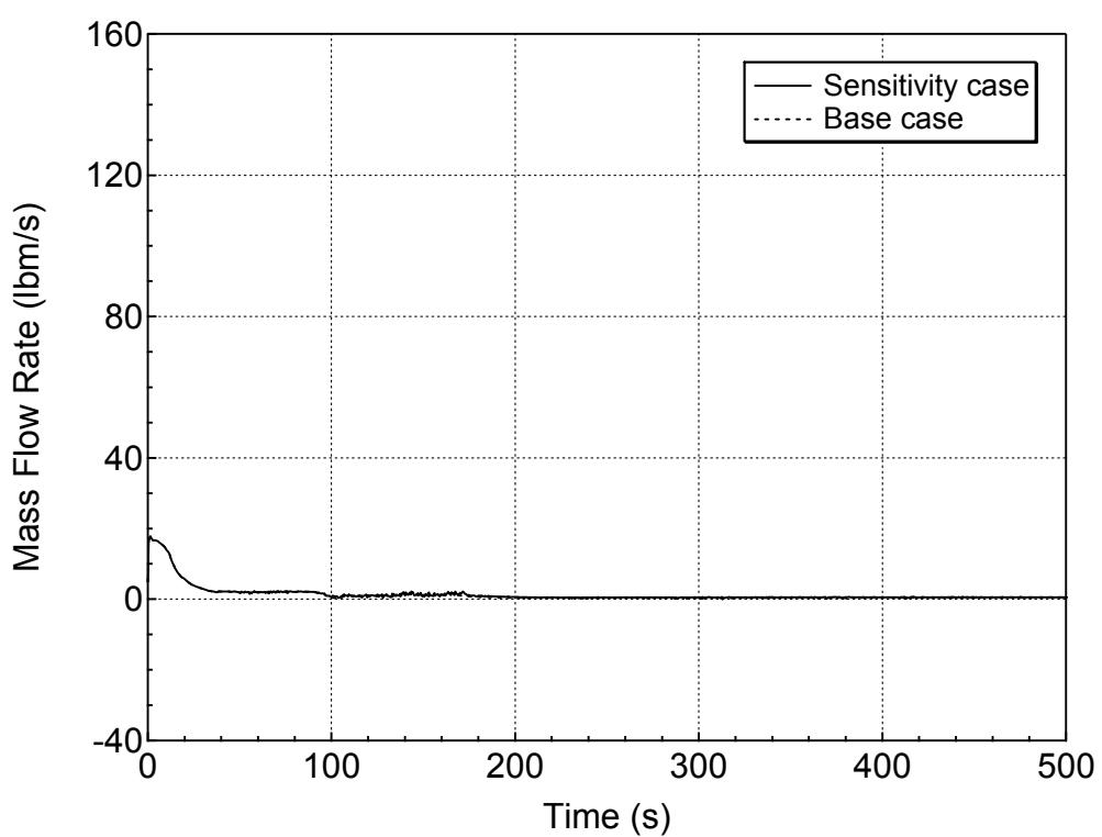
**Figure 5.4.3-26 Hot Assembly Exit Vapor Mass Flowrate for 1-ft<sup>2</sup> Break (Top)
