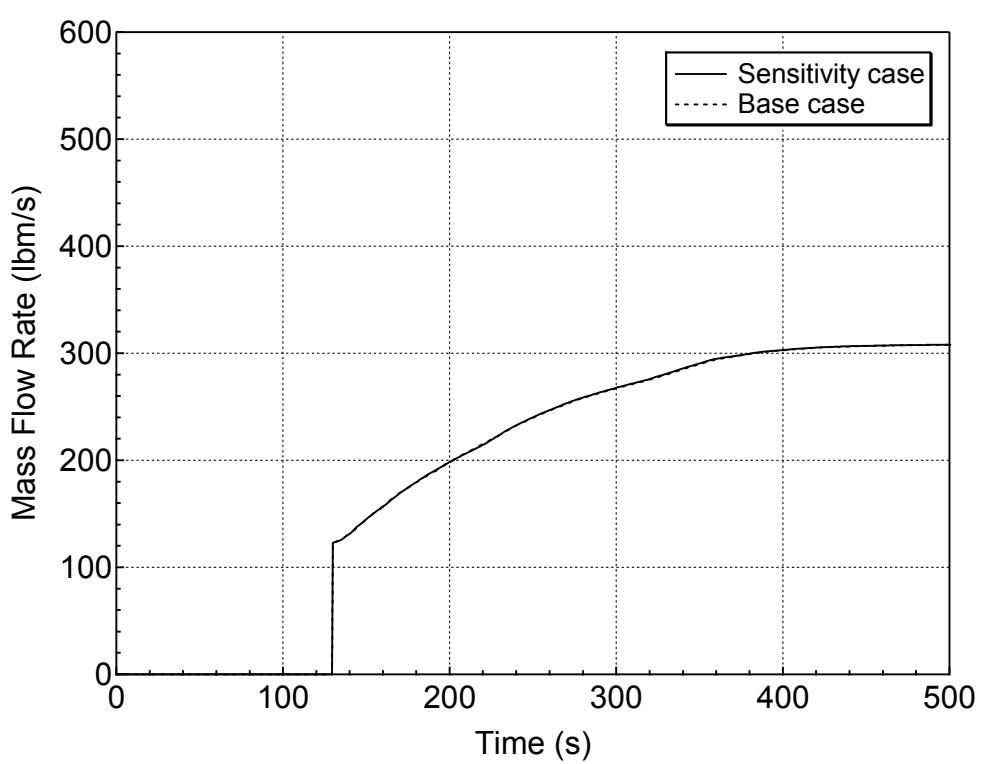
**Figure 5.5.a-6 Safety Injection Mass Flowrate for 7.5-inch Break (Top)
