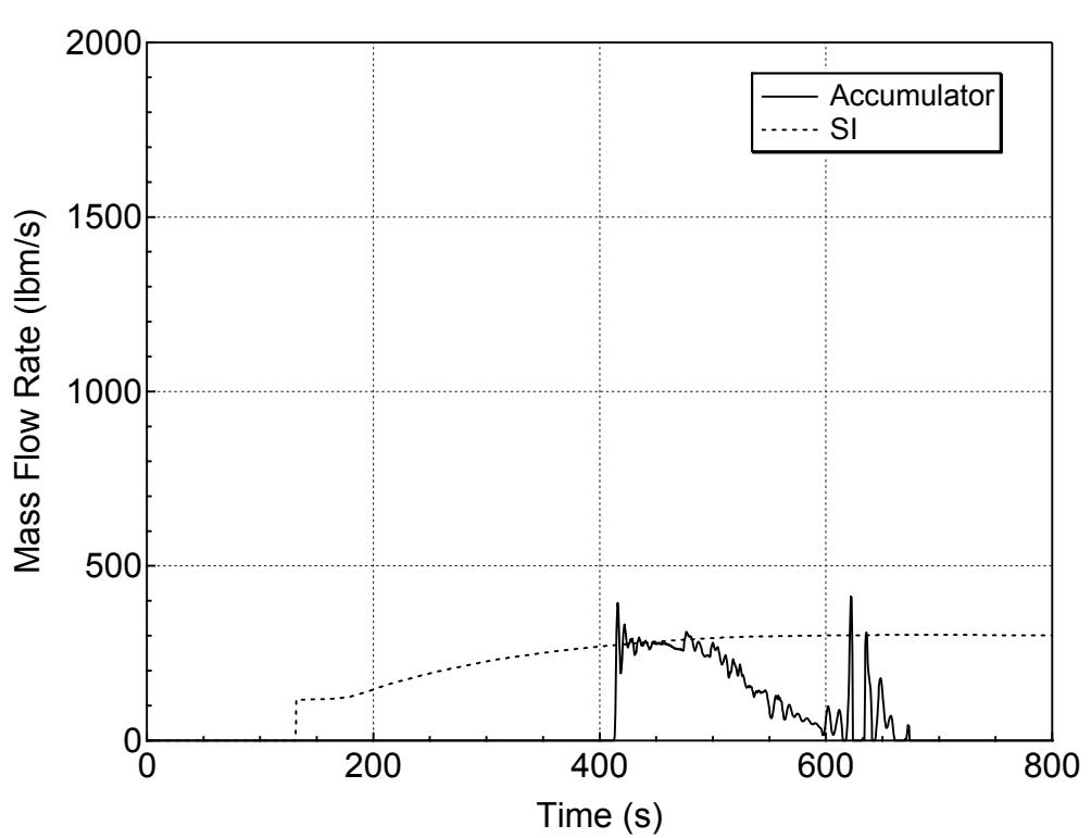
**Figure 5.3.1.b-4 Accumulator and Safety Injection Mass Flowrates
