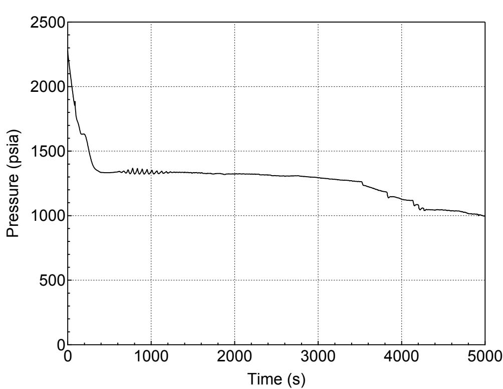
**Figure 5.2.b-1 RCS (Pressurizer) Pressure Transient for 2-inch Break (Bottom)
