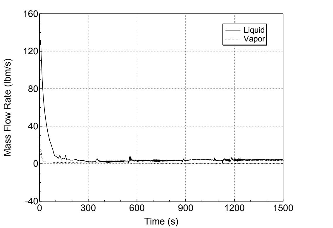
**Figure 5.1.3-9 Hot Assembly Exit Vapor and Liquid Mass Flowrates
