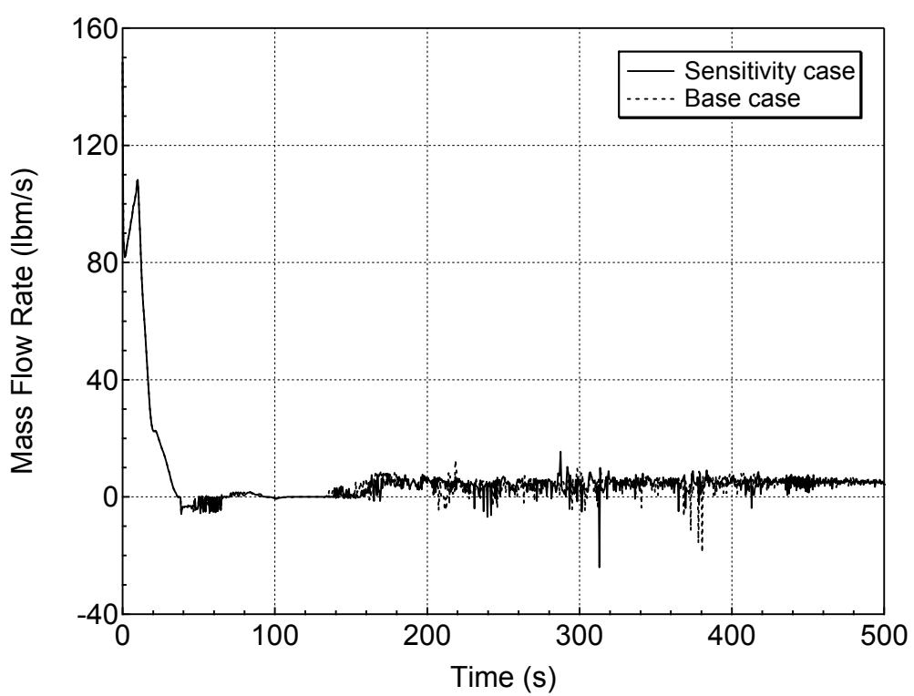
**Figure 5.4.3-25 Hot Assembly Exit Liquid Mass Flowrate for 1-ft<sup>2</sup> Break (Top)
