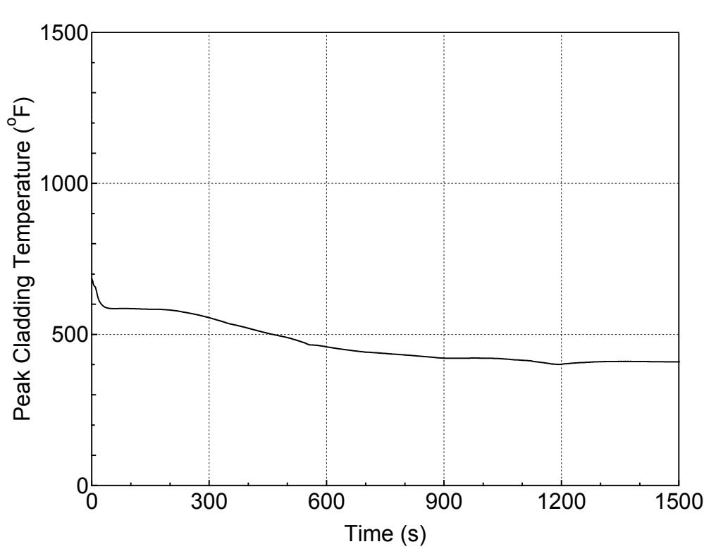
**Figure 5.1.3-8 PCT at All Elevations for Hot Rod in Hot Assembly
