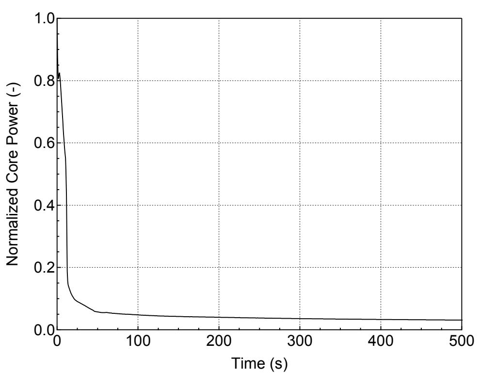
**Figure 5.3.2.a-2 Normalized Core Power for 12-inch Break (Top)
