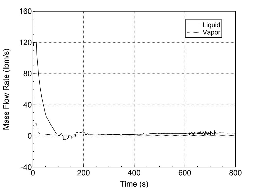
**Figure 5.3.1.b-18 Hot Assembly Exit Vapor and Liquid Mass Flowrates
