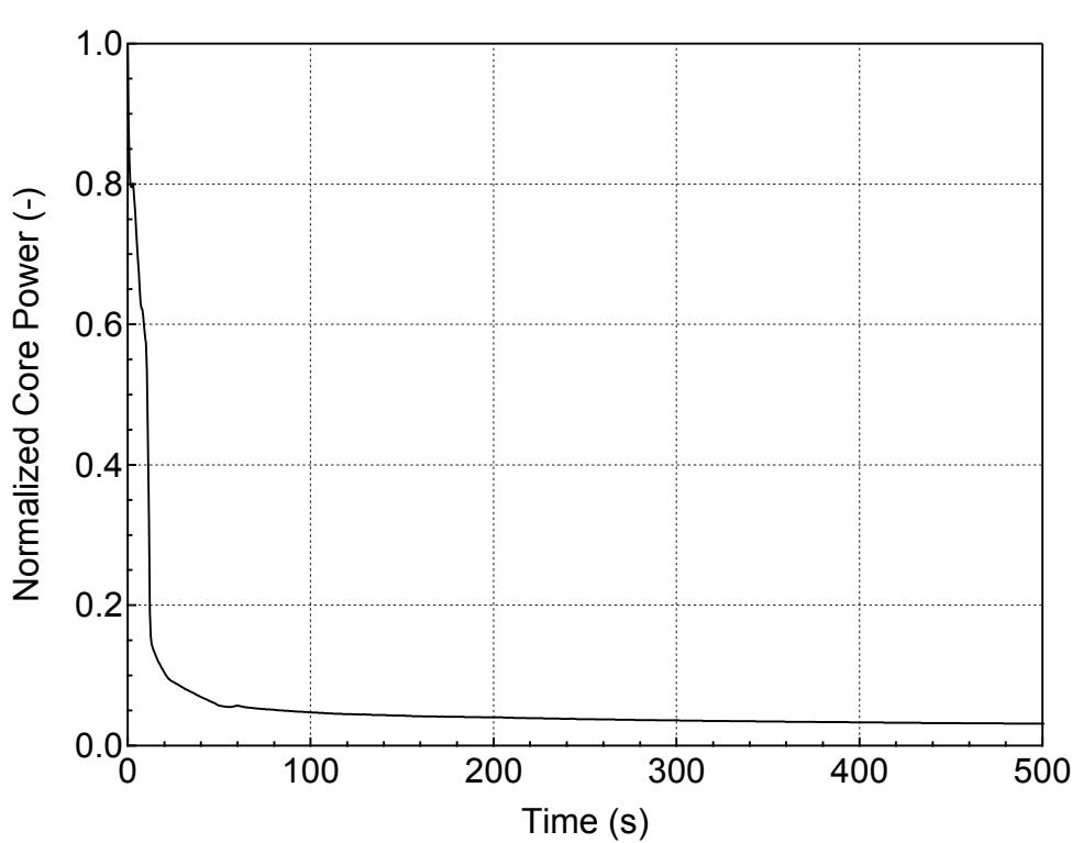
**Figure 5.1.1.c-11 Normalized Core Power for 1-ft<sup>2</sup> Break (Bottom)
