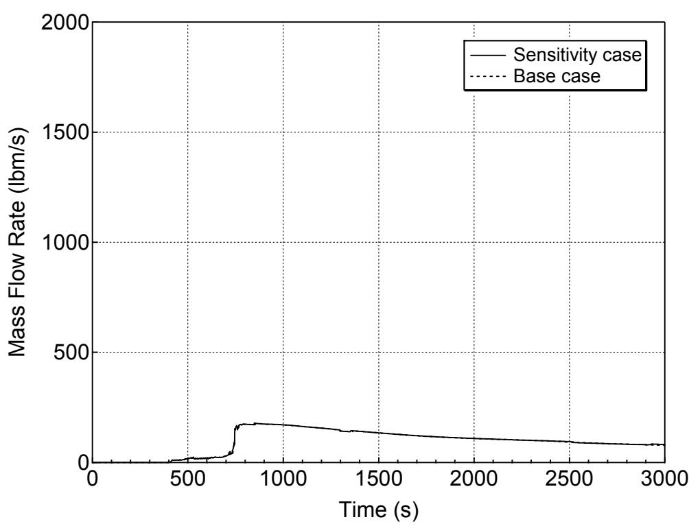
**Figure 5.5.c-4 Vapor Discharge through the Break for DVI-line Break
