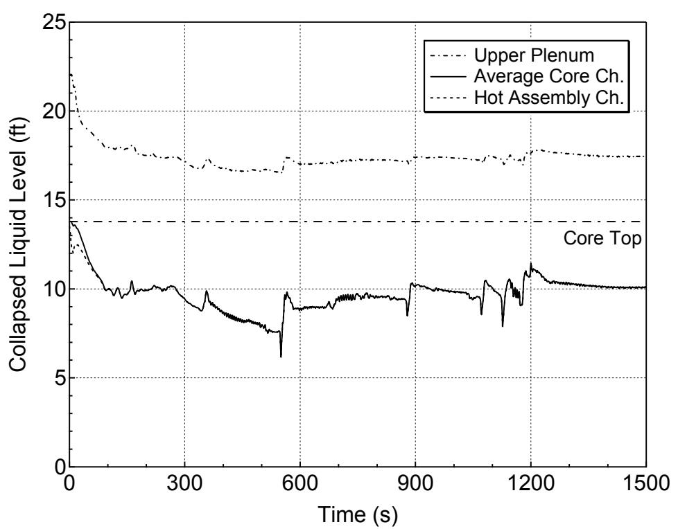
**Figure 5.1.3-7 Core and Upper Plenum Collapsed Levels
