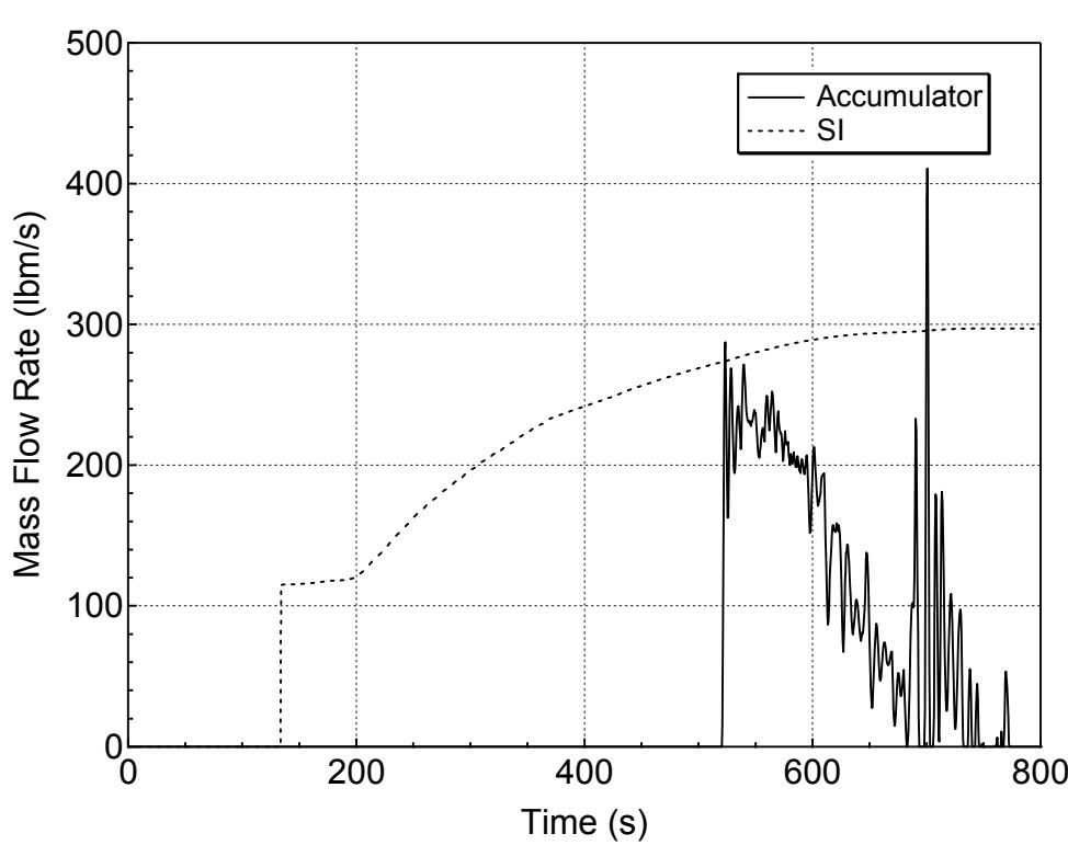
**Figure 5.3.1.a-4 Accumulator and Safety Injection Mass Flowrates
