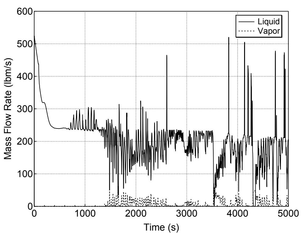
**Figure 5.2.b-3 Liquid and Vapor Discharges through the Break
