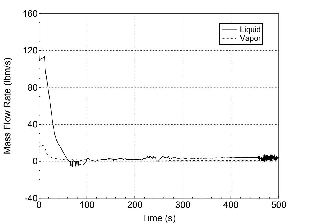
**Figure 5.2.i-9 Hot Assembly Exit Vapor and Liquid Mass Flowrates
