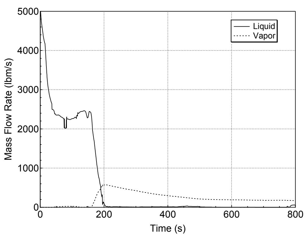
**Figure 5.3.1.b-21 Liquid and Vapor Discharges through the Break
