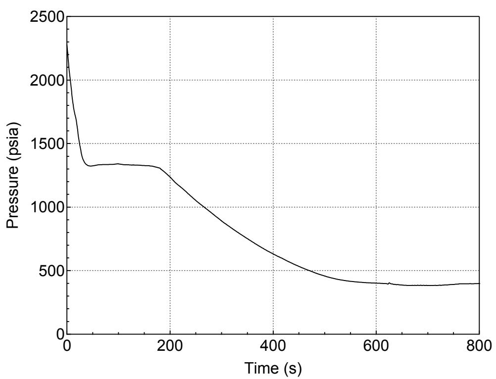
**Figure 5.3.1.b-1 RCS (Pressurizer) Pressure Transient for 6.5-inch Break (Bottom)
