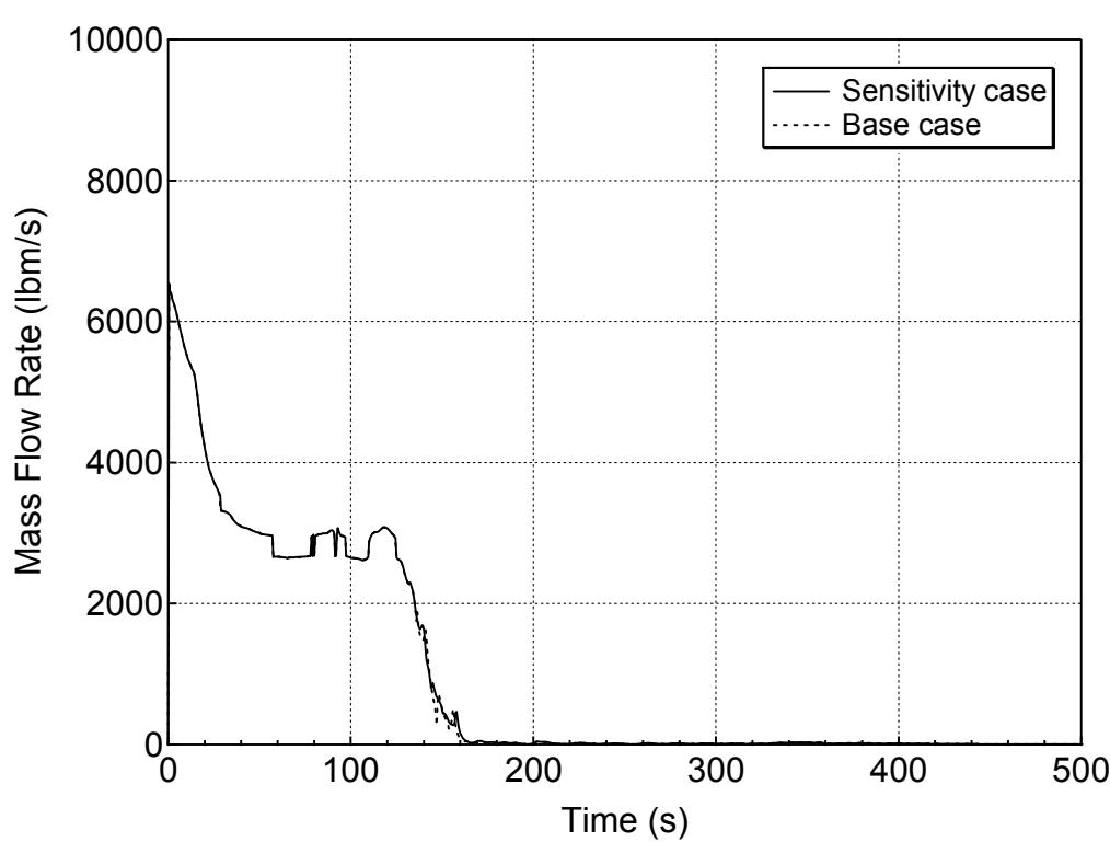
**Figure 5.5.a-3 Liquid Discharge through the Break for 7.5-inch Break (Top)
