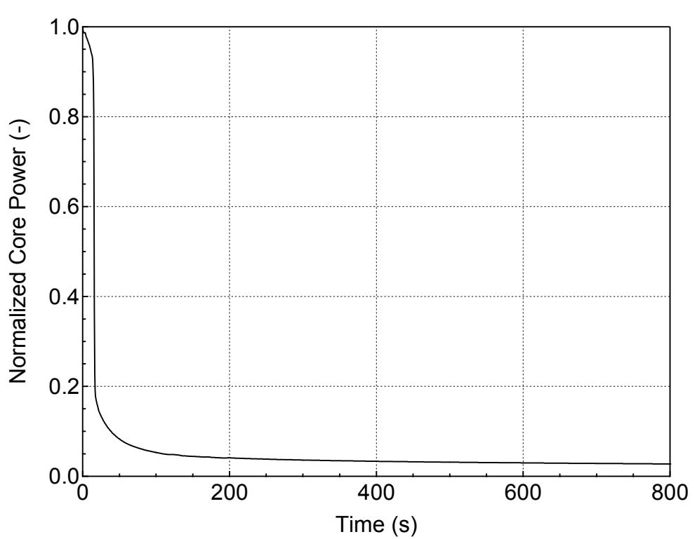
**Figure 5.3.1.a-20 Normalized Core Power for 6-inch Break (Homogeneous)
