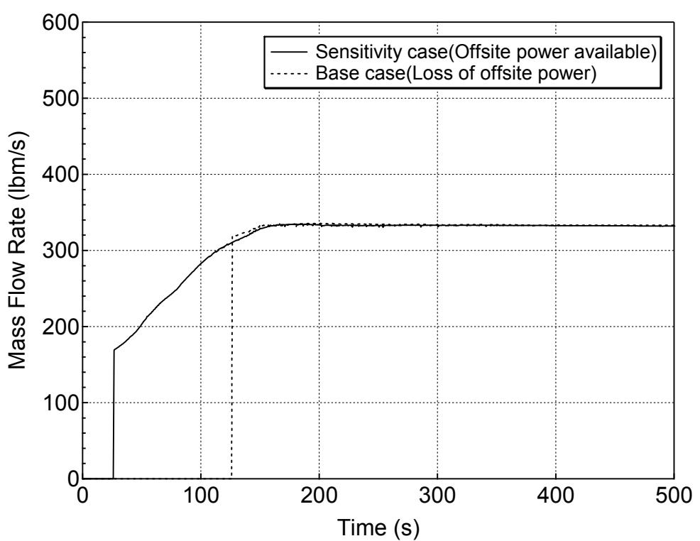
**Figure 5.6.2-19 Safety Injection Mass Flowrate for 1-ft<sup>2</sup> Break (Top)
