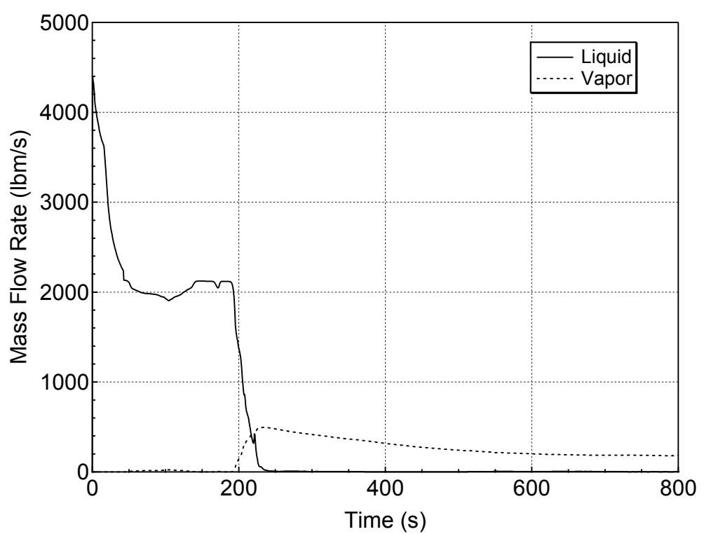
**Figure 5.3.1.a-21 Liquid and Vapor Discharges through the Break
