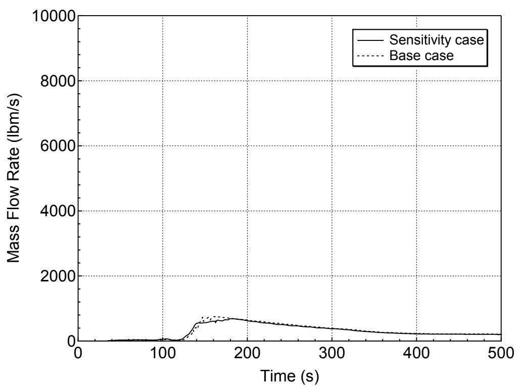
**Figure 5.4.2-4 Vapor Discharge through the Break for 7.5-inch Break (Top)
