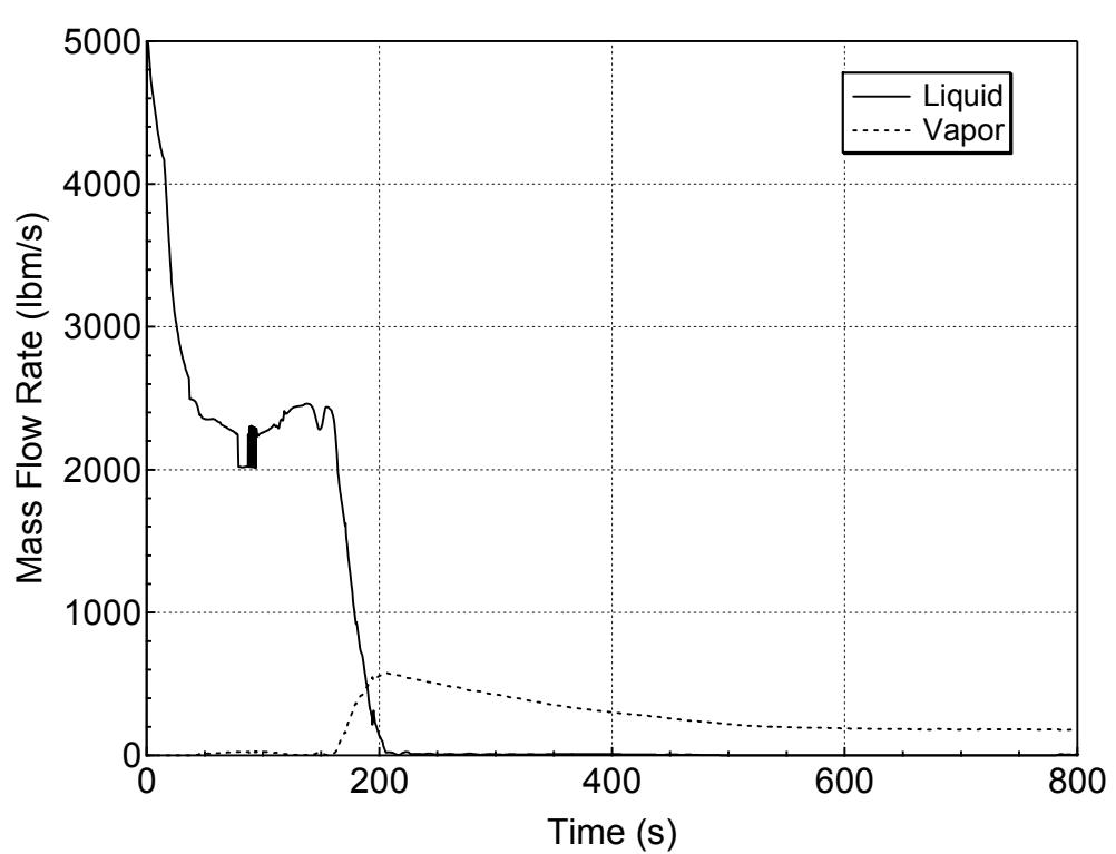
**Figure 5.3.1.b-12 Liquid and Vapor Discharges through the Break
