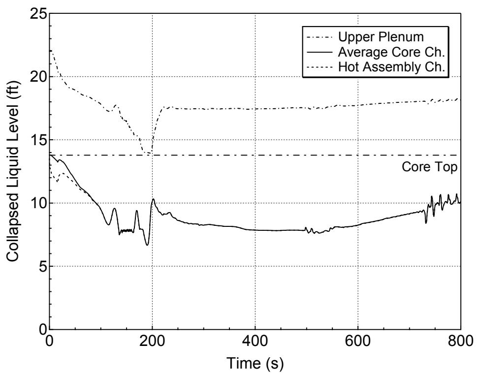
**Figure 5.3.1.a-25 Core and Upper Plenum Collapsed Levels
