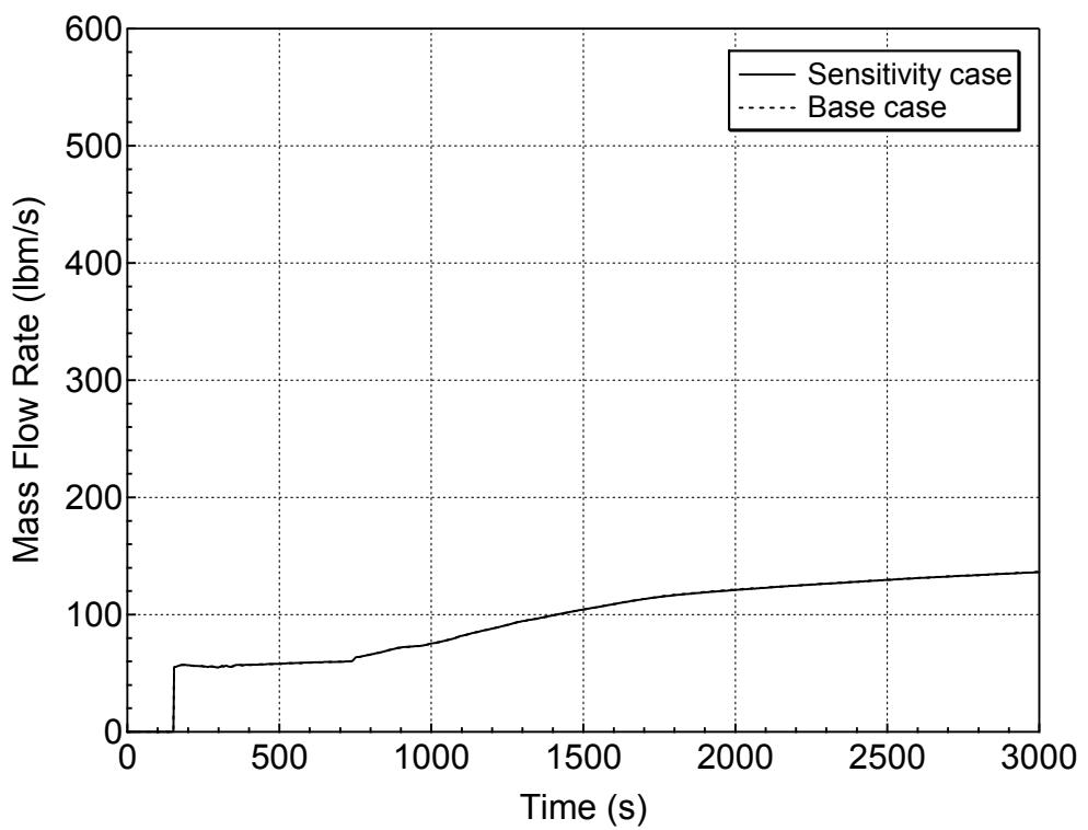
**Figure 5.5.c-6 Safety Injection Mass Flowrate for DVI-line Break
