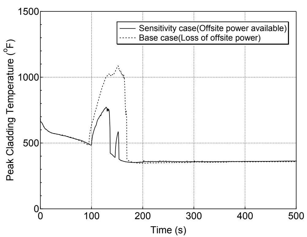
**Figure 5.6.2-24 PCT at All Elevations for Hot Rod in Hot Assembly for 1-ft<sup>2</sup> Break (Top)
