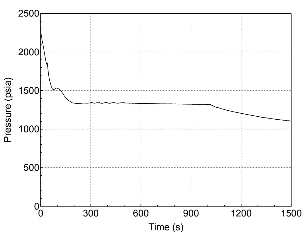
**Figure 5.2.c-1 RCS (Pressurizer) Pressure Transient for 3-inch Break (Bottom)
