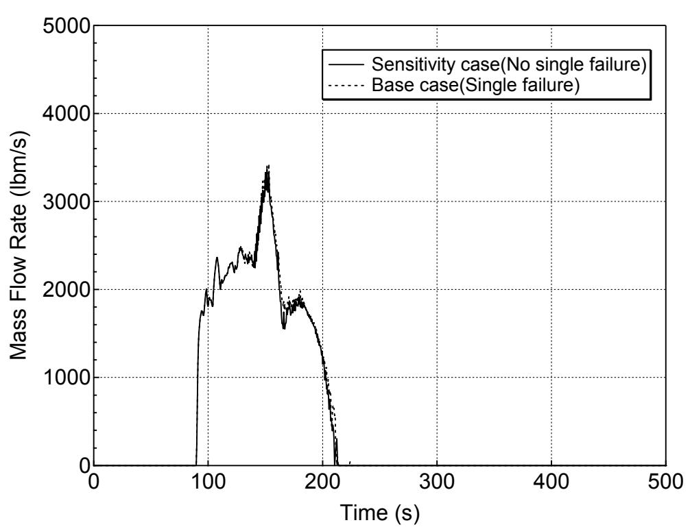
**Figure 5.6.1-18 Accumulator Mass Flowrate for 1-ft<sup>2</sup> Break (Top)
