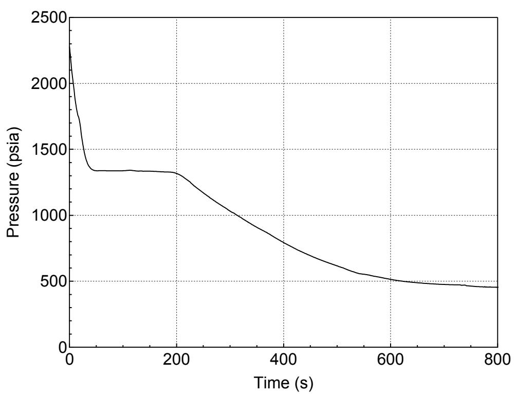
**Figure 5.2.f-1 RCS (Pressurizer) Pressure Transient for 6-inch Break (Bottom)
