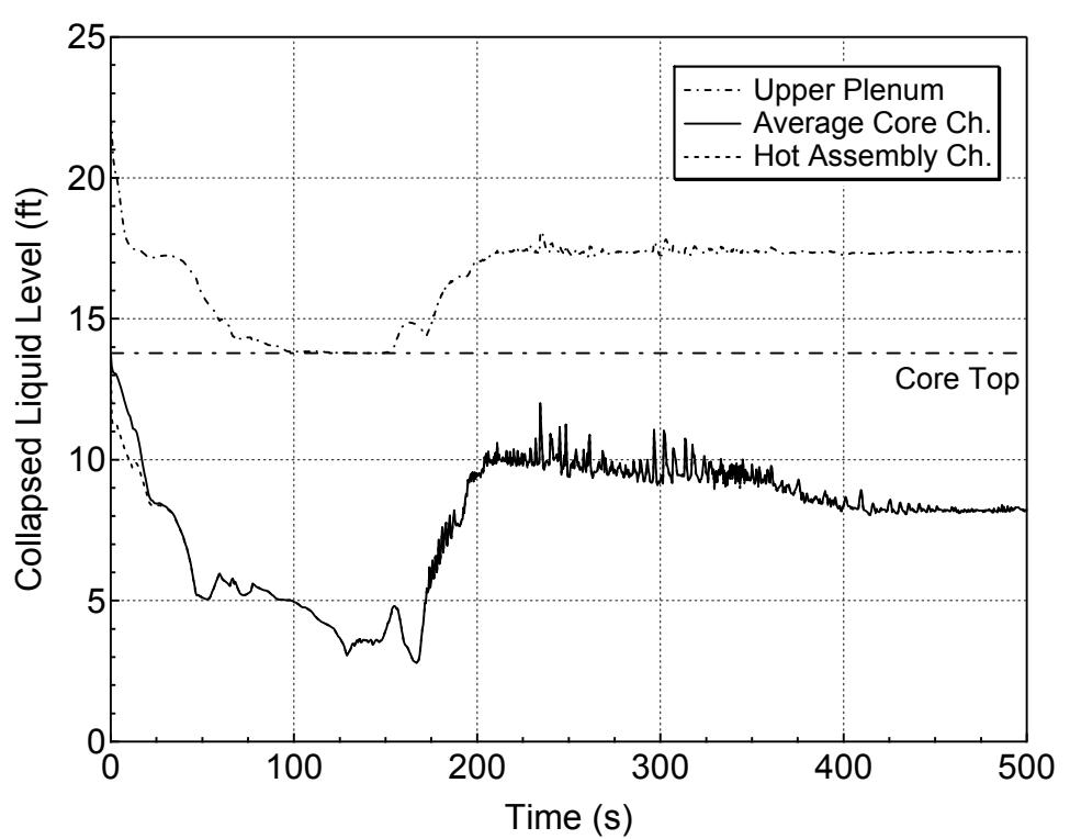
**Figure 5.2.I-7 Core and Upper Plenum Collapsed Levels for 12-inch Break (Bottom)
