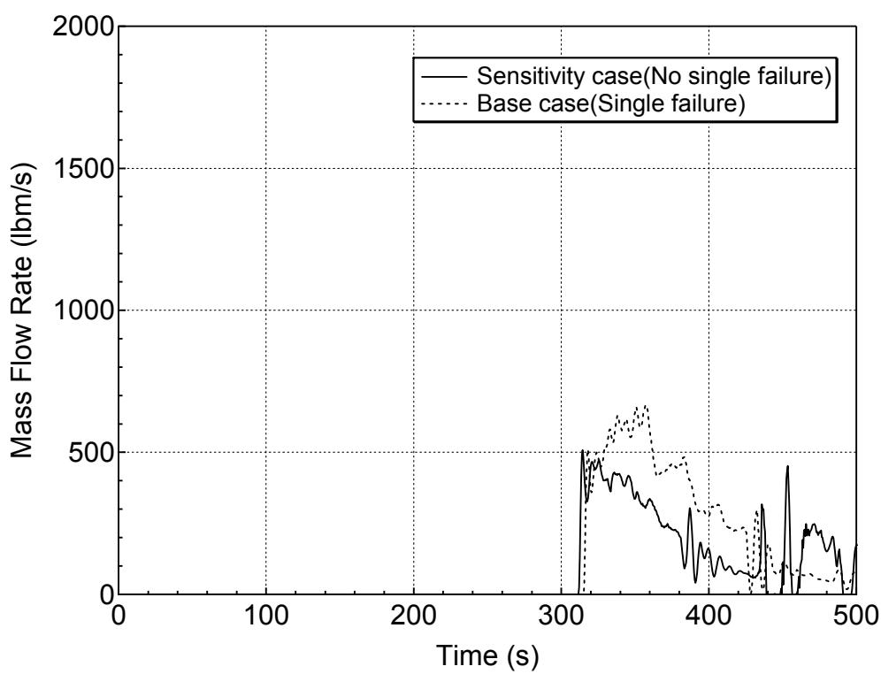
**Figure 5.6.1-5 Accumulator Mass Flowrate for 7.5-inch Break (Top)
