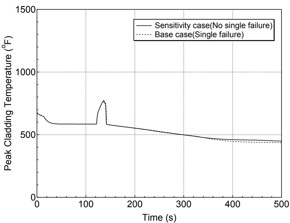
**Figure 5.6.1-11 PCT at All Elevations for Hot Rod in Hot Assembly
