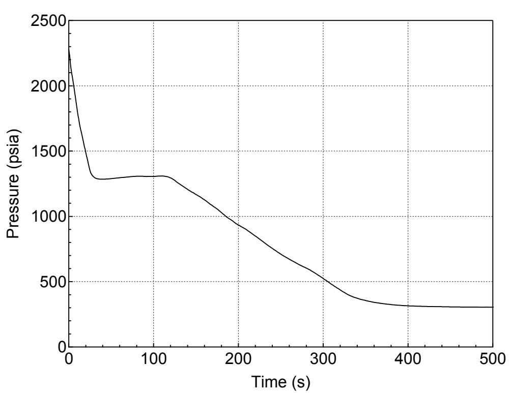
**Figure 5.3.1.e-10 RCS (Pressurizer) Pressure Transient for 8-inch Break (Side)
