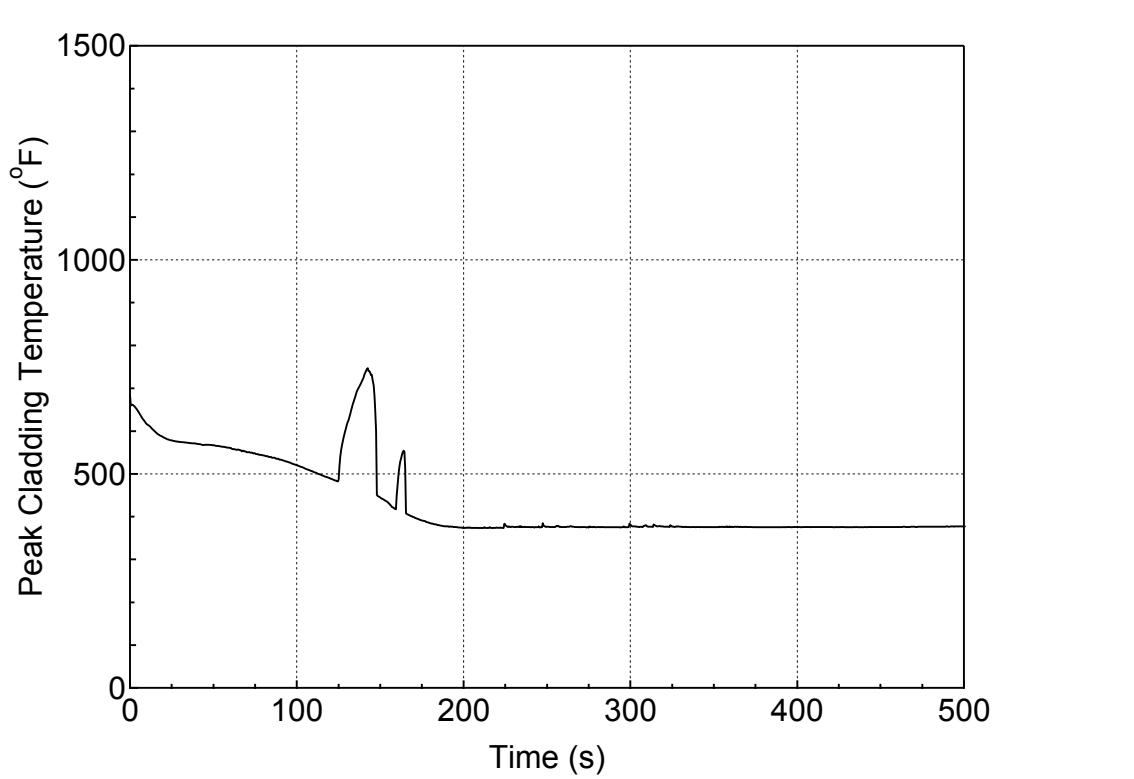
**Figure 5.3.2.a-8 PCT at All Elevations for Hot Rod in Hot Assembly
