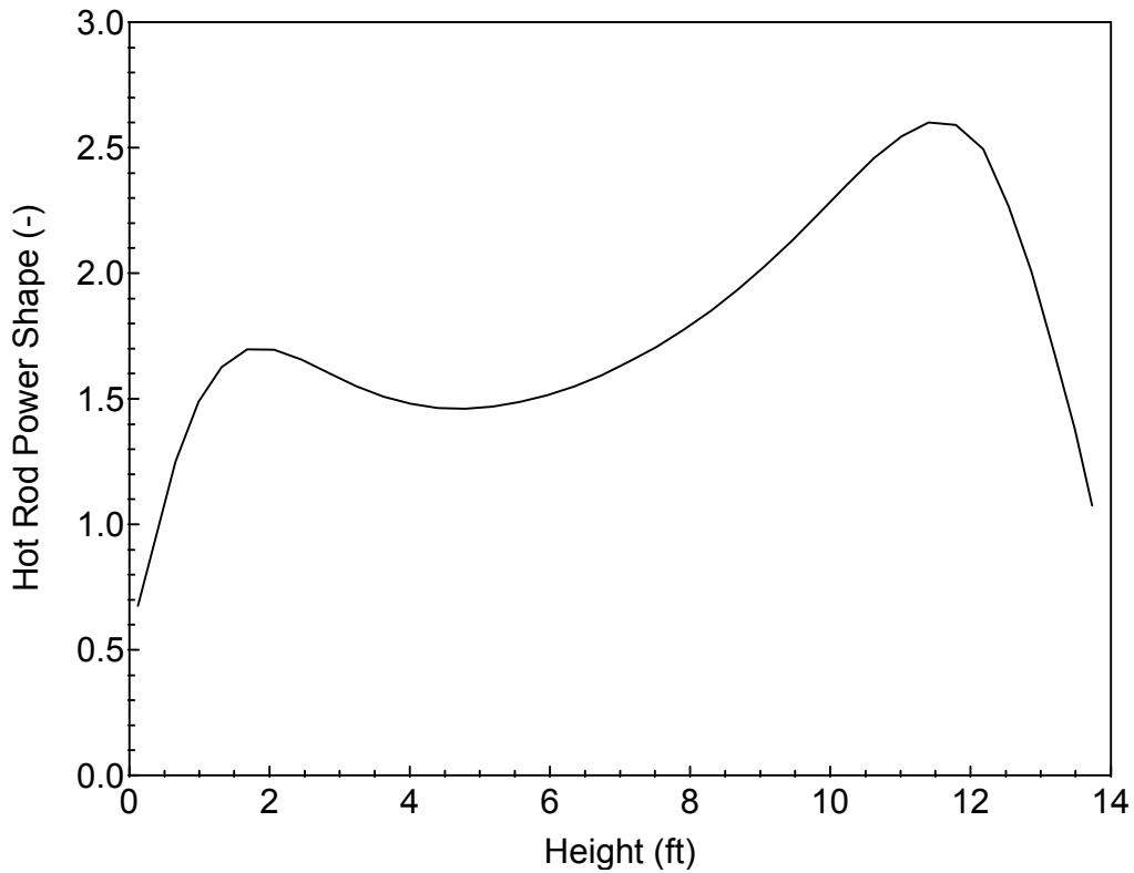
**Figure 4.1-1 Hot Rod Power Shape Used for Small Break LOCA analysis**
