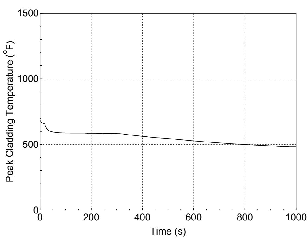
**Figure 5.2.e-8 PCT at All Elevations for Hot Rod in Hot Assembly
