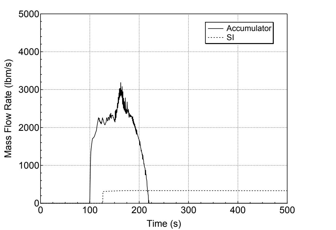
**Figure 5.3.2.b-13 Accumulator and Safety Injection Mass Flowrates
