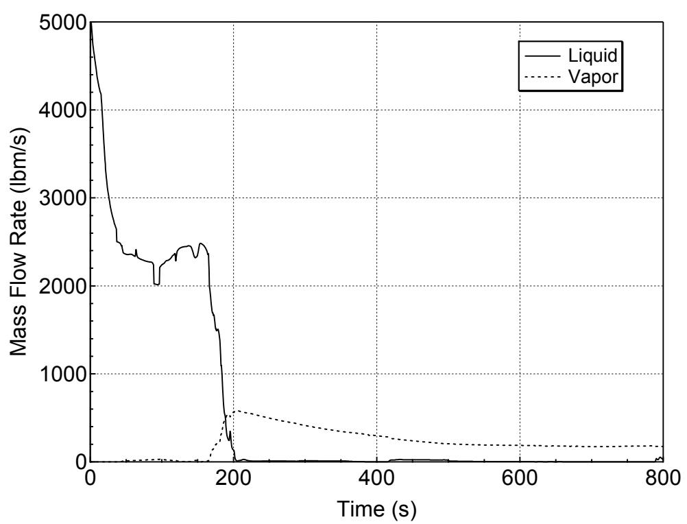
**Figure 5.3.1.b-3 Liquid and Vapor Discharges through the Break
