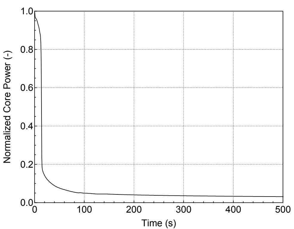
**Figure 5.3.1.d-11 Normalized Core Power for 7.5-inch Break (Top)
