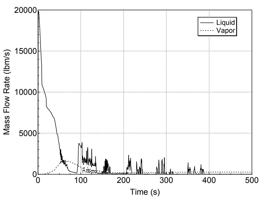
**Figure 5.1.1.a-12 Liquid and Vapor Discharges through the Break
