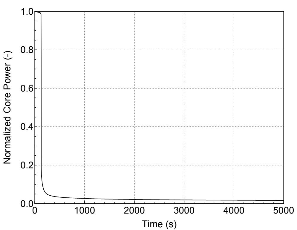
**Figure 5.1.1.b-2 Normalized Core Power for 2-inch Break (Bottom)
