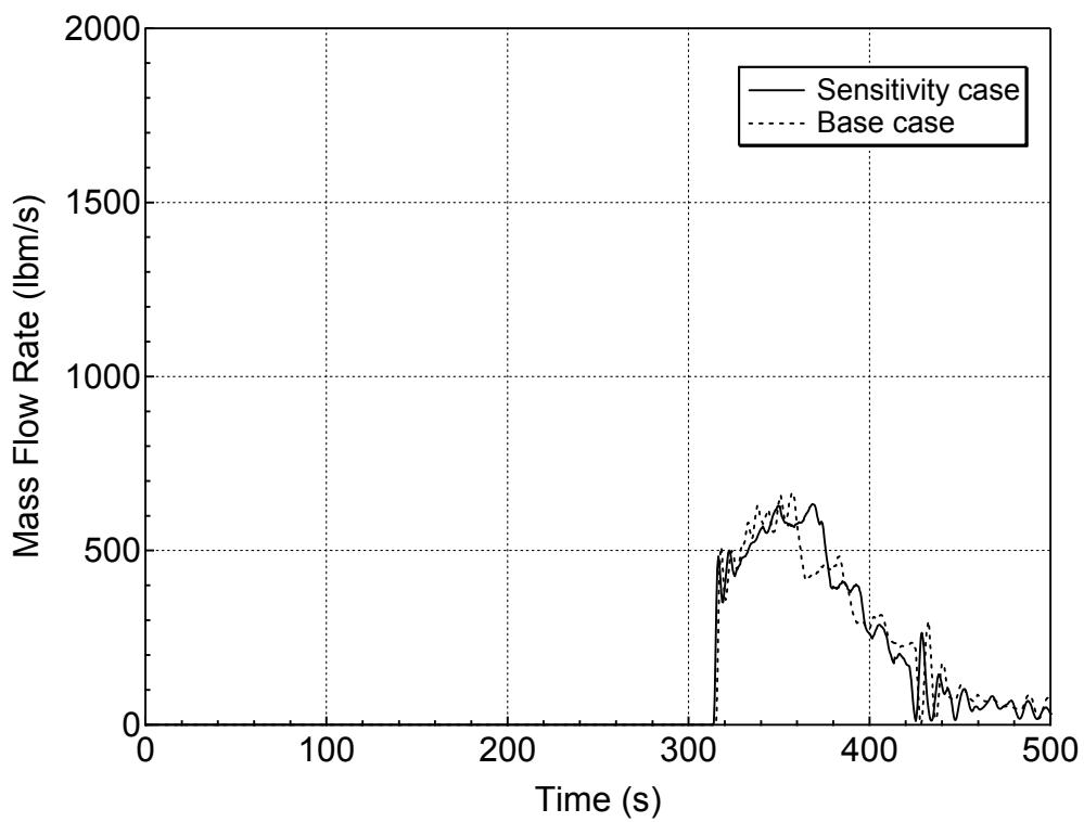
**Figure 5.4.3-5 Accumulator Injection Mass Flowrate for 7.5-inch Break (Top)
