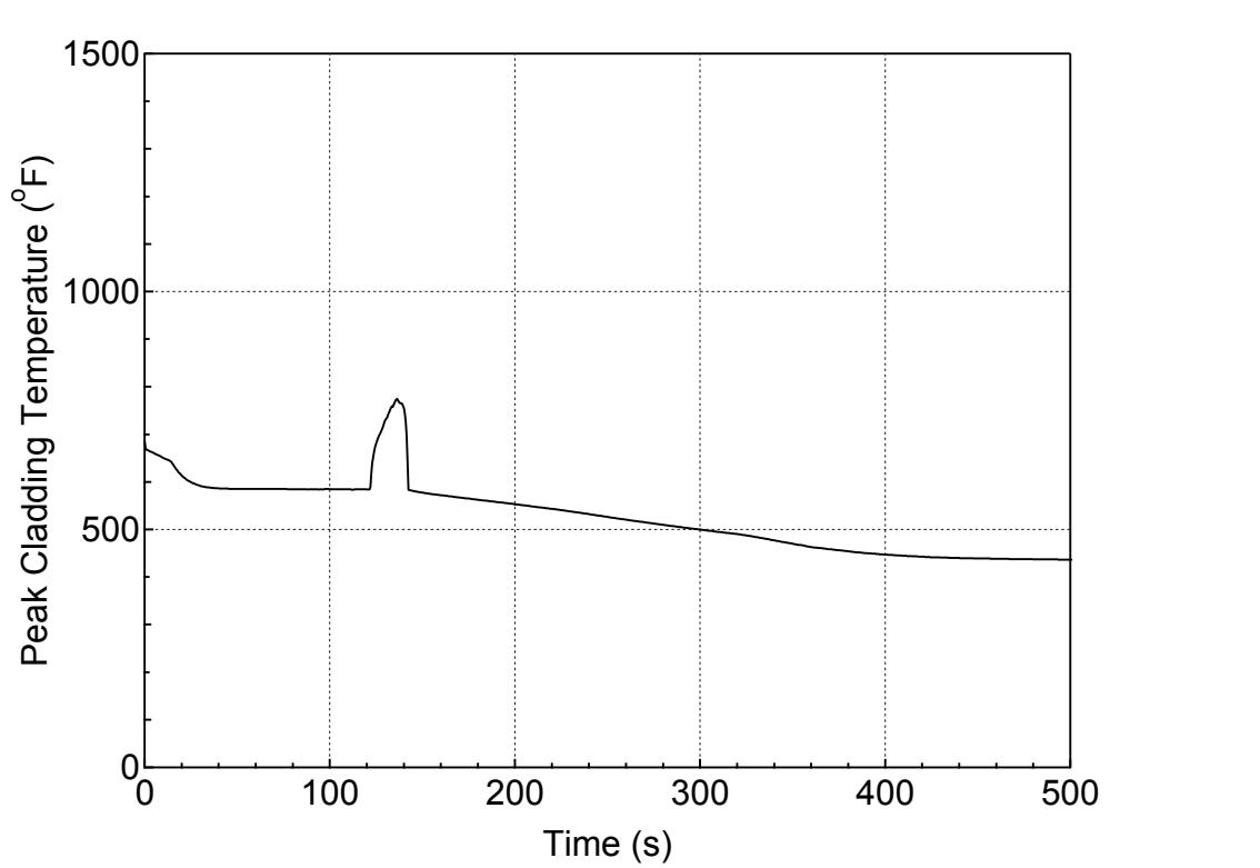
**Figure 5.3.1.d-17 PCT at All Elevations for Hot Rod in Hot Assembly
