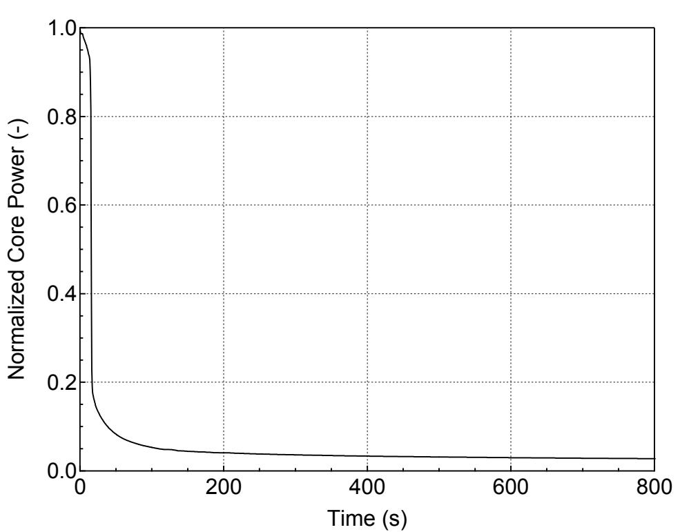
**Figure 5.3.1.a-11 Normalized Core Power for 6-inch Break (Side)
