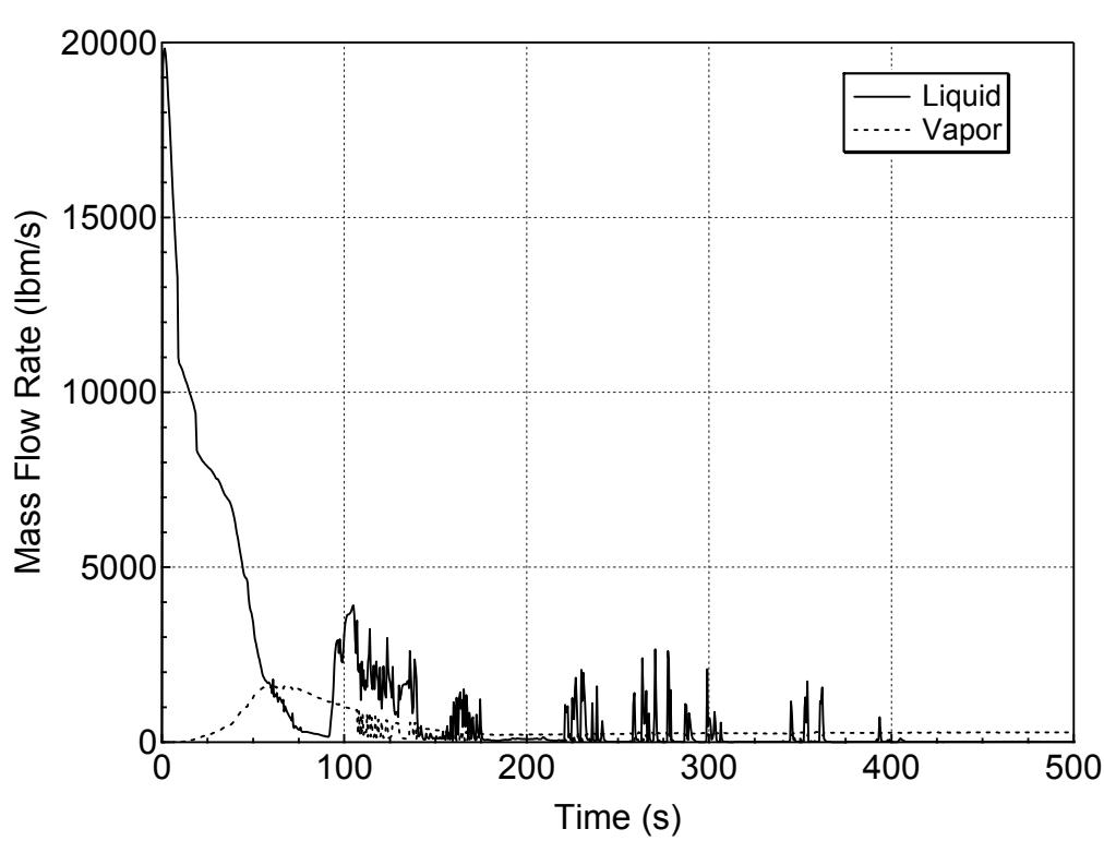
**Figure 5.3.2.c-12 Liquid and Vapor Discharges through the Break for 1-ft<sup>2</sup> Break (Side)
