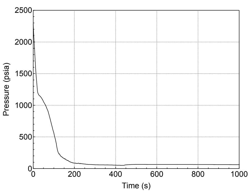
**Figure 5.1.1.b-10 RCS (Pressurizer) Pressure Transient for 1-ft<sup>2</sup> Break (Bottom)
