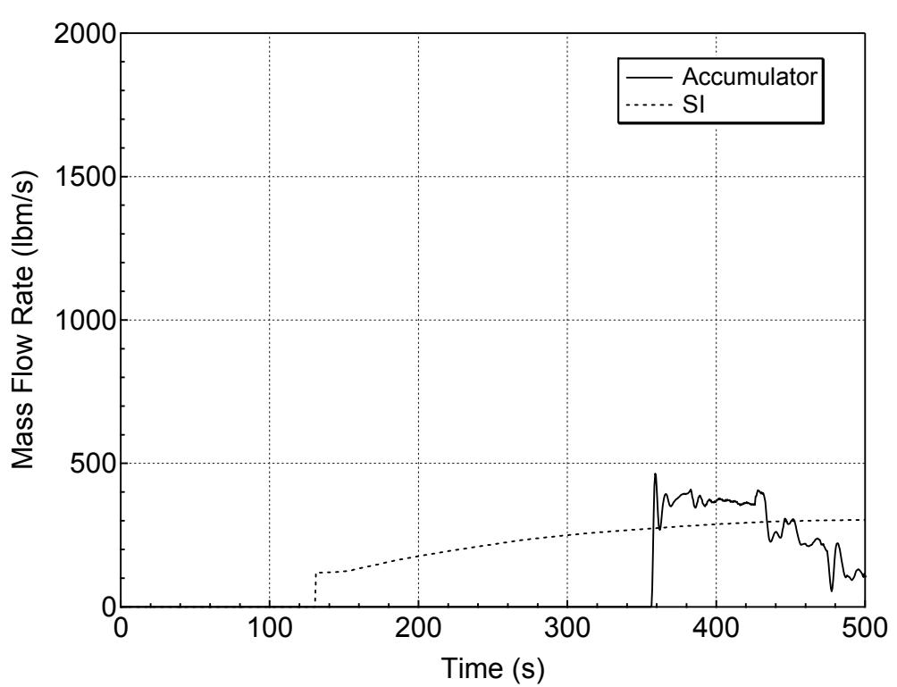
**Figure 5.3.1.c-13 Accumulator and Safety Injection Mass Flowrates
