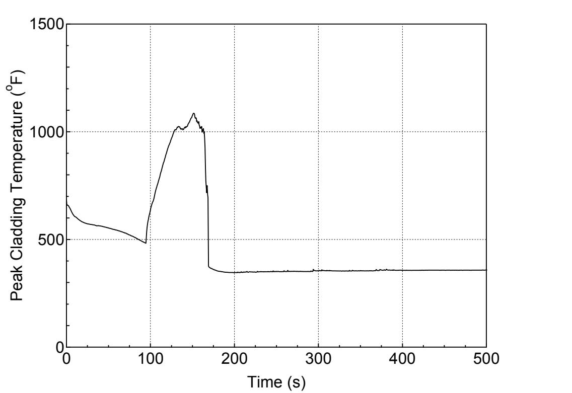
**Figure 5.3.2.c-8 PCT at All Elevations for Hot Rod in Hot Assembly for 1-ft<sup>2</sup> Break (Top)
