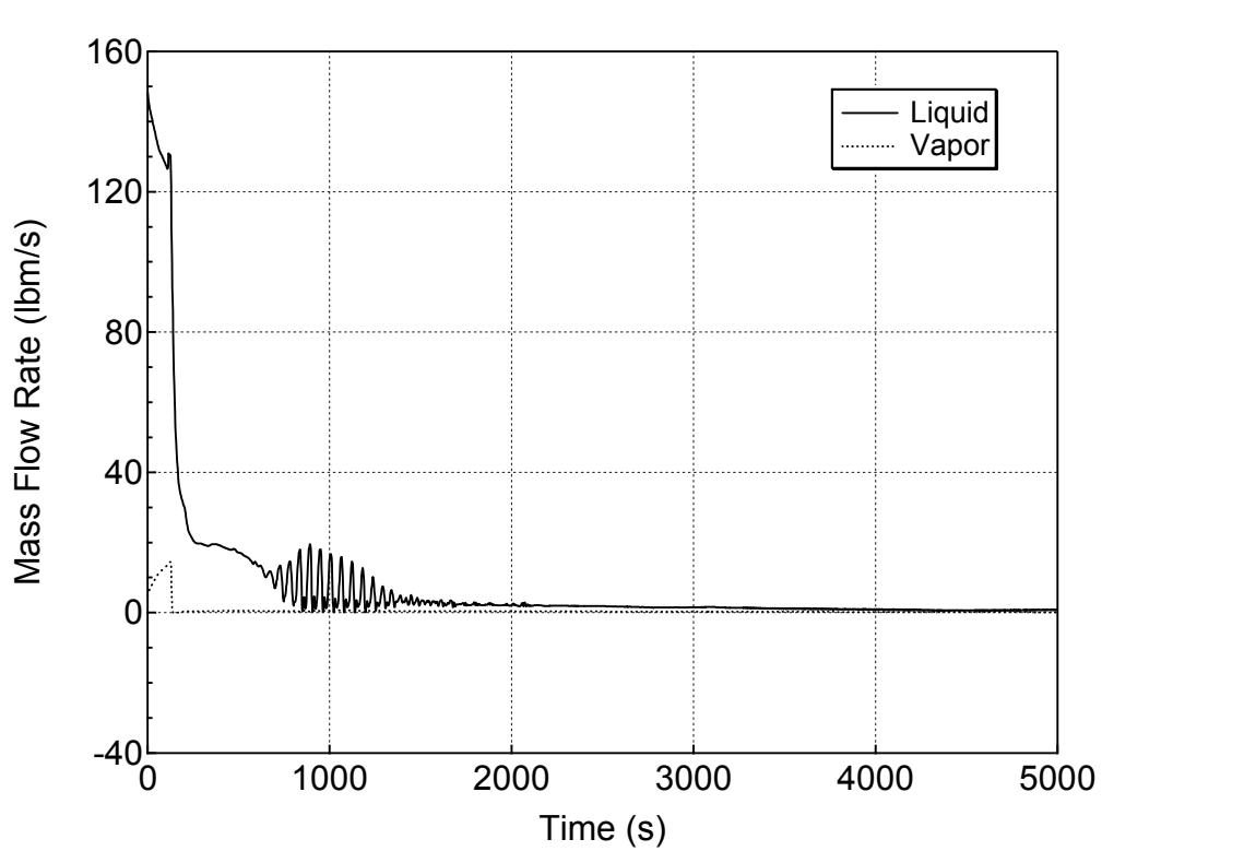
**Figure 5.1.1.b-9 Hot Assembly Exit Vapor and Liquid Mass Flowrates
