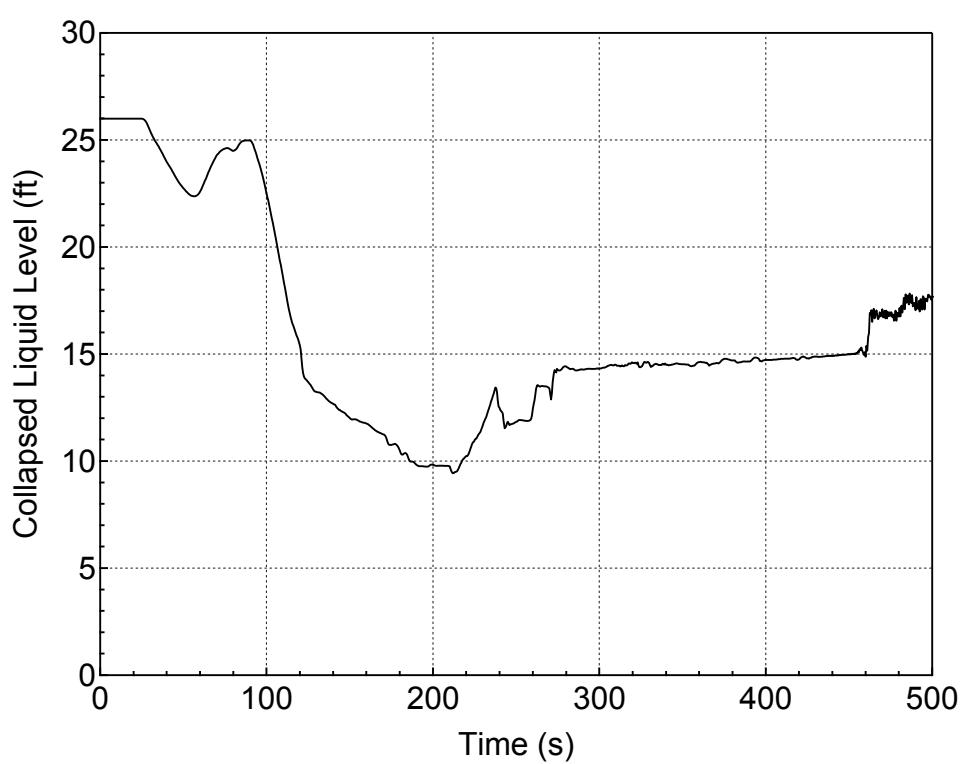
**Figure 5.2.i-6 Downcomer Collapsed Level for 9-inch Break (Bottom)
