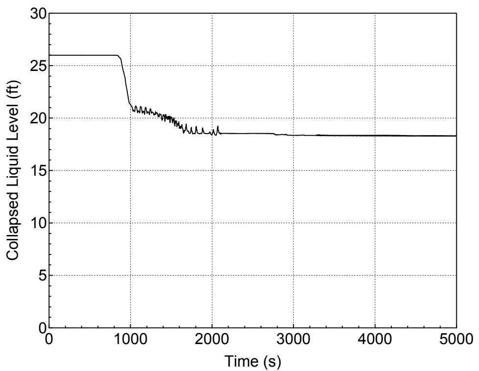
**Figure 5.1.1.b-6 Downcomer Collapsed Level for 2-inch Break (Bottom)
