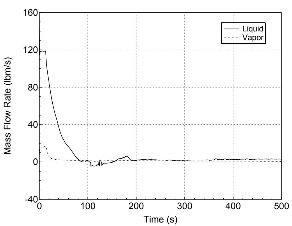
**Figure 5.2.g-9 Hot Assembly Exit Vapor and Liquid Mass Flowrates
