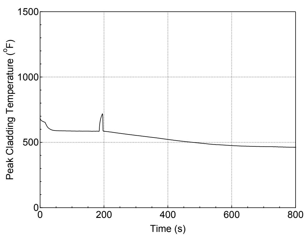
**Figure 5.3.1.a-26 PCT at All Elevations for Hot Rod in Hot Assembly
