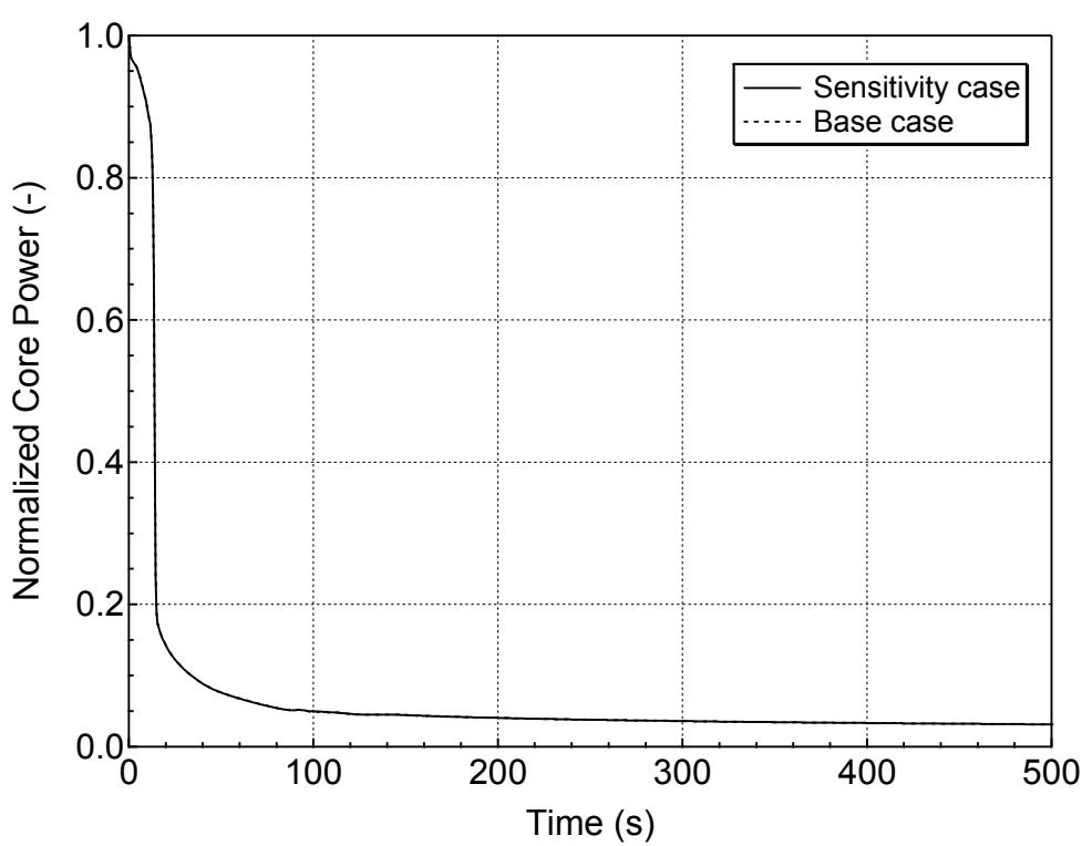
**Figure 5.5.a-2 Normalized Core Power for 7.5-inch Break (Top)
