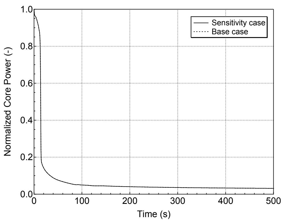
**Figure 5.4.1-2 Normalized Core Power for 7.5-inch Break (Top)
