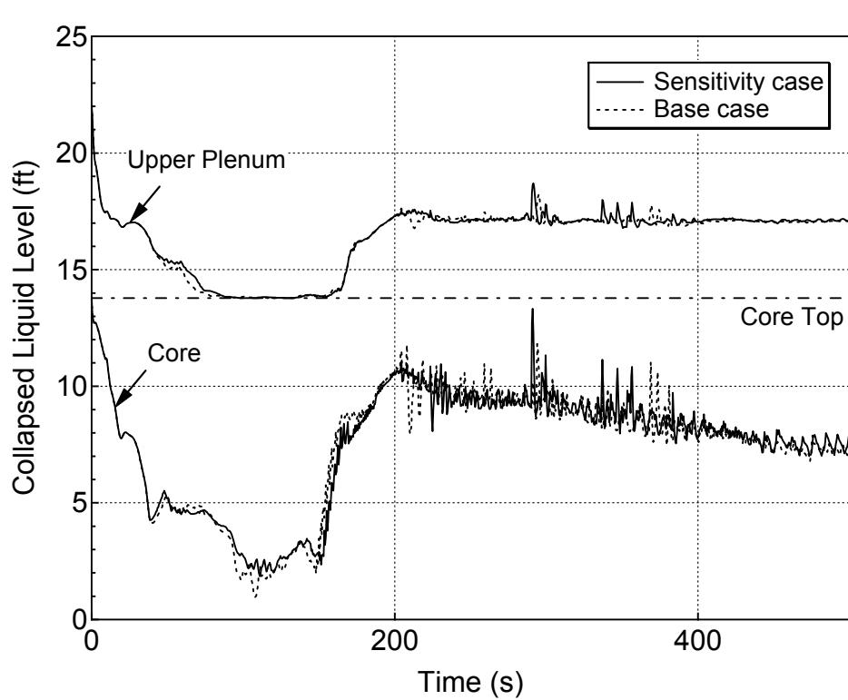
**Figure 5.4.1-22 Average Core and Upper Plenum Collapsed Levels for 1-ft<sup>2</sup> Break (Top)
