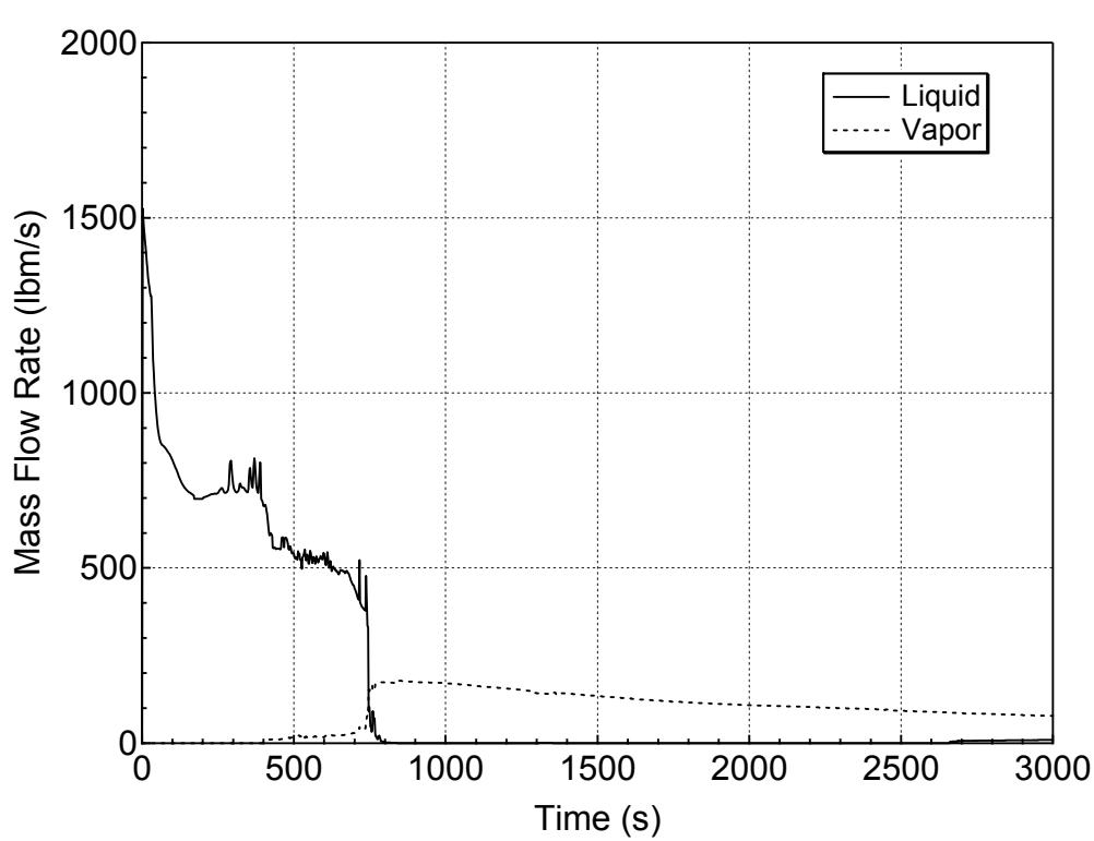
**Figure 5.1.2-3 Liquid and Vapor Discharges through the Break for DVI-line Break
