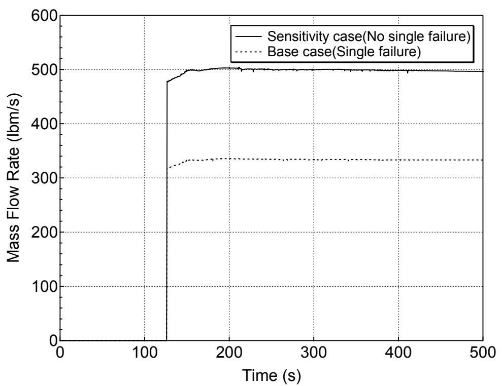
**Figure 5.6.1-19 Safety Injection Mass Flowrate for 1-ft<sup>2</sup> Break (Top)
