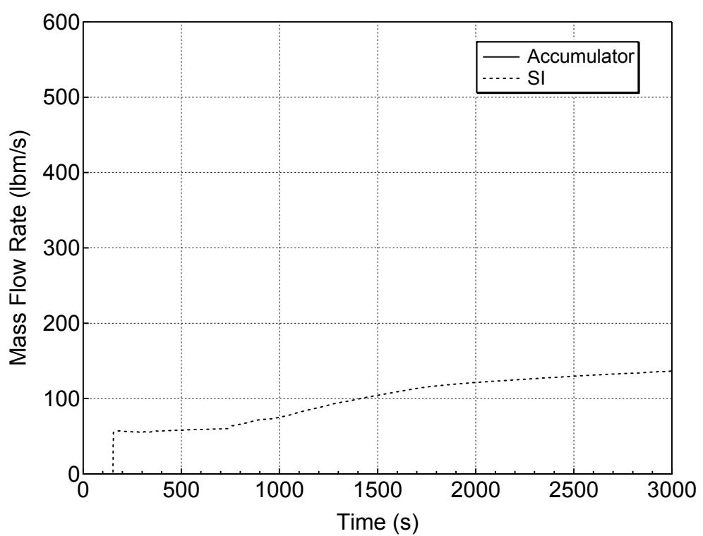
**Figure 5.1.2-4 Accumulator and Safety Injection Mass Flowrates for DVI-line Break
