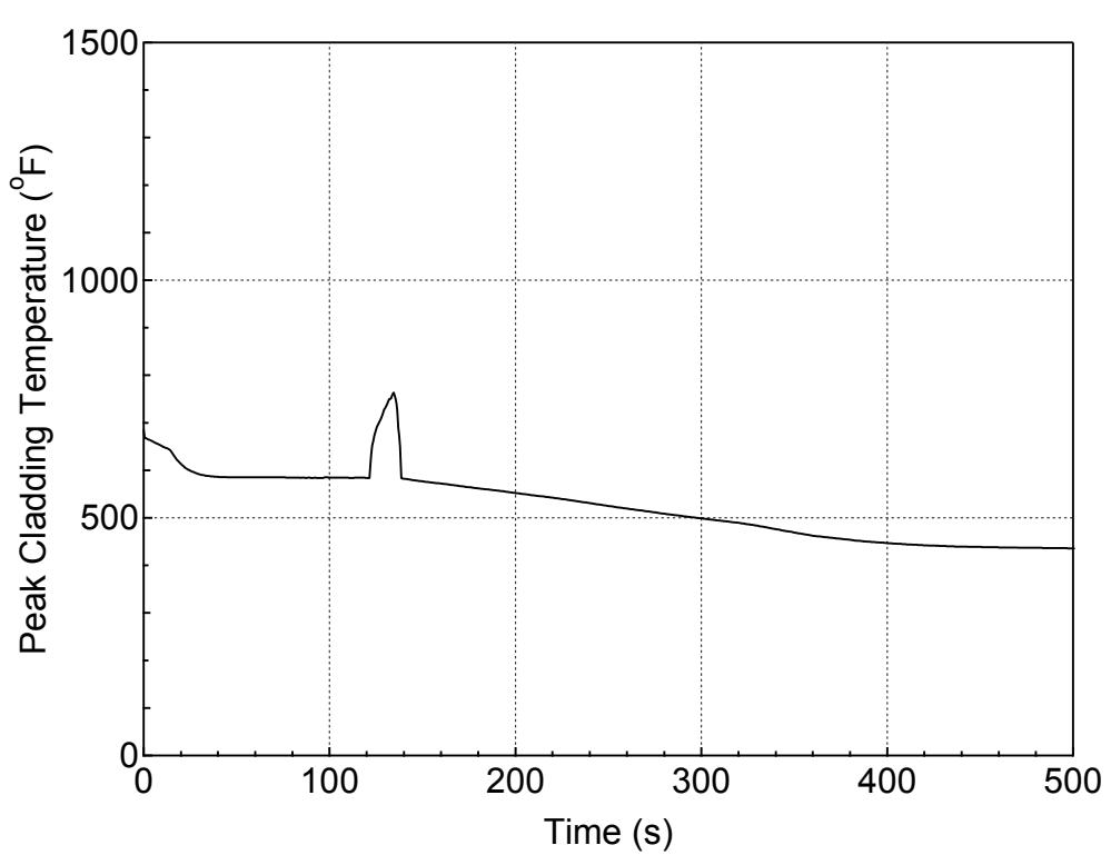
**Figure 5.3.1.d-35 PCT at All Elevations for Hot Rod in Hot Assembly
