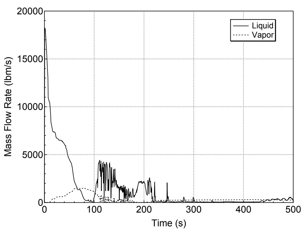
**Figure 5.1.1.c-12 Liquid and Vapor Discharges through the Break
