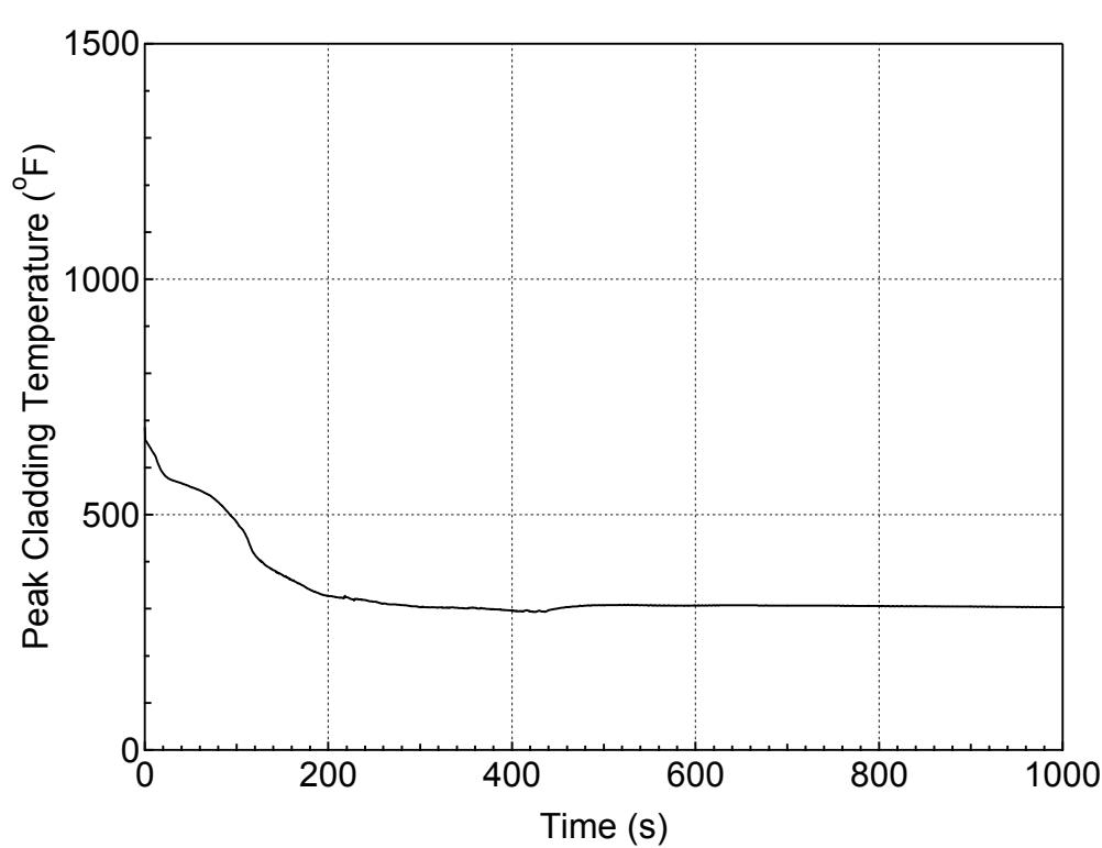
**Figure 5.1.1.b-17 PCT at All Elevations for Hot Rod in Hot Assembly
