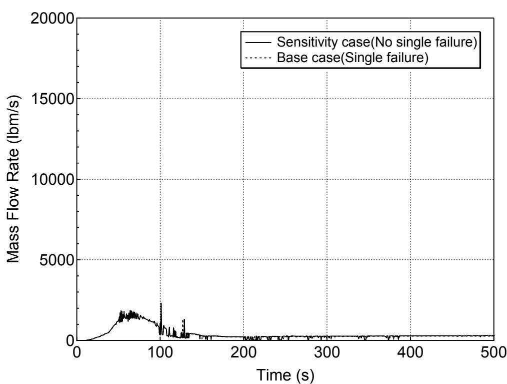
**Figure 5.6.1-17 Vapor Discharge through the Break for 1-ft<sup>2</sup> Break (Top)
