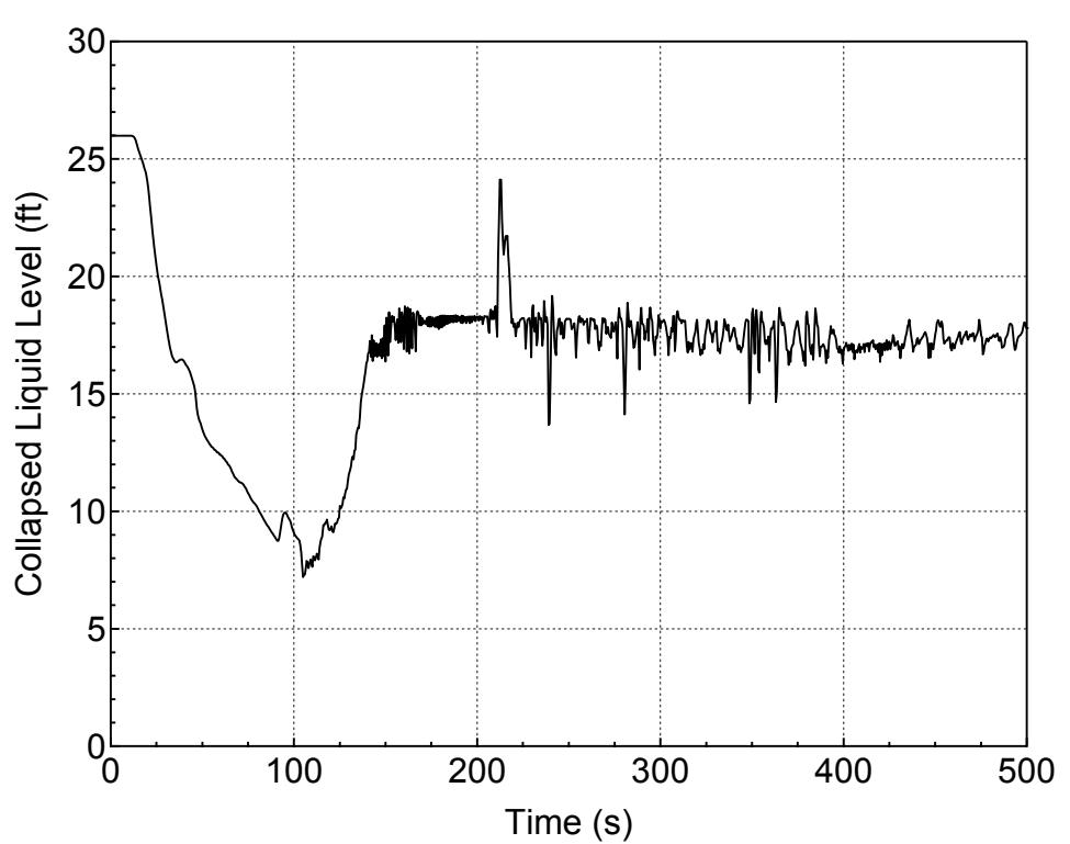
**Figure 5.2.n-6 Downcomer Collapsed Level for 1-ft<sup>2</sup> Break (Bottom)
