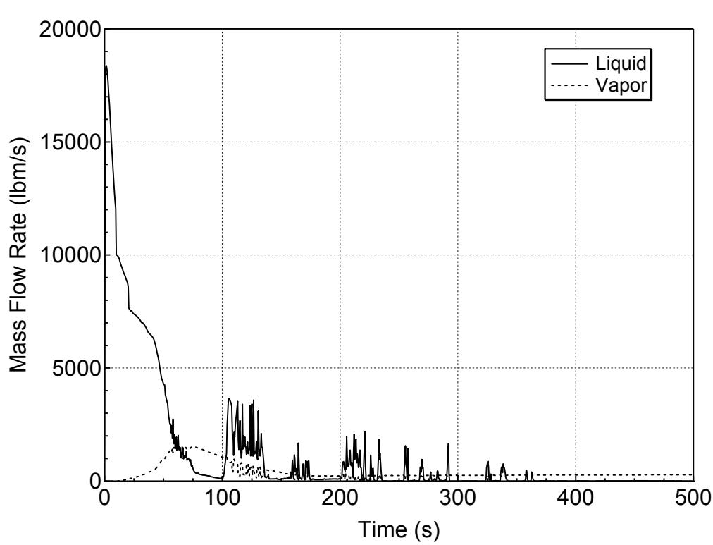
**Figure 5.2.m-3 Liquid and Vapor Discharges through the Break
