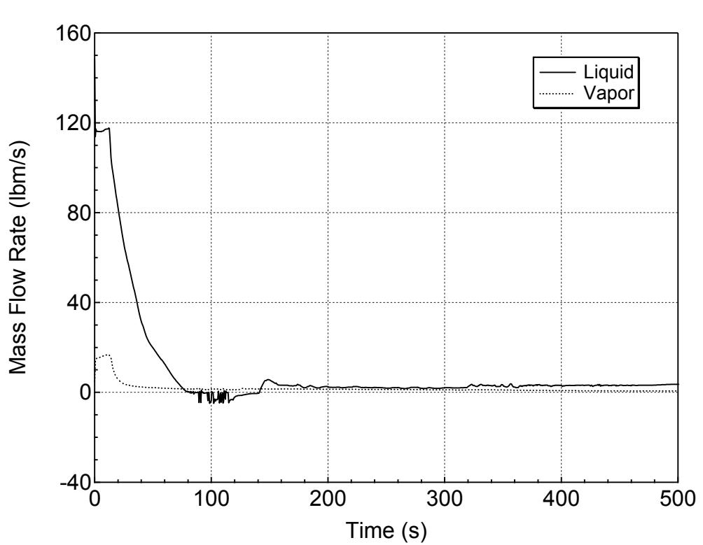
**Figure 5.3.1.d-18 Hot Assembly Exit Vapor and Liquid Mass Flowrates
