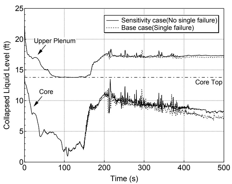
**Figure 5.6.1-22 Average Core and Upper Plenum Collapsed Levels for 1-ft<sup>2</sup> Break (Top)
