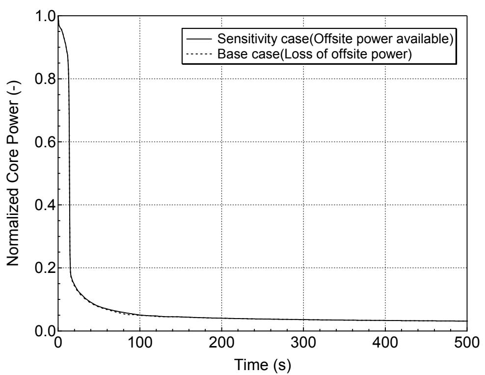
**Figure 5.6.2-2 Normalized Core Power for 7.5-inch Break (Top)
