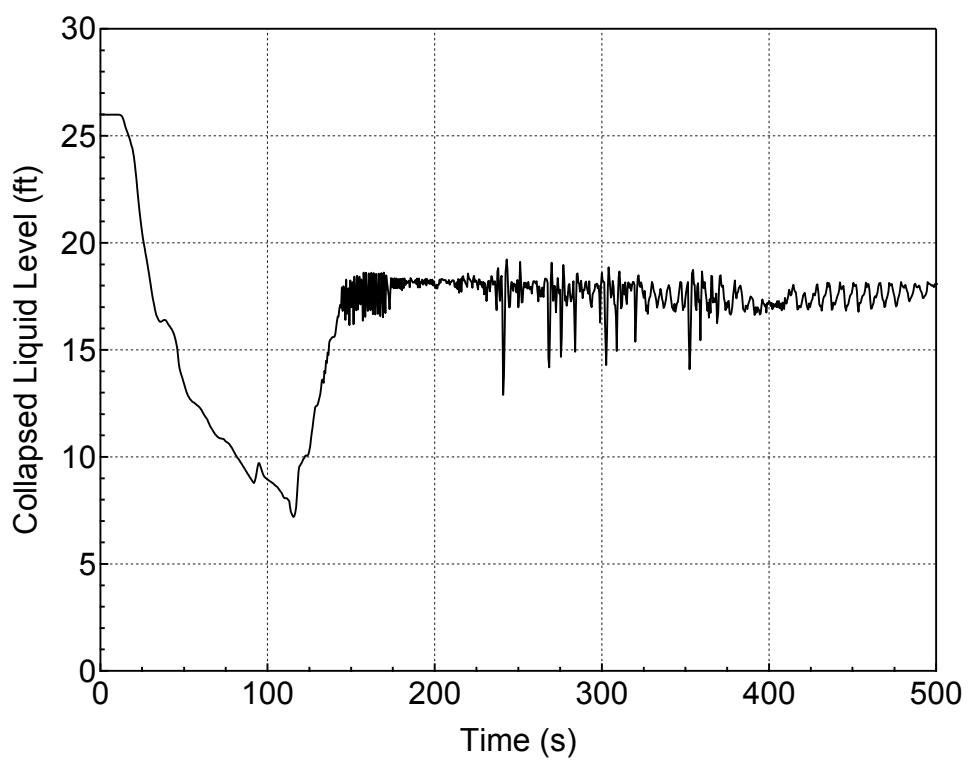
**Figure 5.3.2.c-24 Downcomer Collapsed Level for 1-ft<sup>2</sup> Break (Homogeneous)
