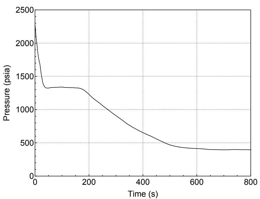
**Figure 5.3.1.b-10 RCS (Pressurizer) Pressure Transient for 6.5-inch Break (Top)
