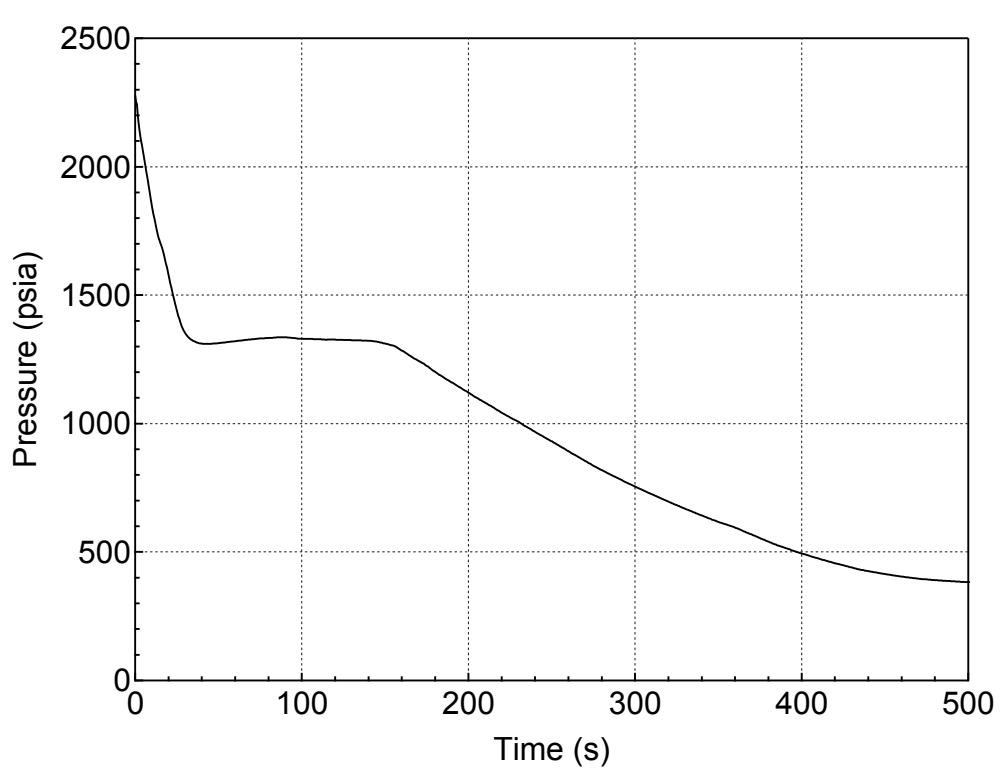
**Figure 5.3.1.c-1 RCS (Pressurizer) Pressure Transient for 7-inch Break (Top)
