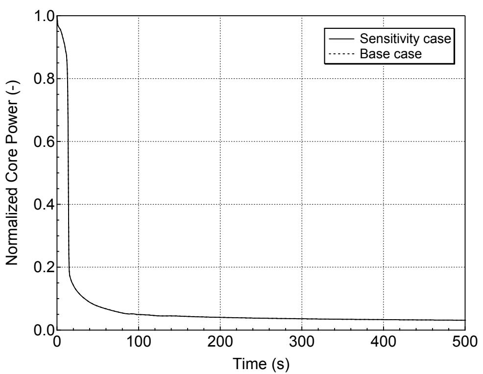
**Figure 5.4.3-2 Normalized Core Power for 7.5-inch Break (Top)
