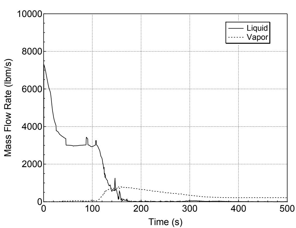
**Figure 5.3.1.e-3 Liquid and Vapor Discharges through the Break for 8-inch Break (Top)
