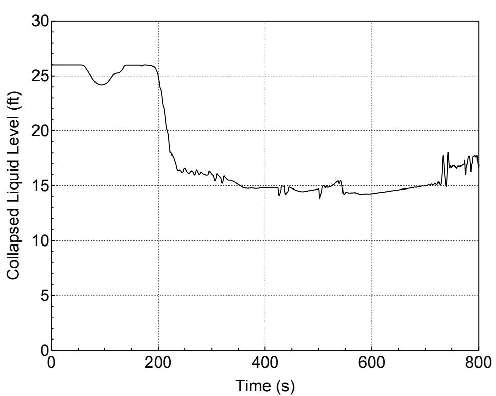
**Figure 5.2.f-6 Downcomer Collapsed Level for 6-inch Break (Bottom)
