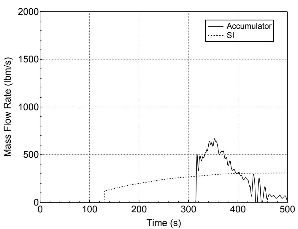
**Figure 5.3.1.d-22 Accumulator and Safety Injection Mass Flowrates
