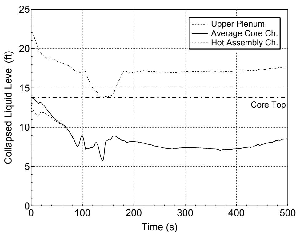
**Figure 5.3.1.c-16 Core and Upper Plenum Collapsed Levels for 7-inch Break (Side)
