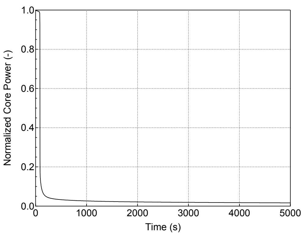
**Figure 5.1.1.a-2 Normalized Core Power for 2-inch Break (Bottom)
