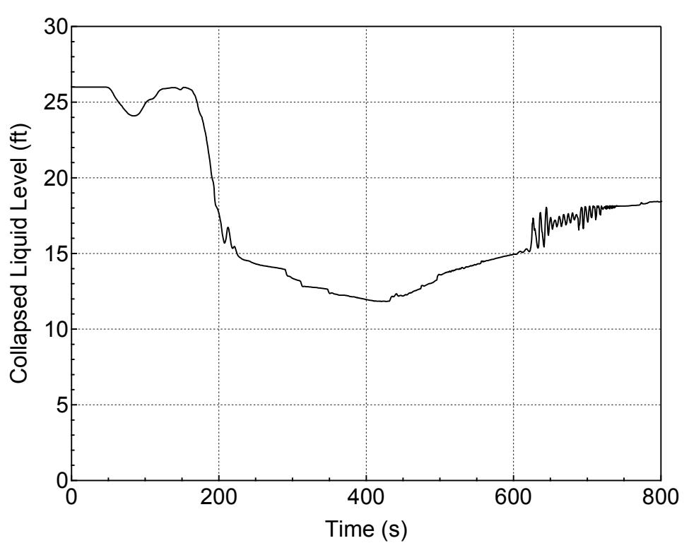
**Figure 5.3.1.b-24 Downcomer Collapsed Level for 6.5-inch Break (Side)
