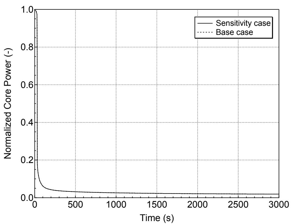
**Figure 5.5.c-2 Normalized Core Power for DVI-line Break
