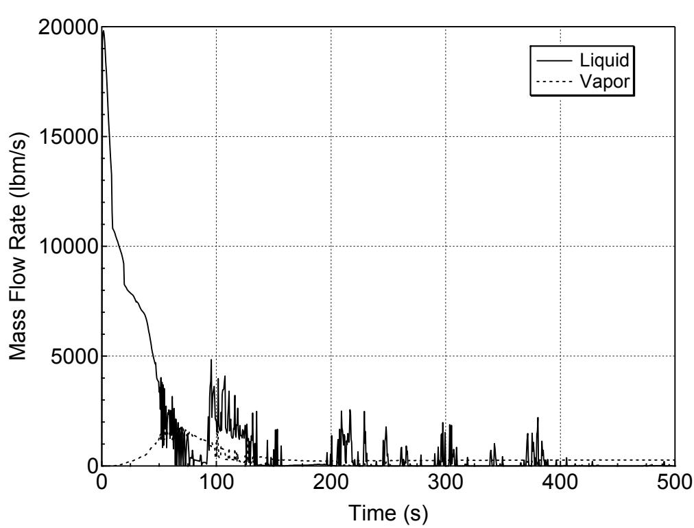
**Figure 5.3.2.c-3 Liquid and Vapor Discharges through the Break for 1-ft<sup>2</sup> Break (Top)
