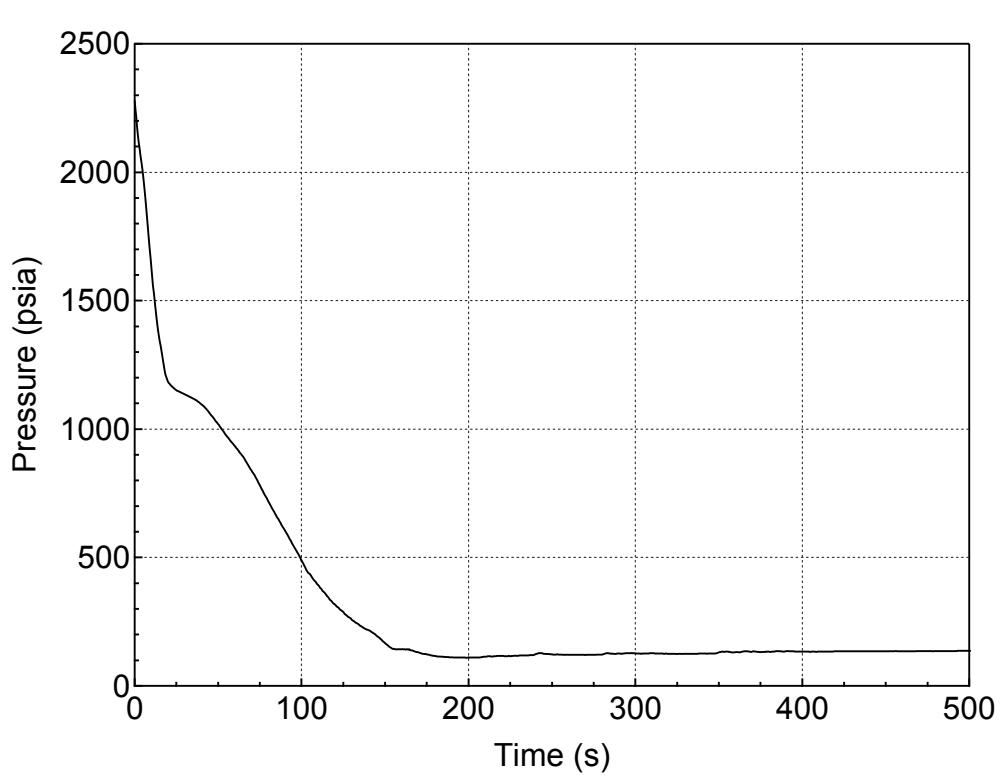
**Figure 5.2.n-1 RCS (Pressurizer) Pressure Transient for 1-ft<sup>2</sup> Break (Bottom)
