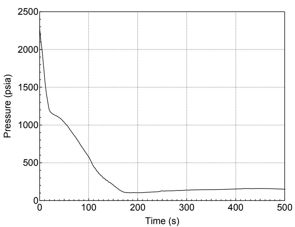
**Figure 5.1.1.c-10 RCS (Pressurizer) Pressure Transient for 1-ft<sup>2</sup> Break (Bottom)
