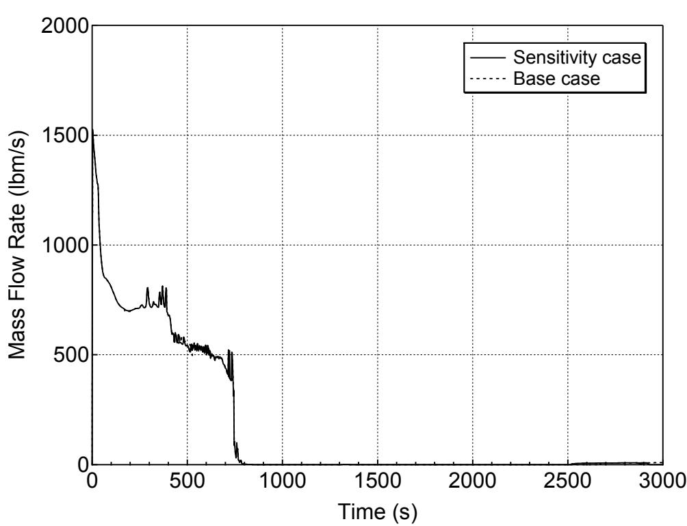
**Figure 5.5.c-3 Liquid Discharge through the Break for DVI-line Break
