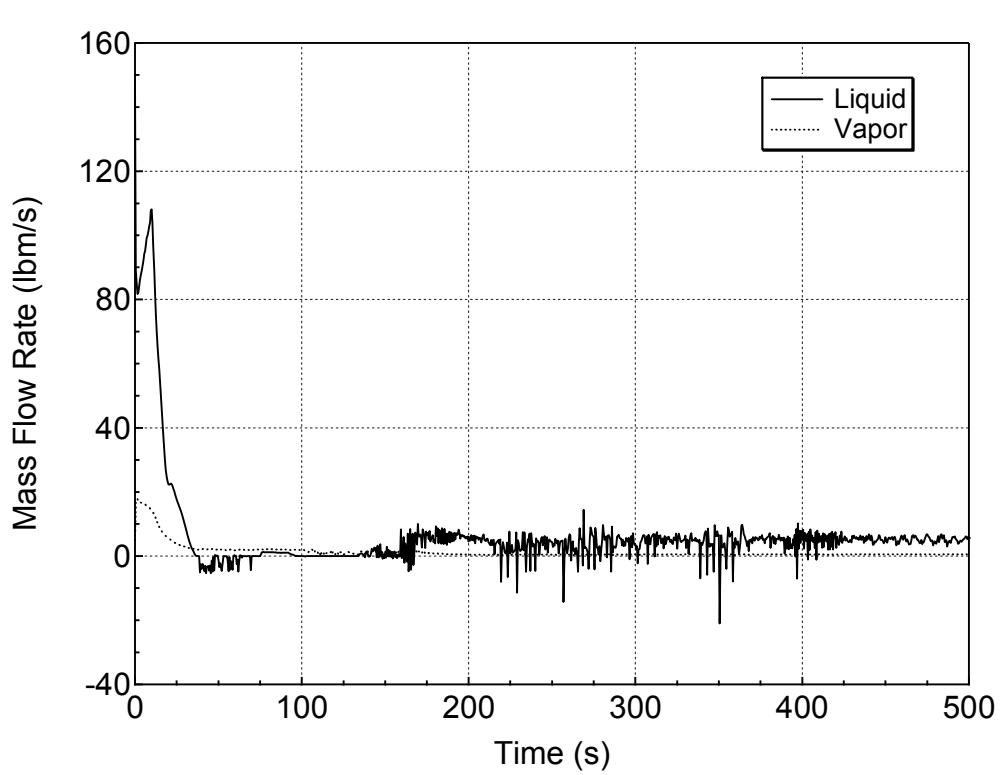
**Figure 5.3.2.c-18 Hot Assembly Exit Vapor and Liquid Mass Flowrates
