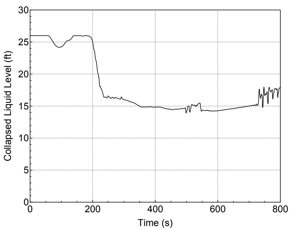
**Figure 5.3.1.a-24 Downcomer Collapsed Level for 6-inch Break (Homogeneous)
