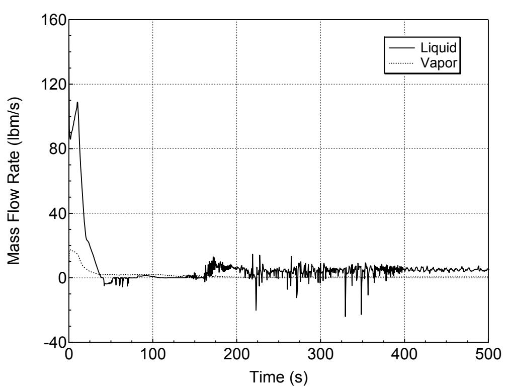
**Figure 5.3.2.b-27 Hot Assembly Exit Vapor and Liquid Mass Flowrates for 13-inch Break (Homogeneous) (Break Orientation Sensitivity Study)**
