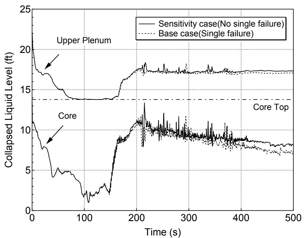
**Figure 5.6.1-23 Hot Assembly Core and Upper Plenum Collapsed Levels
