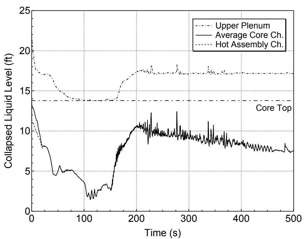
**Figure 5.3.2.b-7 Core and Upper Plenum Collapsed Levels for 13-inch Break (Top)
