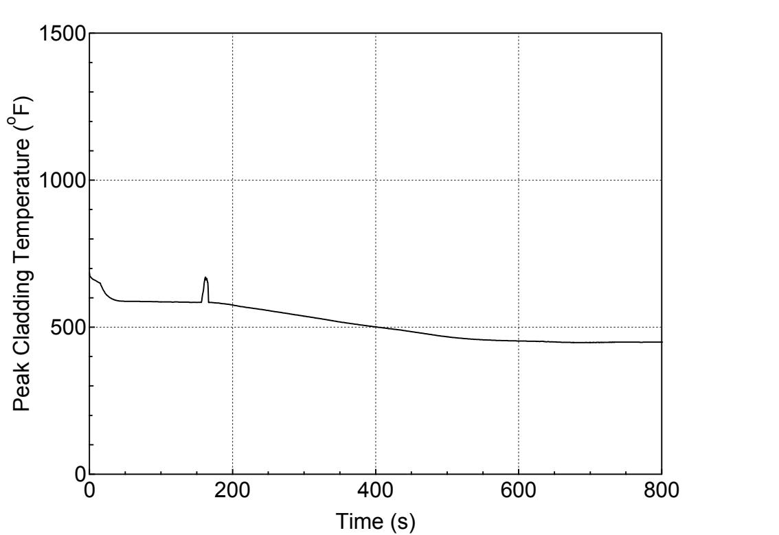
**Figure 5.3.1.b-26 PCT at All Elevations for Hot Rod in Hot Assembly
