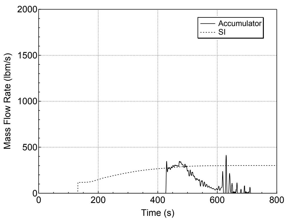
**Figure 5.3.1.b-13 Accumulator and Safety Injection Mass Flowrates
