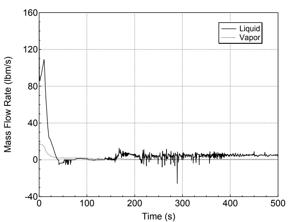
**Figure 5.2.m-9 Hot Assembly Exit Vapor and Liquid Mass Flowrates
