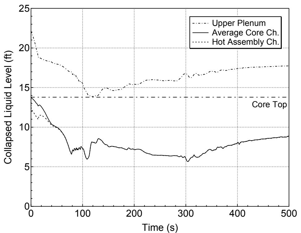
**Figure 5.3.1.e-25 Core and Upper Plenum Collapsed Levels
