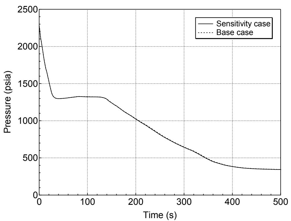
**Figure 5.4.1-1 RCS (Pressurizer) Pressure Transient for 7.5-inch Break (Top)
