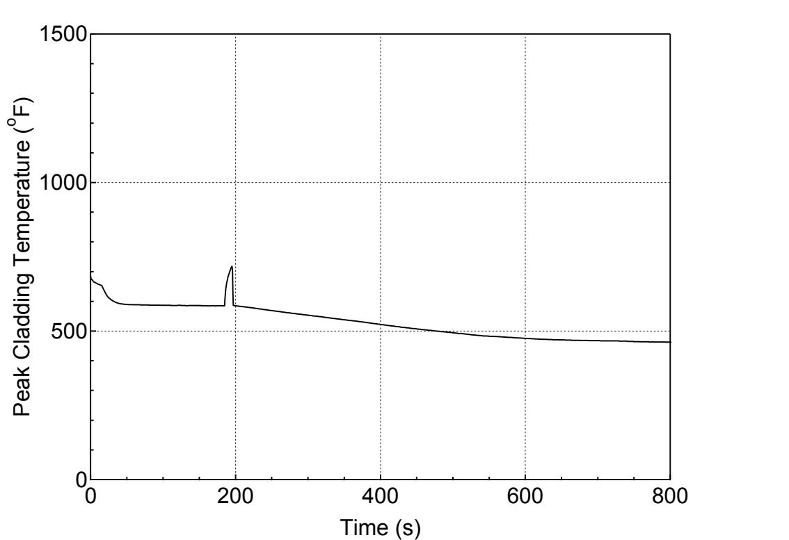
**Figure 5.2.f-8 PCT at All Elevations for Hot Rod in Hot Assembly
