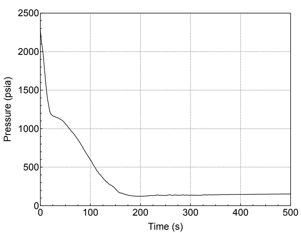
**Figure 5.2.m-1 RCS (Pressurizer) Pressure Transient for 13-inch Break (Bottom)
