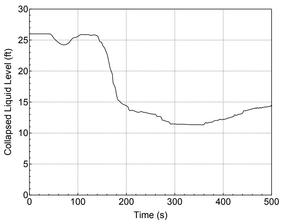
**Figure 5.3.1.c-24 Downcomer Collapsed Level for 7-inch Break (Homogeneous)
