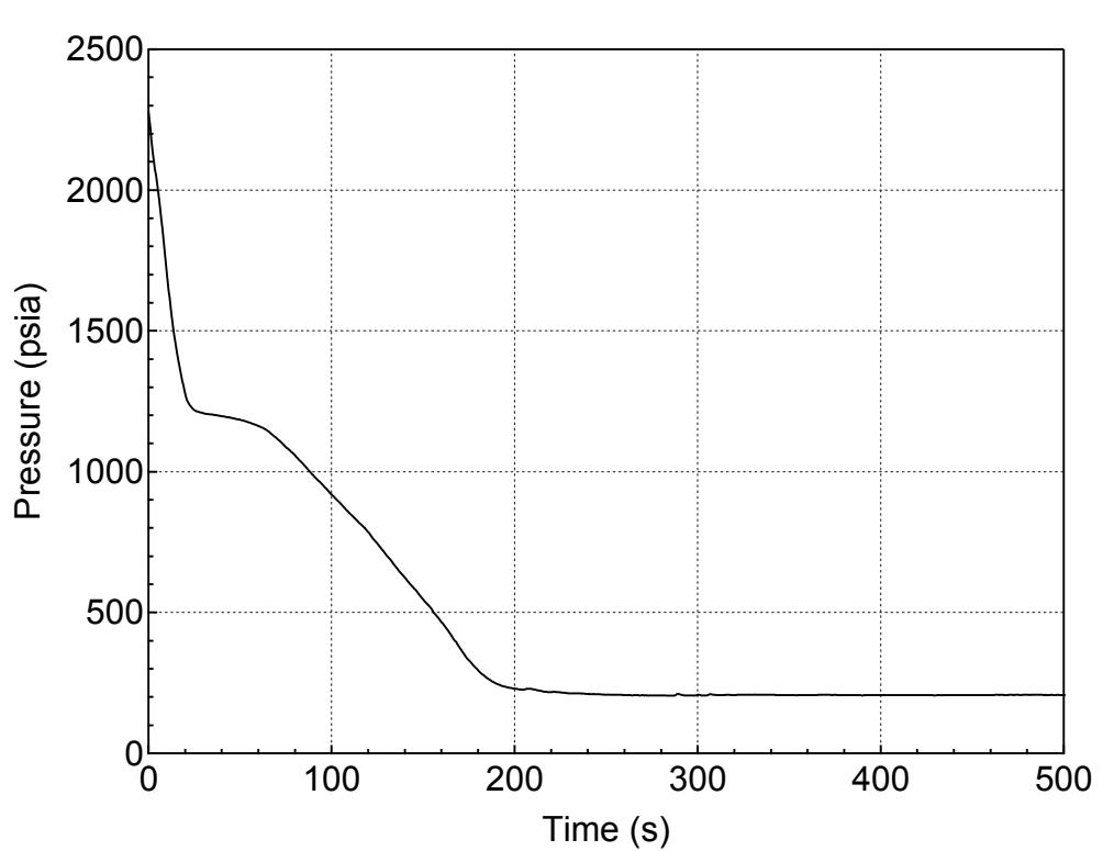
**Figure 5.2.k-1 RCS (Pressurizer) Pressure Transient for 11-inch Break (Bottom)
