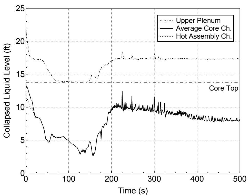
**Figure 5.3.2.a-7 Core and Upper Plenum Collapsed Levels for 12-inch Break (Top)
