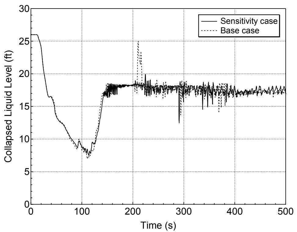
**Figure 5.4.1-21 Downcomer Collapsed Level for 1-ft<sup>2</sup> Break (Top)
