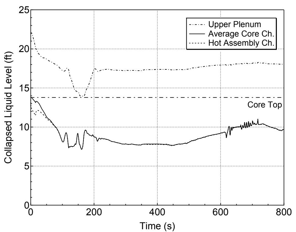
**Figure 5.3.1.b-16 Core and Upper Plenum Collapsed Levels for 6.5-inch Break (Top)
