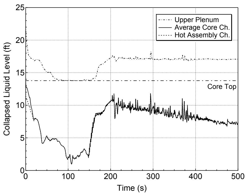
**Figure 5.3.2.c-7 Core and Upper Plenum Collapsed Levels for 1-ft<sup>2</sup> Break (Top)
