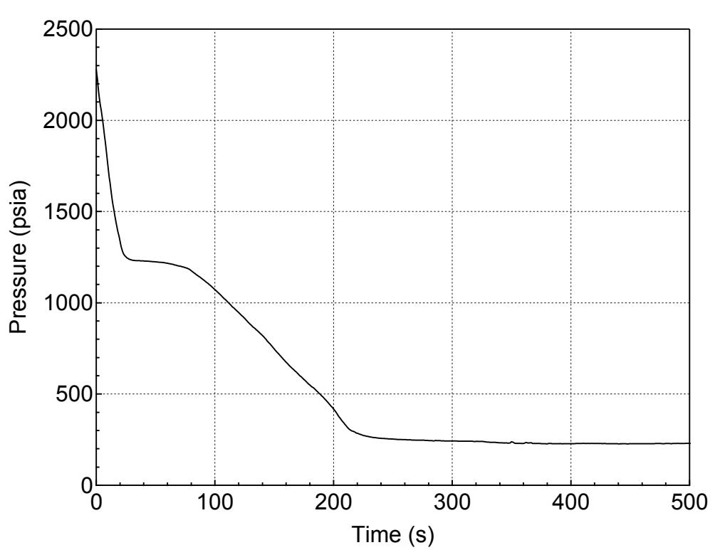
**Figure 5.2.j-1 RCS (Pressurizer) Pressure Transient for 10-inch Break (Bottom)
