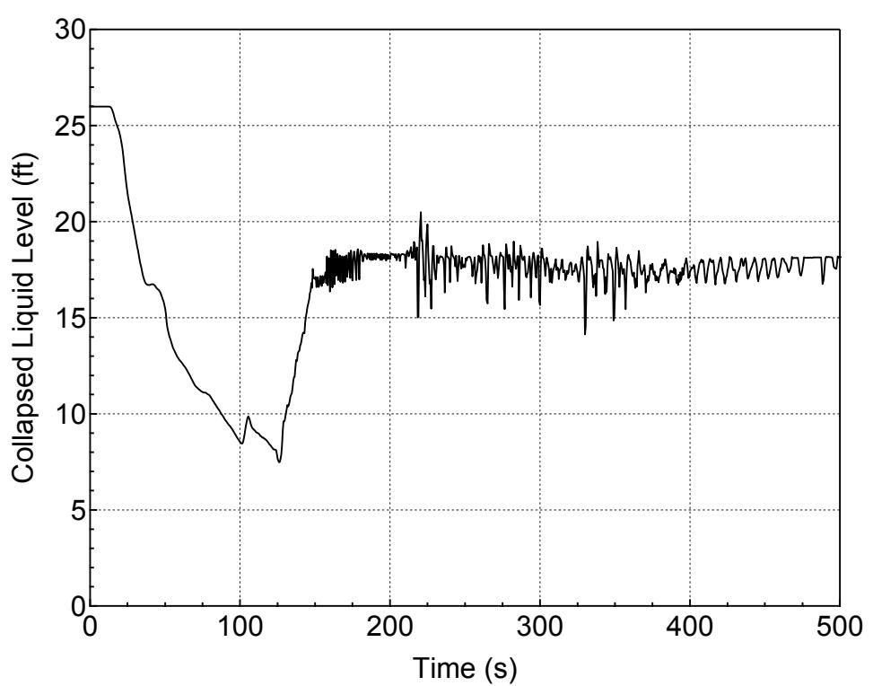
**Figure 5.3.2.b-24 Downcomer Collapsed Level for 13-inch Break (Homogeneous)
