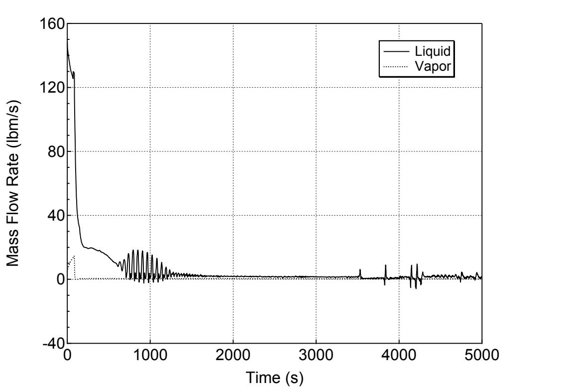
**Figure 5.1.1.a-9 Hot Assembly Exit Vapor and Liquid Mass Flowrates
