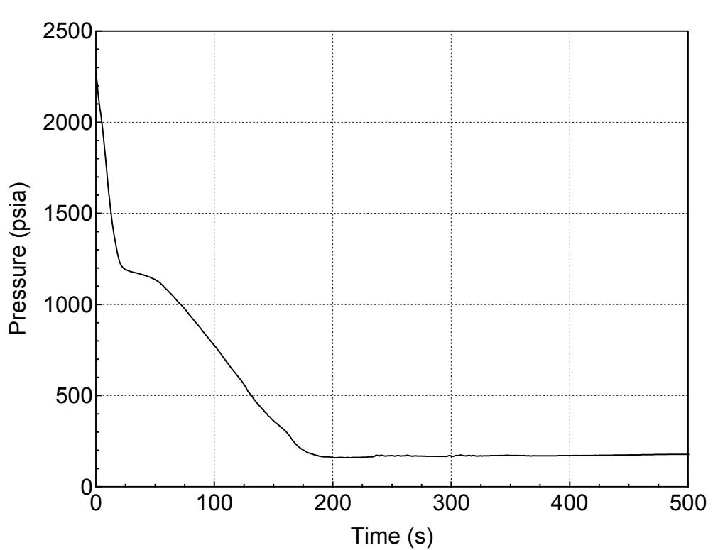
**Figure 5.2.I-1 RCS (Pressurizer) Pressure Transient for 12-inch Break (Bottom)
