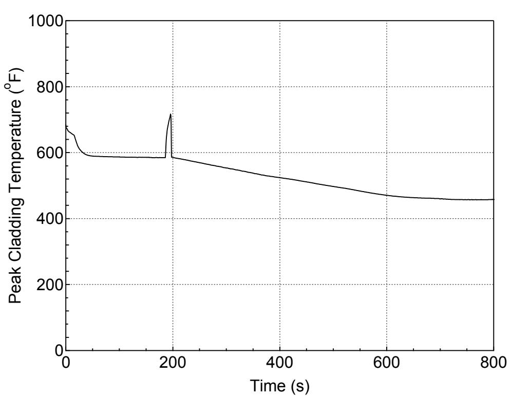
**Figure 5.3.1.a-8 PCT at All Elevations for Hot Rod in Hot Assembly
