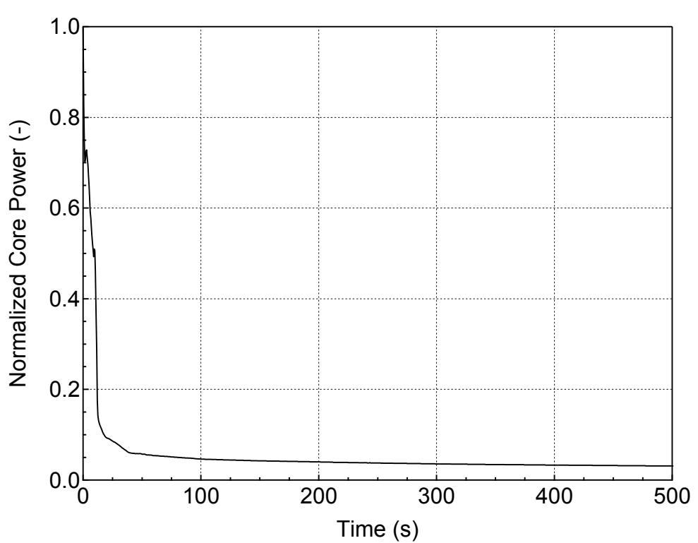
**Figure 5.2.n-2 Normalized Core Power for 1-ft<sup>2</sup> Break (Bottom)
