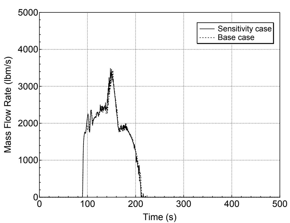
**Figure 5.5.b-5 Accumulator Injection Mass Flowrate for 1-ft<sup>2</sup> Break (Top)
