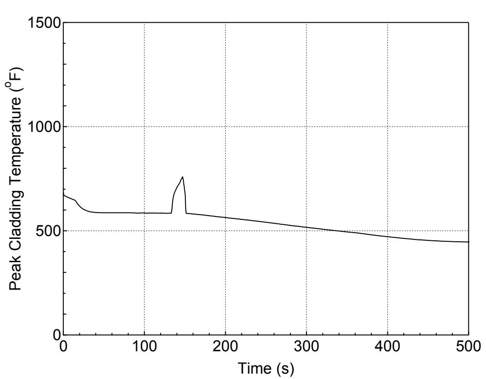
**Figure 5.3.1.c-8 PCT at All Elevations for Hot Rod in Hot Assembly
