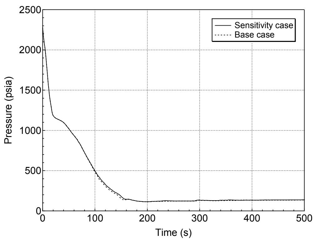
**Figure 5.4.1-14 RCS (Pressurizer) Pressure Transient for 1-ft<sup>2</sup> Break (Top)
