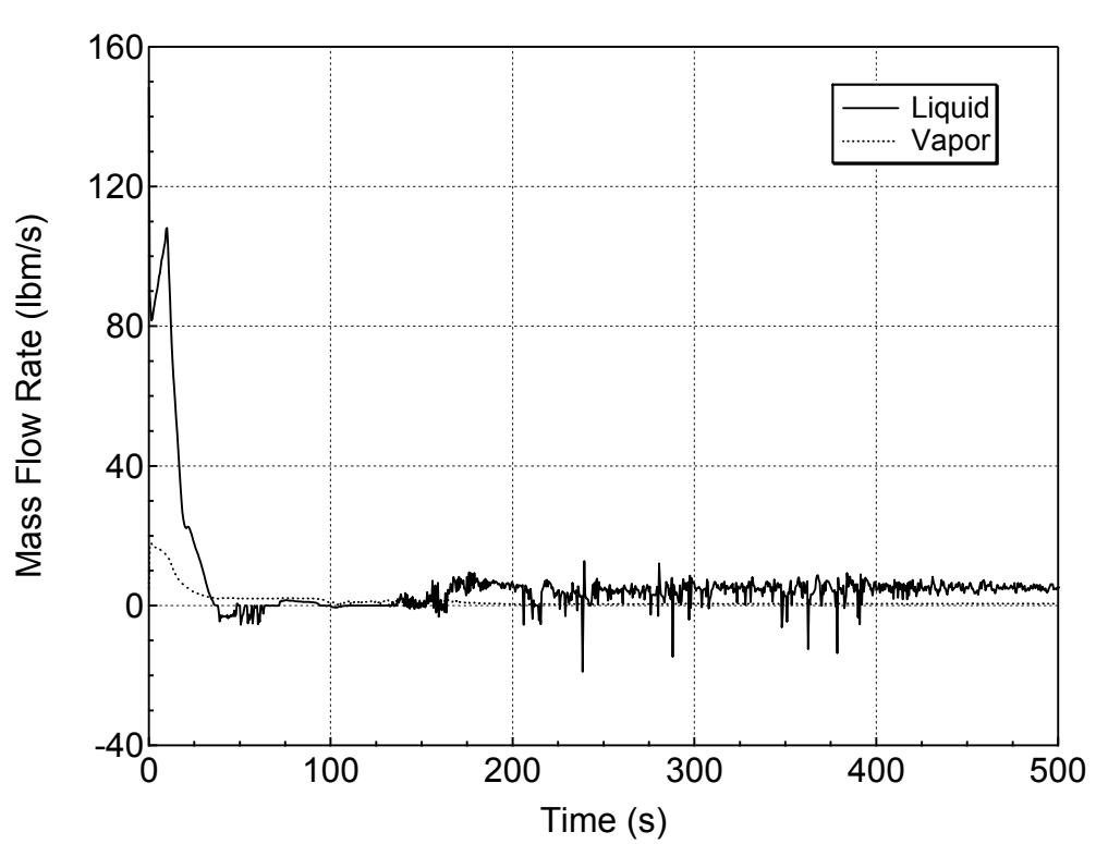
**Figure 5.1.1.a-18 Hot Assembly Exit Vapor and Liquid Mass Flowrates
