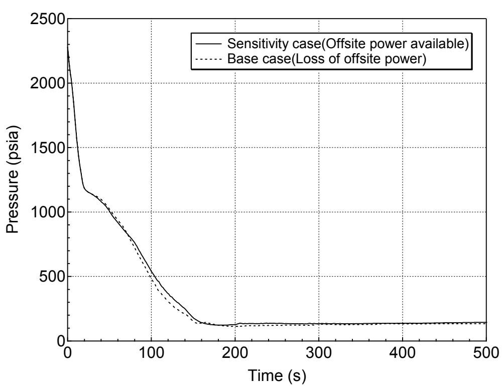
**Figure 5.6.2-14 RCS (Pressurizer) Pressure Transient for 1-ft<sup>2</sup> Break (Top)
