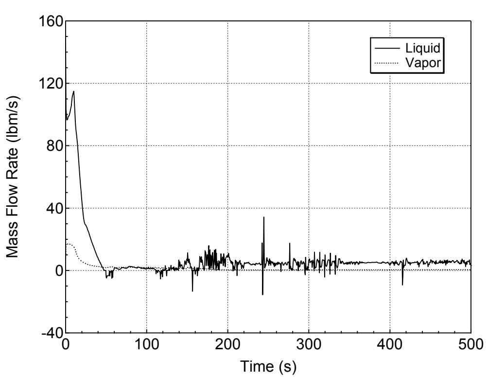
**Figure 5.1.1.c-18 Hot Assembly Exit Vapor and Liquid Mass Flowrates
