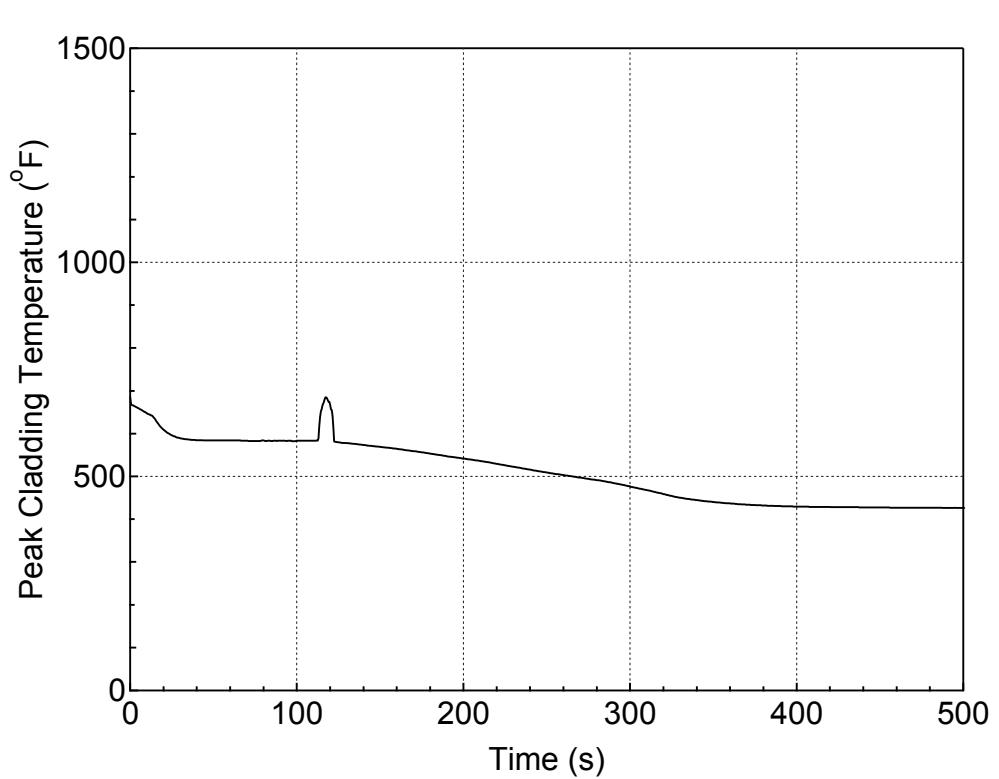
**Figure 5.3.1.e-8 PCT at All Elevations for Hot Rod in Hot Assembly
