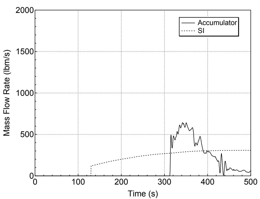
**Figure 5.3.1.d-4 Accumulator and Safety Injection Mass Flowrates
