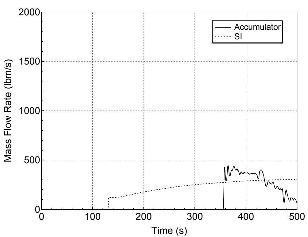
**Figure 5.3.1.c-4 Accumulator and Safety Injection Mass Flowrates
