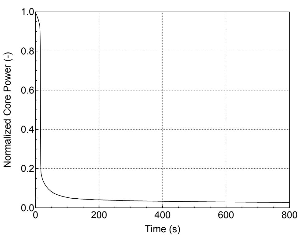
**Figure 5.2.f-2 Normalized Core Power for 6-inch Break (Bottom)
