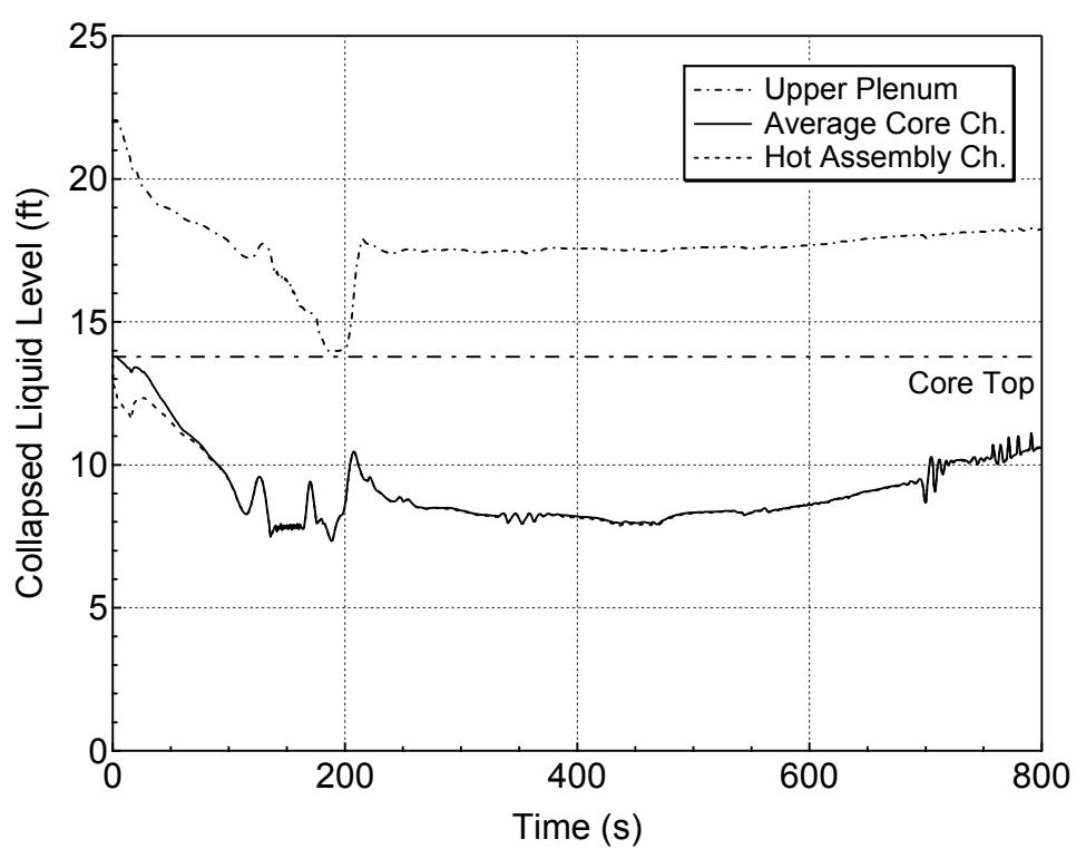
**Figure 5.3.1.a-16 Core and Upper Plenum Collapsed Levels for 6-inch Break (Side)
