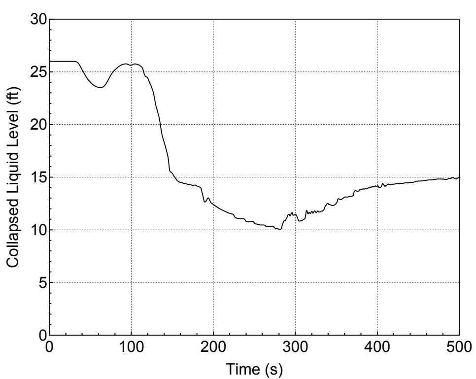
**Figure 5.2.h-6 Downcomer Collapsed Level for 8-inch Break (Bottom)
