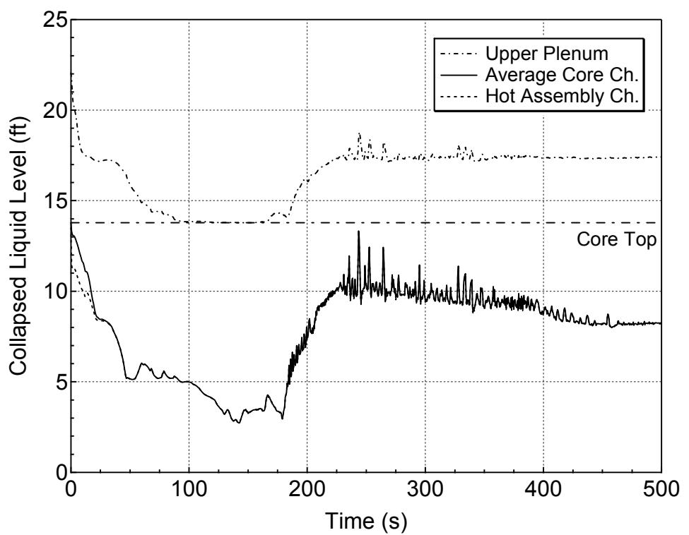
**Figure 5.3.2.a-25 Core and Upper Plenum Collapsed Levels
