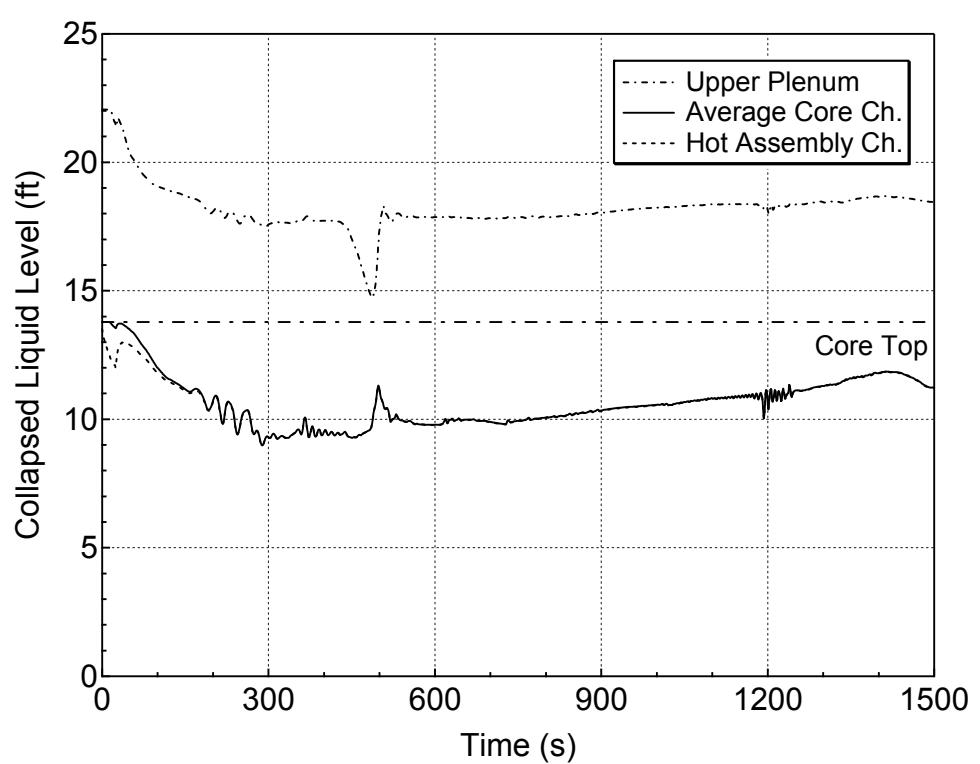
**Figure 5.2.d-7 Core and Upper Plenum Collapsed Levels for 4-inch Break (Bottom)
