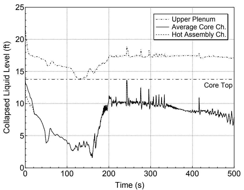
**Figure 5.1.1.c-16 Core and Upper Plenum Collapsed Levels for 1-ft<sup>2</sup> Break (Bottom)
