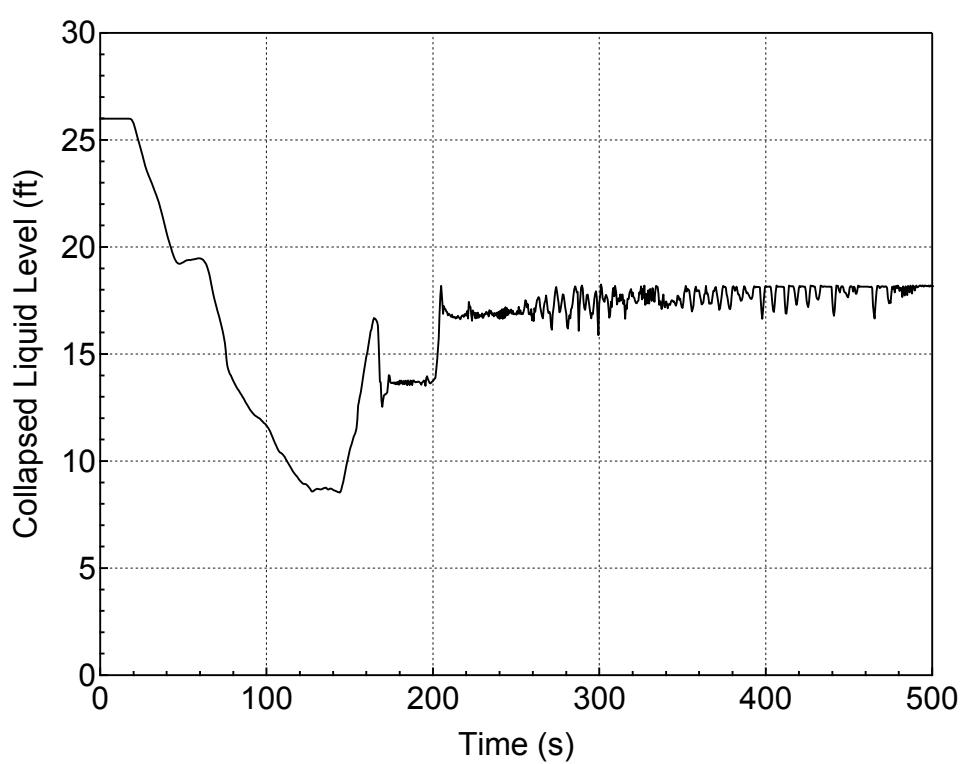
**Figure 5.2.k-6 Downcomer Collapsed Level for 11-inch Break (Bottom)
