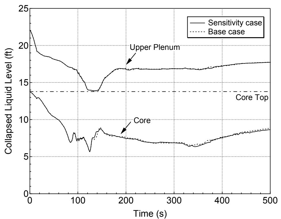
**Figure 5.4.3-9 Average Core and Upper Plenum Collapsed Levels
