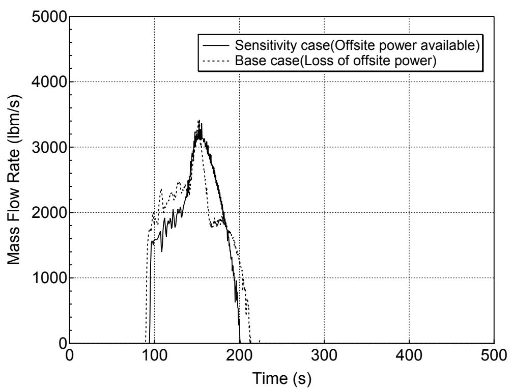
**Figure 5.6.2-18 Accumulator Mass Flowrate for 1-ft<sup>2</sup> Break (Top)
