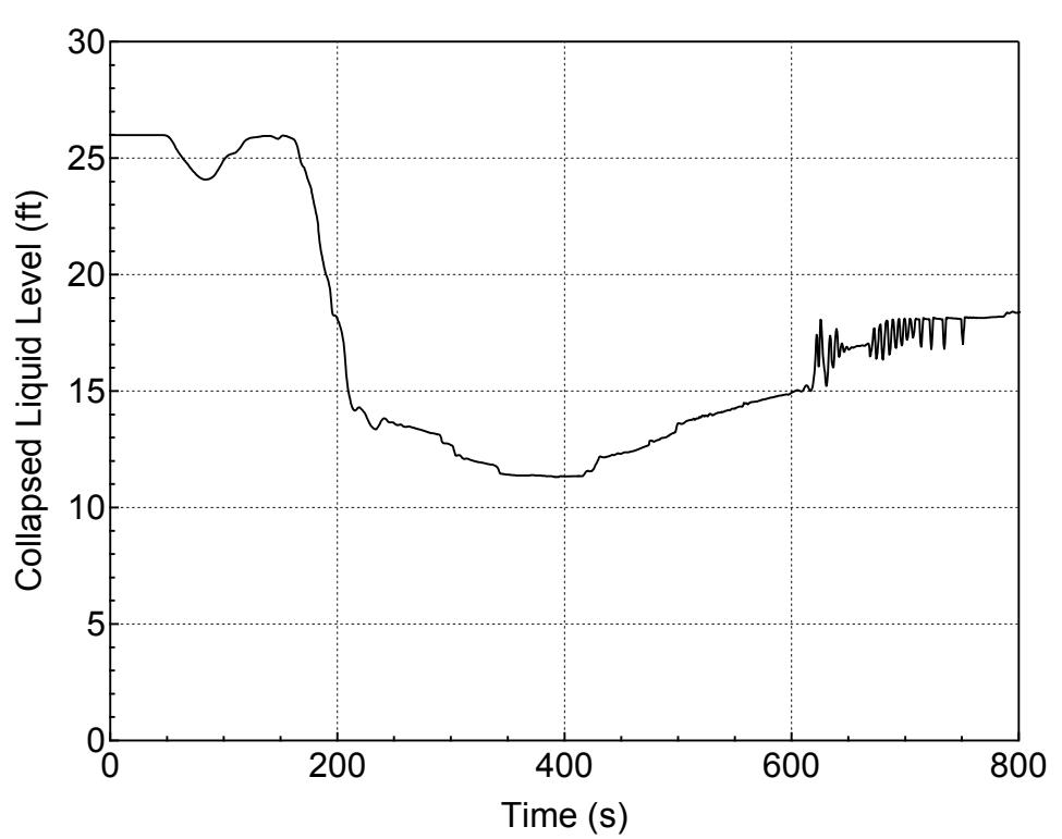
**Figure 5.3.1.b-6 Downcomer Collapsed Level for 6.5-inch Break (Bottom)
