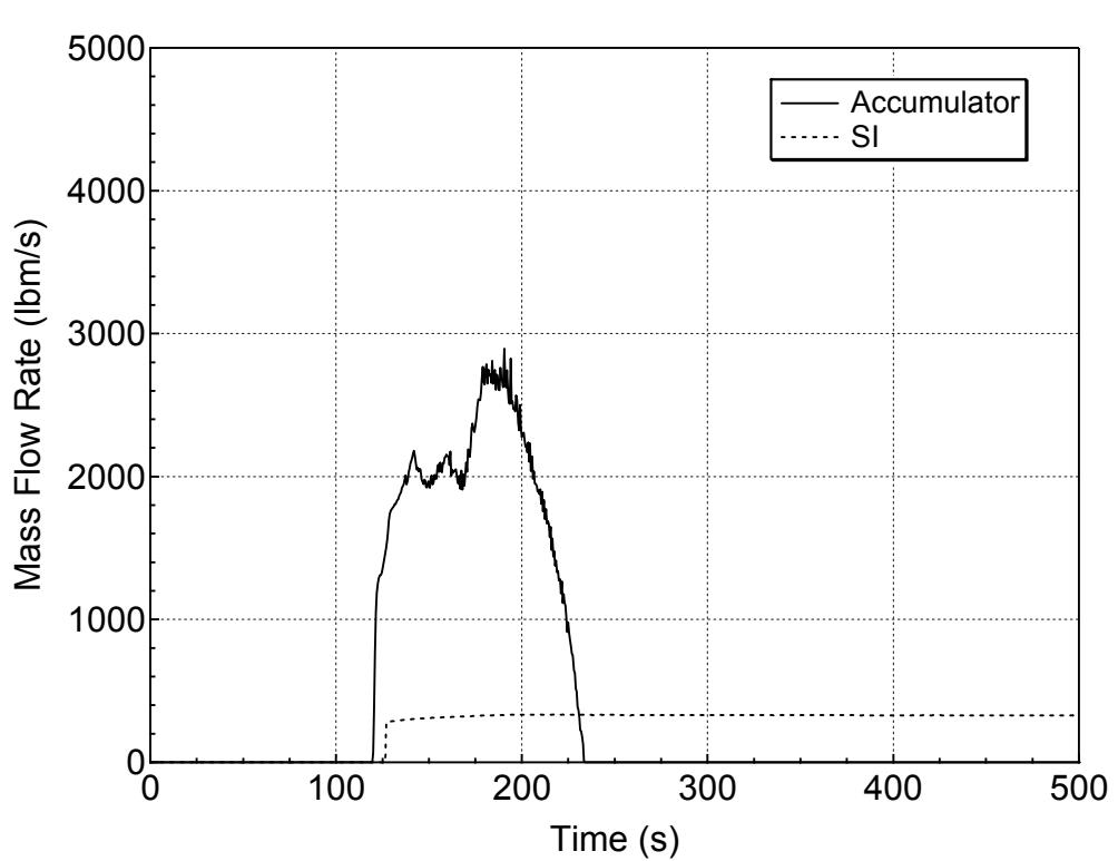
**Figure 5.3.2.a-13 Accumulator and Safety Injection Mass Flowrates
