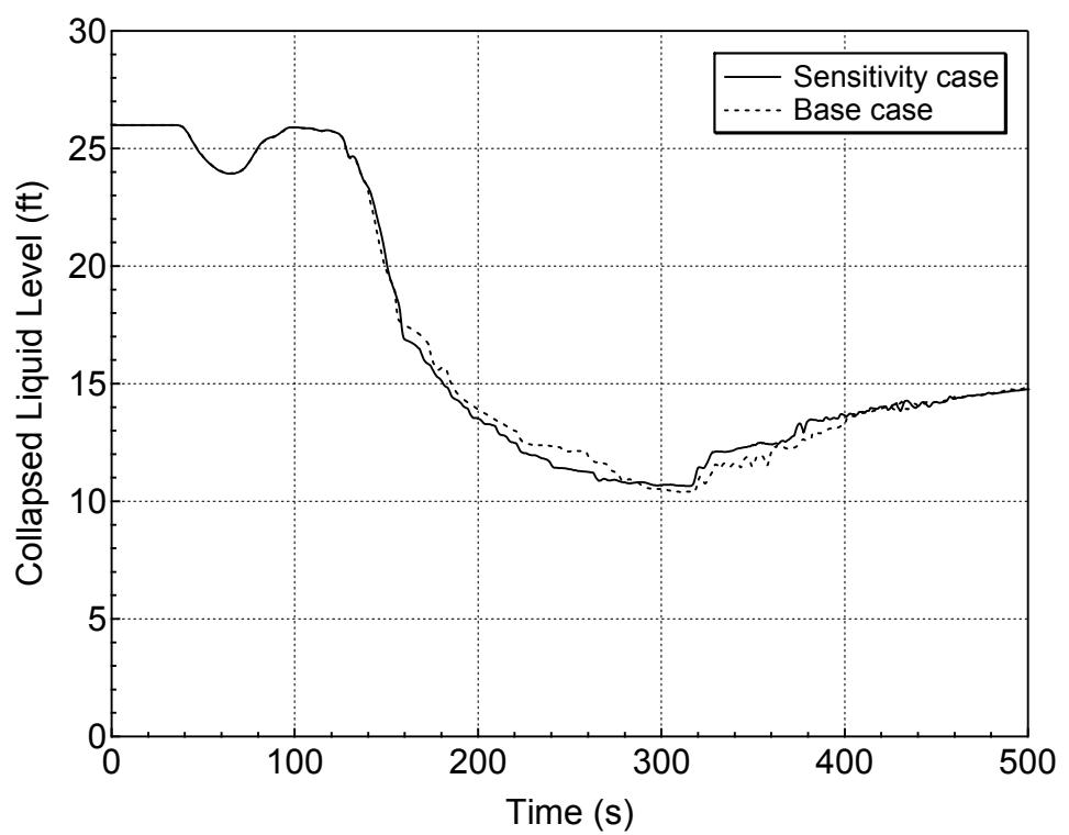
**Figure 5.4.3-8 Downcomer Collapsed Level for 7.5-inch Break (Top)
