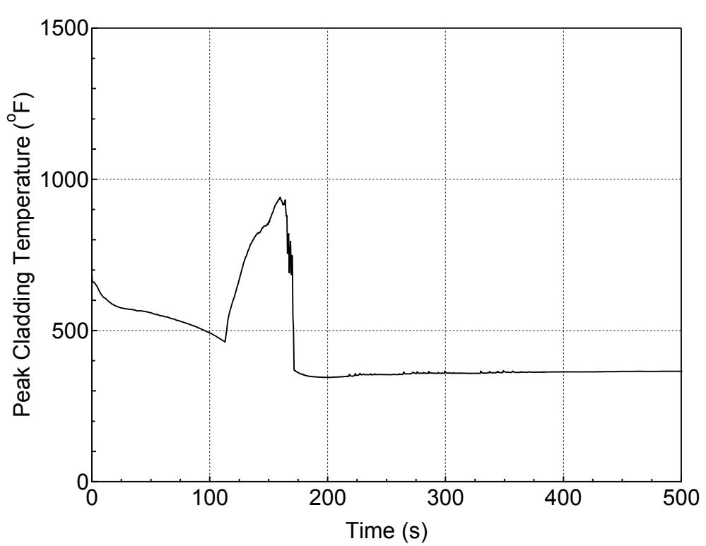
**Figure 5.3.2.b-26 PCT at All Elevations for Hot Rod in Hot Assembly
