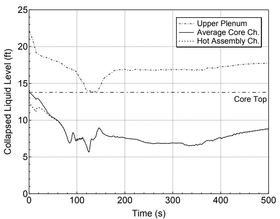
**Figure 5.3.1.d-16 Core and Upper Plenum Collapsed Levels for 7.5-inch Break (Top)
