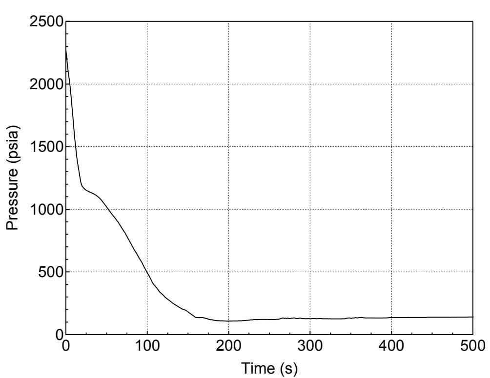
**Figure 5.3.2.c-10 RCS (Pressurizer) Pressure Transient for 1-ft<sup>2</sup> Break (Side)
