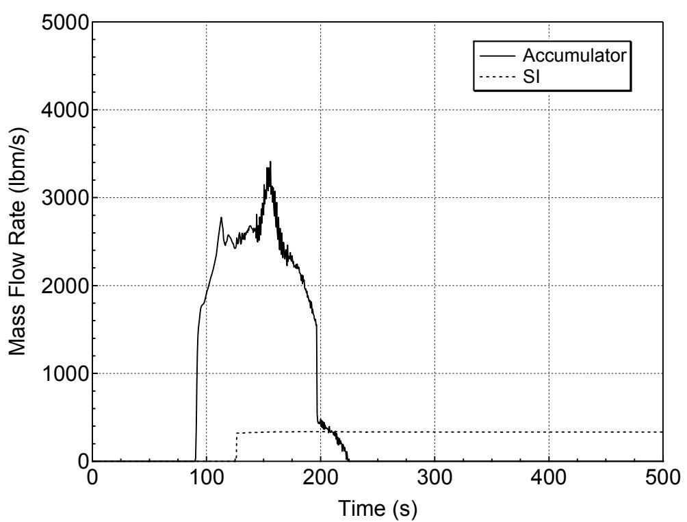
**Figure 5.3.2.c-22 Accumulator and Safety Injection Mass Flowrates
