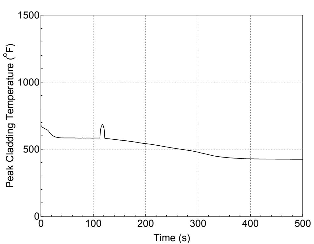
**Figure 5.3.1.e-17 PCT at All Elevations for Hot Rod in Hot Assembly
