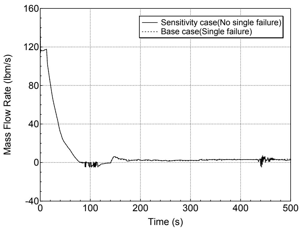
**Figure 5.6.1-12 Hot Assembly Exit Liquid Mass Flowrate for 7.5-inch Break (Top)
