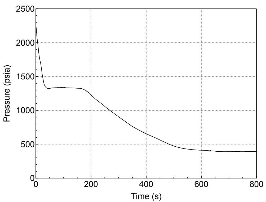
**Figure 5.3.1.b-19 RCS (Pressurizer) Pressure Transient for 6.5-inch Break (Side)
