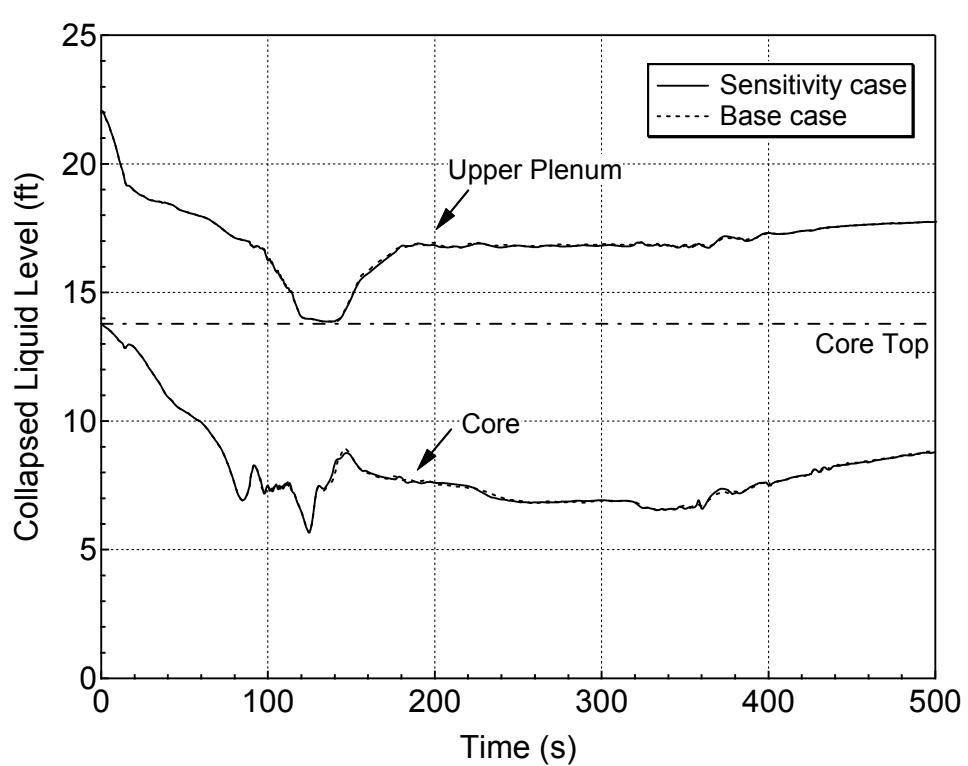
**Figure 5.5.a-9 Average Core and Upper Plenum Collapsed Levels
