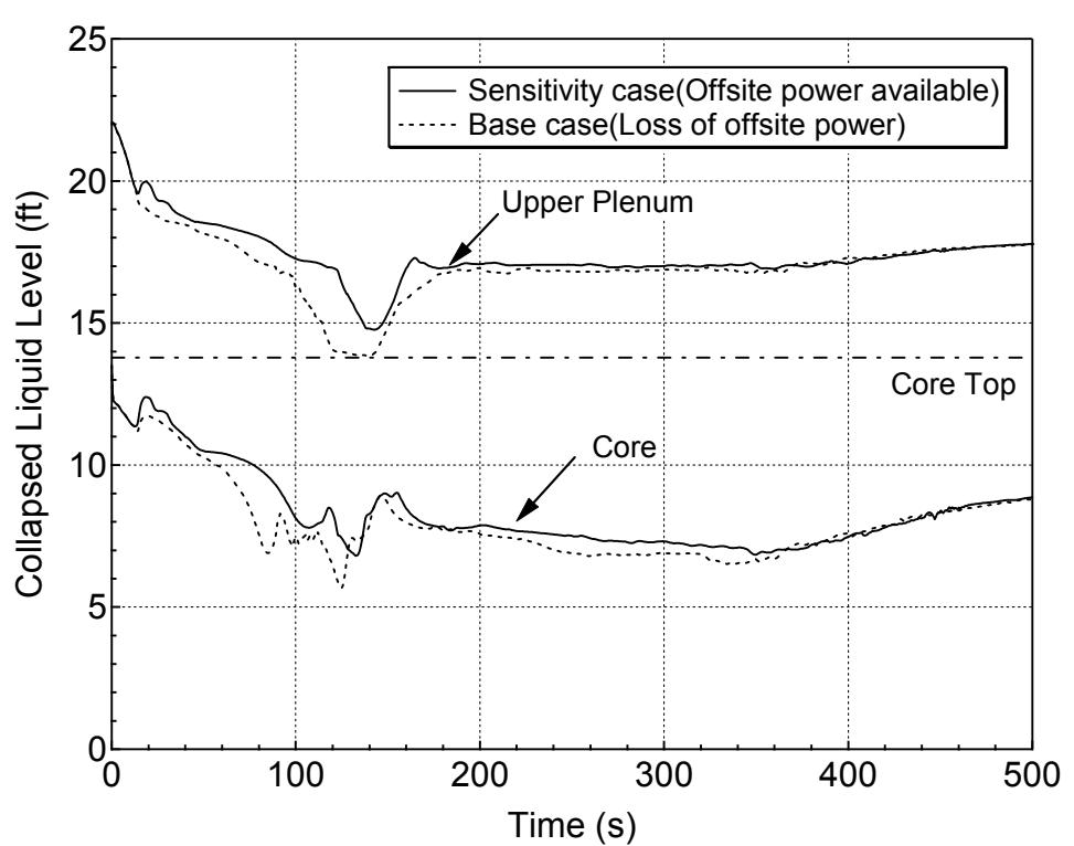
**Figure 5.6.2-10 Hot Assembly Core and Upper Plenum Collapsed Levels
