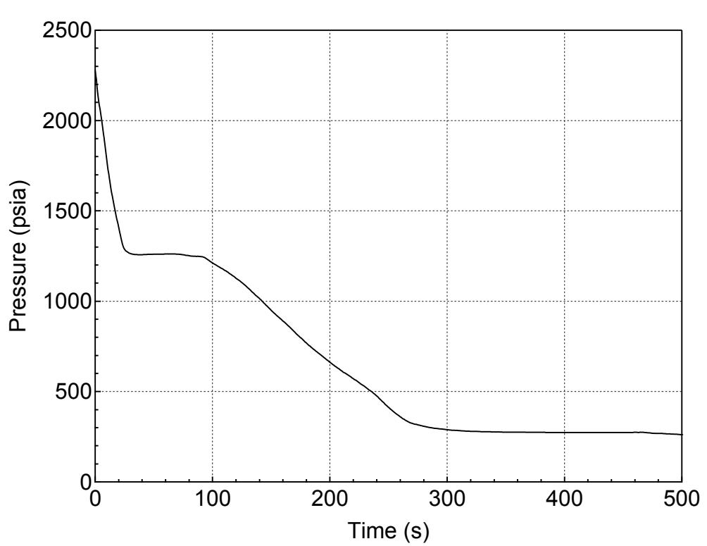
**Figure 5.2.i-1 RCS (Pressurizer) Pressure Transient for 9-inch Break (Bottom)
