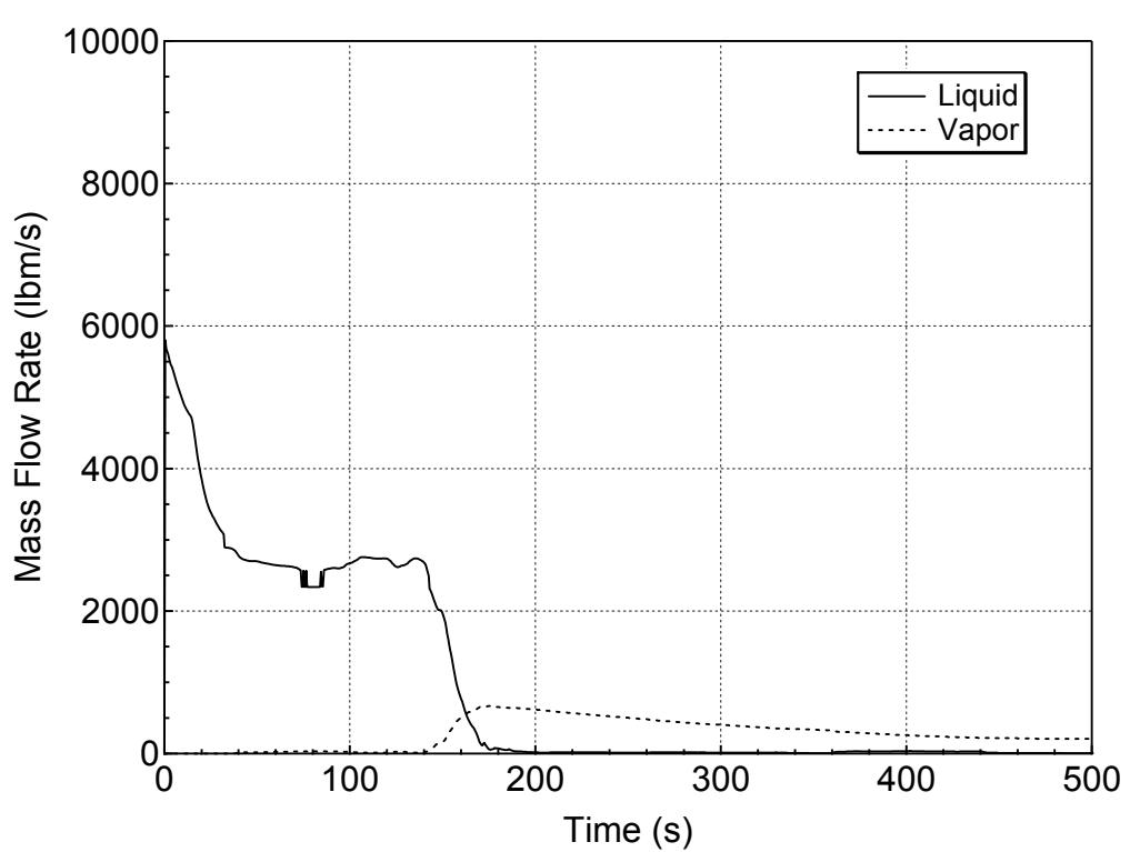
**Figure 5.3.1.c-21 Liquid and Vapor Discharges through the Break
