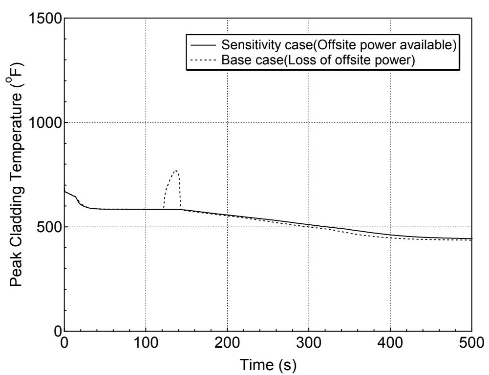
**Figure 5.6.2-11 PCT at All Elevations for Hot Rod in Hot Assembly
