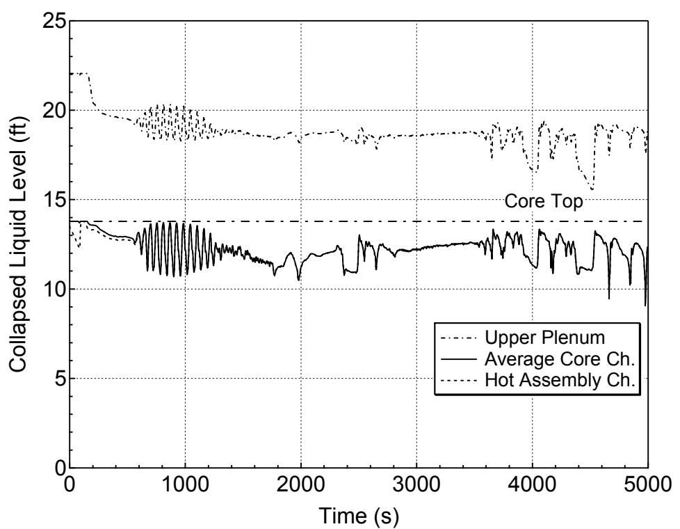
**Figure 5.1.1.c-7 Core and Upper Plenum Collapsed Levels for 2-inch Break (Bottom)
