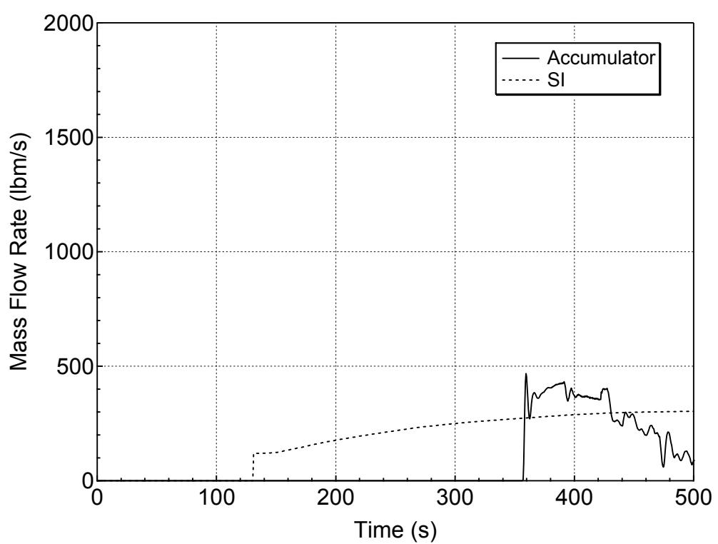
**Figure 5.3.1.c-22 Accumulator and Safety Injection Mass Flowrates
