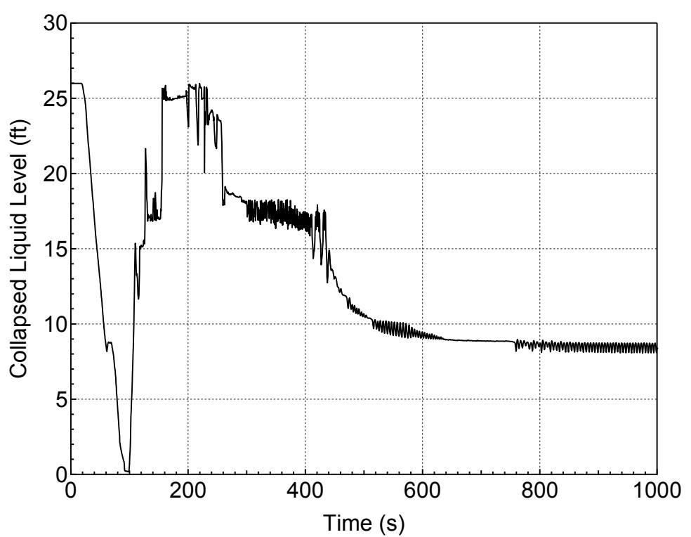
**Figure 5.1.1.b-15 Downcomer Collapsed Level for 1-ft<sup>2</sup> Break (Bottom)
