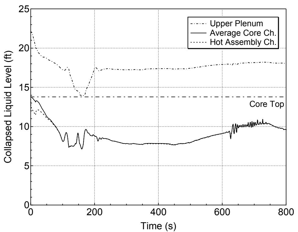
**Figure 5.3.1.b-34 Core and Upper Plenum Collapsed Levels
