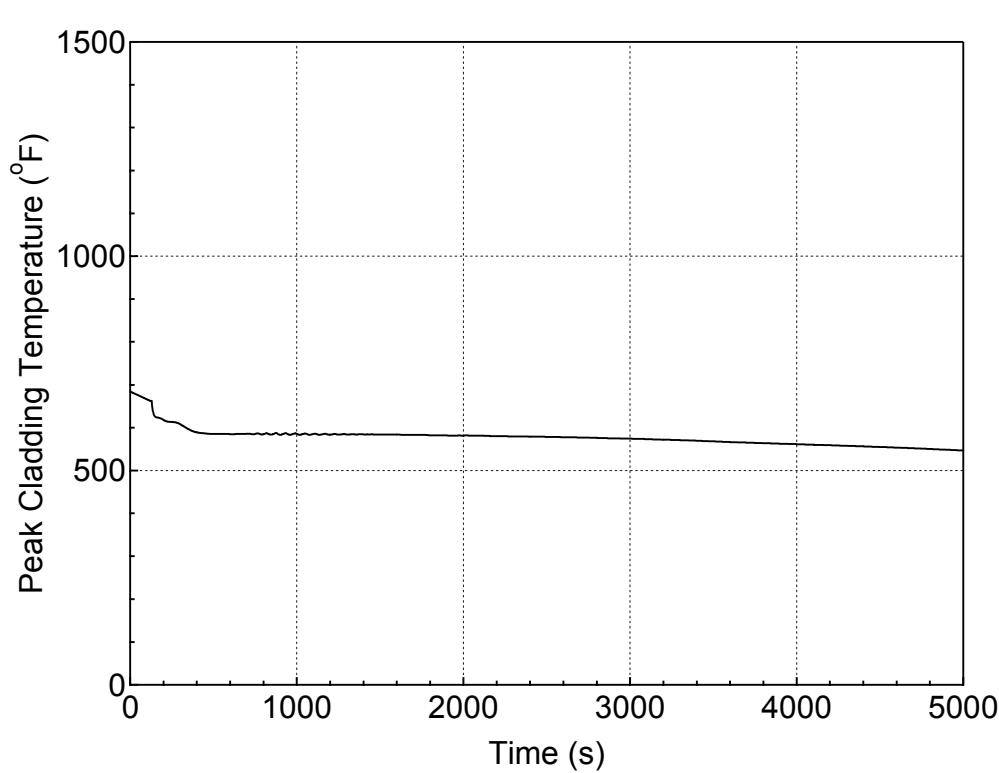
**Figure 5.1.1.b-8 PCT at All Elevations for Hot Rod in Hot Assembly
