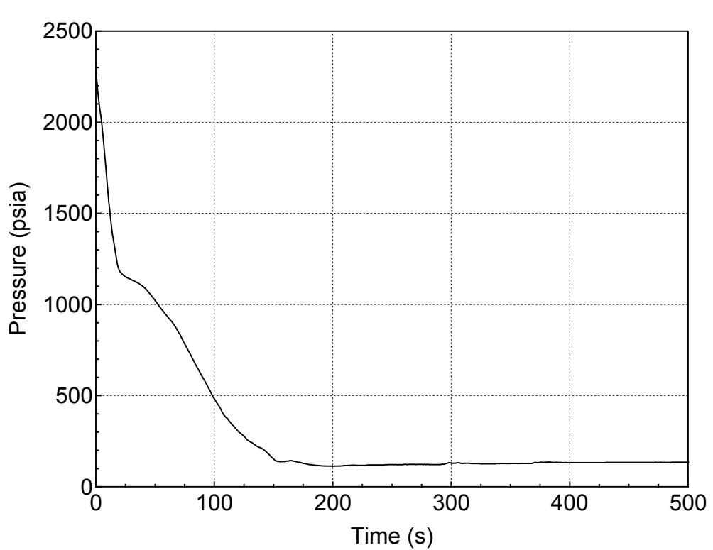
**Figure 5.3.2.c-1 RCS (Pressurizer) Pressure Transient for 1-ft<sup>2</sup> Break (Top)
