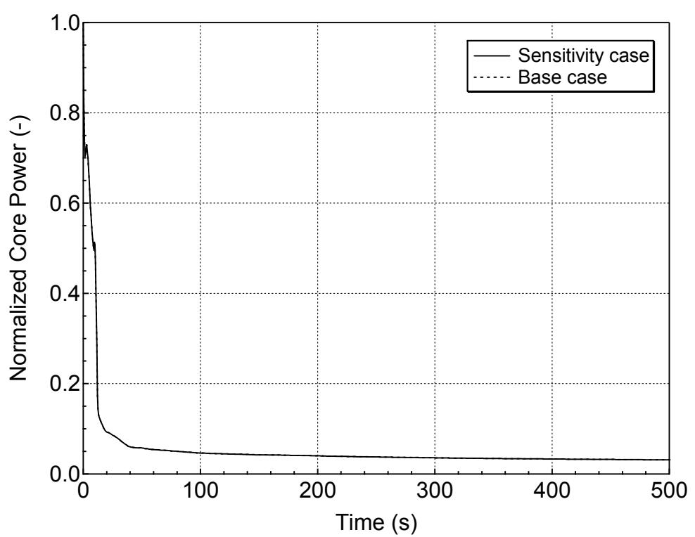
**Figure 5.5.b-2 Normalized Core Power for 1-ft<sup>2</sup> Break (Top)
