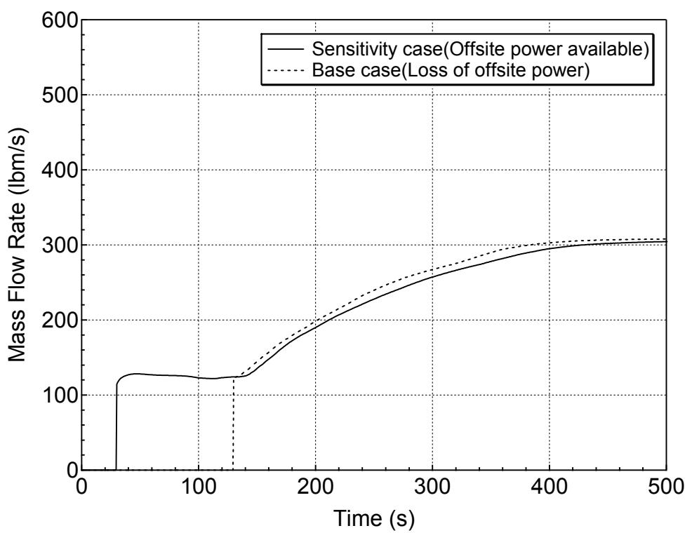
**Figure 5.6.2-6 Safety Injection Mass Flowrate for 7.5-inch Break (Top)
