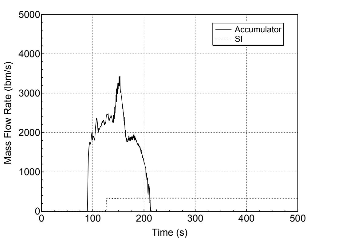
**Figure 5.3.2.c-4 Accumulator and Safety Injection Mass Flowrates for 1-ft<sup>2</sup> Break (Top)
