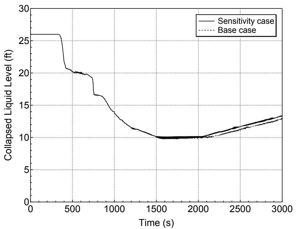
**Figure 5.5.c-8 Downcomer Collapsed Level for DVI-line Break
