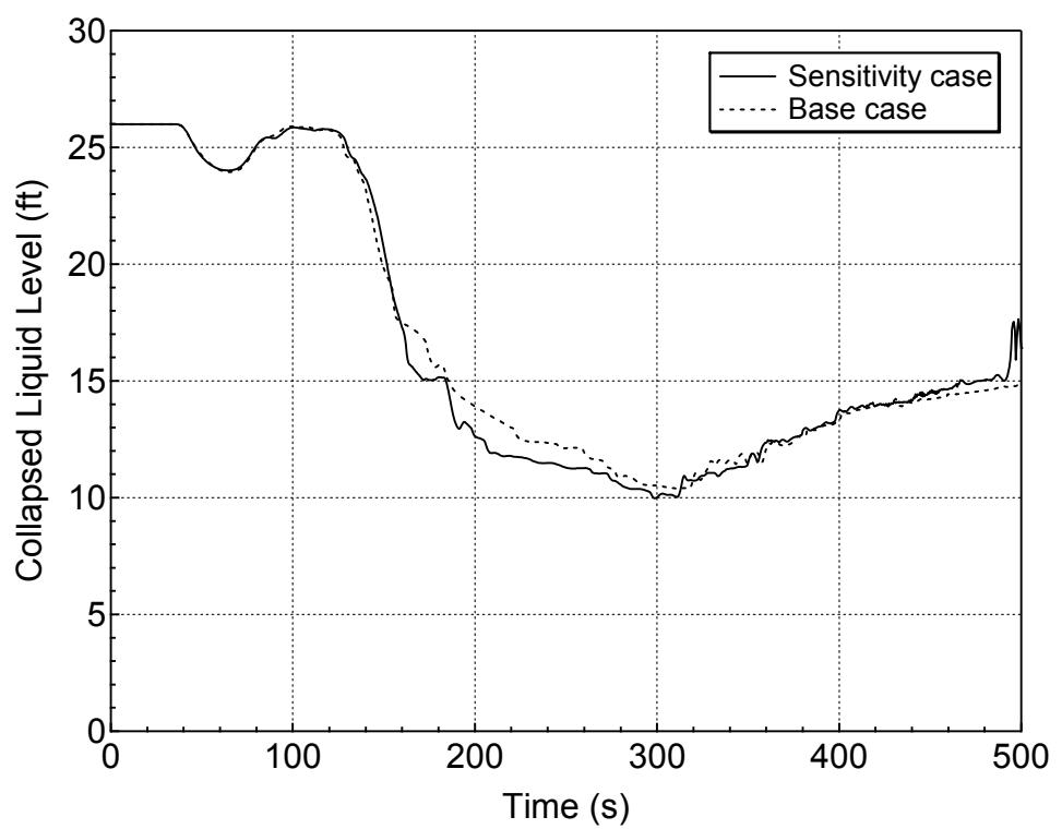
**Figure 5.4.2-8 Downcomer Collapsed Level for 7.5-inch Break (Top)
