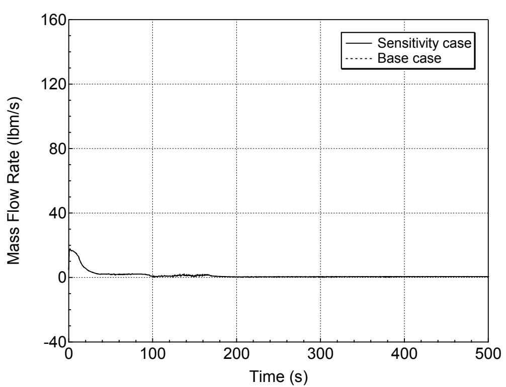
**Figure 5.5.b-13 Hot Assembly Exit Vapor Mass Flowrate for 1-ft<sup>2</sup> Break (Top)
