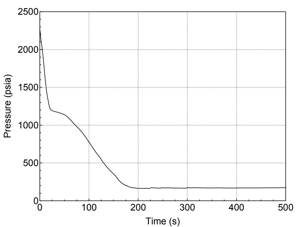
**Figure 5.3.2.a-1 RCS (Pressurizer) Pressure Transient for 12-inch Break (Top)
