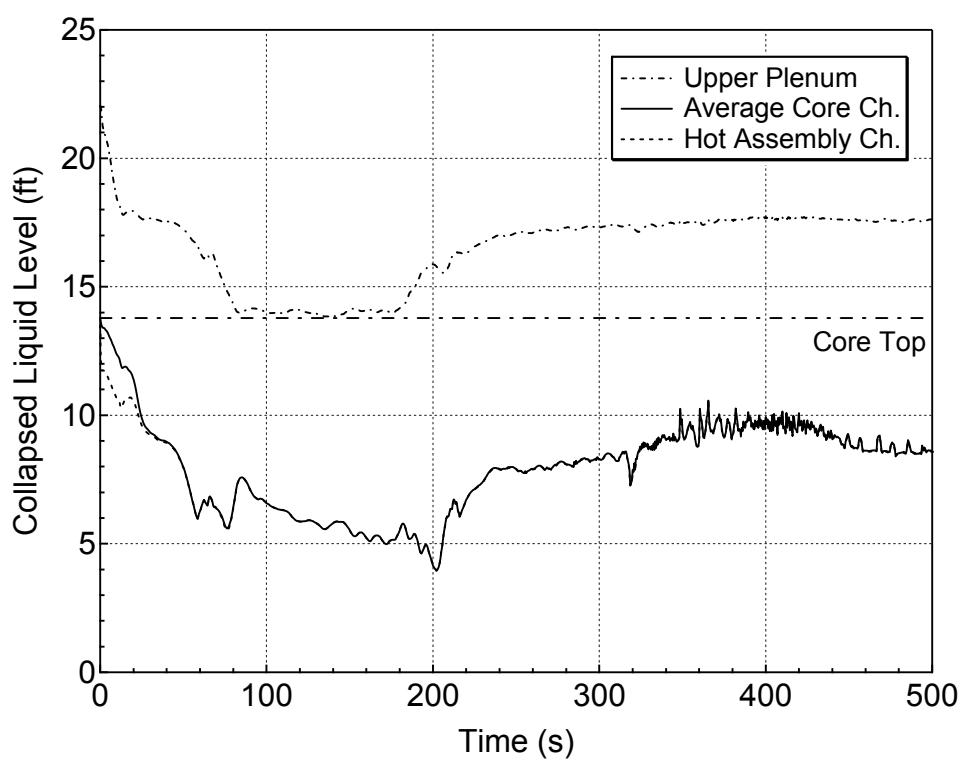
**Figure 5.2.j-7 Core and Upper Plenum Collapsed Levels for 10-inch Break (Bottom)
