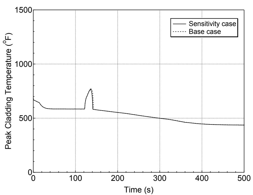
**Figure 5.5.a-11 PCT at All Elevations for Hot Rod in Hot Assembly
