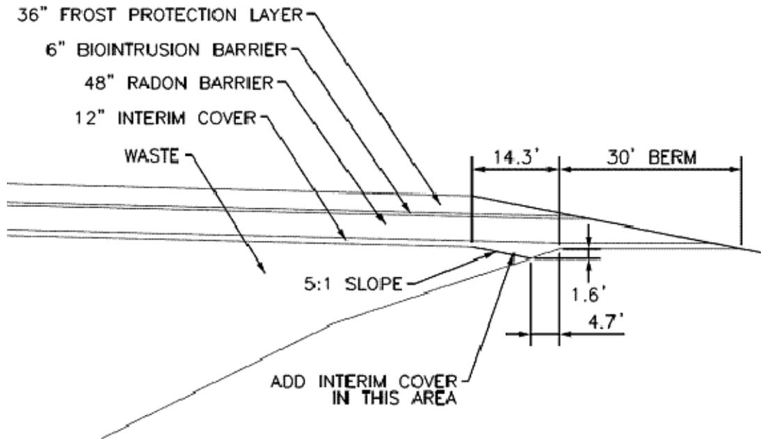
Figure D. Edge Strip Removal and Replacement
