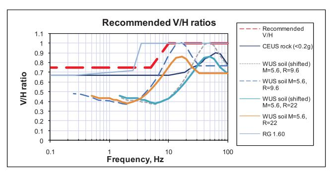
V/H ratios for CEUS rock, WUS soil (for M 5.6 and two distances), for WUS soil with frequency shifted (for M5.6 and two distances), and recommended V/H ratio. Distances, R, are in km. Equivalent distances in miles are: 9.6 km (6 mi); 22 km (13.7 mi).
