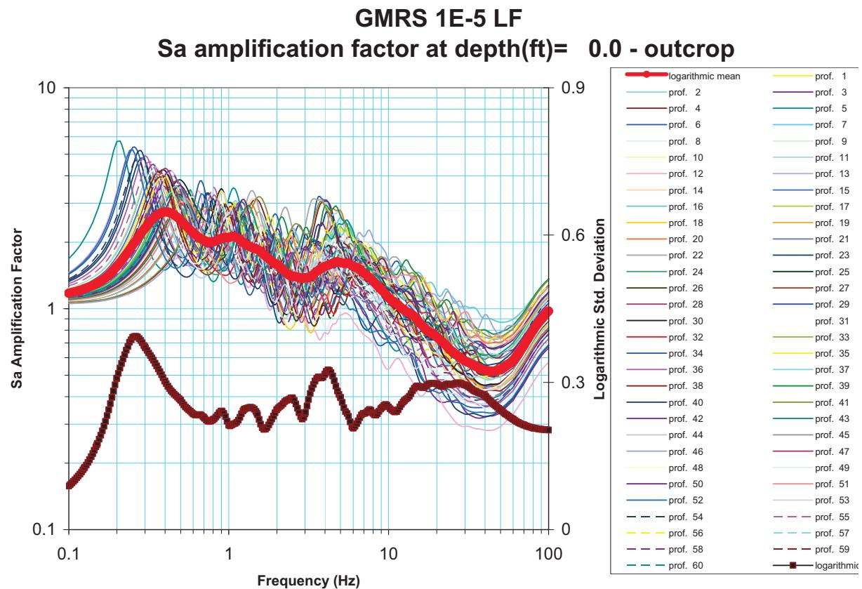
Amplification Factors (Left Y Axis) and Associated Logarithmic Standard Deviation (Right Y Axis) Calculated with the 60 Synthetic Profiles, for the 10-5 Low-Frequency Rock Input
