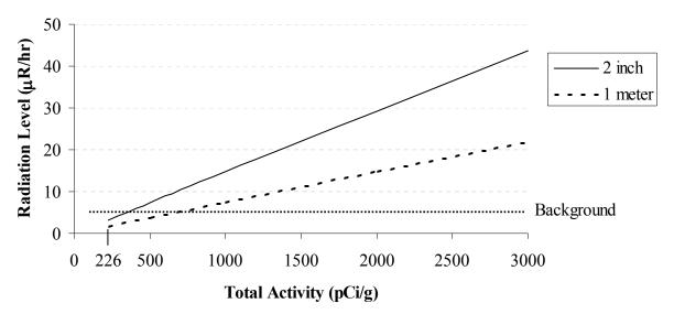
The radiation levels in the figure above at a distance of 2 inches and at a distance of one meter were based on a MicroShield<sup>©</sup> model that assumed a soil density of 1.69 grams per cubic centimeter; a container wall thickness of  $\frac{3}{8}$  inch; the expected median concentration in the first case; and the median concentration scaled to the USEI WAC in the second case.
