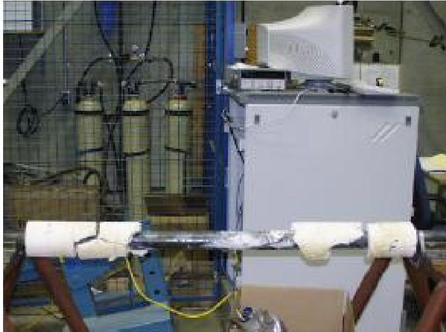
Figure 14.1 - OPG 5D Test Target Post-Destruction (Jacketing Removed) (Figure D4 in Ref. 5)
