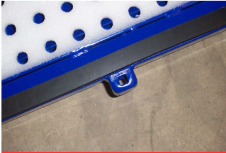
Figure 8-4 Refurbished inner container lid showing welded components
