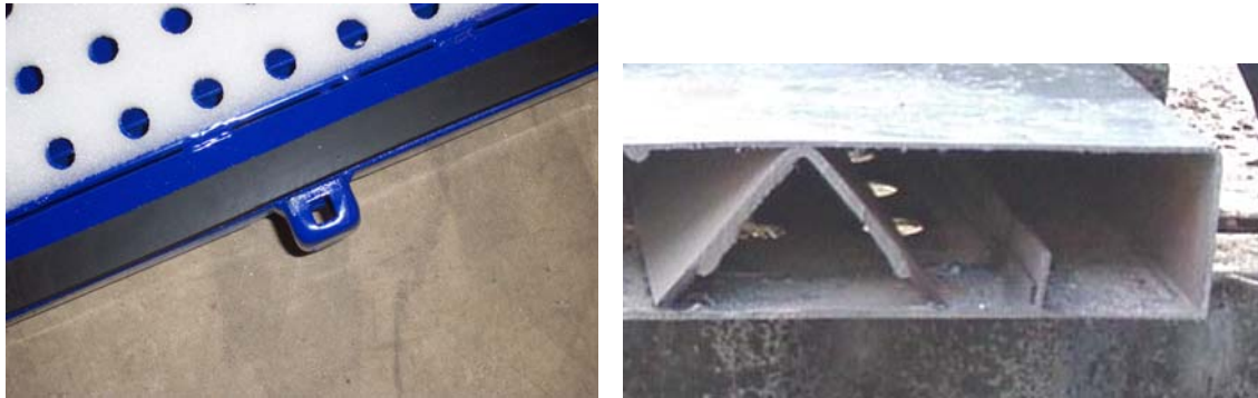
Figure 1: Refurbished (right) and unrefurbished inner containers showing welded components
