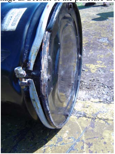
Puncture Impact Damage – No Opening
