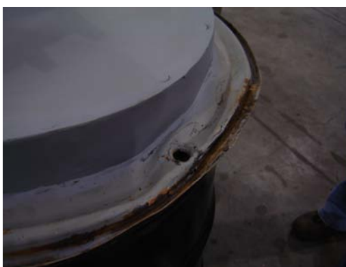
View of Damage to Top Closure
