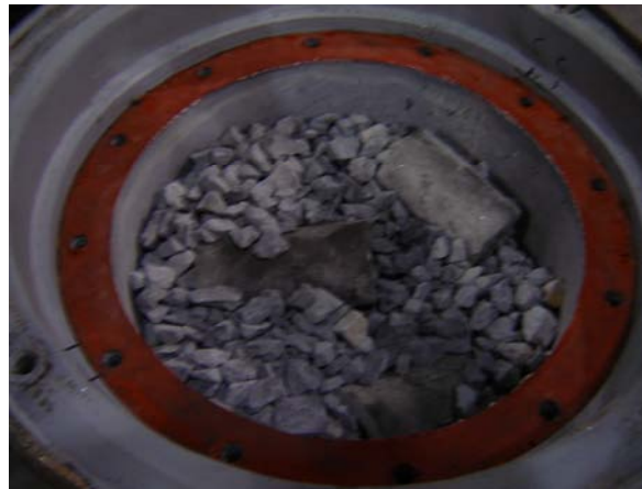
Containment Loaded With 254-1/2 Pounds of Loose Gravel
