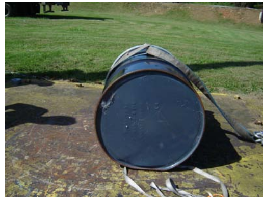
End View – Bottom End Damage
