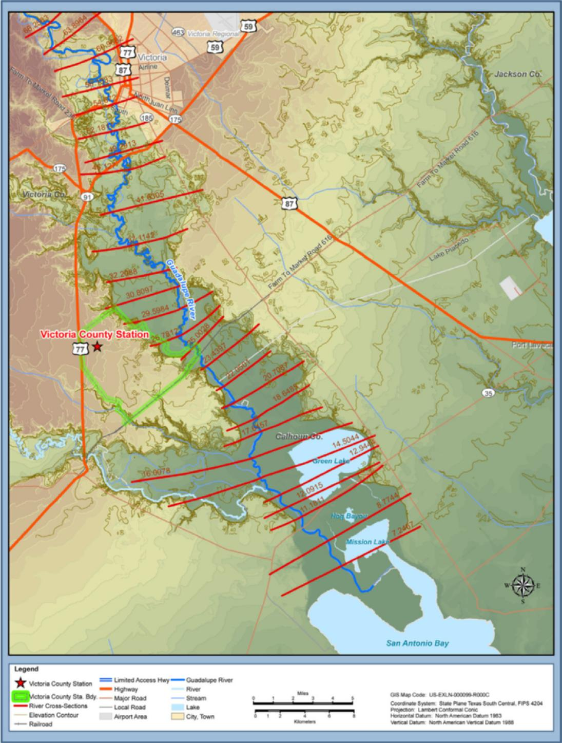
Figure 2.4.5-9 Locations of River Cross Sections Used in the HEC-RAS Model of the Guadalupe River
