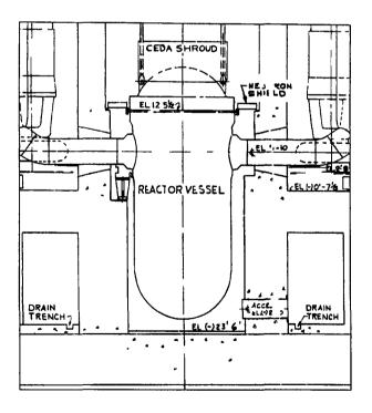
Figure 1: General Arrangement of Reactor Pressure Vessel Area
