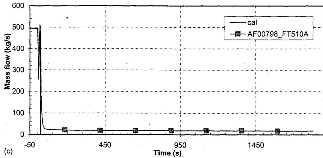
Figure 39 Feedwater flow SG 1—turbine governor valve closure with reactor trip
