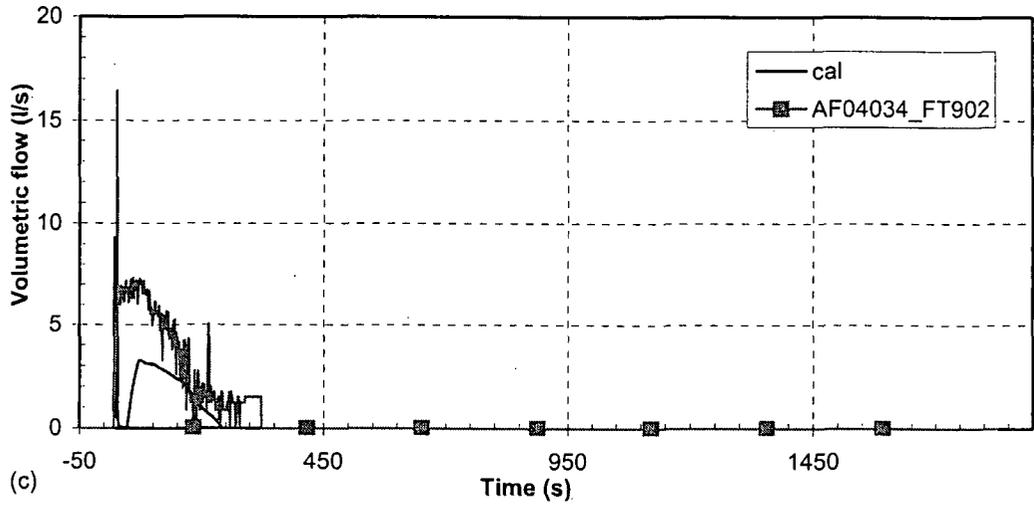
Figure 42 SI 2 volumetric flow—turbine governor valve closure with reactor trip
