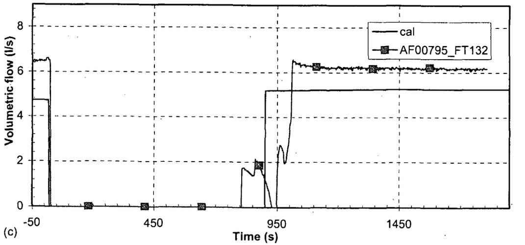
Figure 32 Letdown flow—turbine governor valve closure with reactor trip
