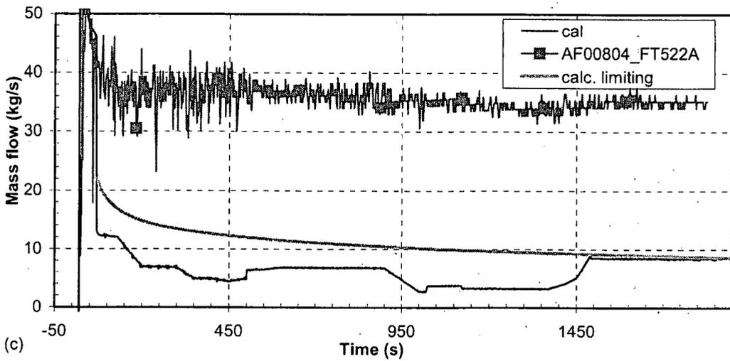
Figure 38 Steamflow SG 2—turbine governor valve closure with reactor trip
