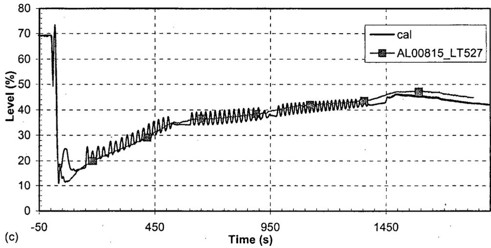
Figure 36 SG 2 narrow range level—turbine governor valve closure with reactor trip
