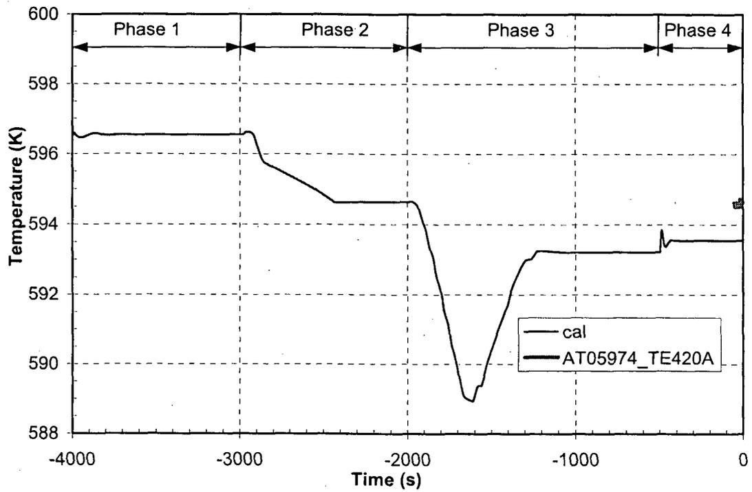
Figure 9 Hot leg loop 2 temperature—testing of turbine governor valve
