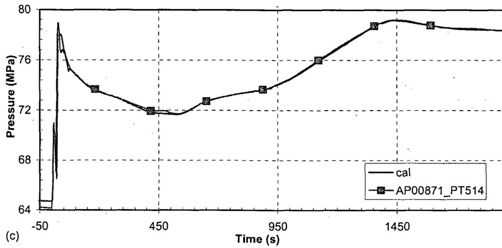
Figure 33 SG 1 pressure—turbine governor valve closure with reactor trip
