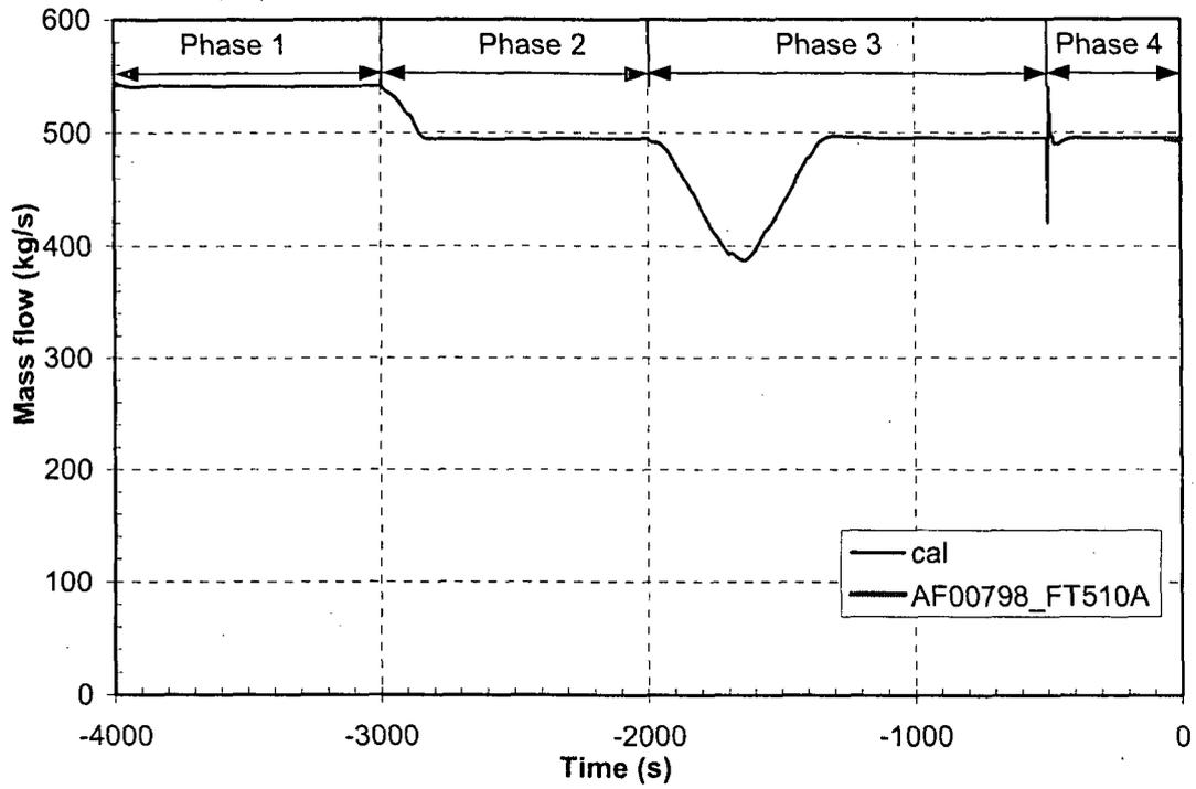
Figure 20 Feedwater flow SG 1 testing of turbine governor valve
