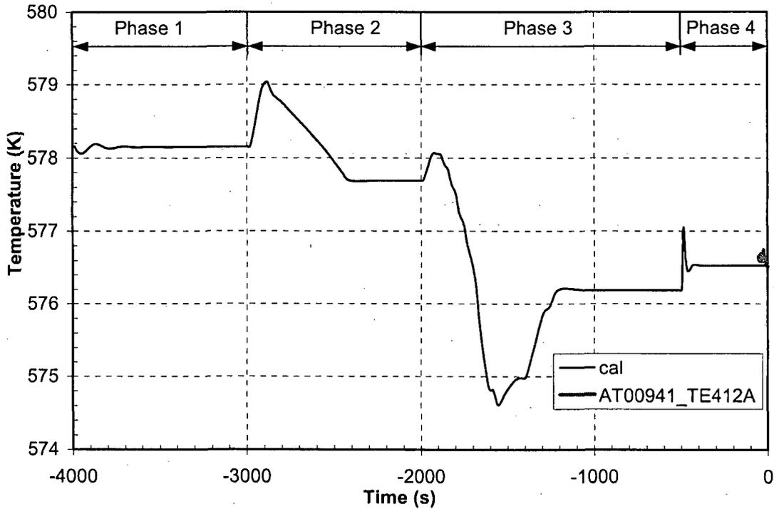
Figure 10 RCS average temperature—testing of turbine governor valve
