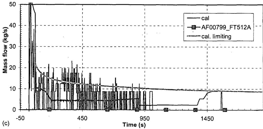
Figure 37 Steamflow SG 1—turbine governor valve closure with reactor trip
