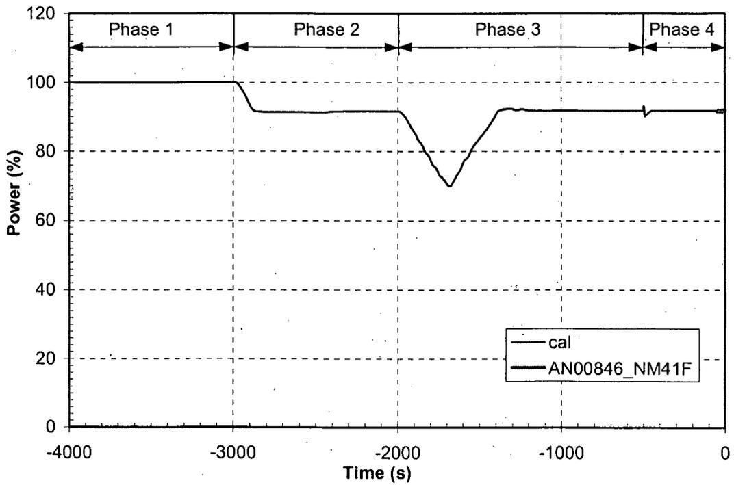
Figure 2 Core power—testing of turbine governor valve
