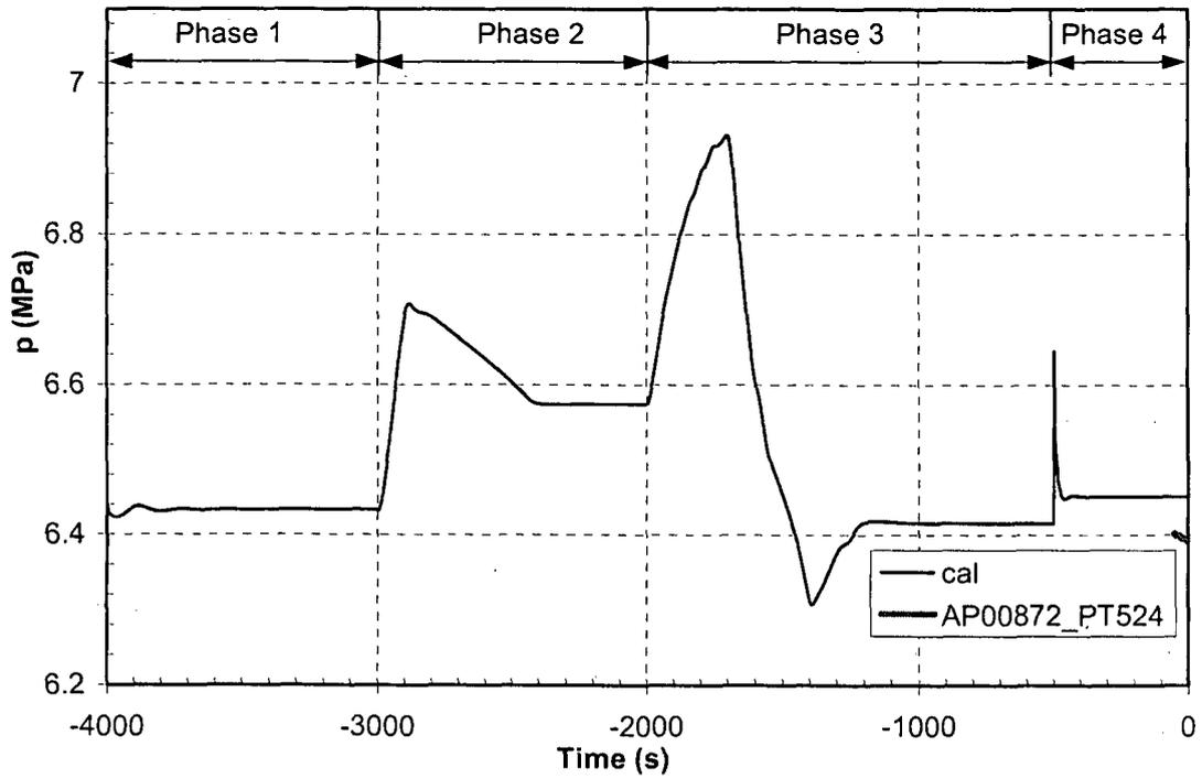
Figure 17 SG 2 pressure—testing of turbine governor valve
