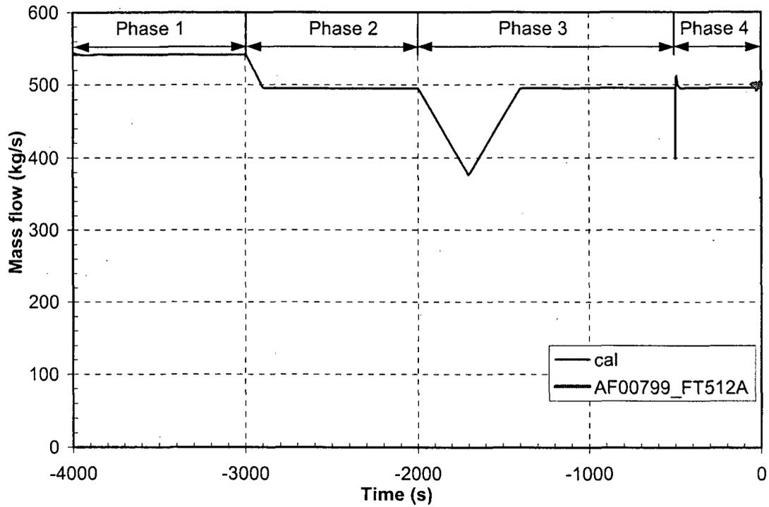
Figure 18 Steamflow SG 1—testing of turbine governor valve
