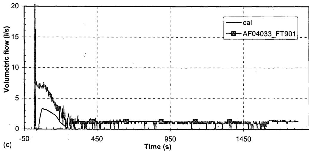
Figure 41 SI 1 volumetric flow—turbine governor valve closure with reactor trip
