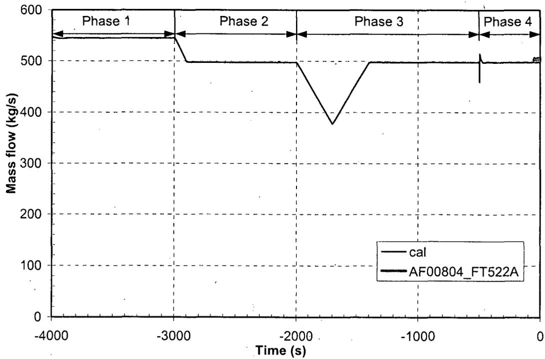
Figure 19 Steamflow SG 2—testing of turbine governor valve
