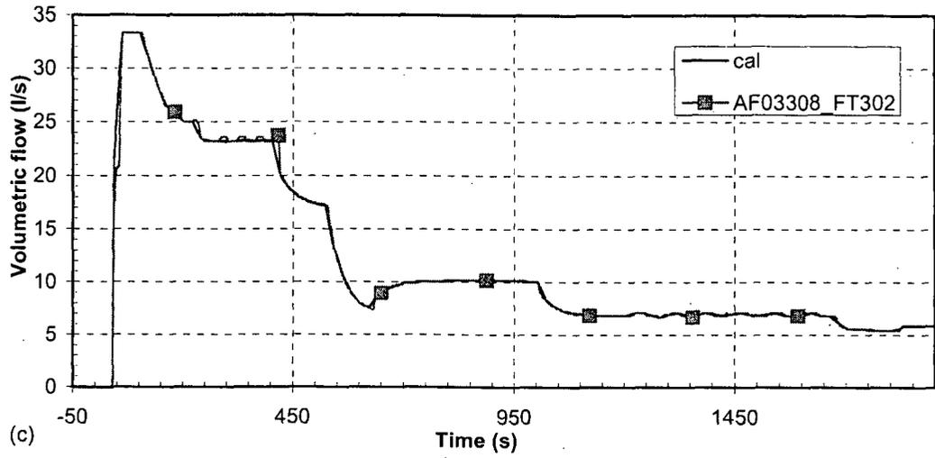
Figure 43 AFW 1 volumetric flow—turbine governor valve closure with reactor trip
