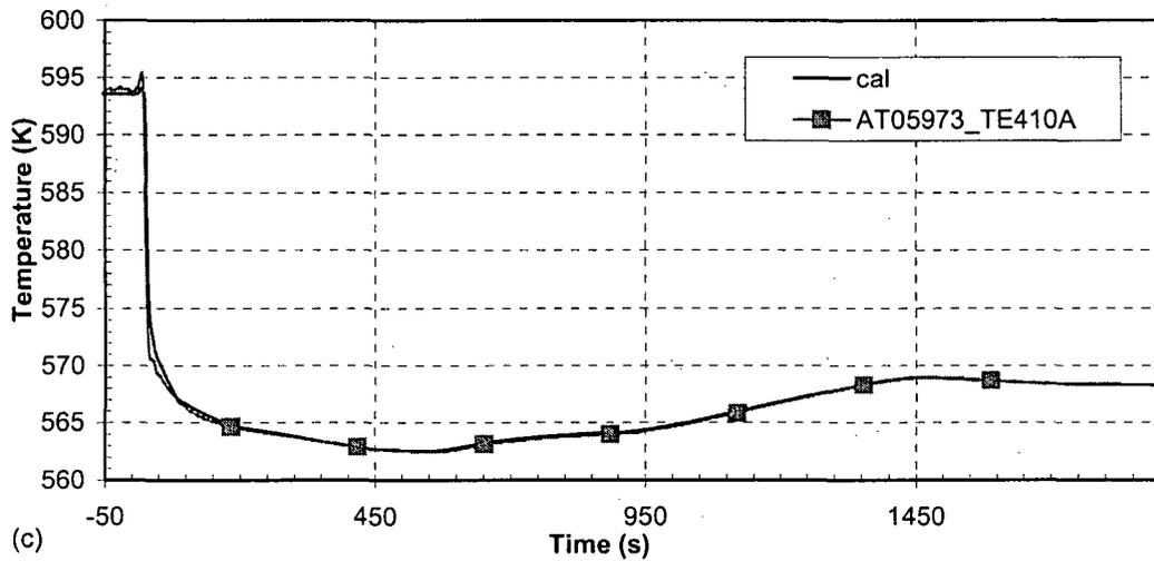
Figure 25. Hot leg loop 1 temperature—turbine governor valve closure with reactor trip
