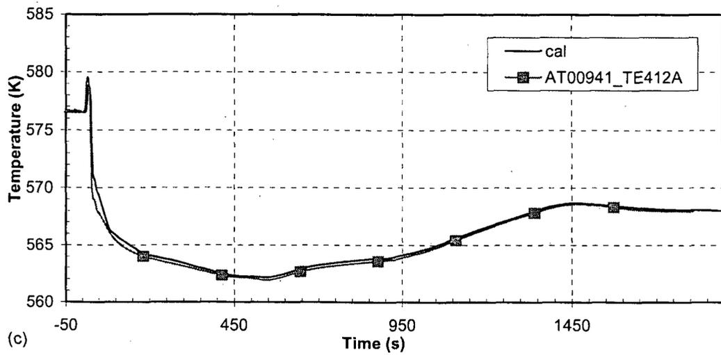
Figure 27 RCS average temperature—turbine governor valve closure with reactor trip
