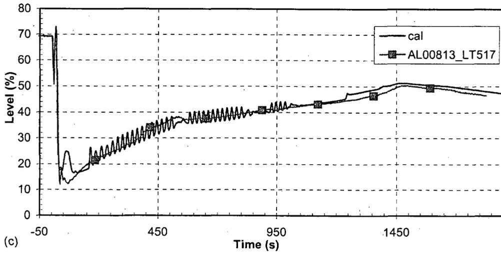
Figure 35 SG 1 narrow range level—turbine governor valve closure with reactor trip
