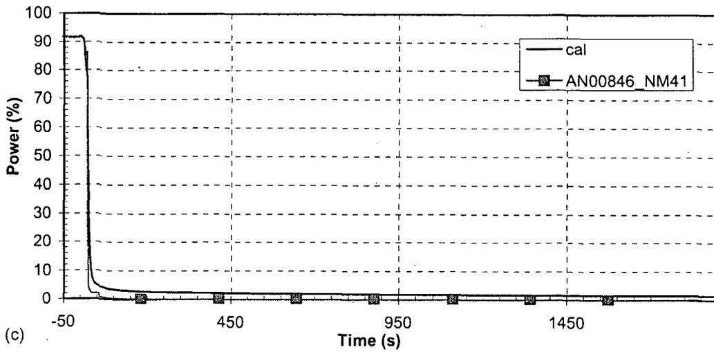
Figure 22 Core power—turbine governor valve closure with reactor trip
