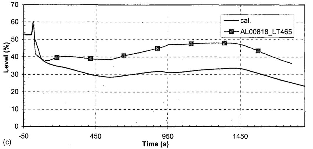
Figure 30 PRZ level—turbine governor valve closure with reactor trip
