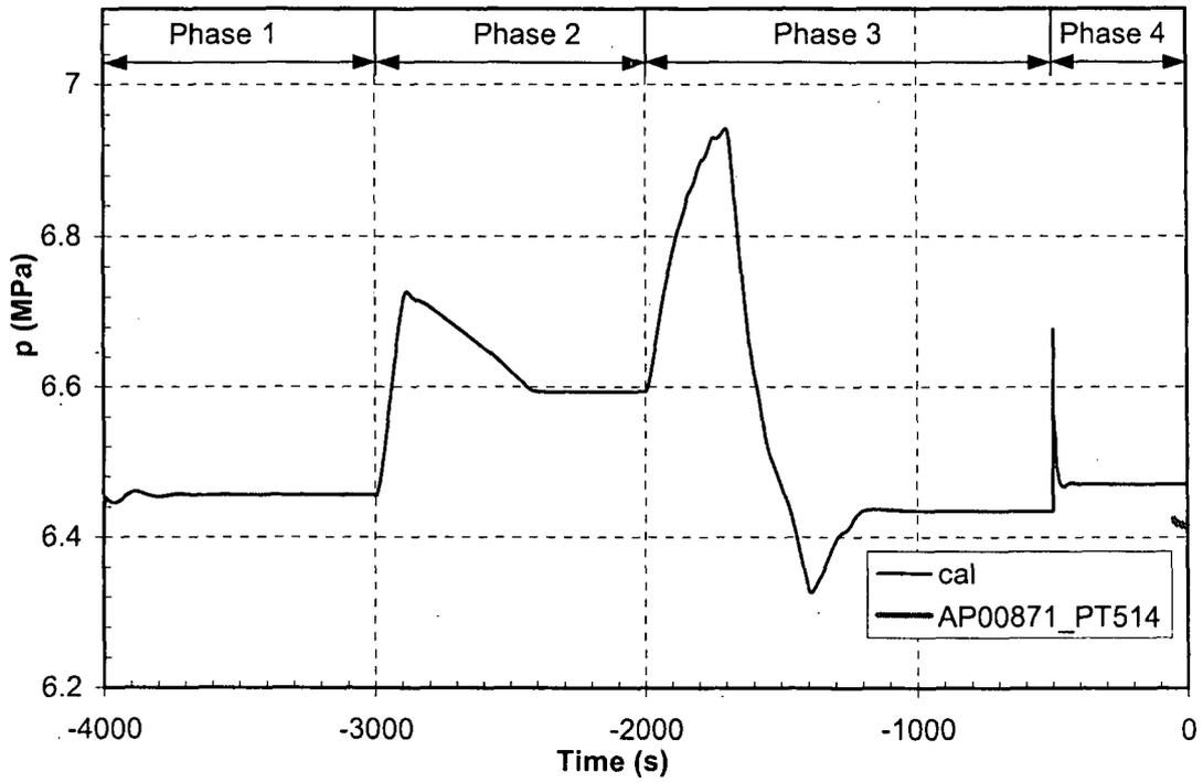
Figure 16 SG 1 pressure—testing of turbine governor valve
