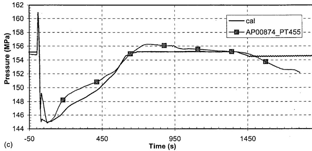
Figure 29 PRZ pressure—turbine governor valve closure with reactor trip
