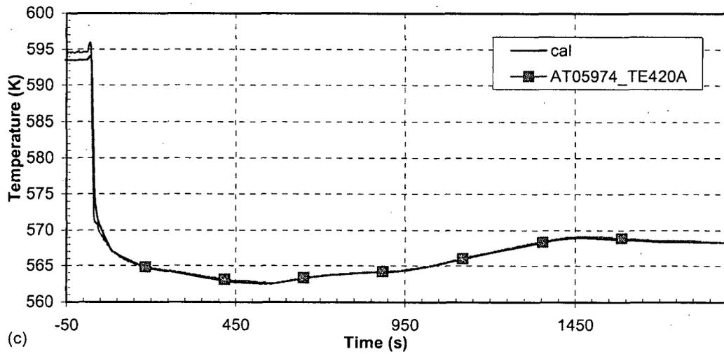
Figure 26 Hot leg loop 2 temperature—turbine governor valve closure with reactor trip
