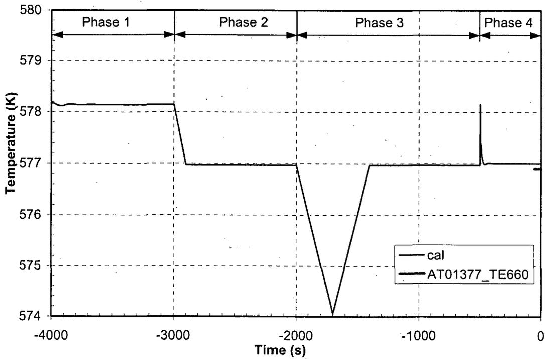
Figure 11 Reference (programmed) temperature—testing of turbine governor valve
