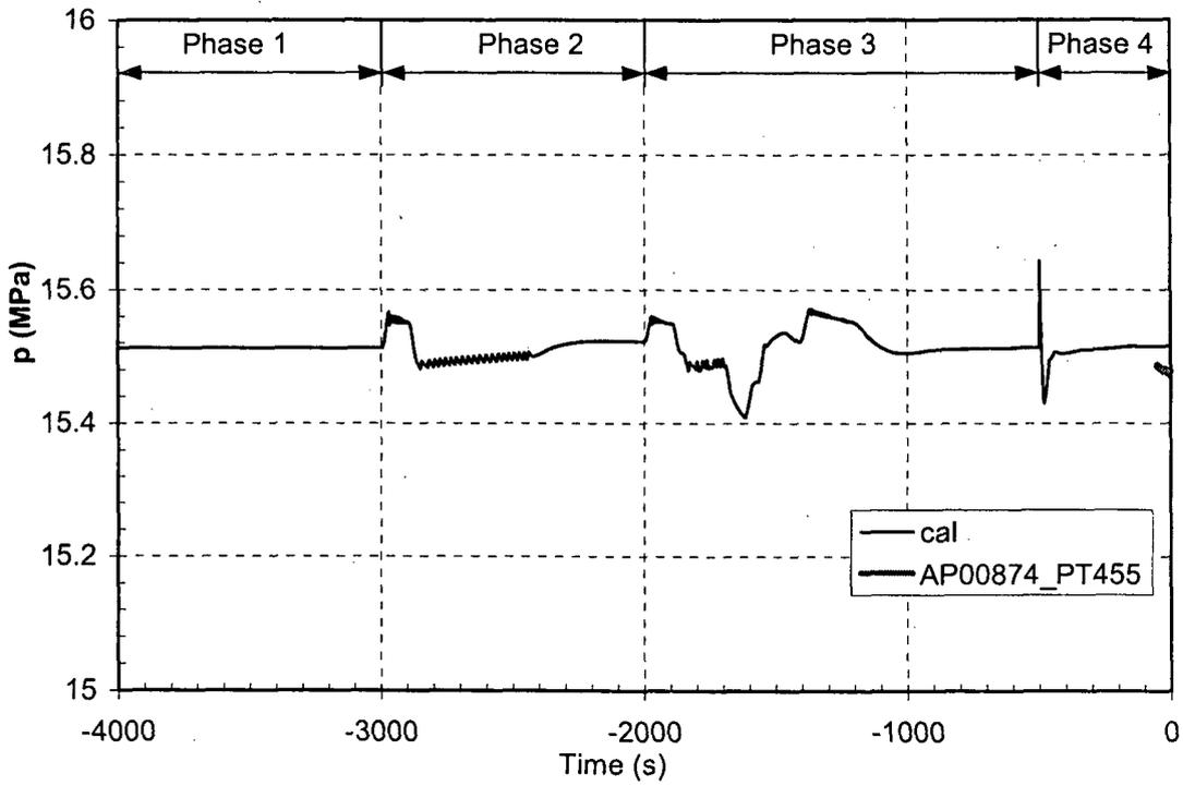
Figure 12 PRZ pressure—testing of turbine governor valve
