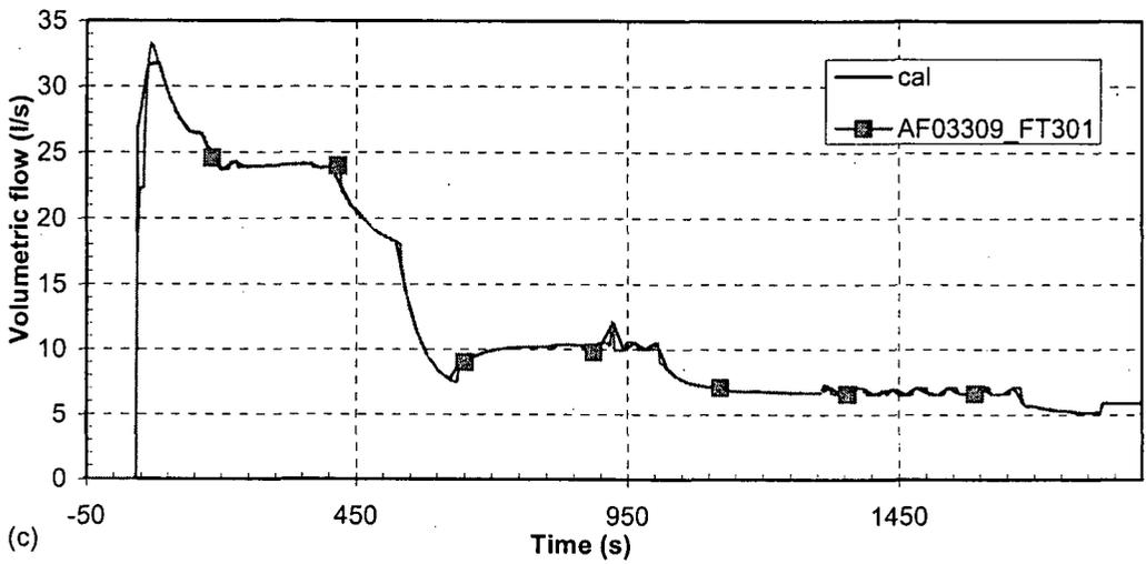
Figure 44 AFW 2 volumetric flow—turbine governor valve closure with reactor trip
