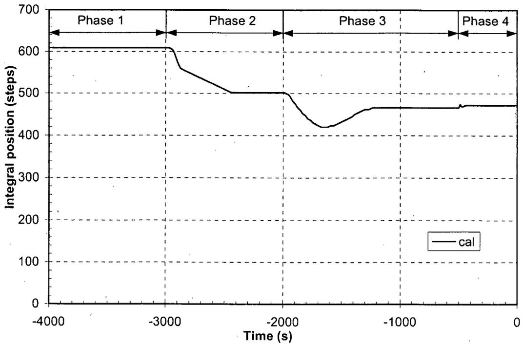
Figure 3 Rod position—testing of turbine governor valve
