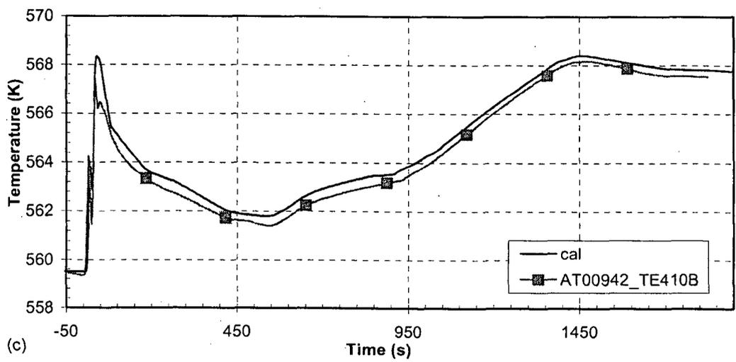
Figure 23 Cold leg loop 1 temperature—turbine governor valve closure with reactor trip
