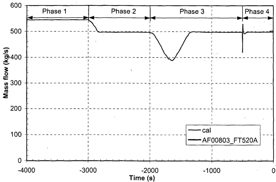
Figure 21 Feedwater flow SG—testing of turbine governor valve
