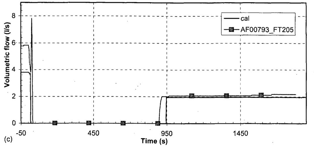
Figure 31 Charging flow—turbine governor valve closure with reactor trip
