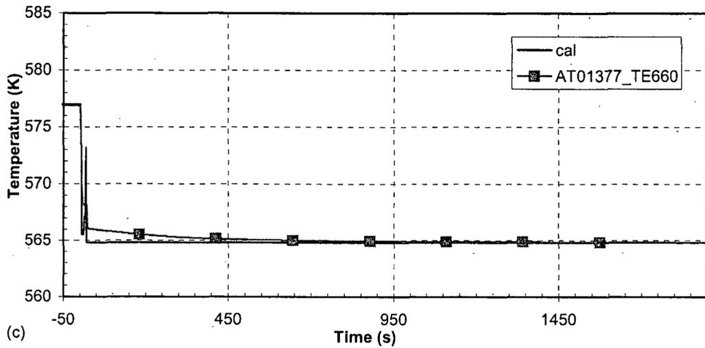
Figure 28 Reference temperature—turbine governor valve closure with reactor trip
