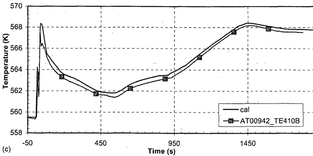
Figure 24 Cold leg loop 2 temperature—turbine governor valve closure with reactor trip
