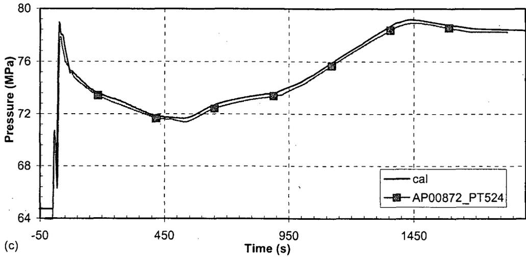
Figure 34 SG 2 pressure—turbine governor valve closure with reactor trip
