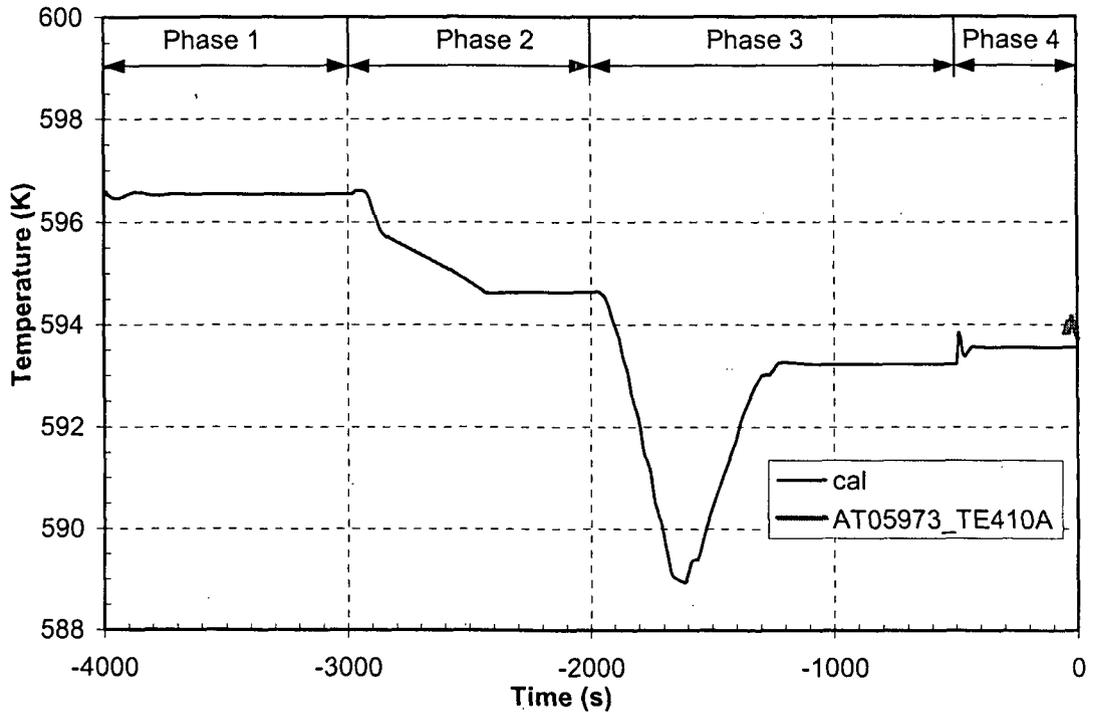
Figure 8 Hot leg loop 1 temperature—testing of turbine governor valve
