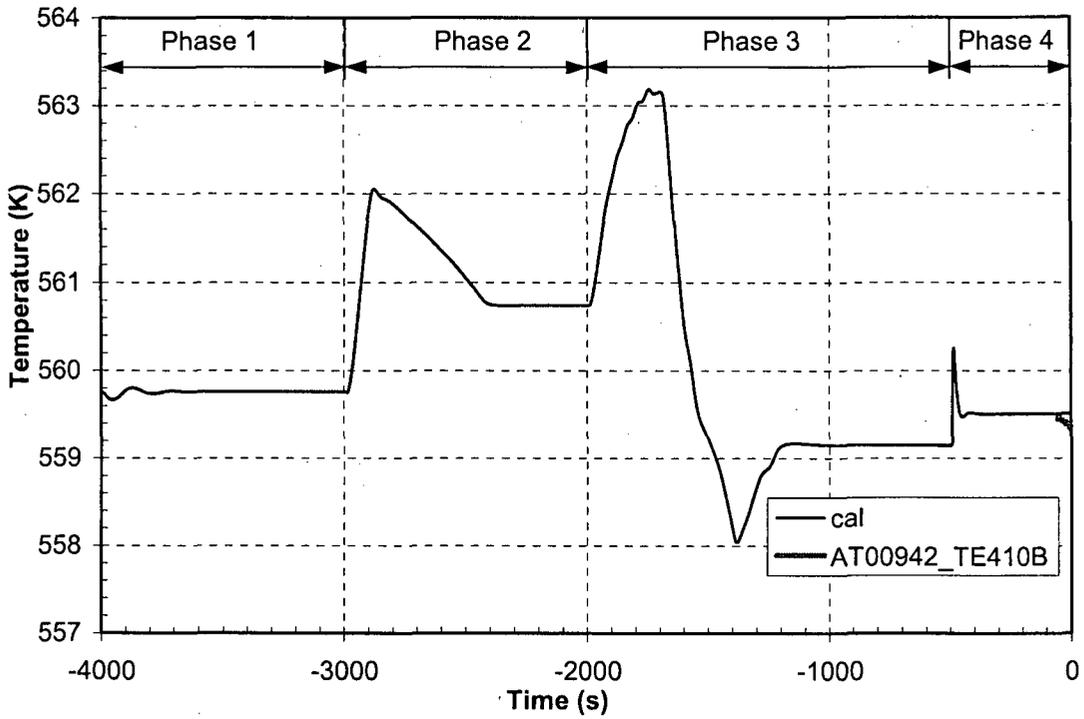
Figure 6 Cold leg loop 1 temperature—testing of turbine governor valve
